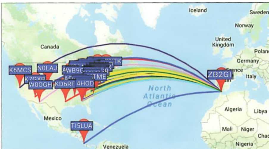
Fig. 6: Results of ZB2GI 20m WSPR transmissions on February 21 at 2100-2200UTC.
