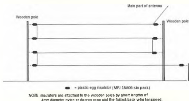
Fig. 3: Using wooden poles to support fold-back capacitive loading using a single length of wire.
