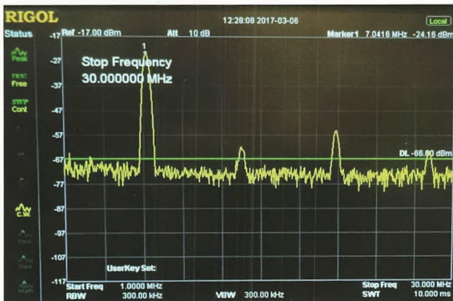
Fig. 5: The harmonics at 14, 21 and 28MHz are still clearly seen even with the use of an ATU.
