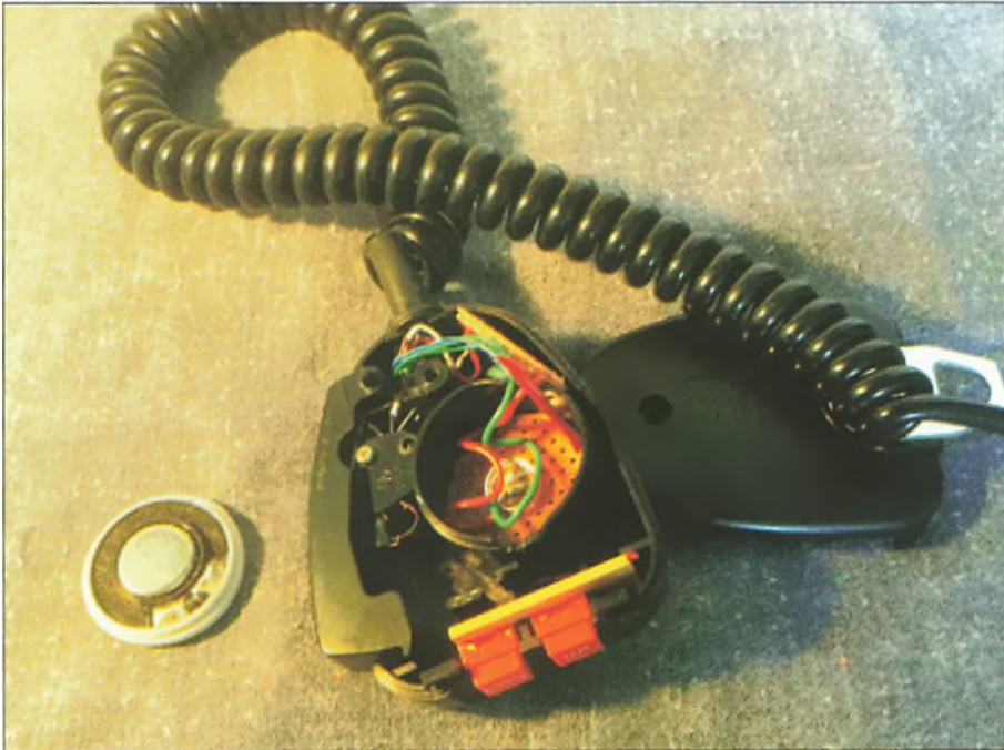
Fig. 4: The rewired microphone with the original speaker insert.
