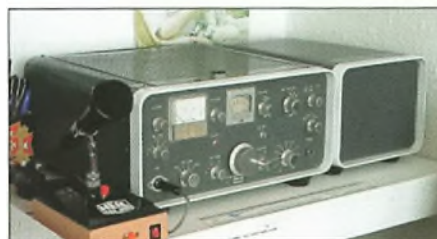
Fig. 1: The author's KW2000A with associated power supply/loudspeaker.
