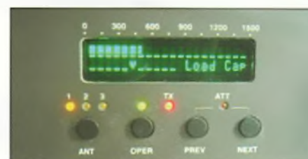
Fig. 5: The 'TRI' in use. (a) The arrow indicates that the Load Capacitor needs to be turned to the left. (b) The arrow changes to a 'v' in the centre of the display when the load is correctly adjusted.
