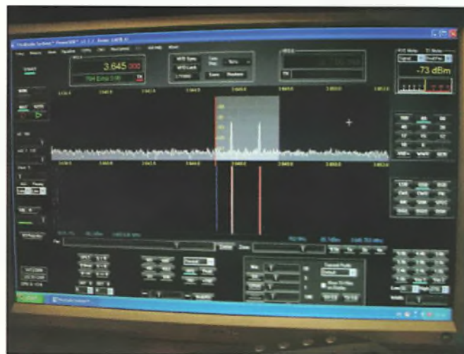
Fig. 7: The waterfall display of a two-tone test. In this screenshot the USB transmitted signal is modulated by a two-tone test oscillator and it can be seen that there are no stray signals outside the two tones.
