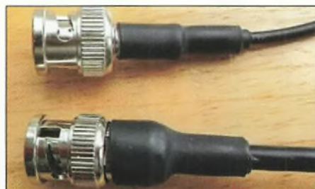
Fig.4: Fitting RG174 into a crimped BNC plug, requires it to be finished off with a strain relief application of heatshrink tubing. Compare this with the lower clamped RG58 type.
