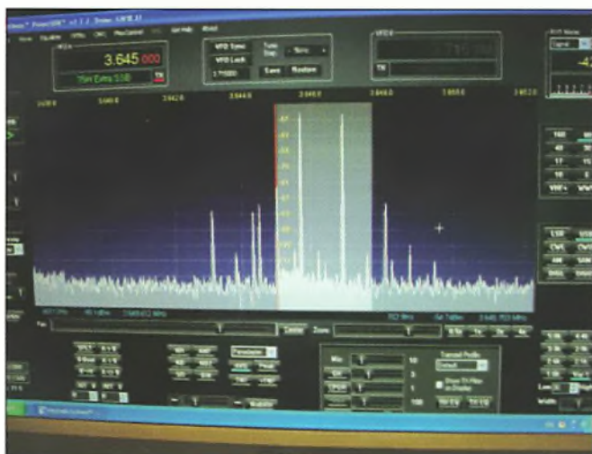
Fig. 8: Incorrect setup of a transmitter with the IMD created by over-modulation or non-linearity.
