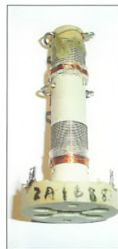
Fig. 2: Original coils just visible at the bottom of each main coil and wound over the main windings.
