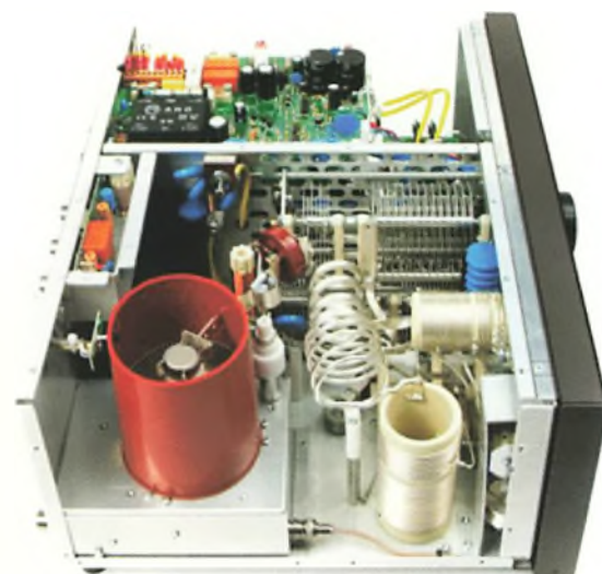
Fig. 2: The Acom 1500 uses a single 4CX100A ceramic valve (bottom left, surrounded by red 'chimney'). (Photo courtesy Acom)
