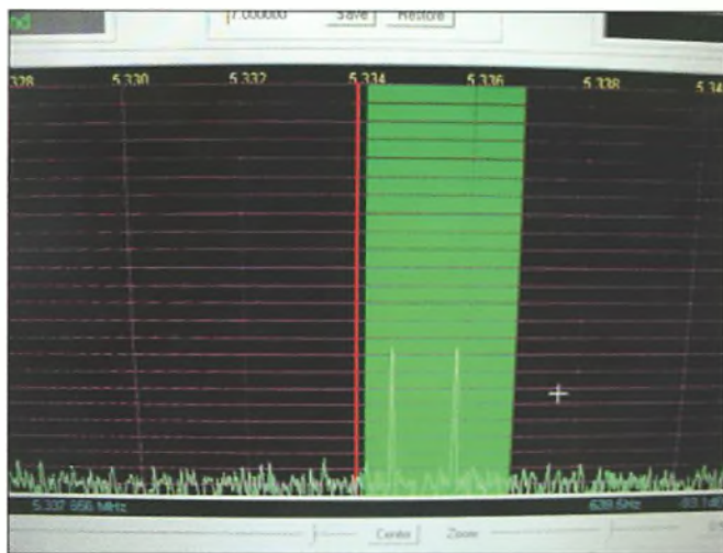
Fig. 6: SDR display of a USB transmission modulated by a two-tone generator. The graduations are 6dB each.
