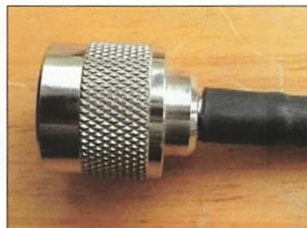
Fig 5: A suitable N-type plug, crimped onto RG58 with its heatshrink strain relief fitted.
