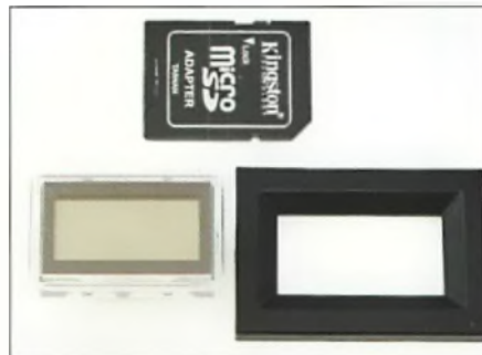
Fig. 6: Miniature digital panel meter and bezel from muRata (The SD card is just for scale).
