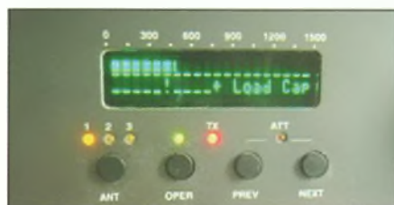
Fig. 5: The 'TRI' in use. (a) The arrow indicates that the Load Capacitor needs to be turned to the left. (b) The arrow changes to a 'v' in the centre of the display when the load is correctly adjusted.
