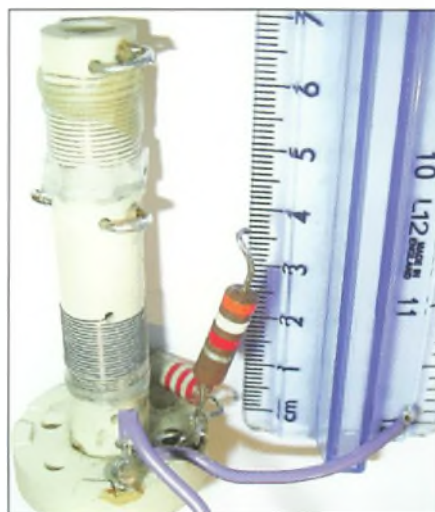
Fig. 2: Original coils just visible at the bottom of each main coil and wound over the main windings.
