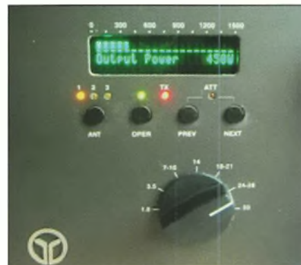
Fig. 4: Close-up of the vacuum fluorescent display, in this case indicating the Output Power of 450W. As can be seen, there is a lot in reserve.
