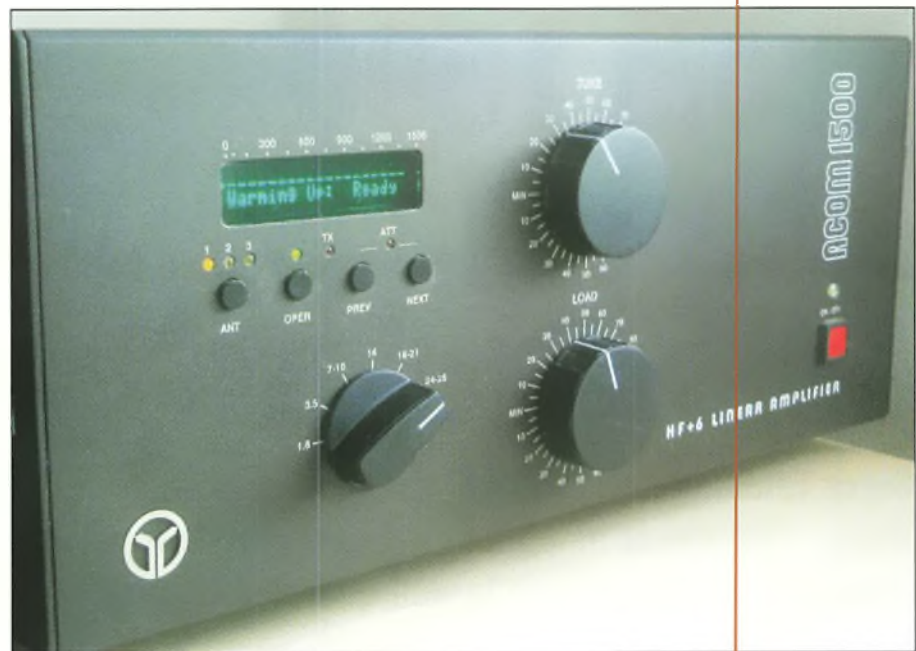
Fig. 3: After 3 minutes warm-up the vacuum fluorescent display shows 'Warming Up: Ready'.
