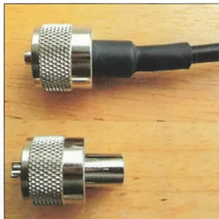
Fig. 3: this is the newer version of the short shank PL259 plug.
