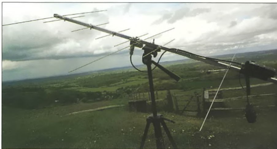
Dick GOLFF's neat portable dual band satellite antenna, mounted on a camera tripod.
