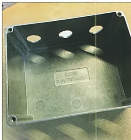
Fig. 1: The diecast box with three holes drilled for the SO239 sockets.
