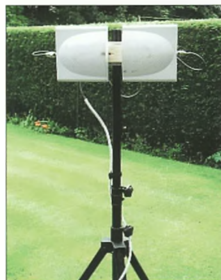
Fig. 1: The first BWC station built by Ross Wilkinson G6GVI using a pair of borrowed Wi-Fi antennas.
