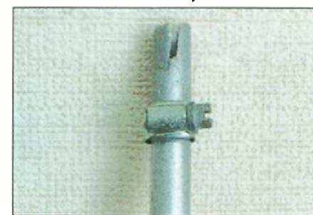
Fig. 3: Clamping one tube inside the other.
