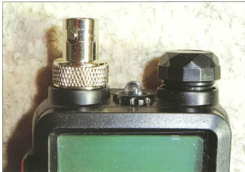
**Fig. 6 A BNC to SMA adaptor fitted to the top of the Baofeng UV-5R transceiver.**
