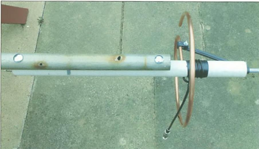
**Fig. 4:** Coach bolts are used to clamp the aluminium mast to the plastic pipe.
