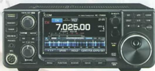
The IC-7300 sports HF + 6m + 4m coverage, it's 100W, houses an eye-catching touchscreen TFT display and includes an internal antenna tuner.
