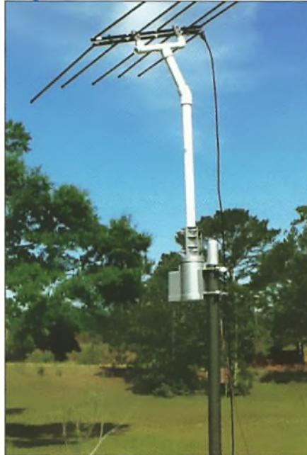
**Fig. 1: Harry K4BAD's Elk antenna, used for working satellites.**
