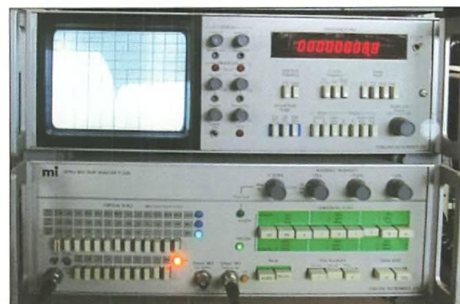
Fig. 3: The 80m filter characteristic as measured in Tony's workshop.
