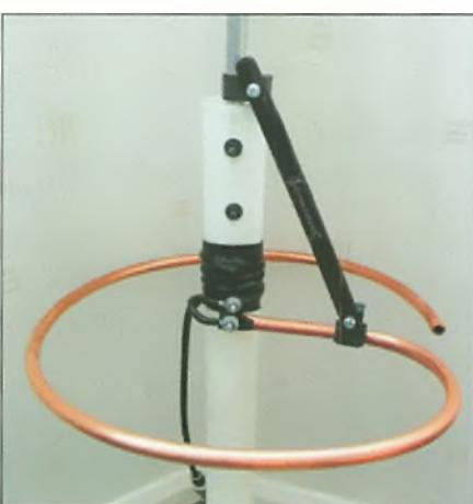
**Fig. 16:** The lower part of the antenna prior to final weatherproofing.
