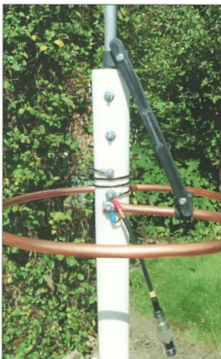
**Fig. 10:** The base of the antenna – the matching coil can be seen wound around the plastic pipe.
