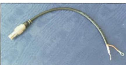
**Fig. 13:** Coaxial assembly for the feedpoint.
