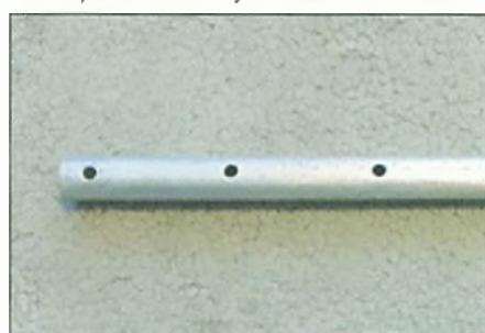
**Fig. 7:** Drilling matching holes in the aluminium.
