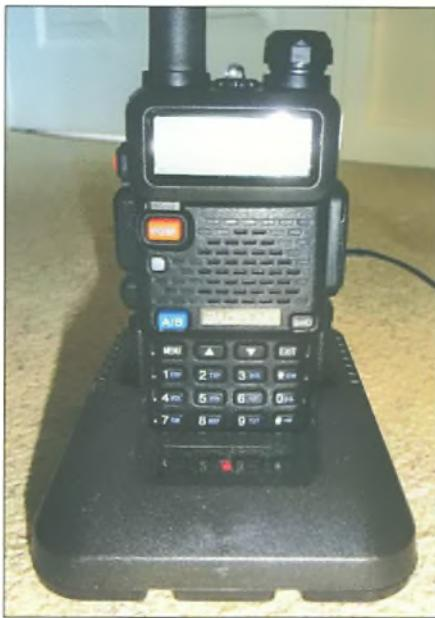
Fig. 2: Charging the Baofeng UV-5R with the battery already fitted. Note the red LED on the base showing charging underway.
