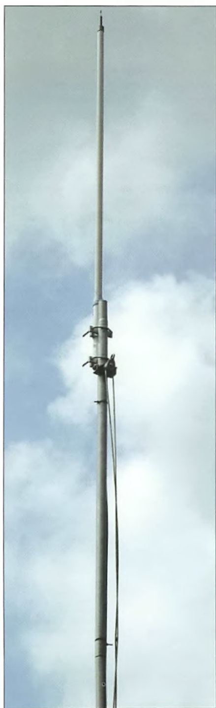
Fig. 1: An external vertically polarised antenna mounted high up and fed with low-loss feeder will certainly increase the range over which you can hear and be heard.
