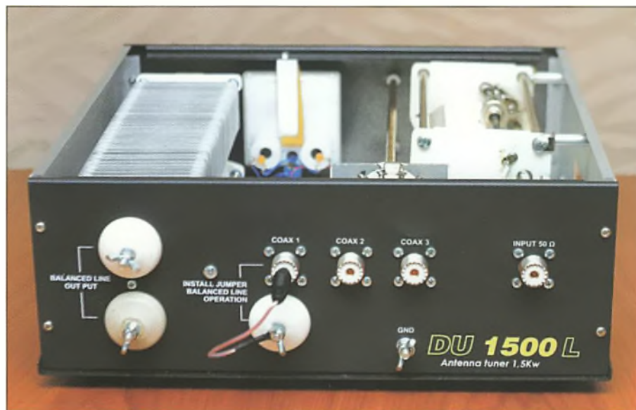
Fig. 7: Rear panel view of the DU1500L. The layout is representative of all three tuners.
