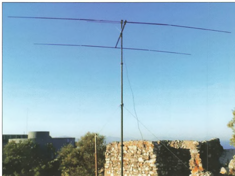
Fig. 5: The 10m 2-element Yagi used by Kevin ZB2GI/P from the top of the Rock of Gibraltar, 412m ASL.
