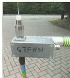
Fig. 3: The vertical dipole arrangement as finished.
