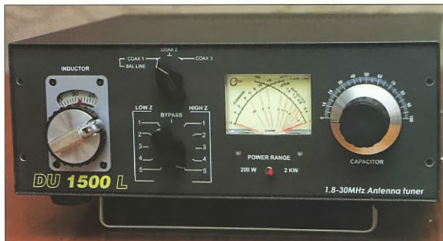
Fig. 1: Lamco DU1500L L-Match Tuner.
