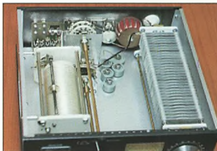
Fig. 5: Internal View of the DU1500L.
