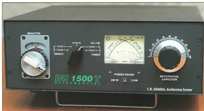
Fig. 3: Lamco DU1500T Differential T-Match Tuner
