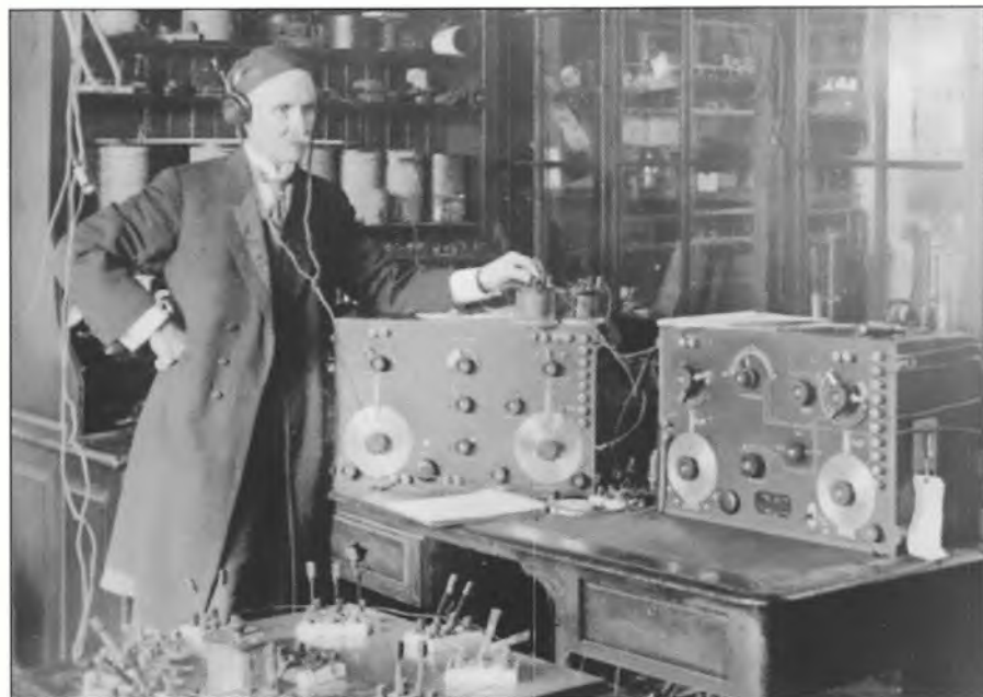
Fig. 7: The Naval Steam Engineering Department development laboratory at Washington Navy Yard with versions of Model SE-143 under test.
