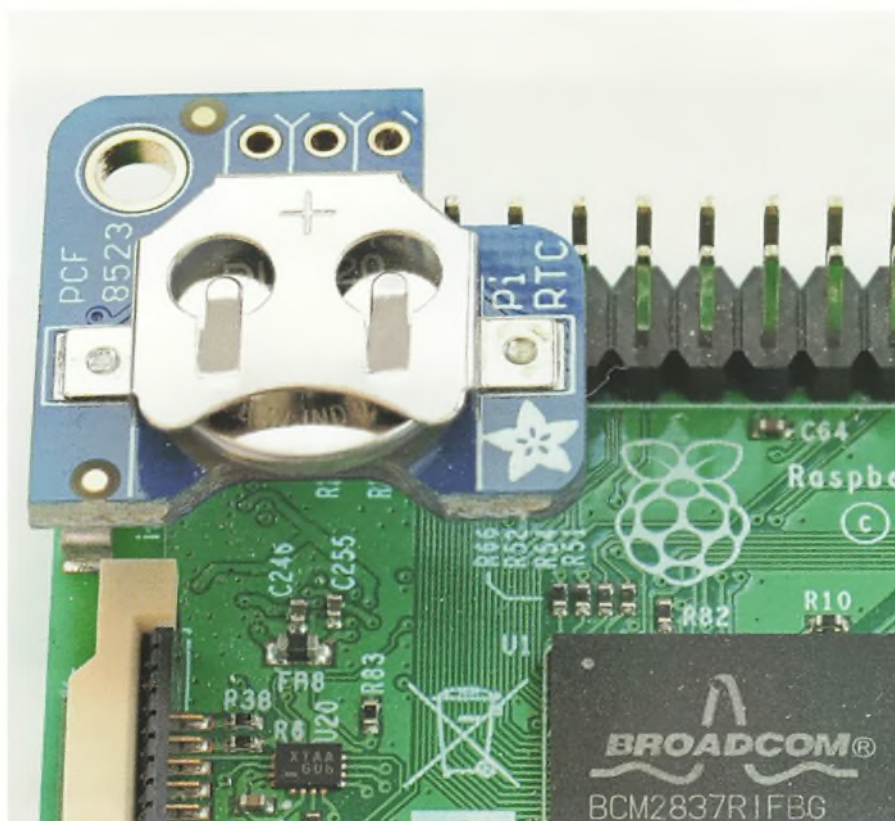
Fig. 1: RTC Clock fitted to a Raspberry Pi 3.
