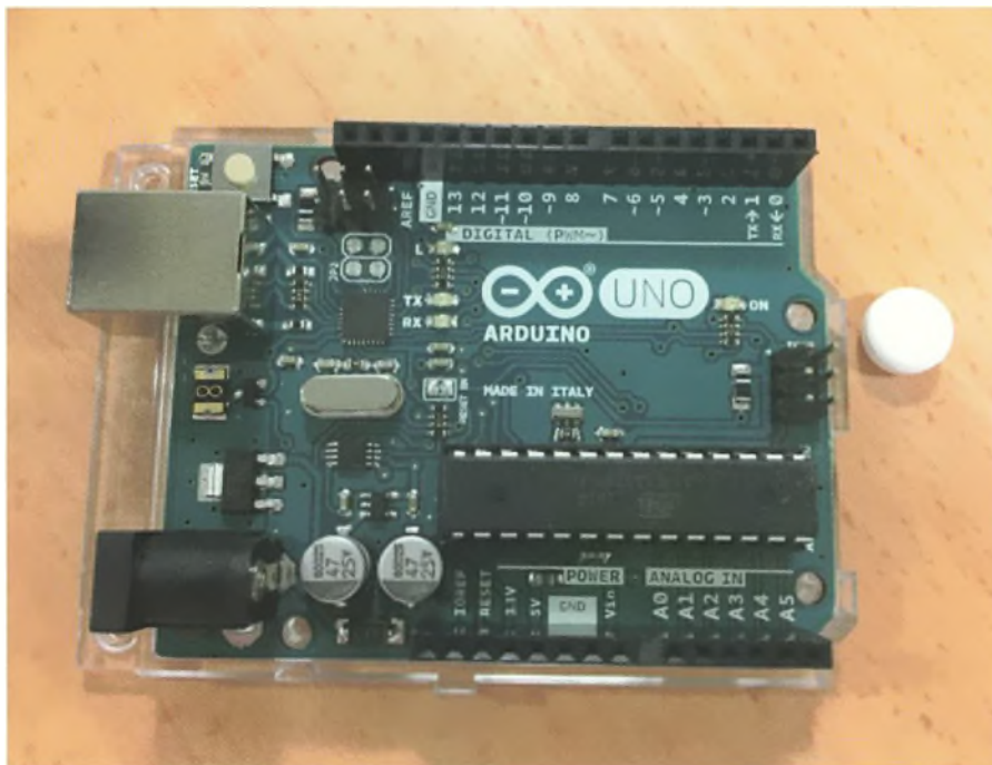
Fig. 4: The 'genuine' Arduino Uno R3.
