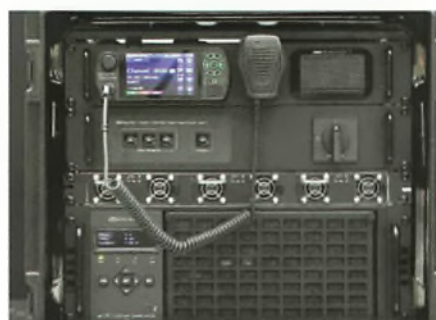
The Barrett 4075 liquid cooled amplifier.
