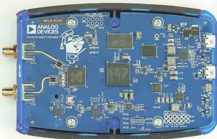
Fig. 6: A peek inside the Pluto showing the AD9363 and the ZYNQ FPGA/Processor.
