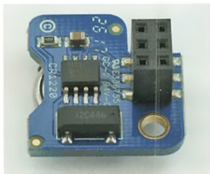
Fig. 2: CF8523-based RTC module.
