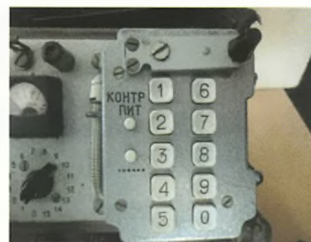
Fig. 6: The keypad and manual Morse key above.
