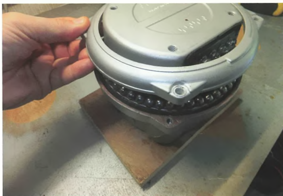
Fig. 2: Removing the guard exposes the ball bearings.
