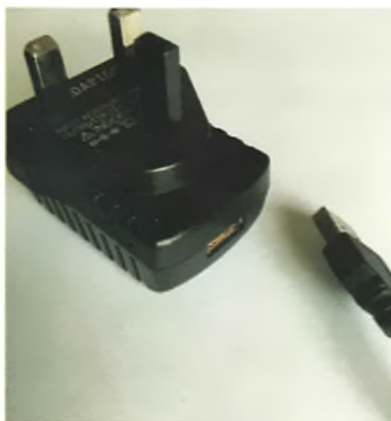
The charger. Beware the USB connectors and non-USB voltages (see text).
