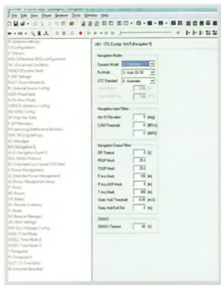
Fig. 4: Setting the GPS dongle to stationary mode with u-centre.
