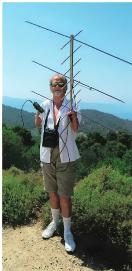
Fig. 3: Bernard (Ben) Nock operating as SV4/G4BXD from Skiathos, using an Arrow 2m/70cm beam antenna, an FT-817ND and a UV-5RE handheld – AO-91 was used mostly, working among others, Russia, Italy, France and, of course, the UK.
