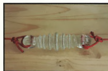
Fig. 5: A bowline to secure a rope to an antenna insulator.
