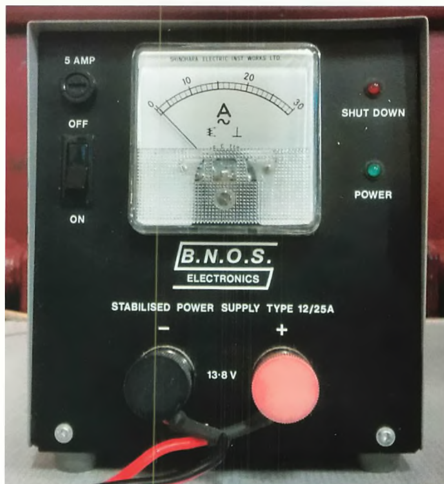
Fig. 1: A BNOS 25A power supply.
