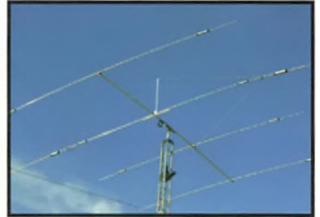
Fig. 12: The author's Mosley TA-34XL antenna with 6mm ropes to provide rigidity.
