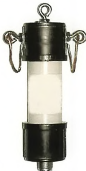
Fig. 1: The old W2AU-type 1:1 balun I had been given.
