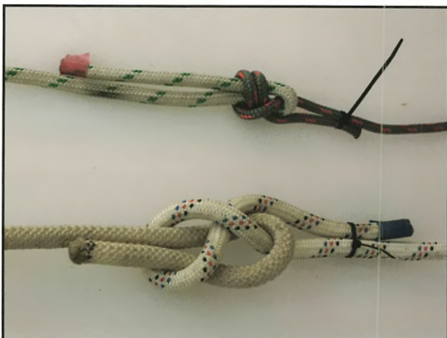
Fig. 8: Sheet bends – the double sheet bend is on top.
