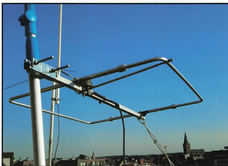
Fig. 1: Jef ON8NT's 4m halo, supported by a broom handle on his balcony.
