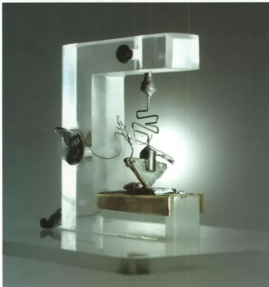
The point contacts of the first transistor were created by a razorblade slit in gold foil wrapped around the edge of a triangular plastic wedge. (Bell Labs)
