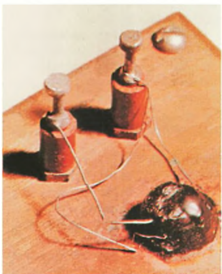
The first germanium junction transistor was fabricated by Morgan Sparks in 1950. (Bell Labs)
