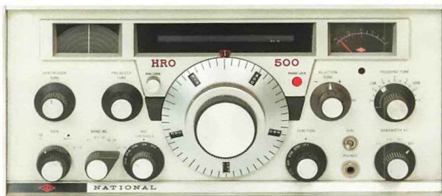
National launched the solid-state HRO 500 in 1964. It was built like a traditional valve receiver but used 37 germanium transistors and 20 diodes. (Merate Chronometer Center)
