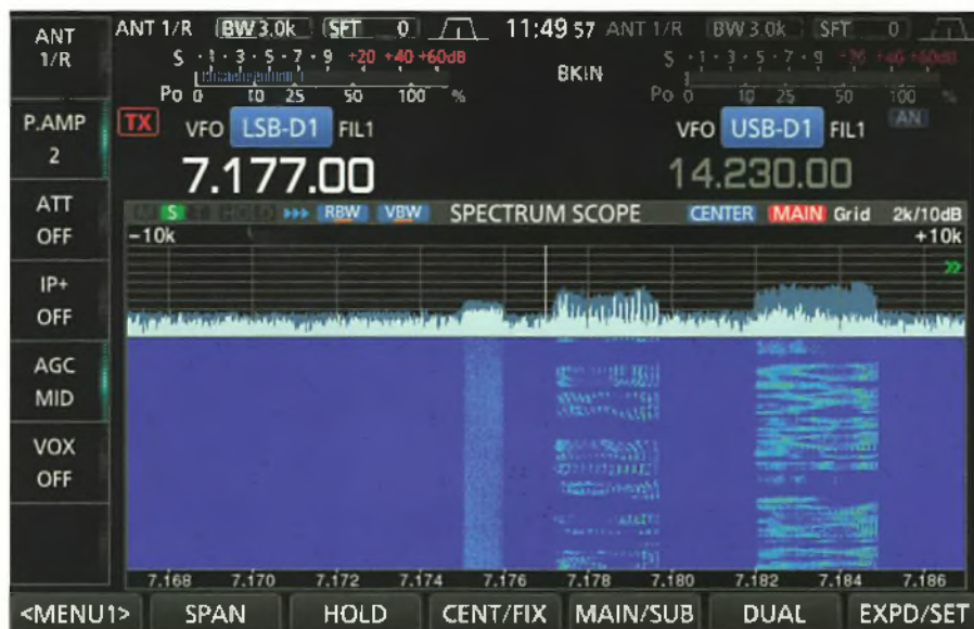
Fig. 1: A comparison between the spectra of FreeDV and SSB signals.
