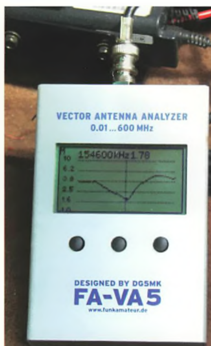
Fig. 7: Plot for the Diamond 8900 antenna.
