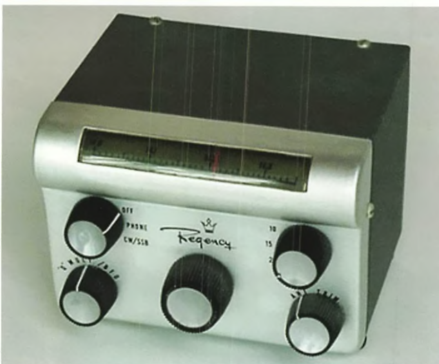
The 1956 Regency ATC-1 HF band converter was one of the first commercial transistor products for radio amateurs. (W8ZR)
