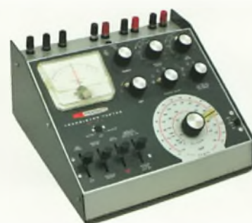
The IM-30 was the first of a series of simple transistor testers that could measure DC gain and leakage current. (Heathkit)
