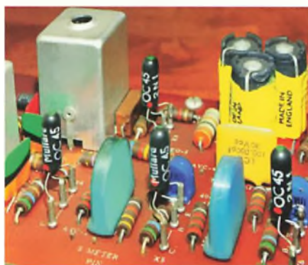
Early transistor receiver technology. The glass-encapsulated Mullard germanium transistors are mounted on solder sockets like little valves. (GM3NZI)
