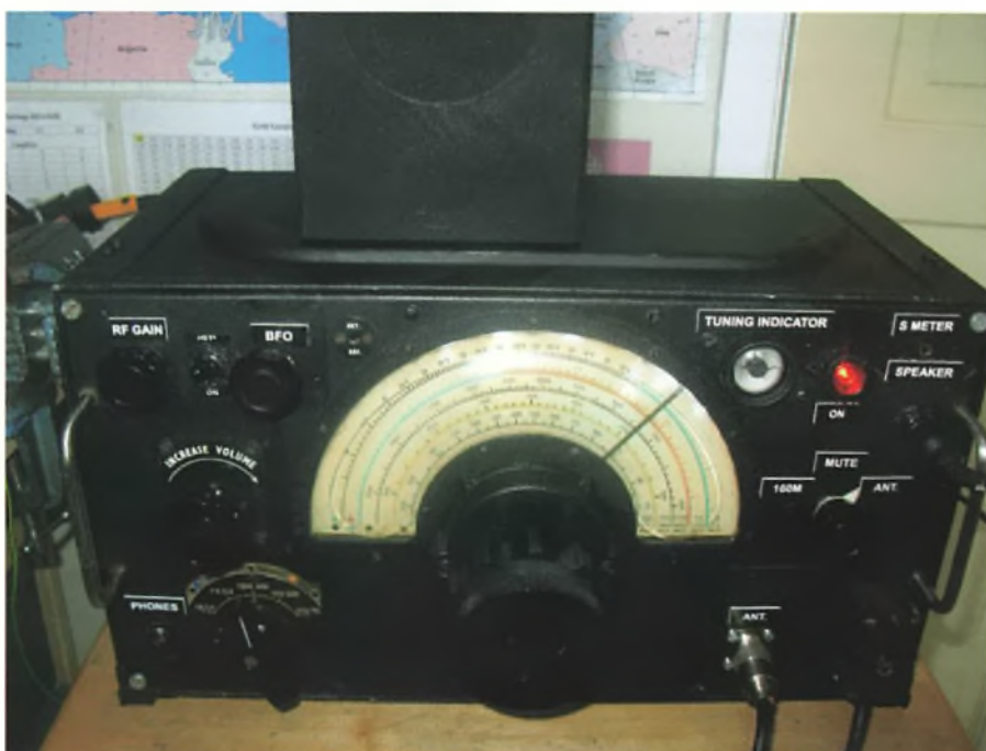
Fig. 4: The R1155 with additional switch setting for the 160m transverter.
