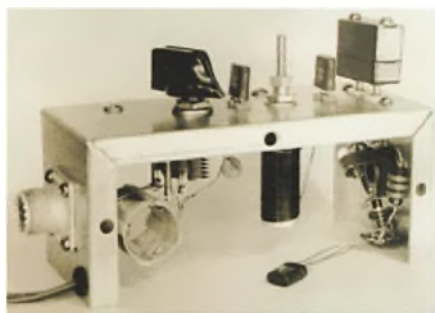
W10GU's historic 14MHz transatlantic transmitter used two germanium 2N113 transistors. (Raytheon)
