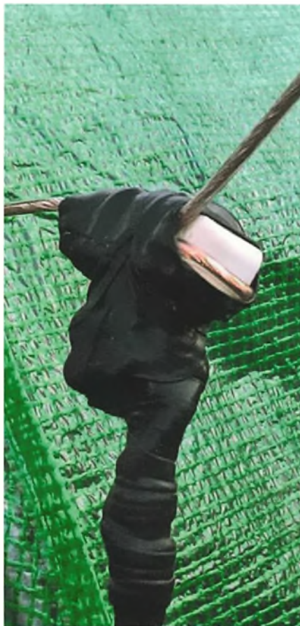
The author's original centre piece with poor weatherproofing.
