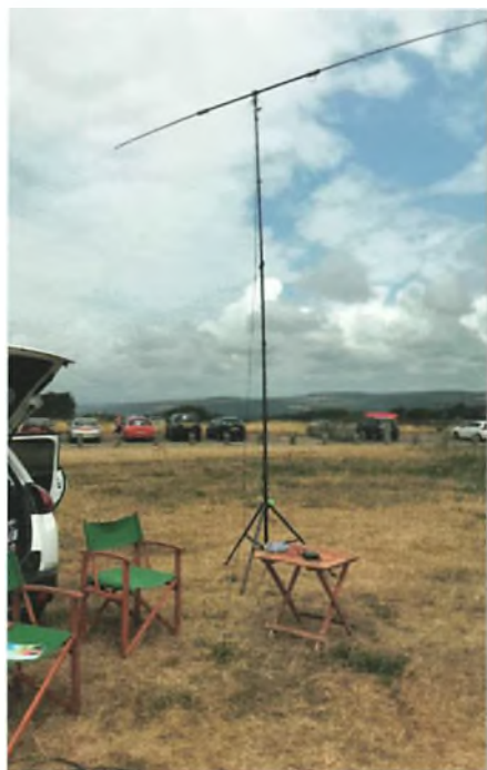
Fig. 2: The Buddipole, configured as a 20m dipole, at a height of 5m.
