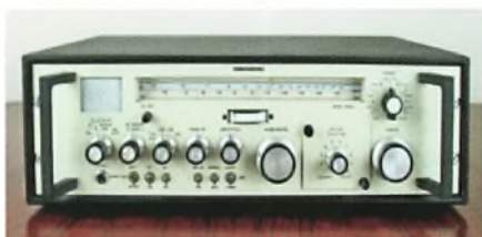
The 33-transistor Eddystone 1830 had a JFET/MOSFET cascode RF amplifier and dual-gate MOSFET first mixer. (Eddystone UC)
