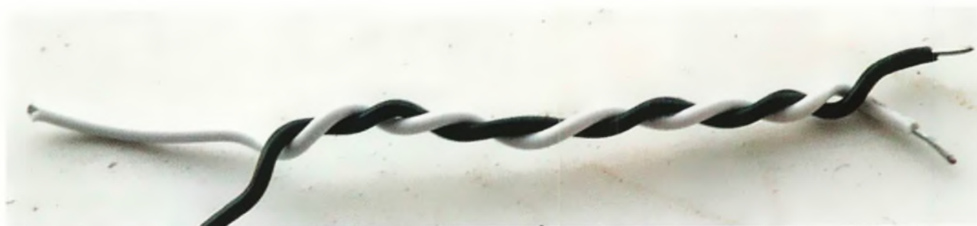
Fig. 11: 'Gimmick' Neutralising capacitor.
