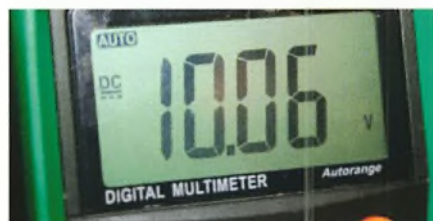
Fig. 6: 3½ digit meter reading just over 10V – the right-hand digit now displays increments of 10mV (hundredths of a volt).
