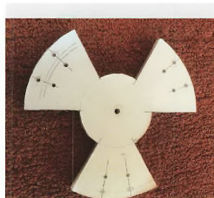
Fig. 3: The first disc, designed to secure rod and coil.
