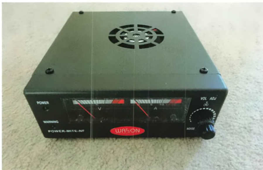
Fig. 2: A modern switch-mode power supply unit capable of powering a 100W HF transceiver.
