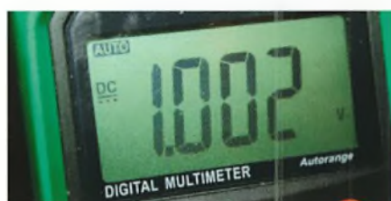
Fig. 5: 3½ digit meter reading just over 1V – the right-hand figure is displaying millivolts.
