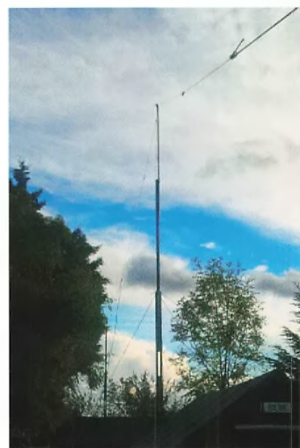
Fig. 1: The 30/40m half-wave inverted-V dipole.
