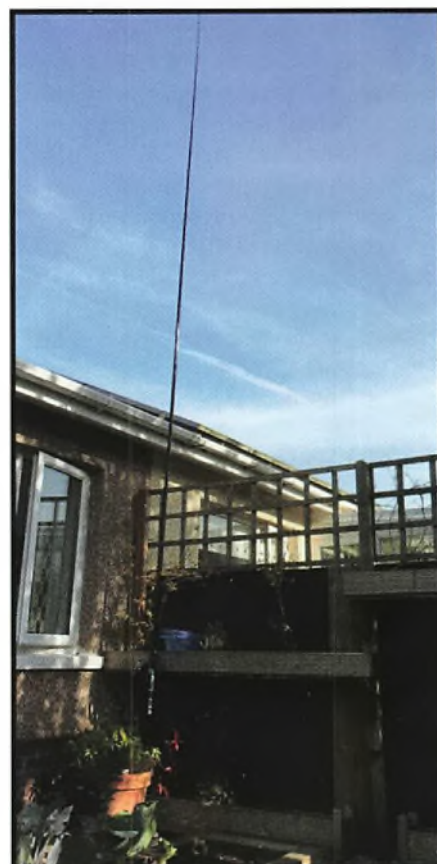
The author's version of a Marconi vertical – a SOTABEAMS 7m pole, with 300Ω ladder line, shorted at the top, as radiator, and a matching coil (the blue box) a metre off the ground.
