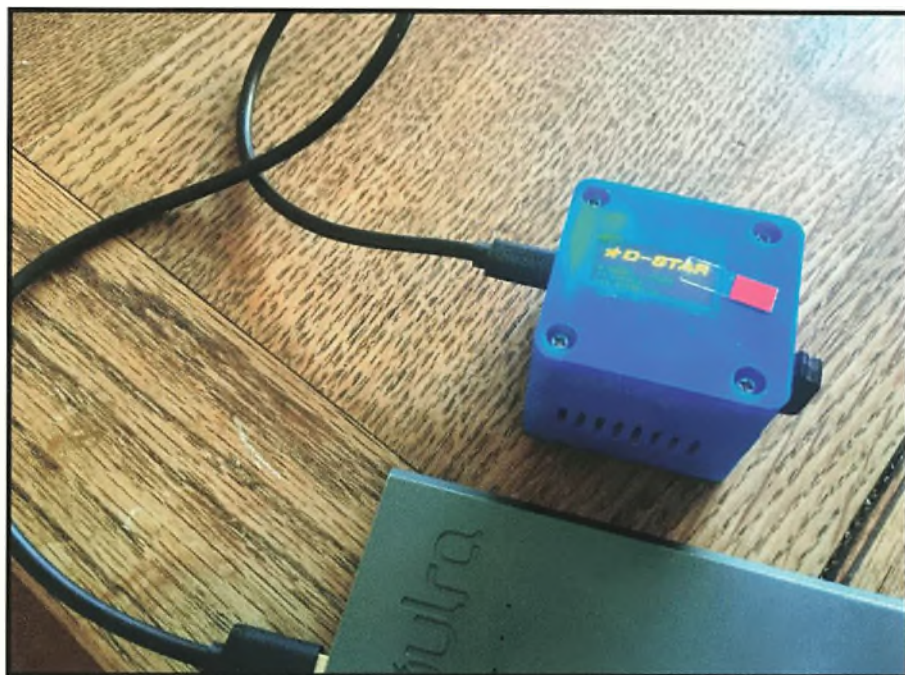
The Nano has low enough power consumption that you can use a USB power bank to provide its power. I found this was more than adequate for several hours use.
