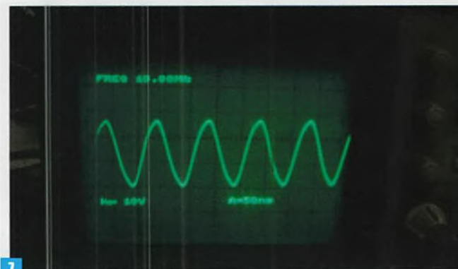
Fig. 5: PCB layout. Fig. 6: 2MHz base signal. Fig. 7: 10MHz output from multiplier.
