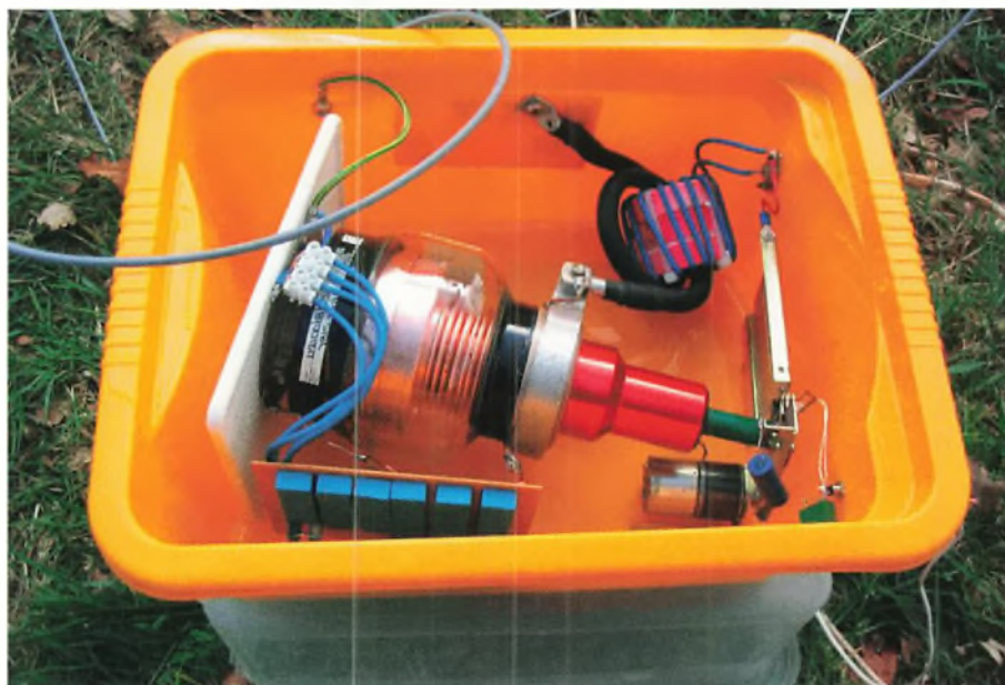
Fig. 5: Tuner for the loop antenna of Fig. 4.
