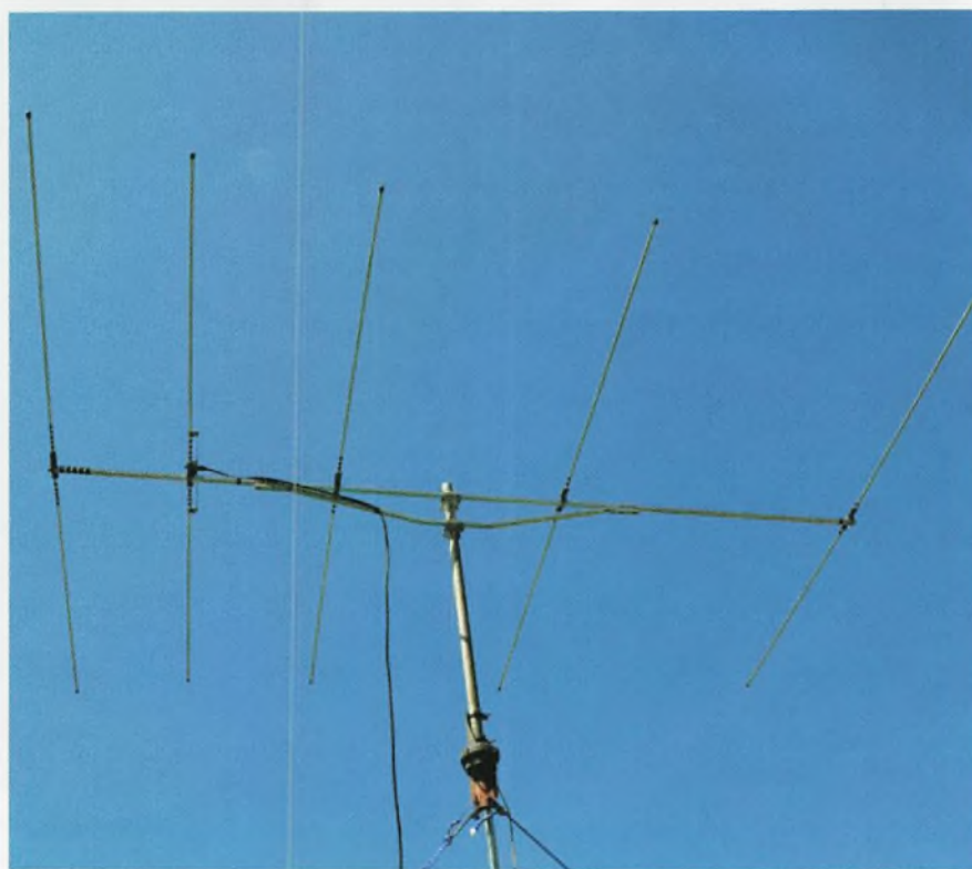
Fig. 1: A fairly compact 5-element Yagi antenna for the 6m band.
