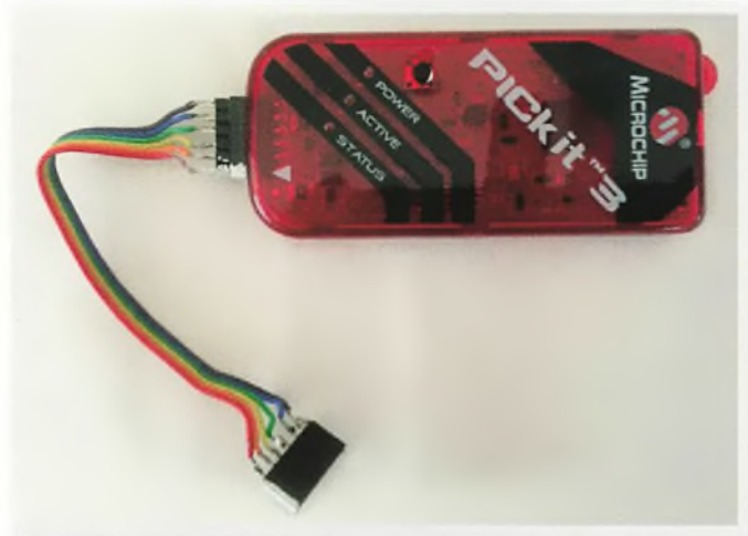
Fig. 4: PICKIT3 Programmer showing in-circuit programming leads.
