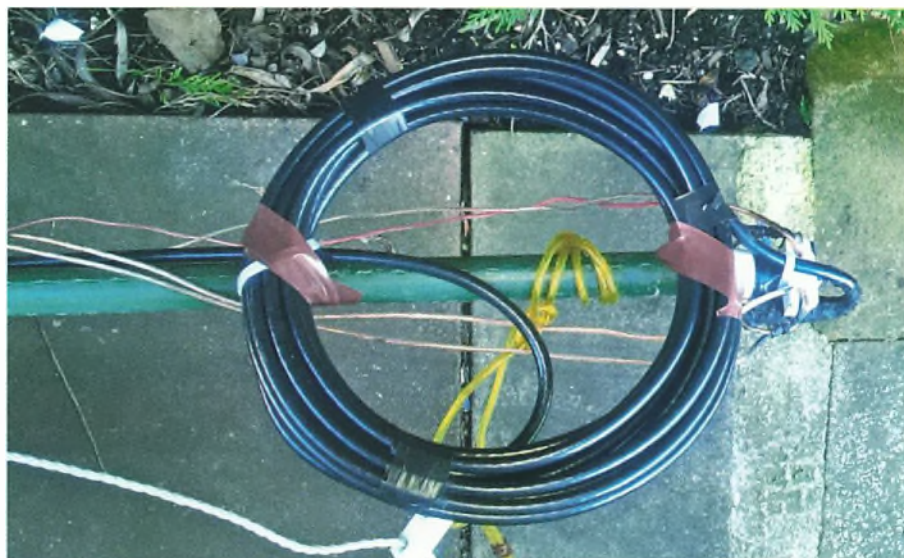
Fig. 2: New 30/40m inverted-V dipole connections.
