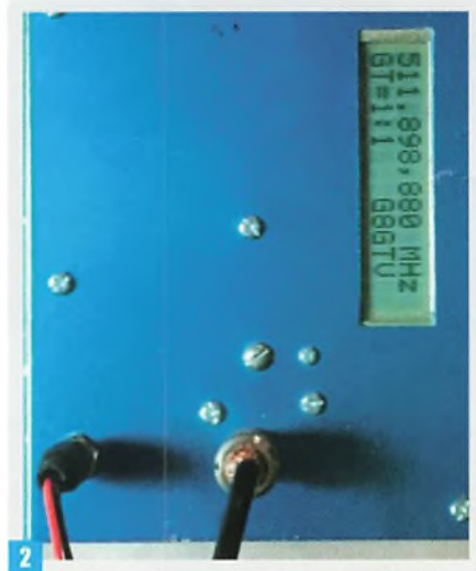
Fig. 1: ECL/TTL-based 500MHz Frequency Counter, footprint: 13 x 28cm. Fig. 2: PIC-based 1.30GHz Frequency Counter, footprint: 4 x 13cm.
