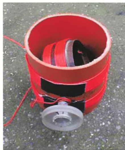
Fig. 3: The author's homebrew variometer.
