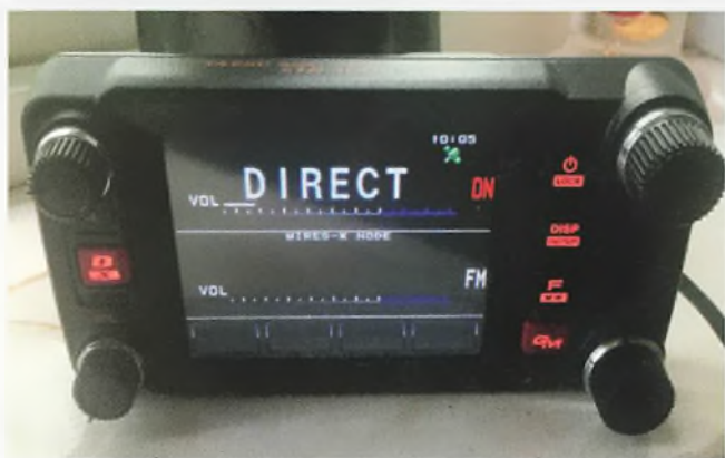
2. & 3. The FTM400XDE supports two new modes, Direct mode where no RF is transmitted and the rig acts as a speaker mike and Access Point mode (second photo), where the rig acts as a local hotspot allowing you to connect to it using a C4FM enabled handheld close by.
