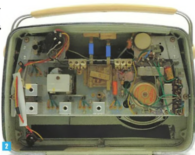
Fig. 2: Interior view of the Bush receiver, showing the construction method.
