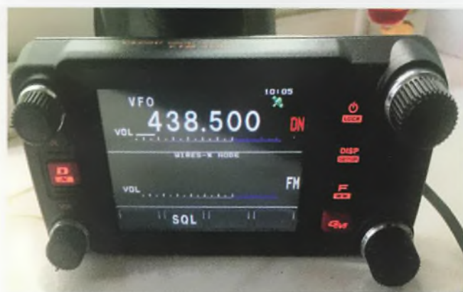
2. & 3. The FTM400XDE supports two new modes, Direct mode where no RF is transmitted and the rig acts as a speaker mike and Access Point mode (second photo), where the rig acts as a local hotspot allowing you to connect to it using a C4FM enabled handheld close by.
