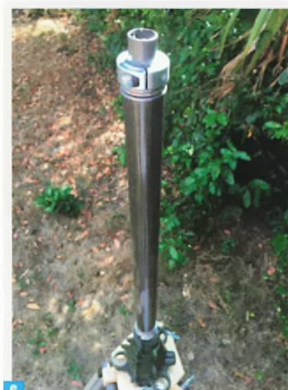
Fig. 3: Tungsten carbide burr to grind the gear to fit the splined motor shaft. Fig. 4: Drive gear fitted to motor splined shaft, secured with metal epoxy and shaft nut. Fig. 5: Backbone tube with spacer springs mounted in the mast. Note the lower thrust bearing and shaft collar. Fig. 6: The outer antenna stub is fitted, sitting between thrust bearings and shaft collars.
