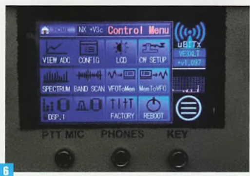
Fig. 4: Raspberry Pi and USB sound card ready for installation. Fig. 5: Raspberry Pi installed and hard wired. Fig. 6: The Nextion touchscreen. Fig. 7: Using VNC Viewer for remote control. Left to right: uBitx with Raspberry Pi, Smartphone running Wi-Fi hotspot, Tablet with VNC Viewer. Fig. 8: First QSO, with F4FSY on 10MHz FT8. Fig. 9: First portable operations on a nearby hilltop with 3D printed CW paddle.
