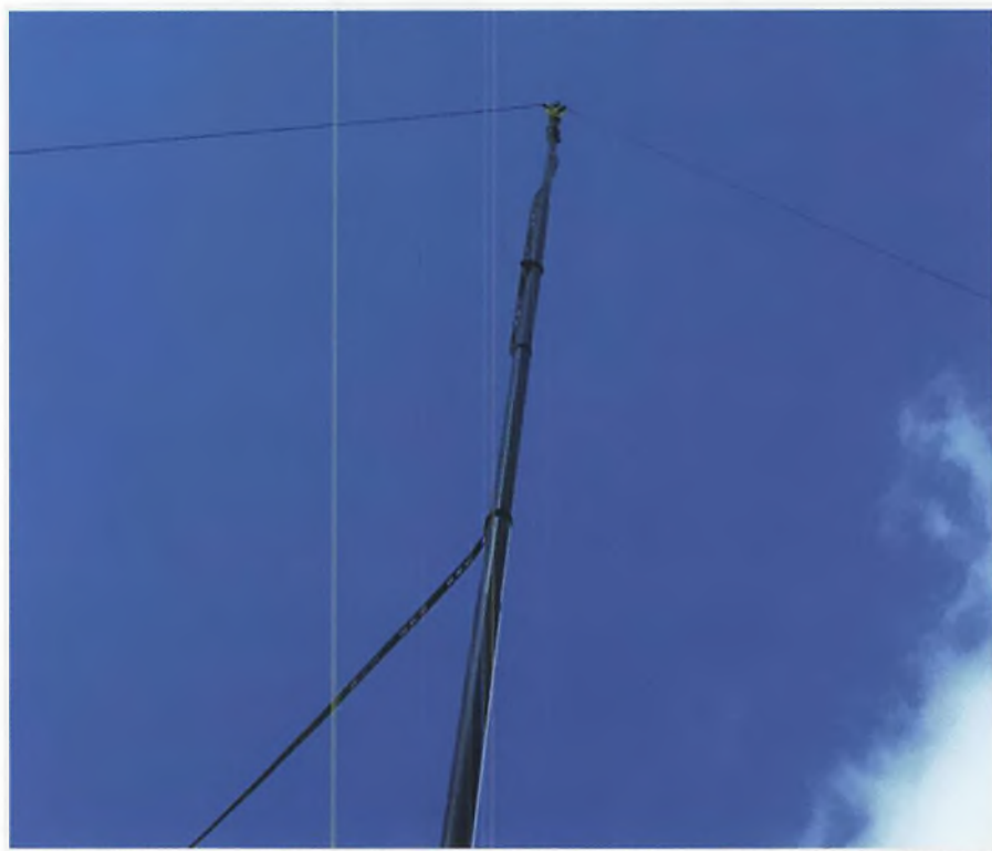
The centre of the inverted-vee supported by an 8m fibreglass pole. Note the 300Ω ladder-line running down as straight as possible to avoid interaction with the doublet legs.
