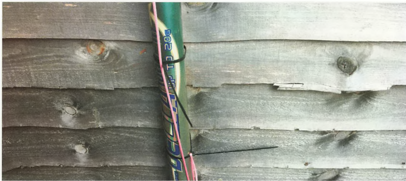
The 4:1 current balun. Simply hooked to the side of a low height shed. The 300Ω ladder-line feeding it from the antenna apex, with a short piece of RG213 running from the balun to the LDC tuner inside the shed itself.
