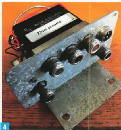
Fig. 4: 'Homebrew' masthead LNA. Note the changeover relay is mounted with the three N connections through the box for easy access. Fig. 5: Replacement driven element on the author's Wimo 44-element Yagi. Fig. 6: Examples of three relays (see text).
