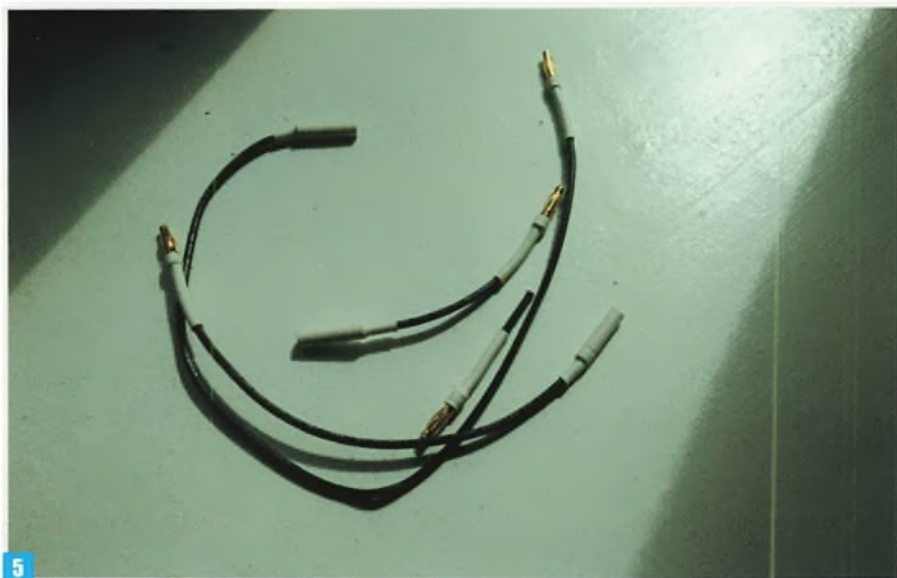
Photo 5: One set of extension wires – various lengths that can be connected in a wide variety of combinations.
