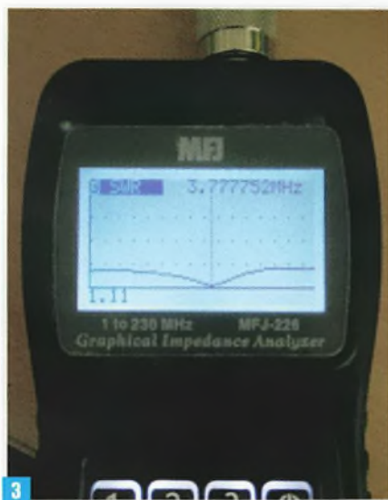
Photo 1: The parts after unpacking from the tube. Photo 2: The antenna on a Rascal ex-military mast. Photo 3: SWR plot on 80m, measured on MFJ-226 analyser.
