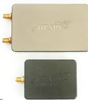
Fig. 1: Block diagram of the Discovery filters. Fig. 2: the latest model is EMI-proof with the key components inside a screened housing (HF+ above Discovery below). Fig. 3: External view of HF+ and Discovery.
