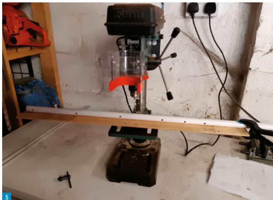
Fig. 1: Drilling the tubing to take the extension. Fig. 2: The extended tubing, with join. Fig. 3: Bending the tubing. Fig. 4: The completed dipole end. Fig. 5: Drilling the boom. Fig. 6: Using copper tape for the joint.
