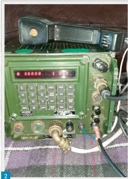
Fig. 1: Remote operating from the balcony using a tablet in a shoebox at ON8NT. Fig. 2: Rhodri MORHO uses this Racal VRM-5080 on 70MHz and hopes to try it soon on 50MHz. Fig. 3: The impressive antenna system of Derek Brown G8ECI. Fig. 4: Graham G3VKV's second system for QO-100
