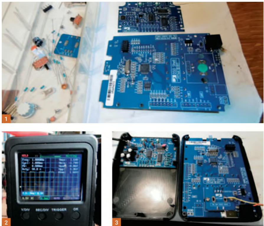
Fig. 1: The kit. The surface mount components arrive already mounted and soldered.
