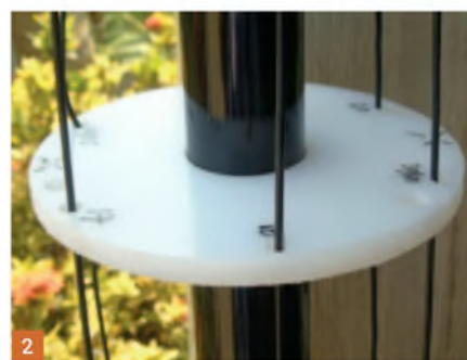
Fig. 1: The completed DX Commander 10mABV vertical. Fig. 2: The vertical wire elements are separated around the pole by spacers. Fig. 3: During construction a short additional length of wire is wrapped back to allow for fine tuning and temporarily held in place with insulating tape.
