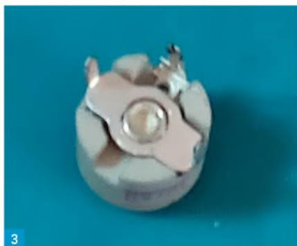
Fig. 1 The G3RJV preselector circuit. Fig. 2 George's preselector. Fig. 3 Ceramic trimmer rivet connection. Fig. 4 Improved grounded area. Fig 5. RF amplifier with screening.
