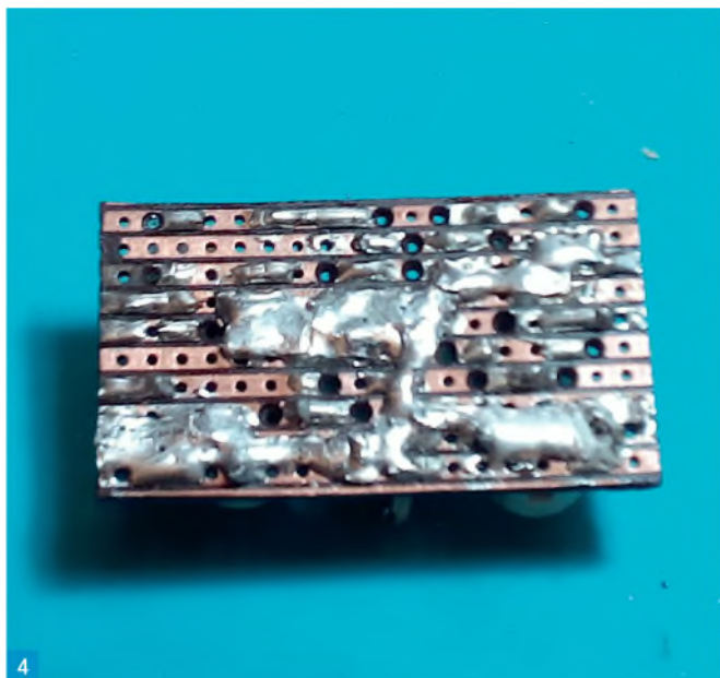
Fig. 1 The G3RJV preselector circuit. Fig. 2 George's preselector. Fig. 3 Ceramic trimmer rivet connection. Fig. 4 Improved grounded area. Fig 5. RF amplifier with screening.
