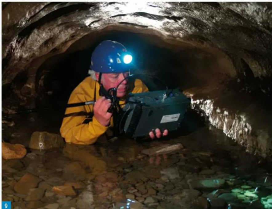
Fig. 9: Mike Bedford, G4AEE, uses a spectrum analyser to monitor propagation at 5.7GHz along a low passage in Kingsdale Mater Cave, Valley Entrance. (Mike Bedford)
