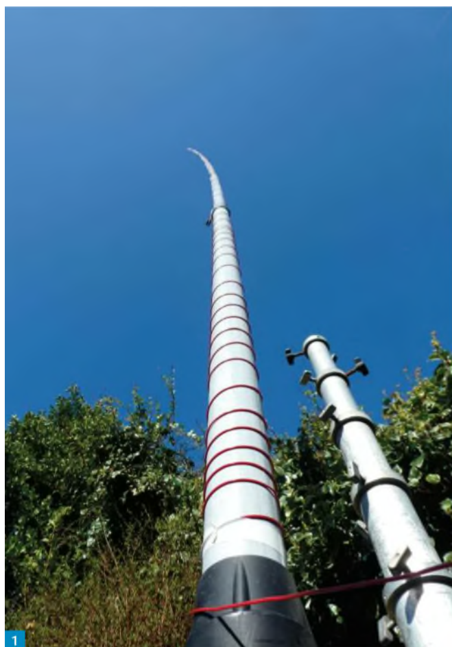
Fig. 1: On the right you can see my retracted 12m aluminium mast (r) next to my 15m fibre mast (l). Both masts can be used independently when the other is down. The lower 2m of the aluminium mast supports the fibre mast using two (35 x 35cm) Tufnol panels and 8 U-bolts. The 15m fibre glass mast is shown here with 20m of wire wound around it forming a helix antenna for 80m (see text).
