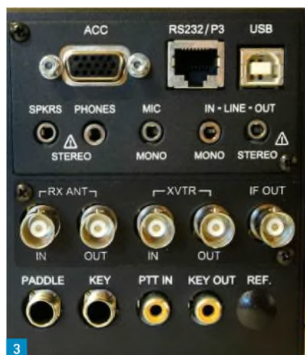
Fig. 1: The SignalLink USB is a popular interface between computers and transceivers. Fig. 2: RTTY messages can become corrupted due to QRM, QRN and QSB. Fig. 3: The Elecraft K3S transceiver includes a built-in sound card. It can be connected to a computer simply with just a USB lead plugged into the rear panel shown here. Fig. 4: An FT4 contact with Thailand on 20m using just 10 Watts to a dipole antenna at about 6m above ground level. Fig. 5: An SSTV picture received from the International Space Station (ISS). Fig. 6: The Full Licence Manual is essential reading for those studying for their Full Licence exam. Fig. 7: The Exam Secrets book contains some additional material for all three exams as well mock exam questions.
