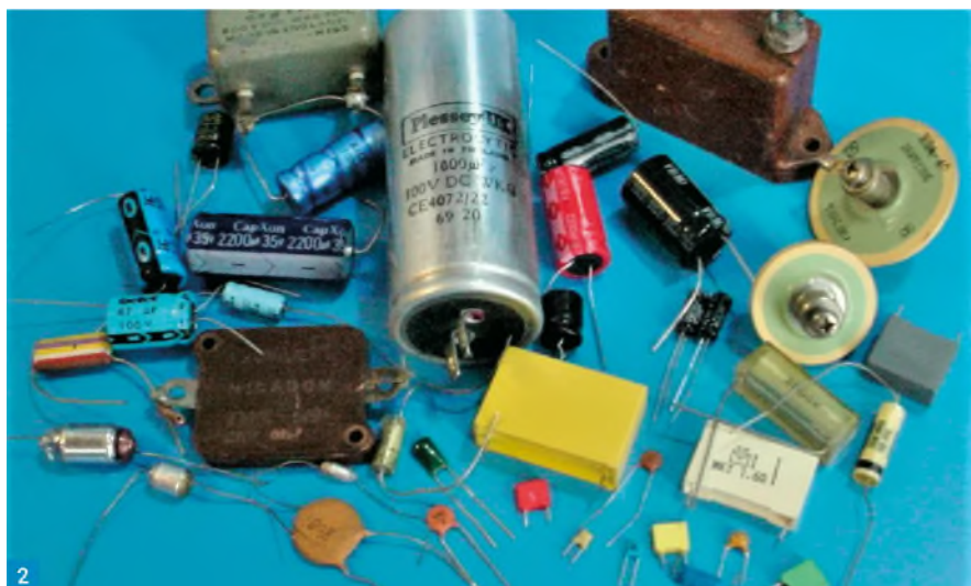
Fig. 1: The basic construction of a capacitor. Fig. 2: A selection of capacitors used in electronic circuits. Fig. 3: Symbols used for capacitors. Fig. 4: Simple circuit showing how charge builds on the capacitor. Fig. 5: As Fig. 3 but with a switch to allow the direction of current flow to be reversed. Fig. 6: Using analogue meters to observe current flow in a capacitor. Fig. 7: The effect of applying a sinewave voltage across a capacitor.
