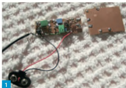
Fig. 1: E-field probe by PA0RDF, taken from G3XBM's comprehensive website: https://tinyurl.com/y6y7qko4
