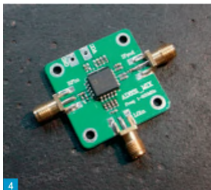
Fig. 1: Circuit diagram. Fig. 2: Bending of the pins on the ployvaricon. Fig. 3: LCD and backboard in plastic holder. Fig. 4: The AD631 mixer module. Fig. 5: Audio amplifier. Fig. 6: Bandpass filter PCB. Fig. 7: VFO PCB. Fig. 8: Audio filter and preamp PCB. Fig. 9: The complete receiver.
