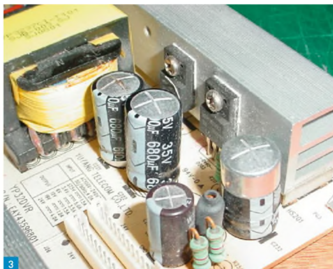
Fig. 1: Bridge rectifier circuit. Fig. 2: An NPN transistor with a collector load resistor. Fig. 3: Switched mode PSU with 'bulging' capacitors. Fig. 4: Another example of a 'bulging' capacitor. Fig. 5: Emitter follower circuit. Fig. 6: Exploded polypropylene capacitor. Fig. 7: Homebrewing a capacitor. Fig. 8: Measuring the homebrew capacitor. Fig. 9: Measuring the 'gimmick' capacitor. Fig. 10: Multivibrator circuit. Fig. 11: Using a capacitor to charge to double voltage.
