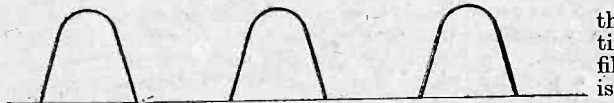
Fig. 2.—The resultant current through the rectifier as a result of applying the voltage of Fig. 1.
