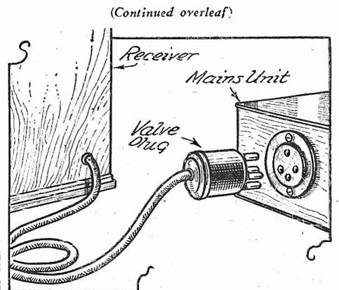
Fig. 2.—When the mains supply system is built as a separate unit, connection to it can be made by means of a valve plug and valve holder mounted as shown.
