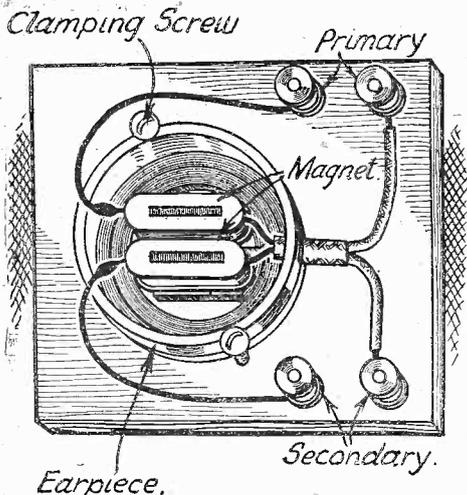
A small transformer made from an ear-phon.
