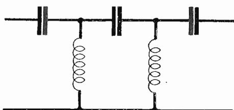
Fig. 2.—An ordinary two section T-filter.
