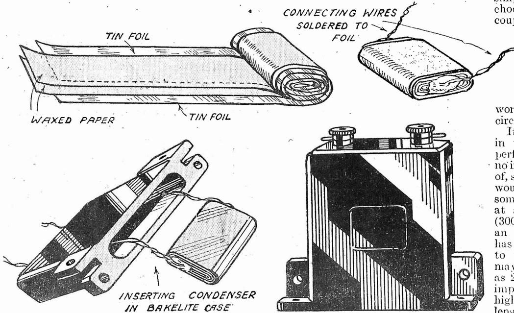
Fig. 5.—A paper condenser and details of its construction.
