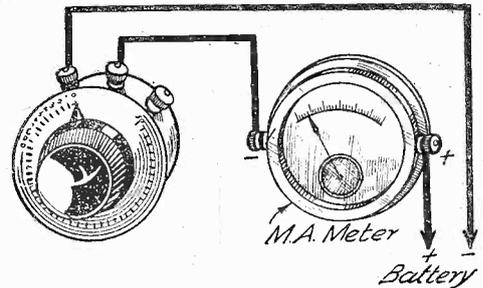
Fig. 2.—Calibrating the variable resistance by means of a milliammeter and battery.
