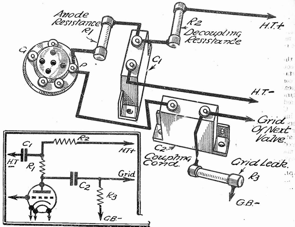
Fig. 1.—A typical resistance-capacity coupled stage. As the grid leak is, in effect, in parallel with the anode resistance, it must be of considerably higher value.
