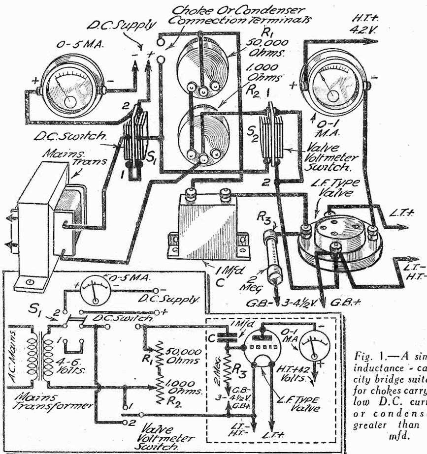
Fig. 1.—A simple inductance-capacity bridge suitable for chokes carrying low D.C. current or condensers greater than .07 mfd.
