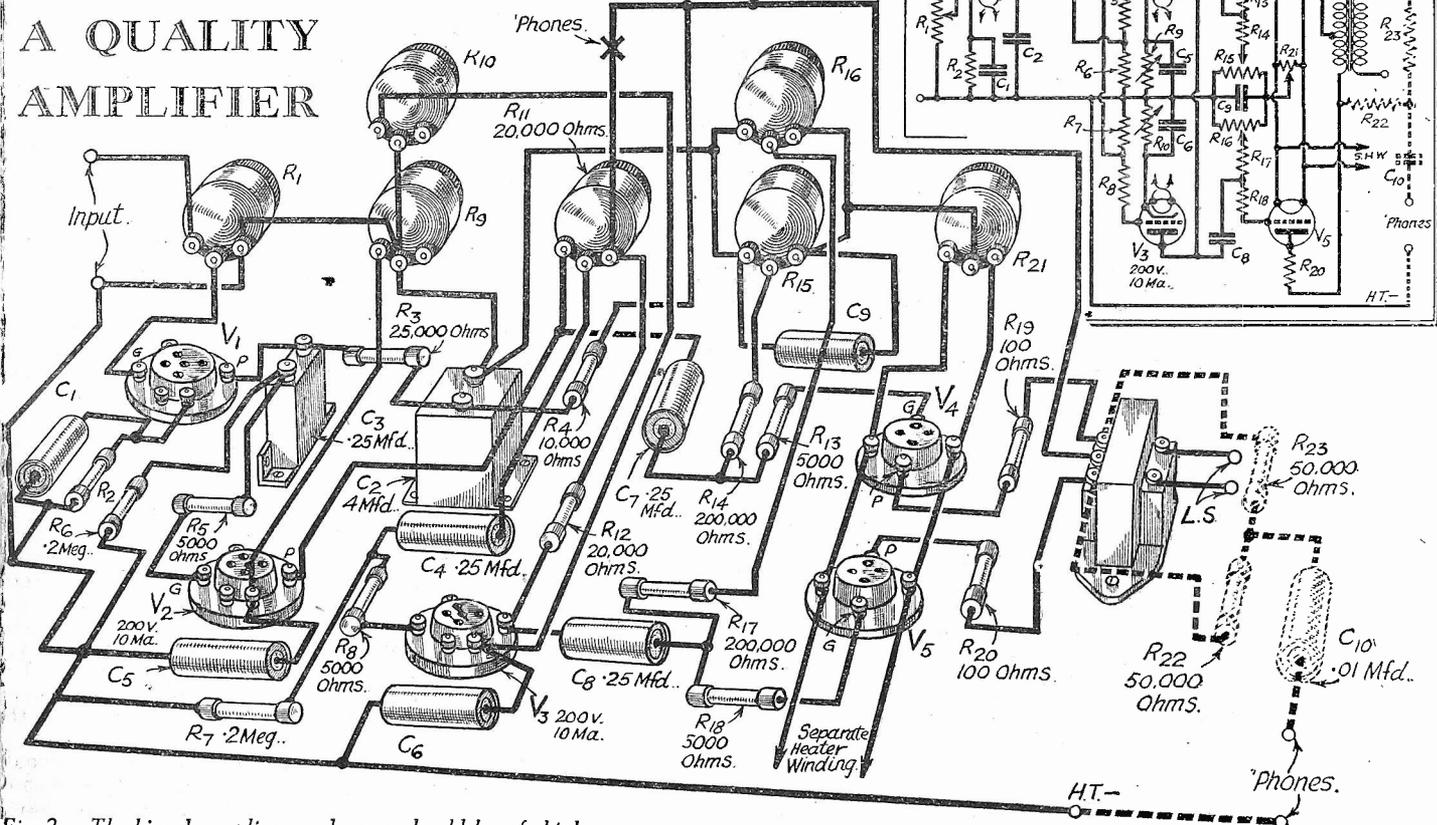
Fig. 2.—The bias decoupling condensers should be of high-capacity electrolytic type. The variable bias controls should be about one-fifth higher resistance than the maker's recommended value.
