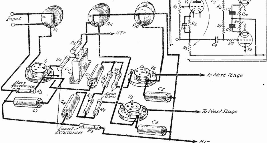
Fig. 3.—In this arrangement the desired phase opposition is obtained by splitting the V.1 anode resistance, inserting one half in the anode circuit and the other half in the cathode circuit.
