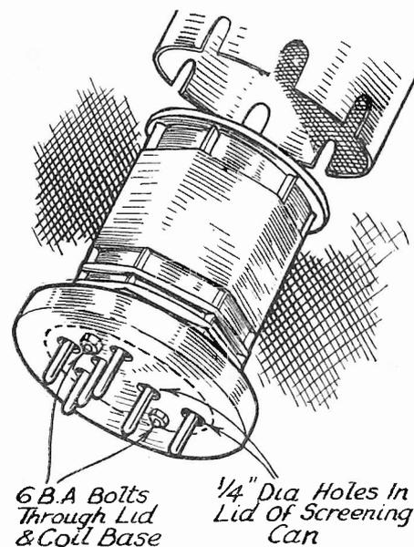
Fig. 2.—Showing how 3in. diameter screens can be fitted to standard 6-pin plug-in coil formers.
