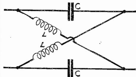
Fig. 6.—A circuit suitable for phase correction.
