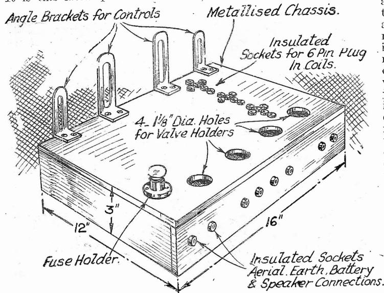
Fig. 1.—A suggested arrangement for the experimental chassis. The dimensions are approximate.
