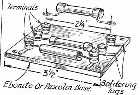
Fig. 4.—An easily made resistance-condenser unit by means of which the components can quickly be replaced.
