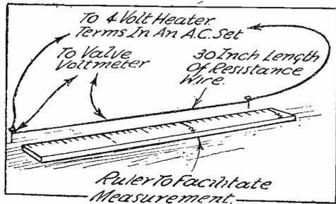
Fig. 4.—An A.C. voltage of '13 is developed across each inch of resistance wire.
