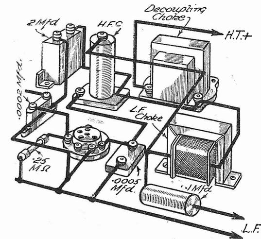
Fig. 1.—The circuit of a power-grid detector using choke capacity L.F. coupling and a choke for decoupling, as mentioned in the accompanying text.
