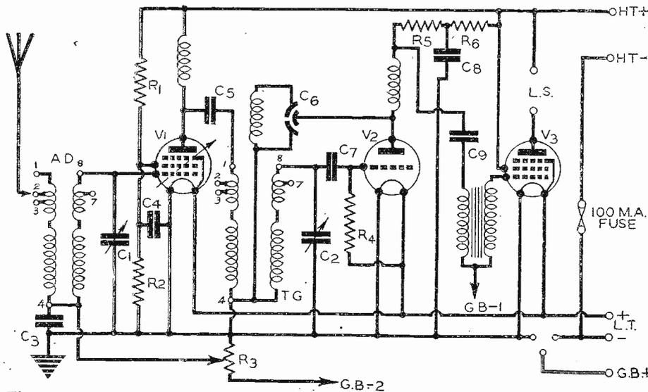
Theoretical circuit of the "Summit," a good example of a straightforward three-valver employing the popular S.G. detector and output arrangement.
