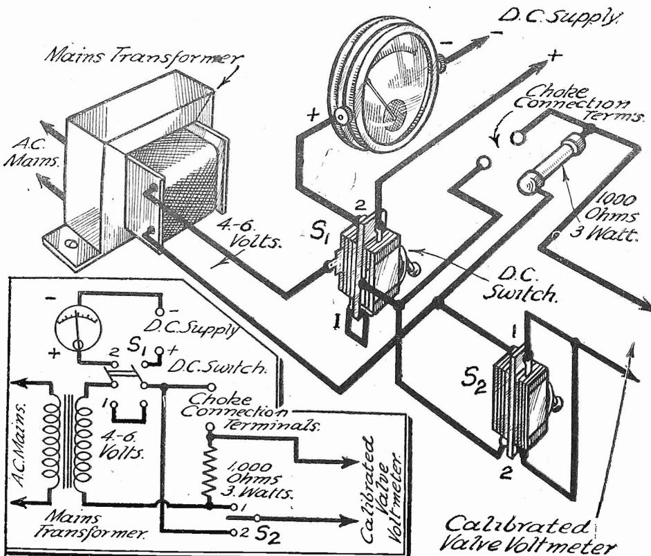
Fig. 3.—This arrangement permits of the measurement of the inductance of an L.F. choke whilst passing a large D.C. current.
