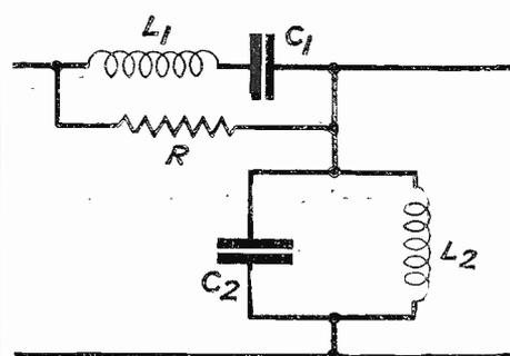
Fig. 5.—An inverted L-type circuit designed for equalization.
