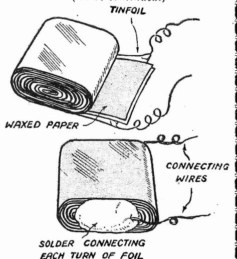
Fig. 6.—The top sketch shows a paper condenser which would be inductive, connections being taken from the ends only of the foil. That shown below is non-inductive since each turn of foil is connected.
