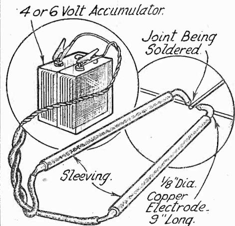
A novel method of soldering small work.
