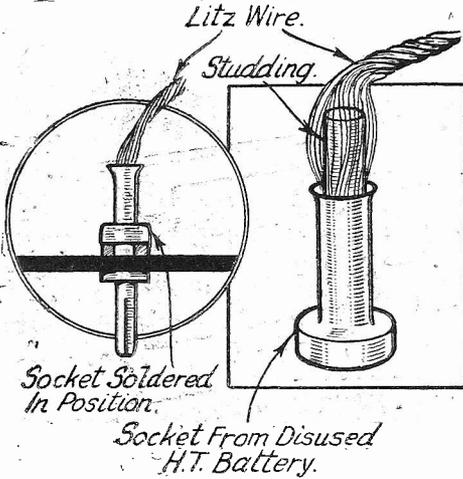
Method of making neat Litz wire connections.
