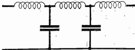
Fig. 3.—A low-pass inverse filter.
