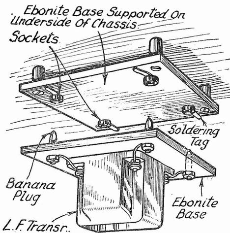
Fig. 3.—Showing the plug-in L.F. transformer idea suggested in the text.
