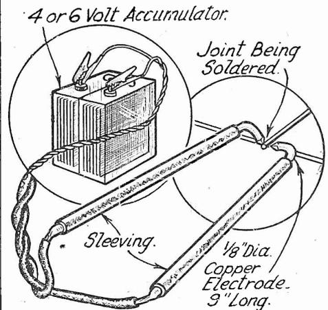
A novel method of soldering small work.
