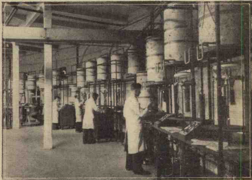
A section of a modern cathode-ray tube factory where the baking and pumping process is undertaken.
