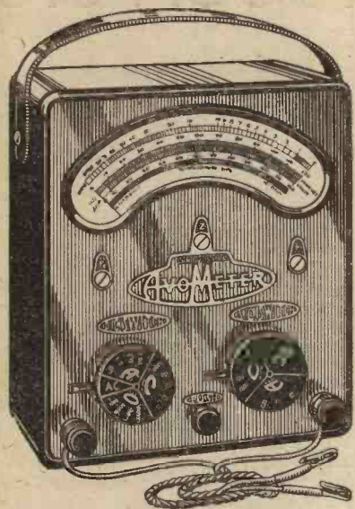
The Avo Test Meter, which has several separate ranges, easily selected by rotary switches.
