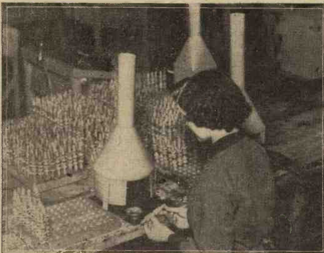
Constructors who have tried to solder the end of a length of fine Litz wire will appreciate the apparatus shown above at the Ekco factory. The small oven burns off the silk covering, the wire is dipped into the three containers, spirit, flux, solder, and a perfect joint is made.
