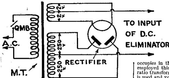
The rectifying section of an eliminator which may be added to an existing D.C. mains unit to convert for A.C. operation.
