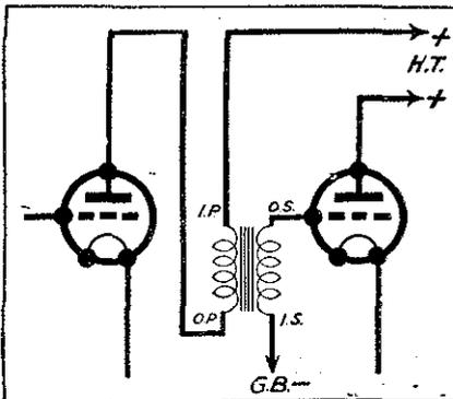
Fig. 2a.—Transformer primary directly in anode circuit.
