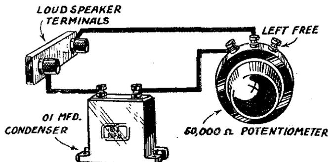
Fig. 10—A high-note filter—a cure for whistle, caused by heterodyning.
