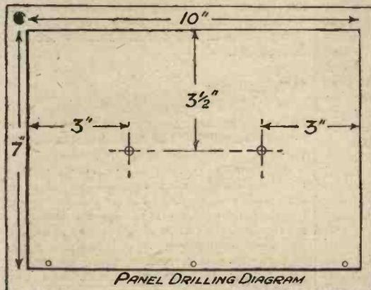
Fig. 2.—How to drill the panel.
