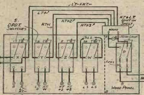
Showing general arrangement for an experimenter's switchboard.
