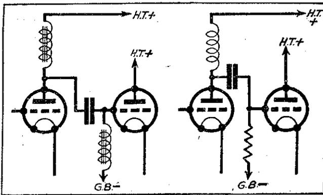
Fig. 3.—Two forms of choke coupling.
