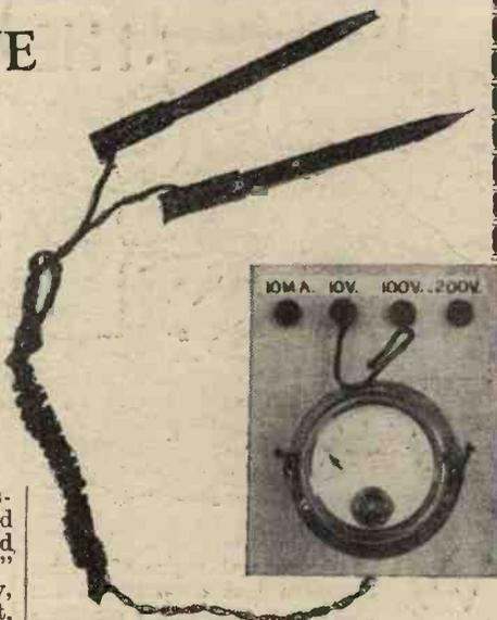
Fig. 2.—The complete four-range test meter with test prods.
