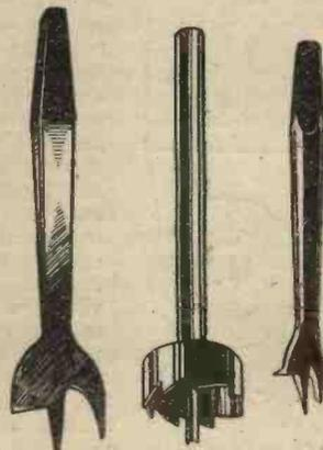
Fig. 5.—Centre-bits, and a panel cutter.
