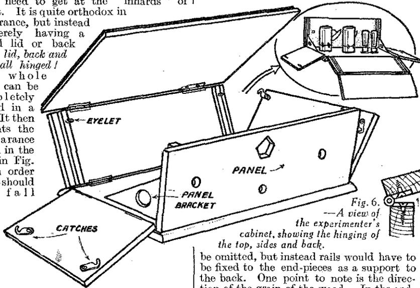
Fig. 6.—A view of the experimenter's cabinet, showing the hinging of the top, sides and back.
