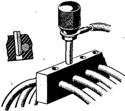
Simple method of tapping short-wave coils.
