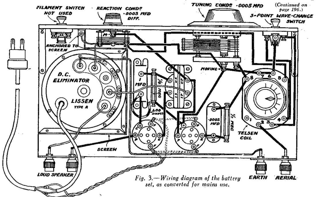
Fig. 3.—Wiring diagram of the battery set, as converted for mains use.
