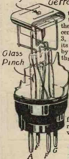
these, as shown in the Figs., are 2 the filament at the centre, surrounded by 3, the grid, which in its turn is surrounded by 4, the anode; these three parts are known as electrodes. Inside the bakelite base from which the valve pins project is cemented a glass pinch; embedded in this are five stout supporting wires, four of which run from the electrodes right through to the valve pins, two of
