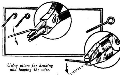
Using pliers for bending and looping the wire.
