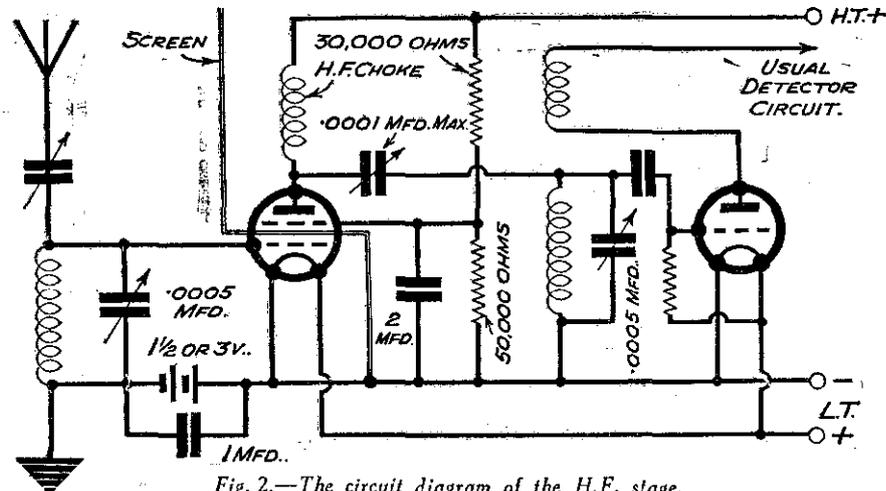
Fig. 2.—The circuit diagram of the H.F. stage.
