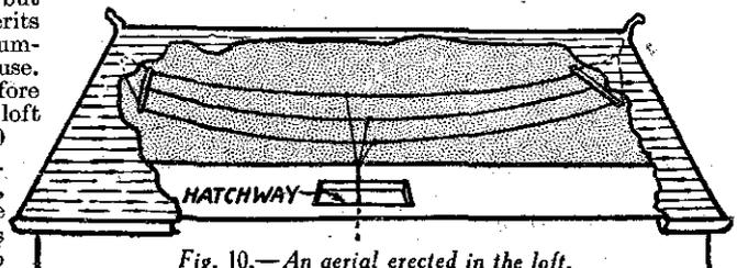
Fig. 10.—An aerial erected in the loft.
