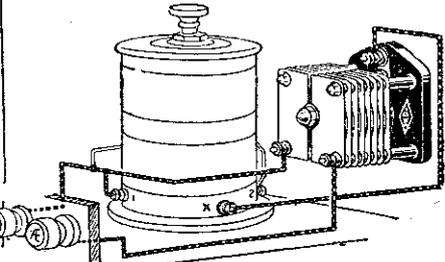
Method of controlling the volume from the input side of a wireless circuit.
