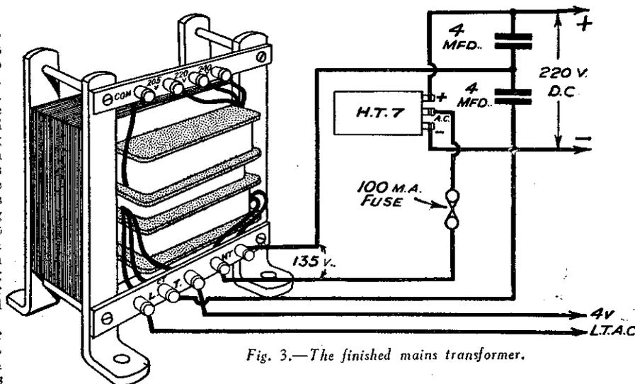
Fig. 3.—The finished mains transformer.
