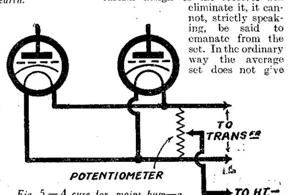
Fig. 5.—A cure for mains hum—a potentiometer is connected across the heater supply wiring.
