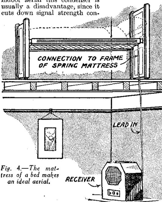
Fig. 4.—The mattress of a bed makes an ideal aerial.
