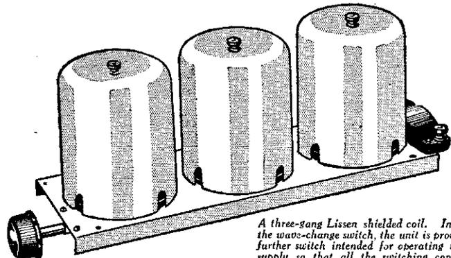
A three-gang Lissen shielded coil. In addition to the wave-change switch, the unit is provided with a further switch intended for operating the filament supply so that all the switching control of the receiver is operated by one knob.
