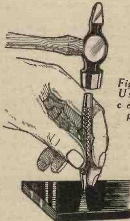
Fig. 3.—Using a centre punch.
