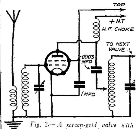
Fig. 2.—A screen-grid valve with tuned grid coupling.
