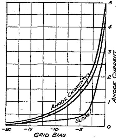
Fig. 1. The characteristic curve of the variable mu valve. Note the long, gentle slope caused by the irregularly spaced grid.
