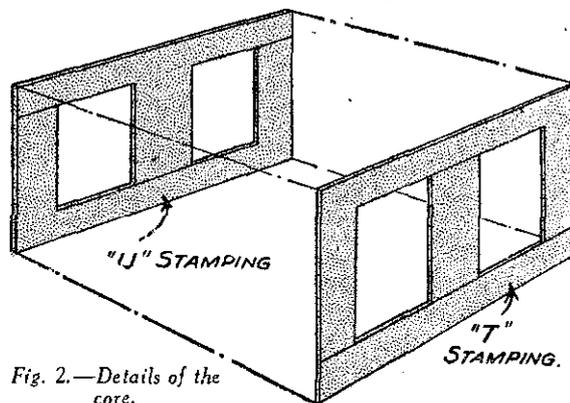
Fig. 2.—Details of the core.
