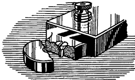
Fig. 5.—Use of the wrong screw will cause this! Don't use countersunk screws unless the lug hole is countersunk.
