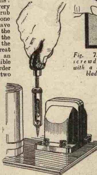
Fig. 6.—A special screw-driver which grips the head of a screw.
