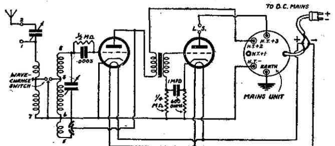
Fig. 2.—The circuit shown by Fig. 1 modified to suit the new Universal full mains voltage valves.
