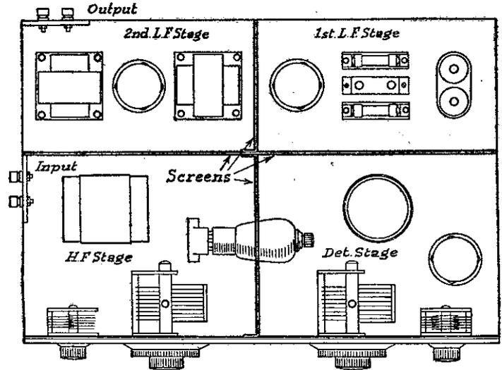
Fig. 4.—When the input and output ends of the receiver come close together the set should be screened as shown.
