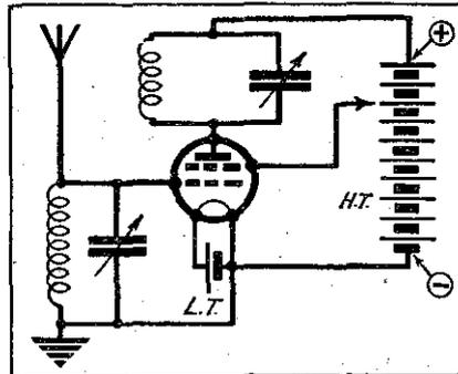
Fig. 3.—A screen-grid valve employing tuned-anode coupling.
