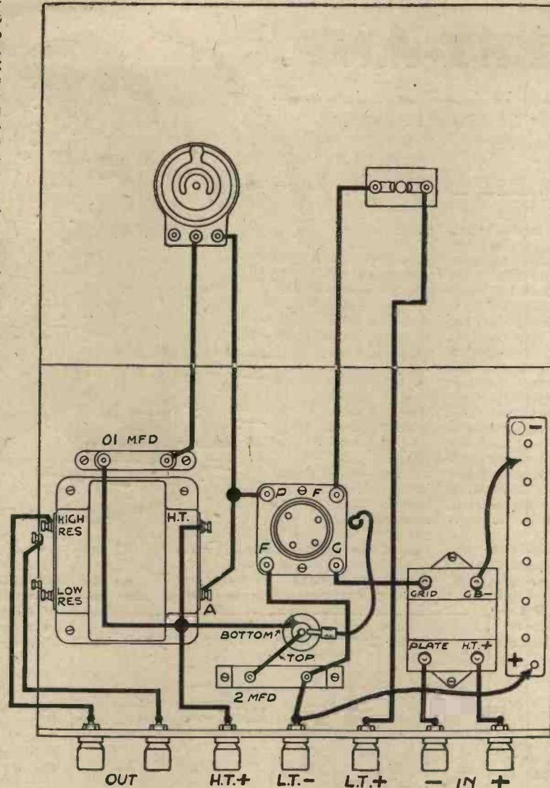
Fig. 4.—Wiring diagram of the Pent-Amp.
