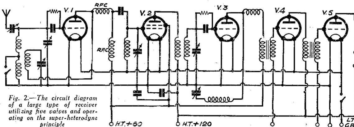
Fig. 2.—The circuit diagram of a large type of receiver utilizing five valves and operating on the super-heterodyne principle
