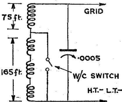
Fig. 1.—Diagram illustrating reply concerning frame aerial windings.
