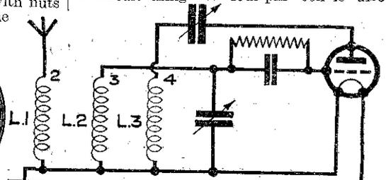
A coil former made from the base of an old valve REACTION COIL and (right) a circuit diagram using the four-pin coil.
