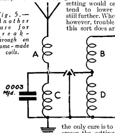
the only cure is to increase the setting of the series aerial condenser and make up for the reduced selectivity by decreasing the coupling between the primary and secondary circuits. If the coil is a home-made one, this can easily be arranged, either by reducing the number of turns in the tapped portion C, in the case of Fig. 4, or by placing the windings C and D farther apart, in the case of Fig. 5.
