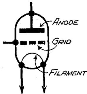
Fig. 3.—Conventional diagram of a three-electrode valve, indicating the essential parts.
