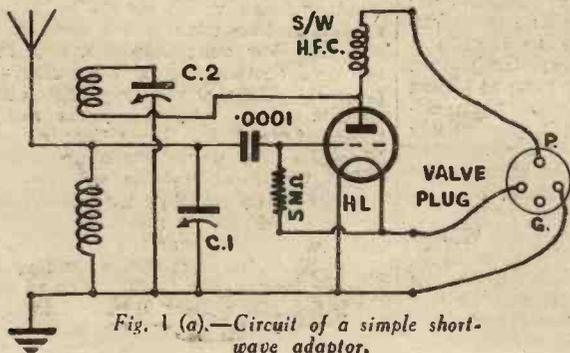
Fig. 1 (a).—Circuit of a simple short-wave adaptor.
