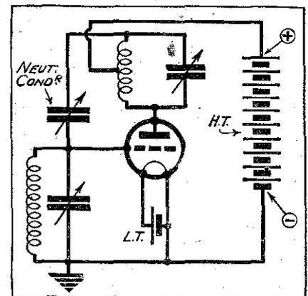
Fig. 2.—The well-known neutrodyne method of H.F. coupling.
