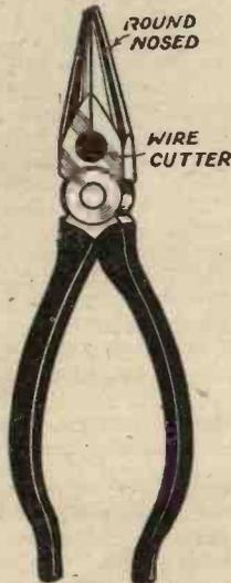
Fig. 10.—A pair of round nose pliers with wire-cutter.
