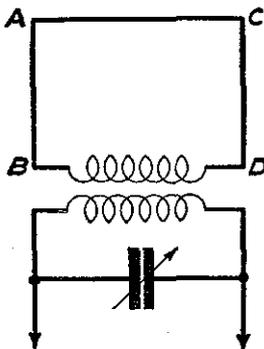
Fig. 3.—The frame aerial with its small coil coupled to the main tuning circuit.
