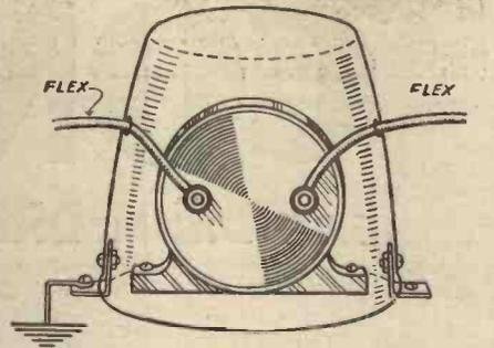
An efficient improvised screen for small H.F. chokes.
