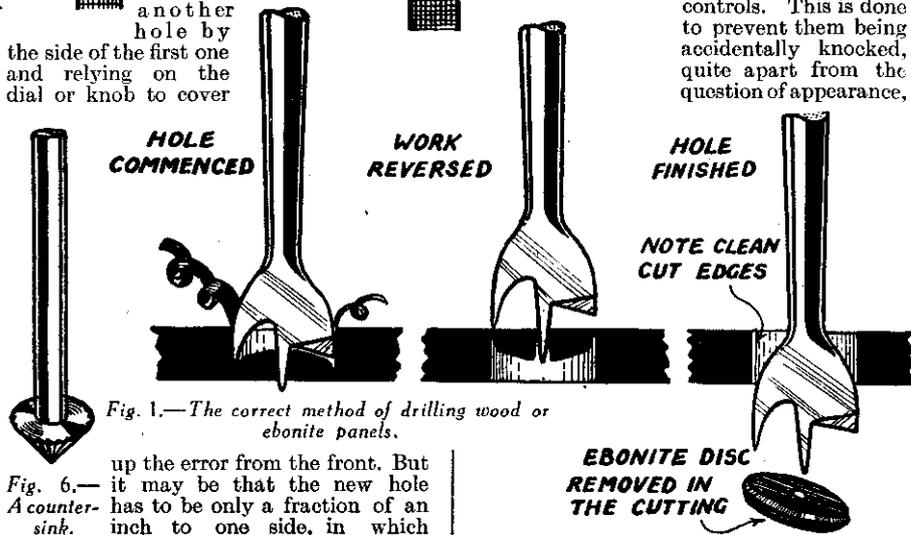
Fig. 1.—The correct method of drilling wood or ebonite panels.
