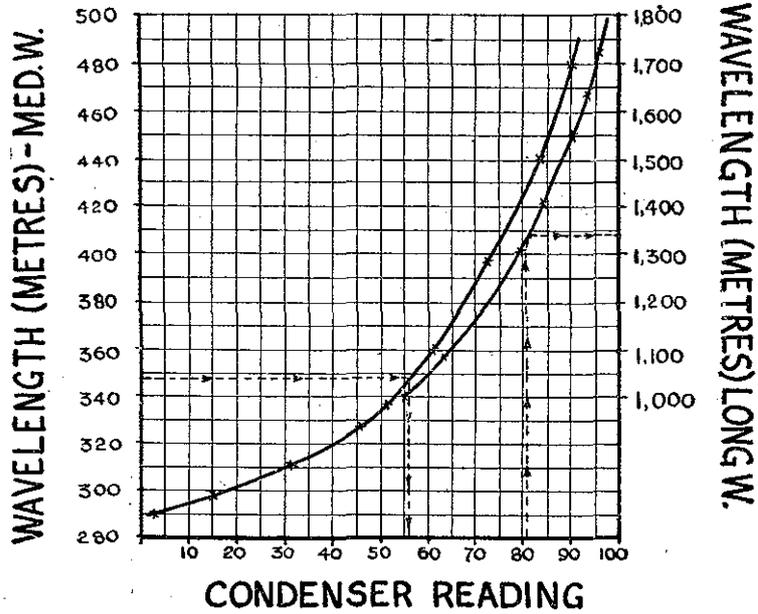
Fig. 5.—How to draw a calibration chart.
