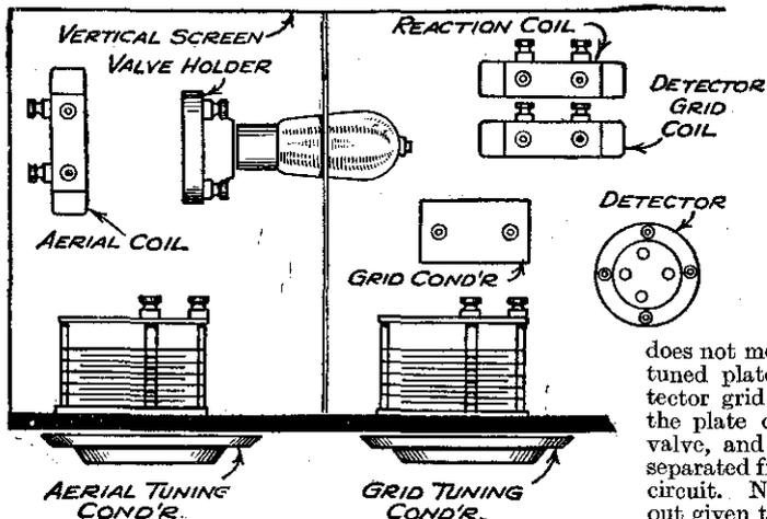
Fig. 1.—The layout of the H.F. stage.
