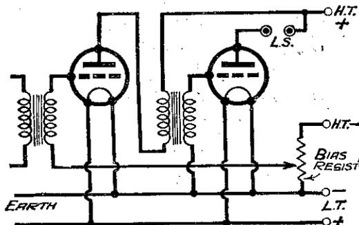
Fig. 6.—A common resistance connected up to provide bias for two battery-heated valves.
