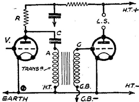
Fig. 2.—The method of parallel-feeding a transformer.
