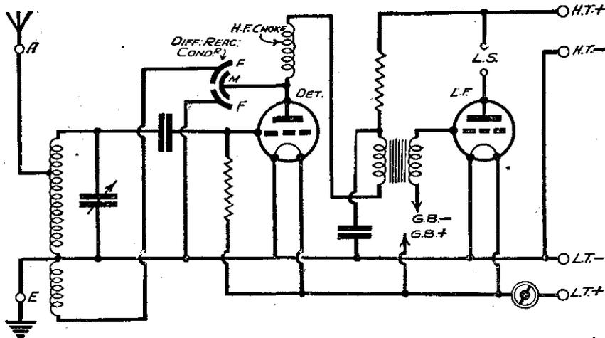
Fig. 2.—Circuit of a two-valve receiver.
