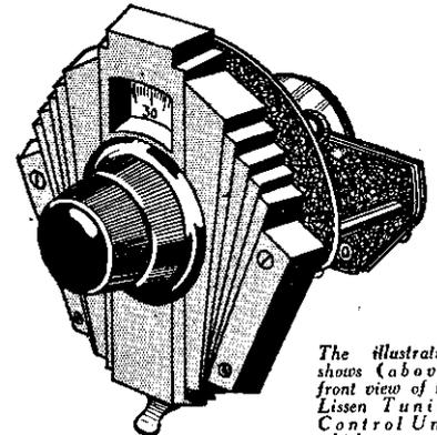
The illustration shows (above) front view of the Lissen Tuning Control Unit which was described last week. The rear view (below) shows the arrangement of the two condensers and the switch contacts. The operating lever can be seen below the dial.
