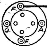
Fig. 4.—Always earth the filament terminal shown so that valves of the metallised type may be interchanged.
