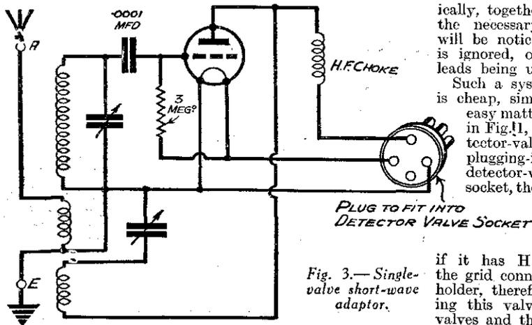
Fig. 3.—Single-valve short-wave adaptor.
