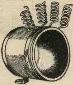
Fig. 1.—The single layer wound solenoid coil.
