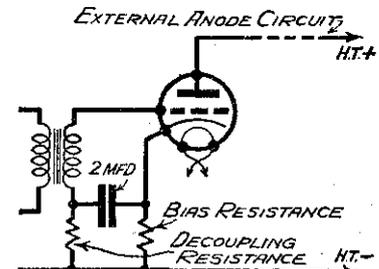
Fig. 2.—The arrangement of Fig. 1 with a de-coupling circuit added.
