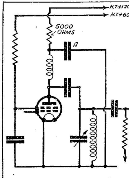
Fig. 4.—S.G. stage decoupled.
