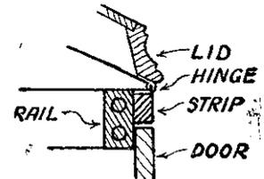
Fig. 16.—How the lid is hinged.
