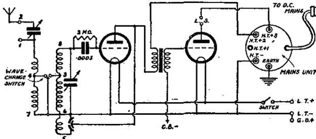
Fig. 1.—The circuit of the battery set before conversion.
