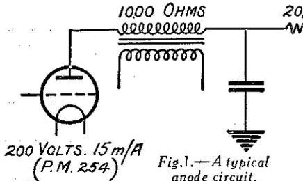
Fig. 1.—A typical anode circuit.
