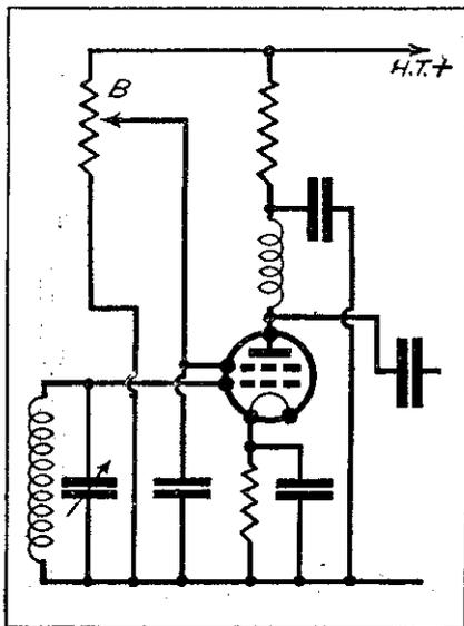
Fig. 5.—With the usual arrangement of a mains set the potentiometer acts as a decoupler.
