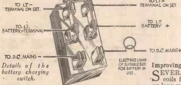
Details of the battery charging switch.
