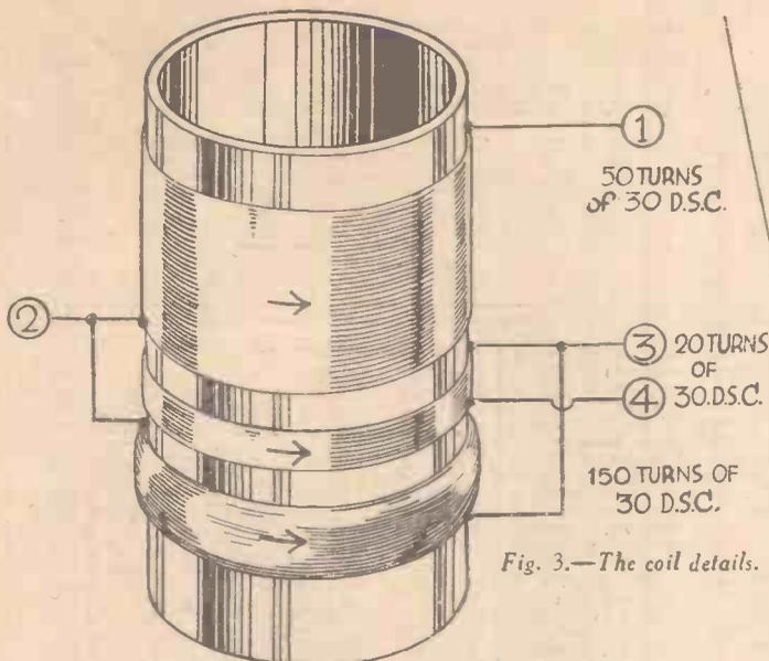
Fig. 3.—The coil details.
