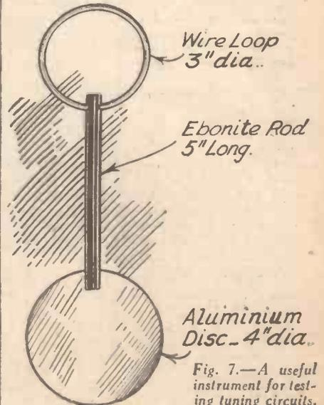
Fig. 7.—A useful instrument for testing tuning circuits.
