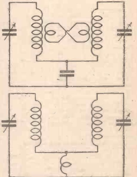
Fig. 4.—Inductive coupling between circuits.
