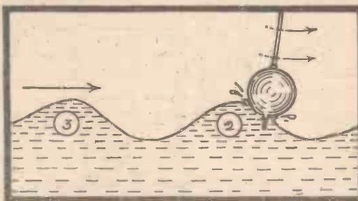
Fig. 7.—A further impetus is given to the pendulum by the next wave.
