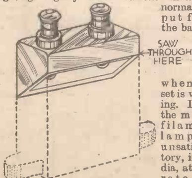
By cutting the top off a fixed condenser as shown it will make a useful terminal block.
