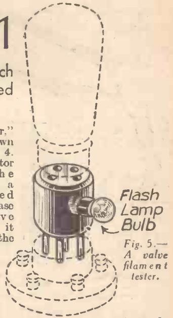
Fig. 5.—A valve filament tester.
