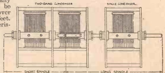
spindle is gripped by one of the grub screws of the middle condenser. The resultant assembly is quite rigid, and has remained so for some time.—F. J. HAYWARD (New Malden).
