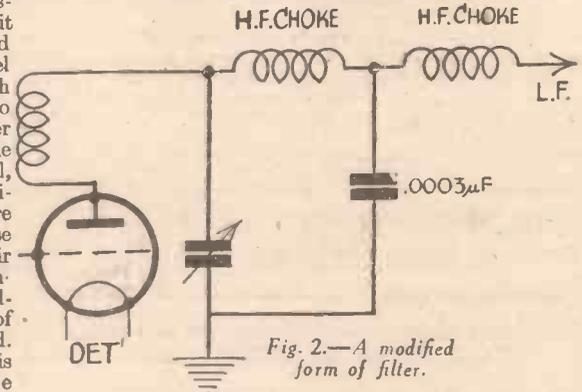
Fig. 2.—A modified form of filter.
