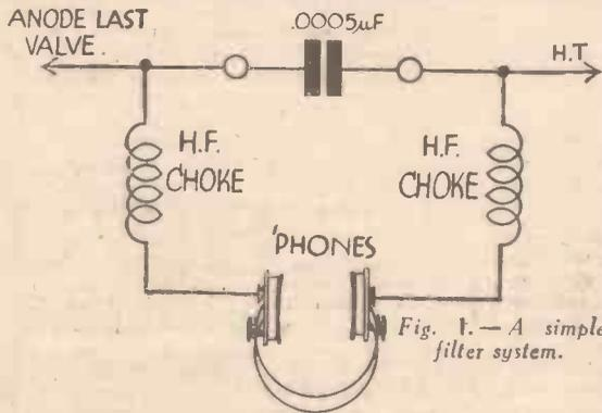
Fig. 1.—A simple filter system.
