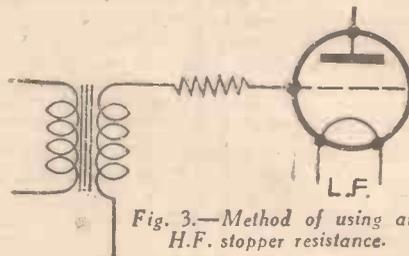
Fig. 3.—Method of using an H.F. stopper resistance.
