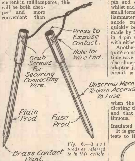
Fig. 6.—Test prods as referred to in this article.
