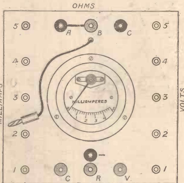
however, and that is—in case of doubt plug into socket No. 5 and get some idea of the amount of current flowing, before coming down to the correct socket.
