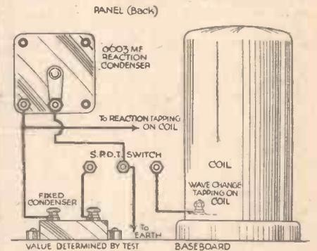
Adding reaction on the long waves to modern tuning coils.
