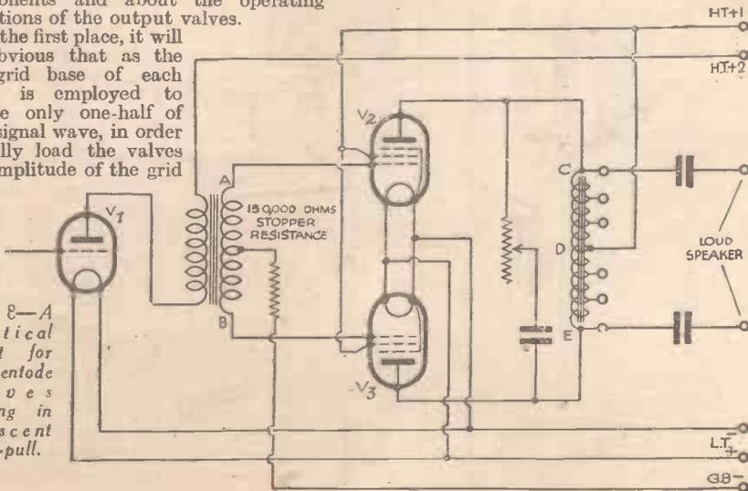
loud-speaker being disconnected accidentally and thus to restrict the extent to which the high peak voltages will be generated. For ordinary pentode valves the value of the protective resistance may be from 20,000 to 25,000 ohms, and for low-consumption pentode valves from 40,000 to 50,000 ohms. The condenser, which should be of the mica dielectric, may be of about .01 mfd.
