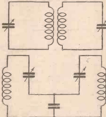
Fig. 1 (a) and (b)—Two methods of coupling two tuned circuits.
