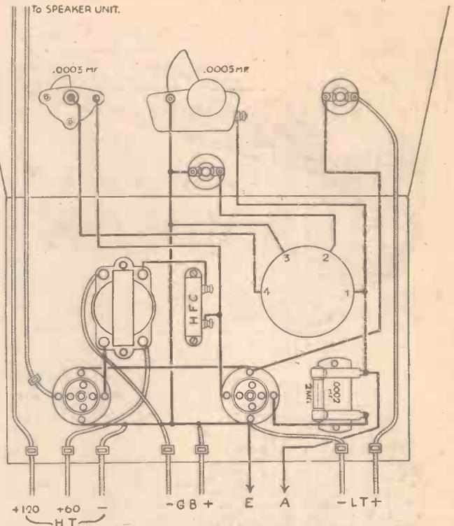
Fig. 4.—Wiring diagram of the Stand-by Two.
