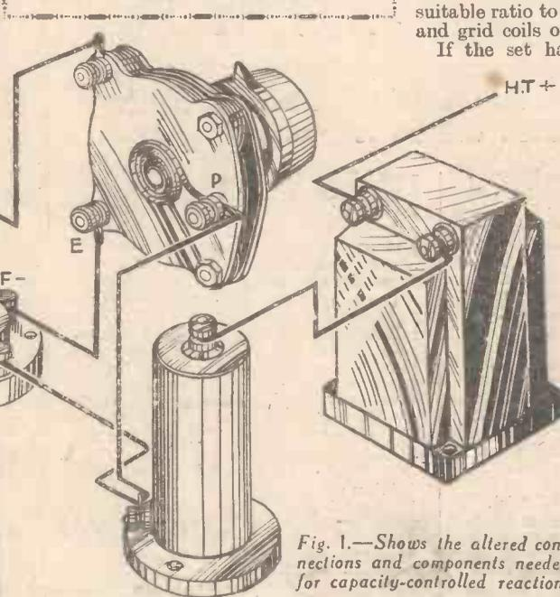
Fig. 1.—Shows the altered connections and components needed for capacity-controlled reaction.
