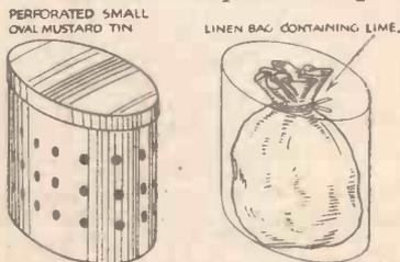
How to keep the inside of a receiver cabinet free from dampness.
