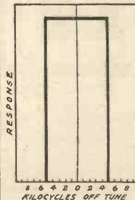
Fig. 2.—Ideal "curve" for a band-pass tuner.
