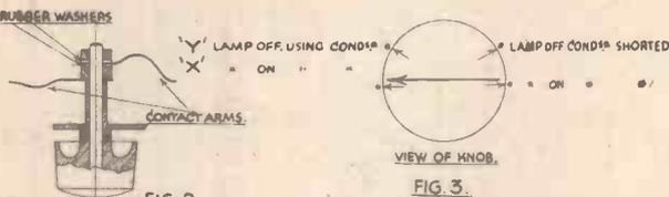
A multi-control switch made from an old rheostat.
