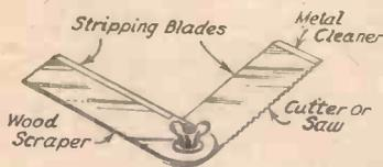
A handy tool made from parts of a hack-saw blade.
