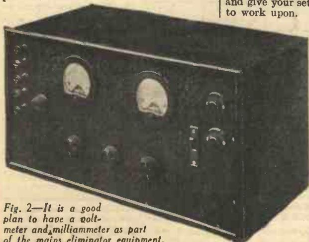
Fig. 2.—It is a good plan to have a voltmeter and milliammeter as part of the mains eliminator equipment.
