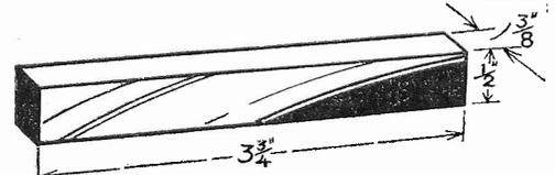
Fig. 5.—The supports, and method of fixing to the end pieces.
