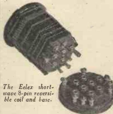
The Eelex short-wave 8-pin reversible coil and base.
