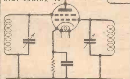
Fig. 1.—Circuit arrangement of bi-grid valve.
