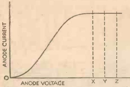
Fig. 4—Anode-volts anode-current curve of two-electrode valve.
