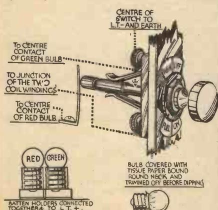
Fig. 1.—A switching arrangement for controlling dial lights.
