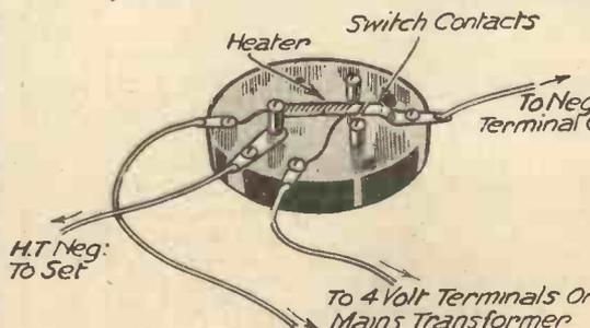
Fig. 13.—The connections for a thermal delay switch.
