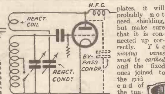
potential, acting as a condenser in conjunction with the wire of the coils, the other. If it has ebonite end plates, then the moving vanes should still be earthed, but make sure that the heads of any bolts passing through the end plates do not touch the shield. Keep them clear of the shield by means of washers, as in Fig. 5.
