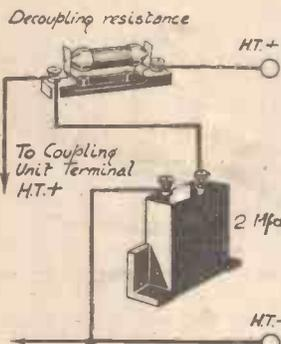
Fig. 2.—D:coupling connections.
