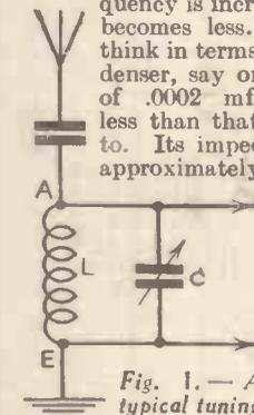
Fig. 1. — A typical tuning circuit. As the capacity of C is reduced a smaller "load" is placed on L, so that the impedance between points A and B becomes greater.
