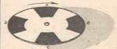
Fig. 2.—The simplest illustration of a stroboscope.
