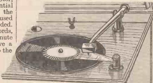
Fig. 3.—The gramophone equipped for speed identification.
