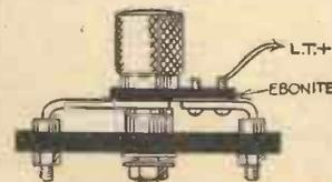
completed switch is screwed to the back of the baseboard alongside the earth terminal, or the earth terminal could be mounted on the same piece of ebonite as the switch. —C. E. HOLDUP (Finchley).
