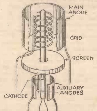
Fig. 4.—Showing the form of construction of a double-diode triode valve.
