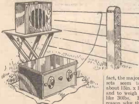
Fig. 2.—Using a wire fence as a temporary aerial.
