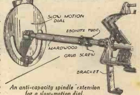
*An anti-capacity spindle extension for a slow-motion dial.*
