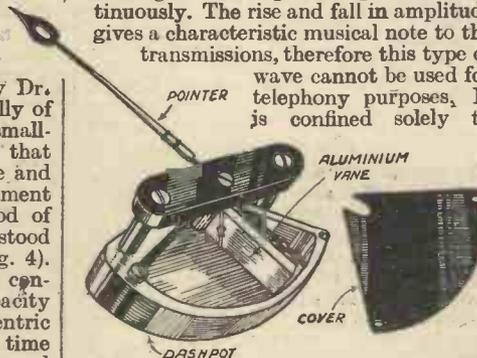
Fig. 7.—How a moving iron type of instrument can be damped.
