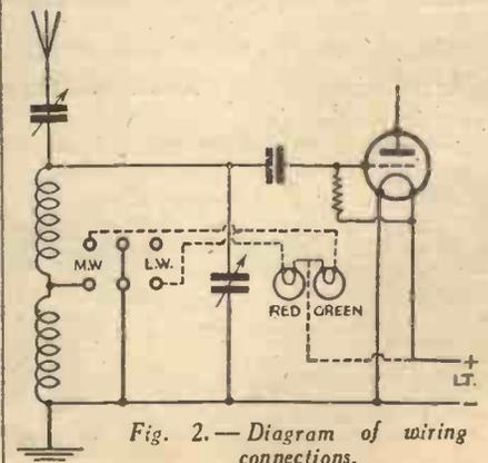
Fig. 2.—Diagram of wiring connections.
