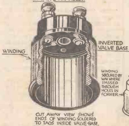
Using an old valve base as a choke former.
