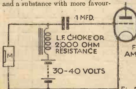
Fig. 5.—How the microphone should be connected in the grid circuit.
