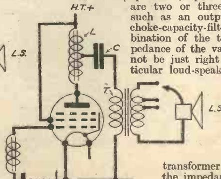
Fig. 5.—A combination of choke and transformer coupling.
