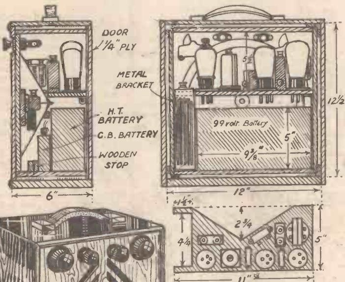
Fig. 5.—Sectional drawings showing the interior arrangements.
