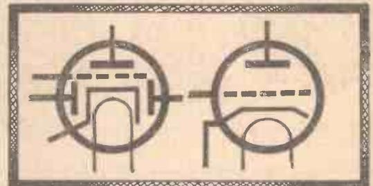
Fig. 3.—Circuit diagram of double-diode-triode compared with that of an ordinary triode.
