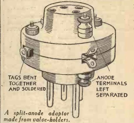
A split-anode adaptor made from valve-holders.
