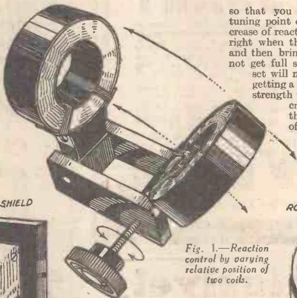
Fig. 1.—Reaction control by varying relative position of two coils.
