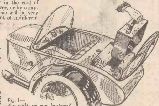
Fig. 1—A portable set may be stowed in a side-car locker if packed round with resilient material such as blankets or coats.
