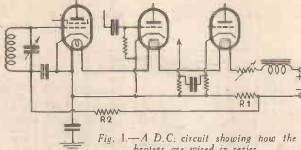
Fig. 1.—A D.C. circuit showing how the heaters are wired in series.
