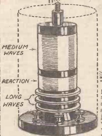
your hand forming one plate and the coils the other. A similar effect may also occur between your hand and the tuning condenser, especially if the latter is of an old pattern in which the fixed vanes instead of the moving ones are connected to the end plates.
