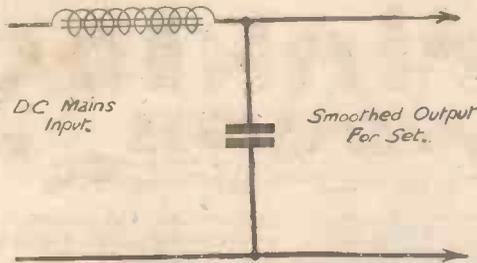
Fig. 4—A simple smoothing circuit for D.C. mains.
