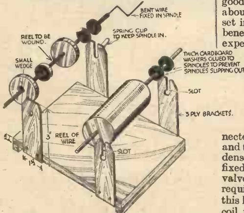
A simple machine for winding chokes and coils.
