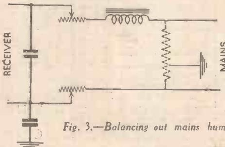
Fig. 3.—Balancing out mains hum.
