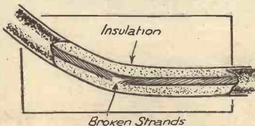
Fig. 2.—Flexible wire fractured inside the rubber covering.
