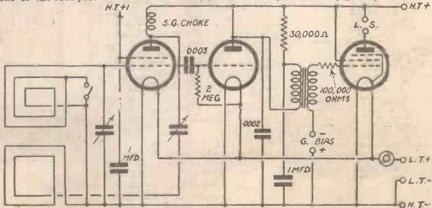
Fig. 7.—The circuit of the lightweight portable described in this article.
