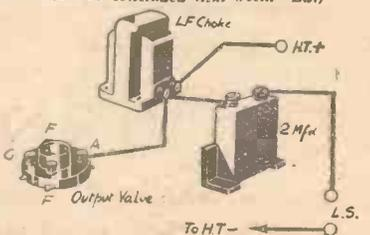
Fig. 7.—Choke output connections.
