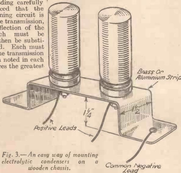
Fig. 3.— An easy way of mounting electrolytic condensers on a wooden chassis.
