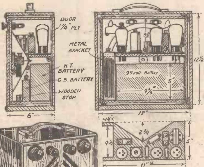
Fig. 5.—Sectional drawings showing the interior arrangements.
