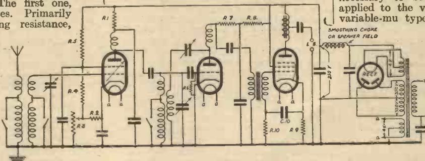
Fig. 1.—Circuit of a typical all-mains receiver showing the various resistances employed. The text deals with the function and value of each.
