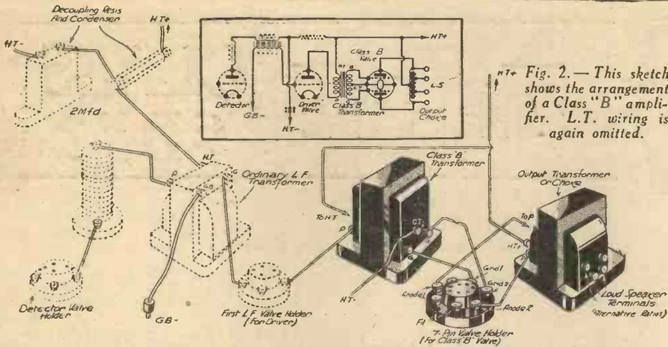
Fig. 2.— This sketch shows the arrangement of a Class "B" amplifier. L.T. wiring is again omitted.
