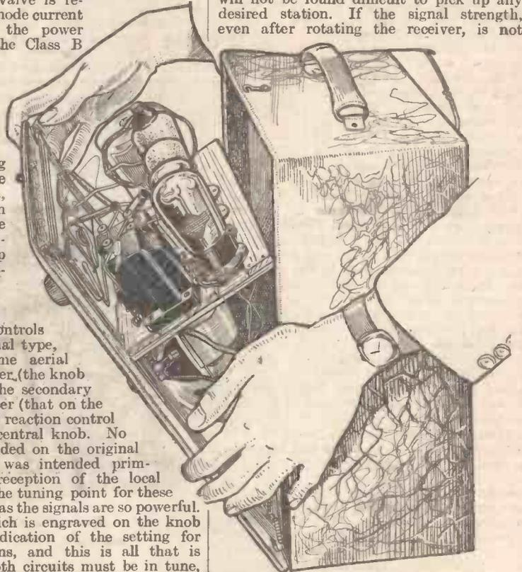
sufficient, the central control should be adjusted to bring the signals to the desired strength. As I pointed out last week, should any adjustments be necessary, the swing hook is simply released and the front of the cabinet lowered when all parts are immediately brought within your reach, and there is no part which is inaccessible.
