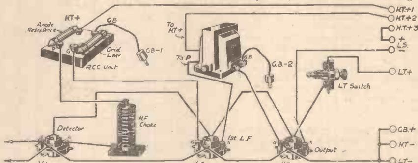
Fig. 1.—L.F. portion of typical battery-fed receiver.
