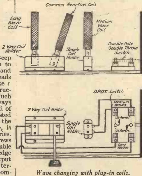
the method illustrated the only drawback attached to the use of these coils is removed. The only extras required are a double-pole double-throw switch, and a single coil holder. The single coil holder (which accommodates the medium-wave coil) is screwed to the baseboard about
