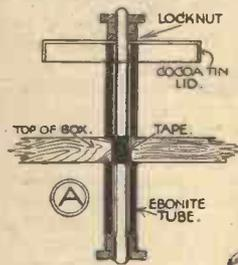
the insulating tape is in the hole, as in sketch A. Treat all three lead-in tubes the same, with the exception of the top one, which has the cocoa-tin lid threaded on in addition under the
