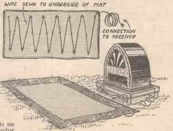
Fig. 3.—How a capacity earth can be arranged by sewing a length of wire to the underside of a car mat.
