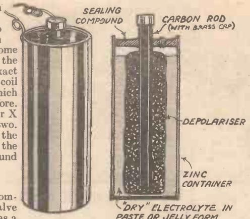
Fig. 5.—Cell of a dry battery showing construction.
