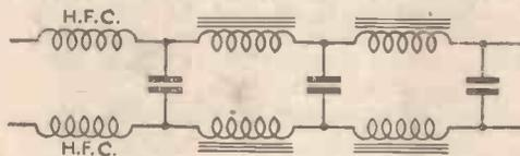
Fig. 2.—An elaborate smoothing circuit for a D.C. mains supply.
