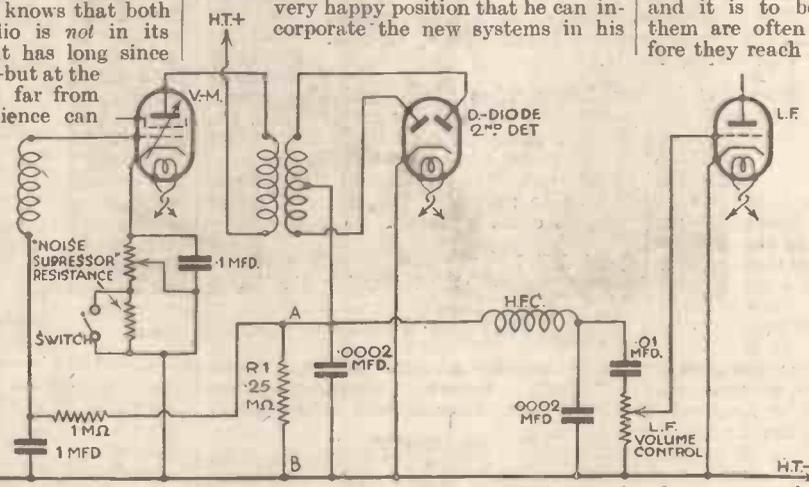
Fig. 1.—An automatic volume control arrangement which is employed in commercial superheterodynes. Notice the "noise suppressor" resistance used for quiet automatic volume control (or A.V.C.).
