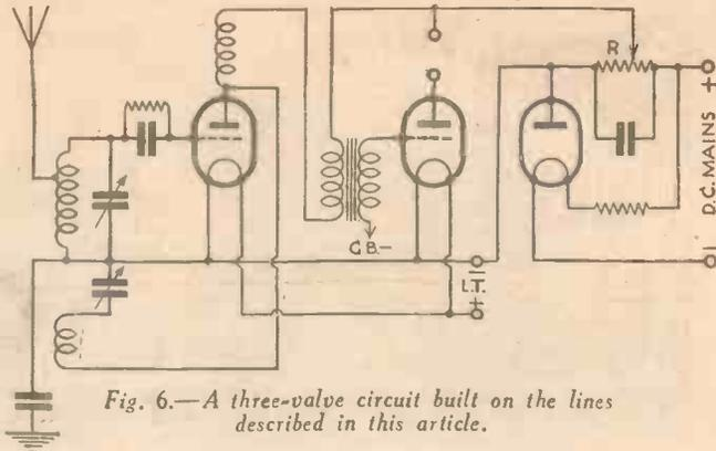
Fig. 6.—A three-valve circuit built on the lines described in this article.
