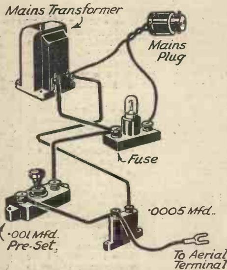
Fig. 1.—The method of eliminating interference with a mains aerial.
