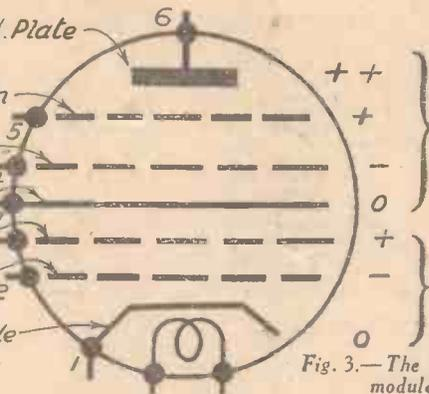
Fig. 3.—The Hexode oscillator-modulator valve.
