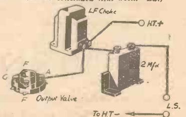
Fig. 7.—Choke output connections.
