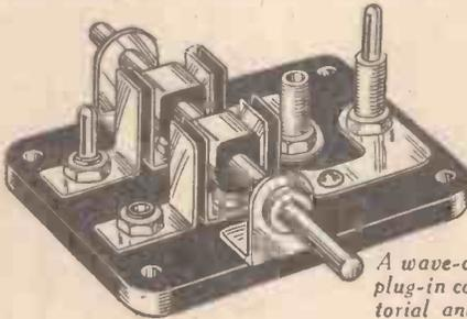
A wave-change switch for plug-in coils shown in pictorial and sectional view.
