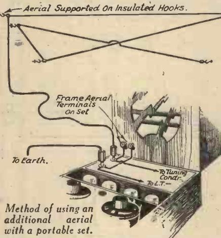
Method of using an additional aerial with a portable set.
