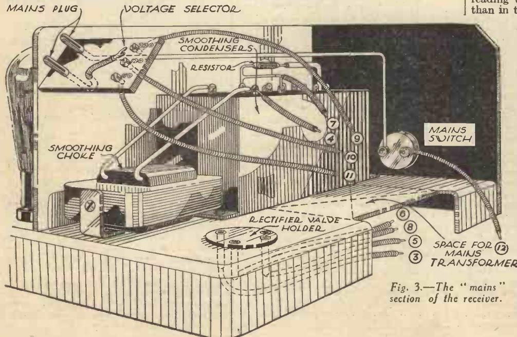
Fig. 3.—The "mains" section of the receiver.
