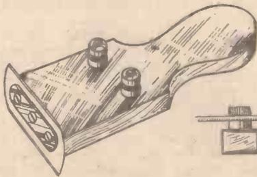
A handy tool for removing the insulation from connecting wire.
