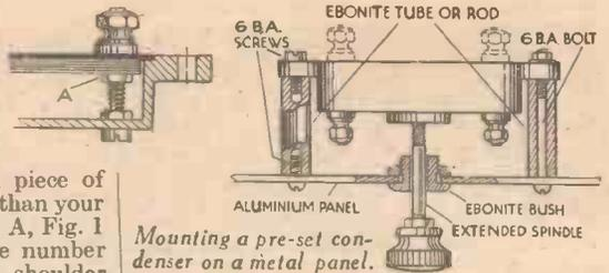
Mounting a pre-set condenser on a metal panel.
