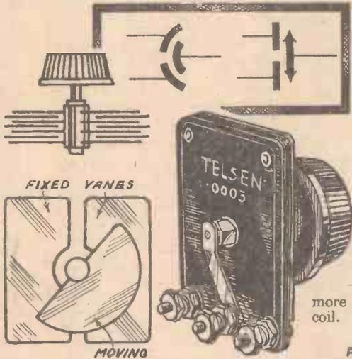
Fig. 1.—The essential parts of a differential condenser (left) and the actual component (right). Inset:—The conventional signs used to denote a differential condenser.
