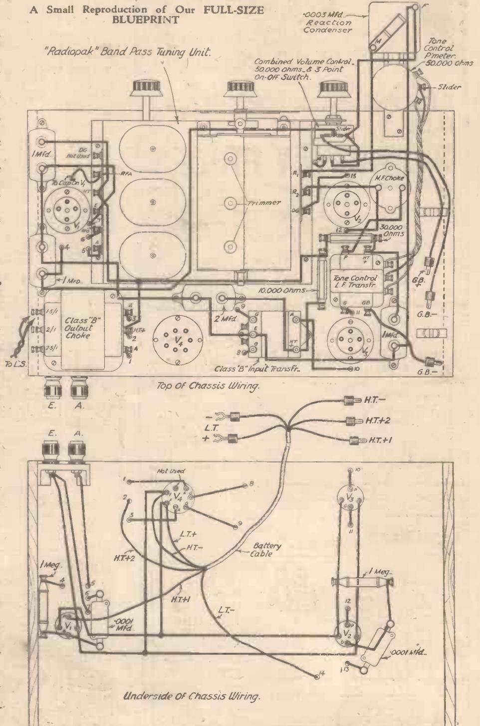
Top and Sub-baseboard Wiring Diagram of the Radiopax "Class B" Four. A full-size Blueprint can be obtained for 1s. post free from George Newnes, Ltd., 8-11, Southampton Street, Strand, London, W.C.2.
