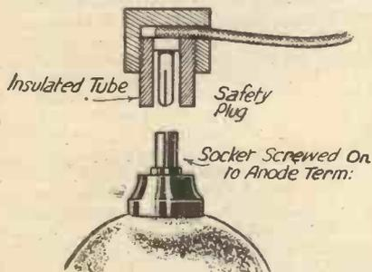
Fig. 11.—A safety anode connector.
