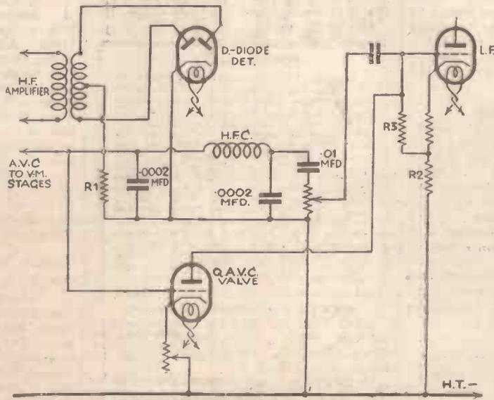
Fig. 2.—A method of obtaining quiet automatic volume control. When the set is "off tune" the Q.A.V.C. valve draws current through R.3 and so over-biases the L.F. amplifier.
