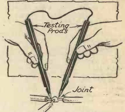
Fig. 5.—Bridging a joint to test a soldered connection.
