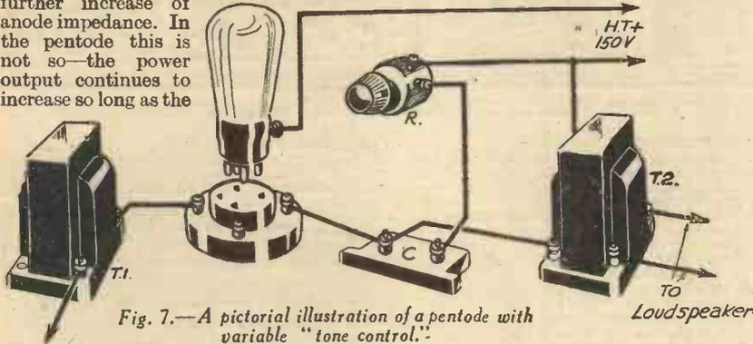
Fig. 7.—A pictorial illustration of a pentode with variable "tone control."
