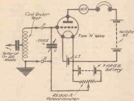
Fig. 2.— A simple method of comparing the efficiencies of coils.
