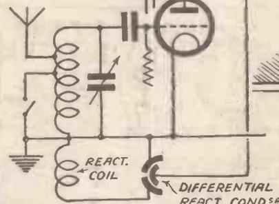
Fig. 8.—Circuit using differential control, also a typical differential condenser.
