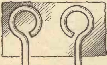
Fig. 2.—The correct method of making a loop to avoid looseness.
