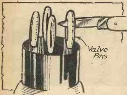
Fig. 6.—The old type valve legs should be opened to ensure a tight fit in the socket.
