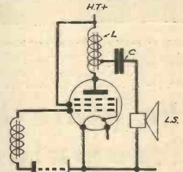
Fig. 4.—A choke filter output.
