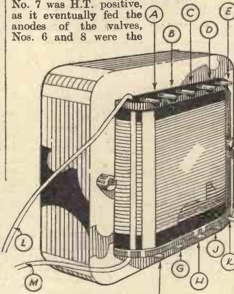
Fig. 1.—The transformer as sent from the makers.
