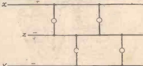
Fig. 6—How the three-wire D.C. system is arranged.
