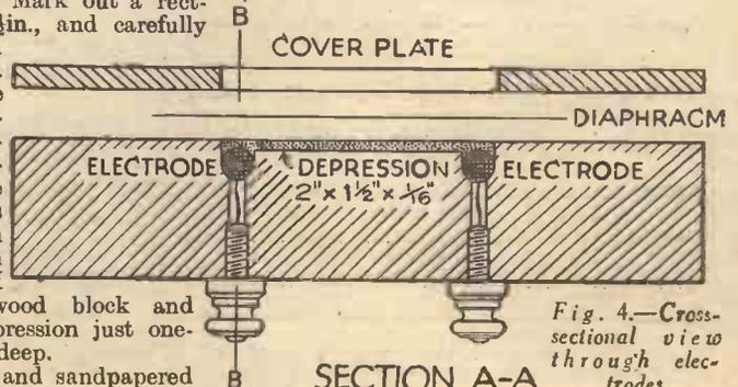
Fig. 4.—Cross-sectional view through electrodes.
