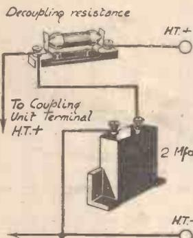
Fig. 2.—D:coupling connections.
