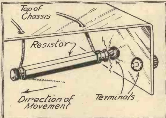
Fig. 1.—Slack leads allowing a resistor to short circuit against a metal chassis.
