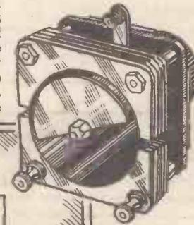
advantage over the former in that the capacity between plate and filament remains constant, whatever the setting of the condenser, therefore, there is no chance of attenuation of the high notes with increase of reaction. In practice, however, there is really nothing between the two arrangements as with that shown in Fig. 7.
