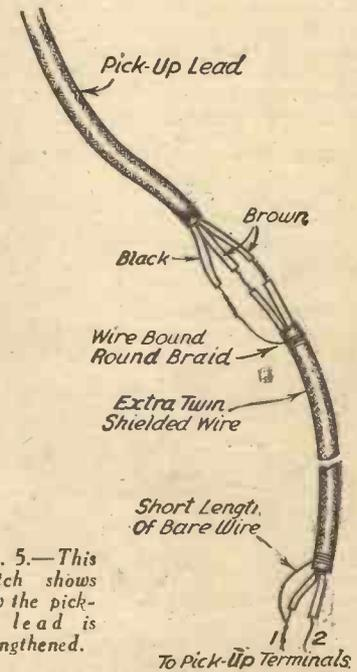
Fig. 5.—This sketch shows how the pick-up lead is lengthened.
