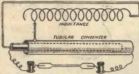
Fig. 4.—Diagrammatic representation of the essential parts of a cymometer.
