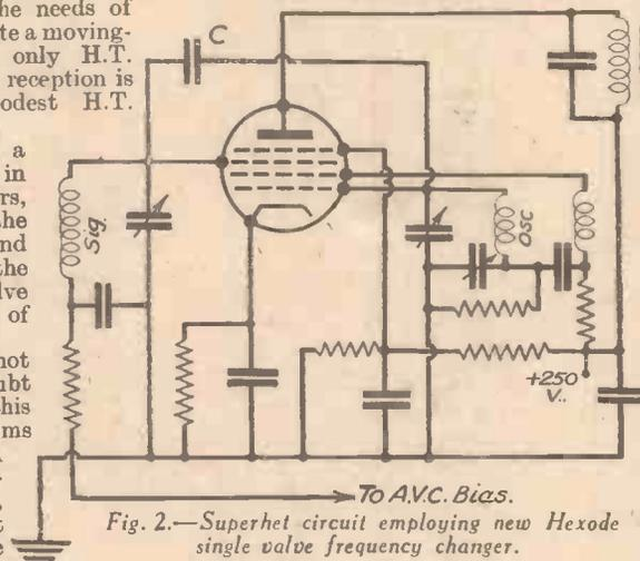
Fig. 2.—Superhet circuit employing new Hexode single valve frequency changer.
