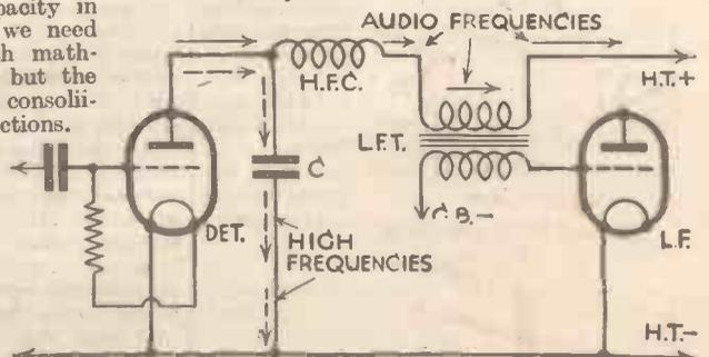
Fig. 2.—The anode circuit of a detector valve where high and low frequencies have to be separated. The H.F. choke passes the low frequencies and condenser C the high frequencies.
