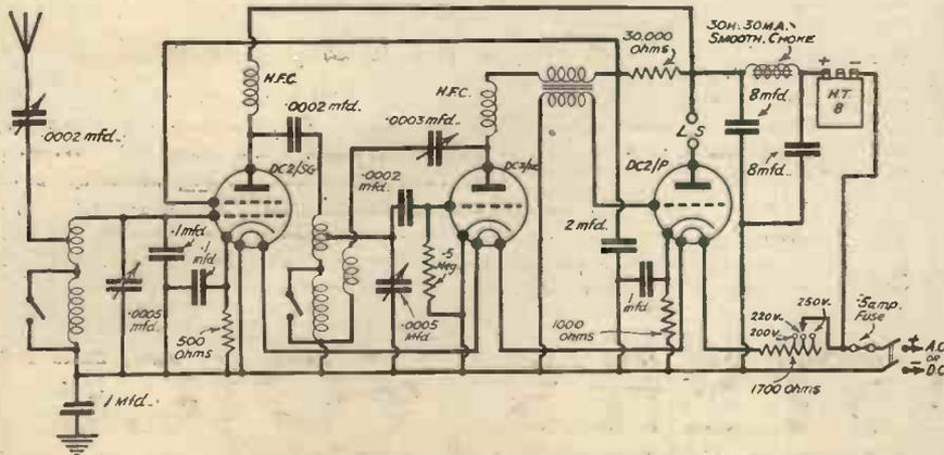
Fig. 2.—The circuit of an S.G.-Det.-P. Universal (A.C. or D.C.) receiver using standard D.C. valves.
