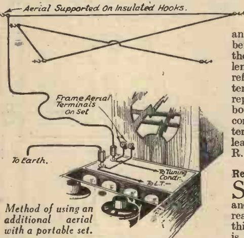
Method of using an additional aerial with a portable set.
