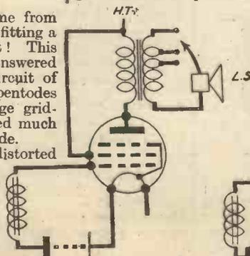
Fig. 3.—A pentode output transformer.
