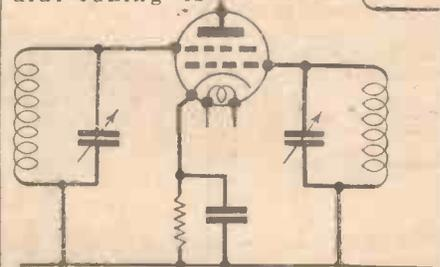
Fig. 1.—Circuit arrangement of bi-grid valve.
