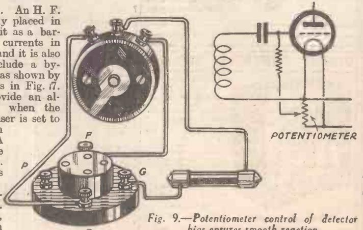
Fig. 9.—Potentiometer control of detector bias ensures smooth reaction.
