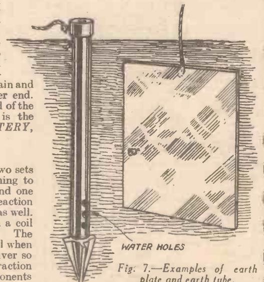
Fig. 7.—Examples of earth plate and earth tube.
