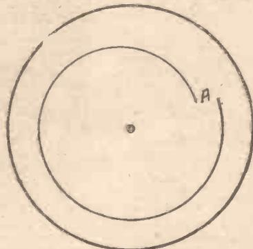
Fig. 3.—The scanning disc and hole spiral. The direction of rotation is anti-clockwise.
