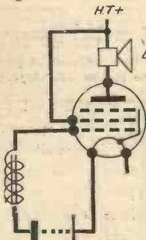
Fig. 2.—A direct anode connection.
