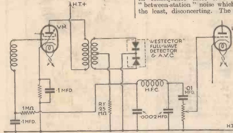
Fig. 3.—This circuit shows how a full-wave "Westector" can be employed as second detector and A.V.C. in a superheterodyne. Compare the arrangement with that of Fig. 1.
