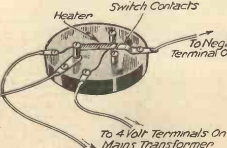
Fig. 13.—The connections for a thermal delay switch.
