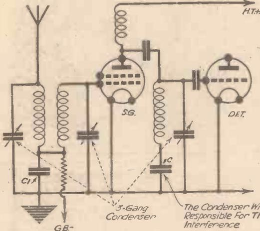
Fig. 1.—Tuning circuits of the set with which a peculiar form of interference was experienced.
