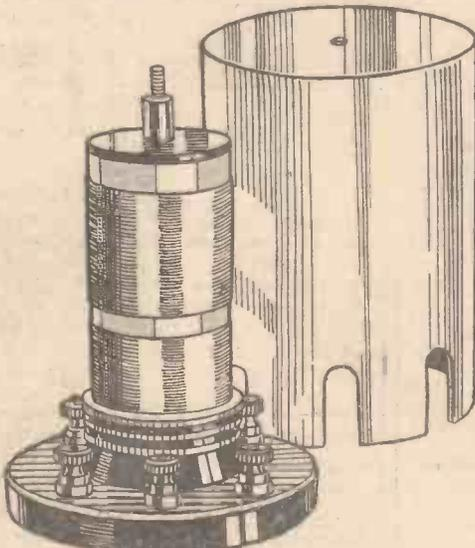
Fig. 6.—A screened dual-range coil.
