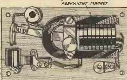
Fig. 2.—Example of a cut-out.
