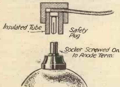
Fig. 11.—A safety anode connector.
