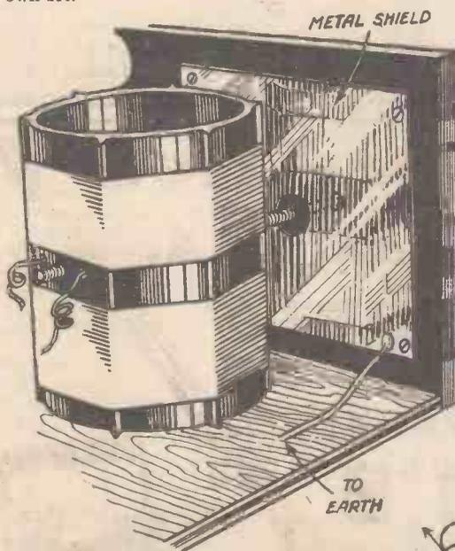
Fig. 4.—Shielding reaction control to prevent hand-capacity effect.
