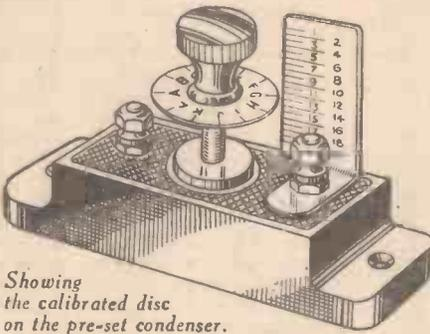
Showing the calibrated disc on the pre-set condenser.
