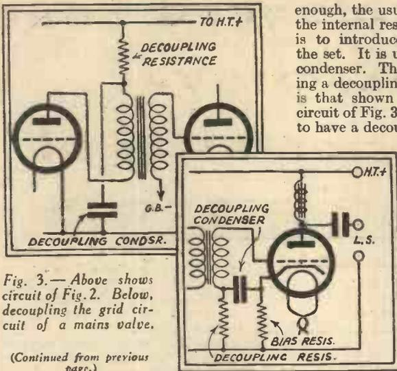
Fig. 3.— Above shows circuit of Fig. 2. Below, decoupling the grid circuit of a mains valve.
