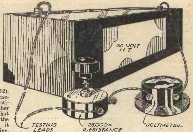
Fig. 2.—The testing equipment.
