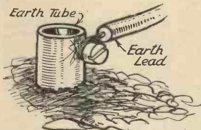
Fig. 7.—Make sure the earth connection is sound.
