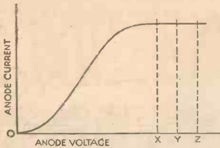
Fig. 4—Anode-volts anode-current curve of two-electrode valve.
