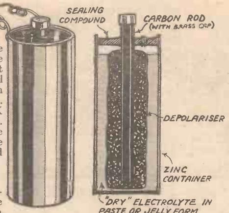
Fig. 5.—Cell of a dry battery showing construction.
