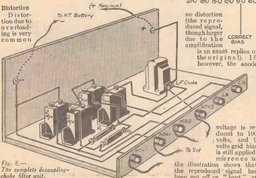
Fig. 8.—The complete decoupling-choke filter unit.
