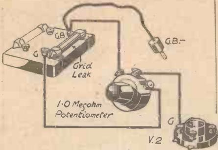
Fig. 4.—Volume control connections.
