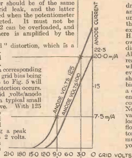
Fig. 6.—Showing danger of under-biasing.
