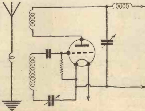
Fig. 2.—An alternative position for the tuning condenser.
