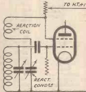
Fig. 10.—Reaction from screening-grid of S.G. detector valve
