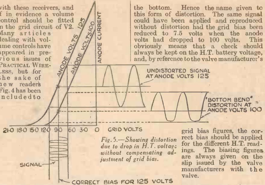
Fig. 5.—Showing distortion due to drop in H.T. voltage without compensating adjustment of grid bias.
