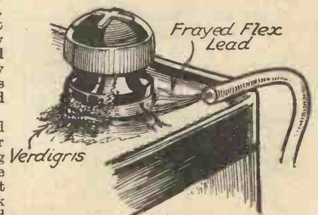
Fig. 4.—The effect of acid splashes and fumes to work loose and jam the screw thread.
