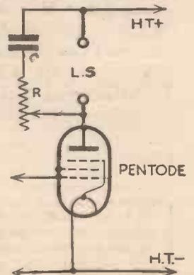
Fig. 4.—The arrangement used to counteract the high note emphasis given by a pentode. The impedance of C and R must be less than that of the speaker at higher audio frequencies.
