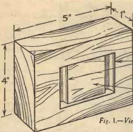
Fig. 1.—View of back block with cover removed.
