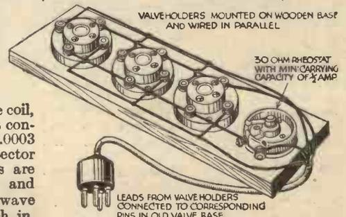
Using old valves as half-wave rectifiers.
