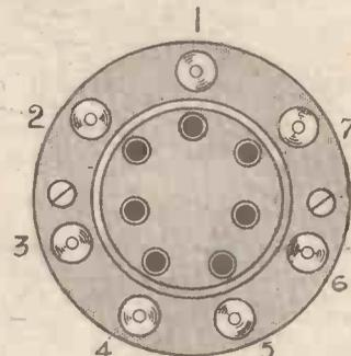
of the valve pins, and the drawing herewith shows the valveholder numbering. The drawing on the Data Sheet in question shows the base of the valve, and, obviously, the numbering is reversed in this case.
