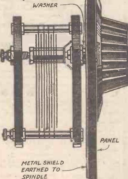
Fig. 5.—Shielding a condenser with ebonite end plates.
