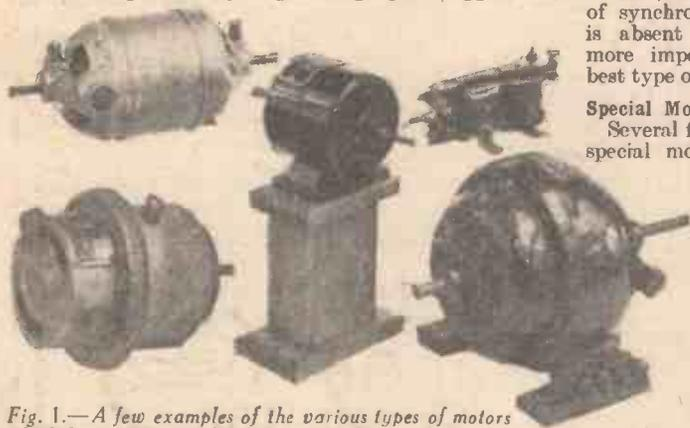
Fig. 1.—A few examples of the various types of motors which have been used for driving the disc at the receiving end.
