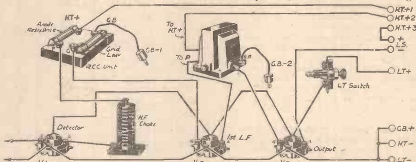
Fig. 1.—L.F. portion of typical battery-fed receiver.
