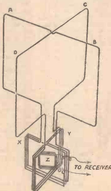
Fig. 2.—Diagram showing the essential parts of a direction finder.
