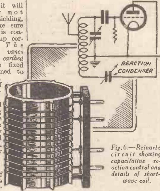
Fig. 6.— Reinartz circuit showing capacitive reaction control and details of short-wave coil.
