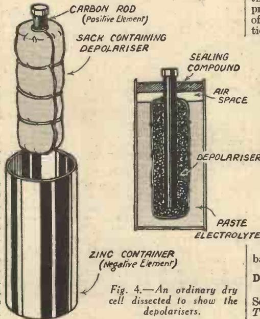
Fig. 4.—An ordinary dry cell dissected to show the depolarisers.
