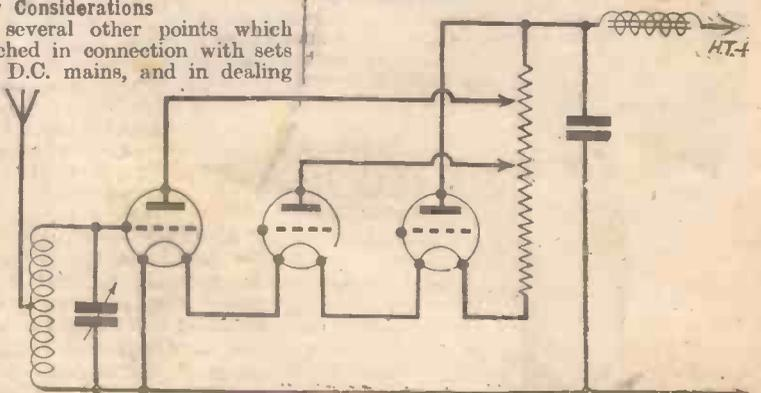
Fig. 7—One method of subdividing H.T. and L.T. voltages in a D.C. receiver. H.T.—
