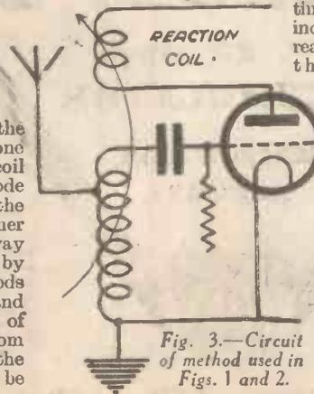
Fig. 3.—Circuit of method used in Figs. 1 and 2.
