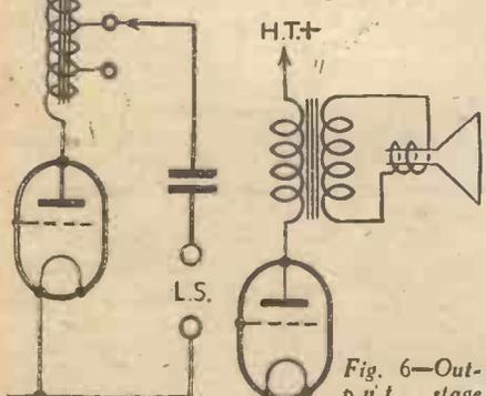
Fig. 5.—Output stage filter-circuit using a tapped choke.
