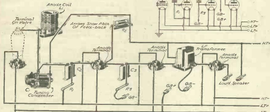
Fig. 1.—Tuned anode, detector, 2 L.F. stages without decoupling. Arrows indicating path of feed-back to grid of detector valve.
