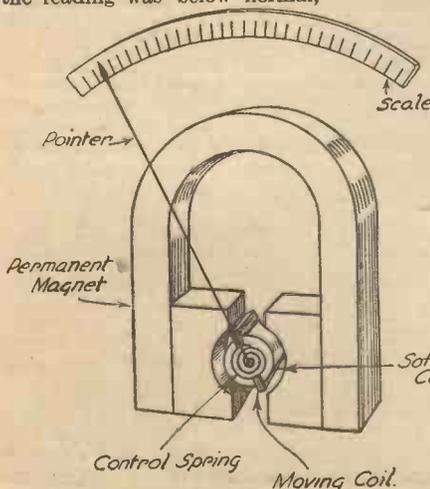
Fig. 3.—Illustrating the elementary principles of a moving-coil instrument.
