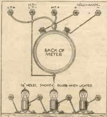
Fig. 2.—Rear view of the tester showing connections.
