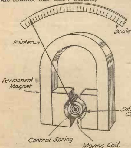
Fig. 3.—Illustrating the elementary principles of a moving-coil instrument.
