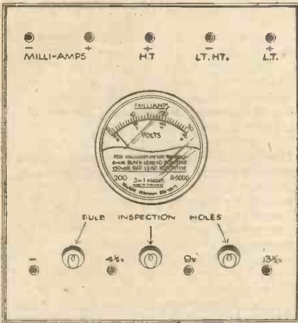
Fig. 1.—Front view of the finished instrument.
