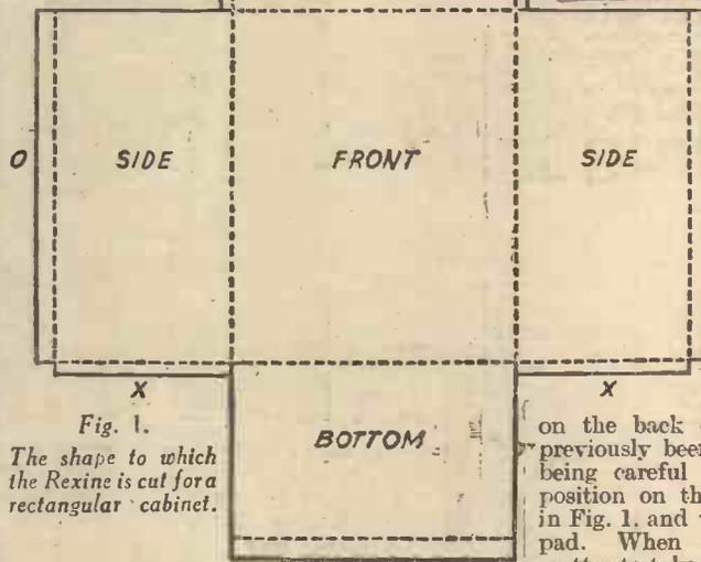
Fig. 1. The shape to which the Rexine is cut for a rectangular cabinet.
