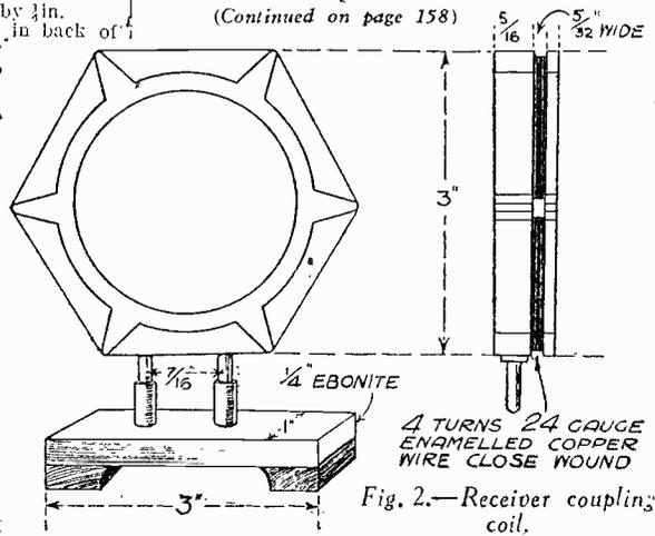
Fig. 2.—Receiver coupling coil.
