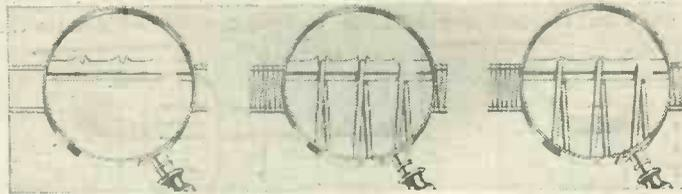
Fig. 5.—How the Cossor Factory overcome grid welding and its attendant disadvantages.
