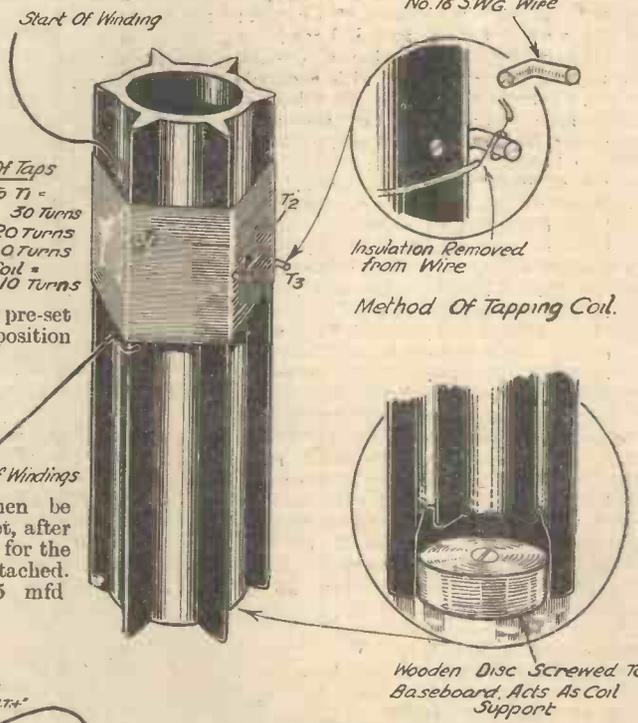
Fig. 4.—All constructional details for the tuning coil may be obtained from the above sketch.
