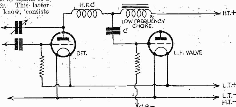
Fig. 21.—Choke-capacity L.F. coupling.
