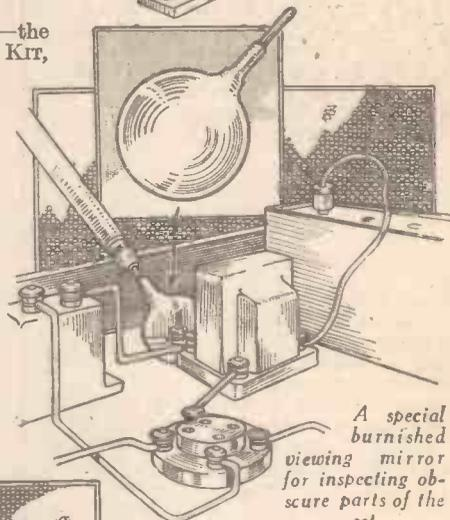
A special burnished viewing mirror for inspecting obscure parts of the set.
