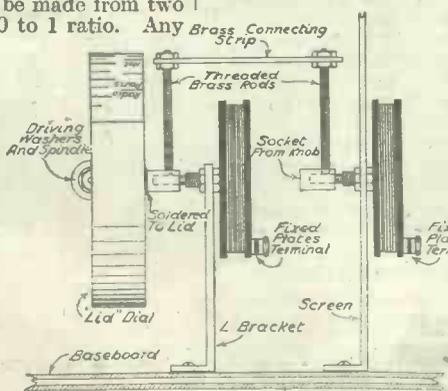
Fig. 1.—Details for making a twin-gang slow-motion condenser.
