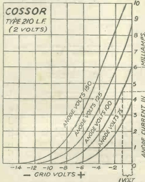
Fig. 3.—The slope can be found by applying one grid volt and noticing the change in milliamps. The slope of the accompanying valve curve shows that one volt (grid) brings about a change in anode current of 1.4 mA. Hence the slope of this valve is 1.4 m.a./V.
