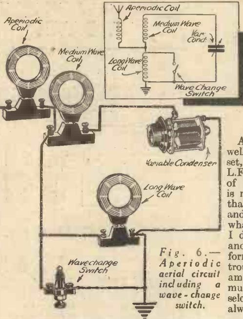
Fig. 6.—Aperiodic aerial circuit including a wave-change switch.
