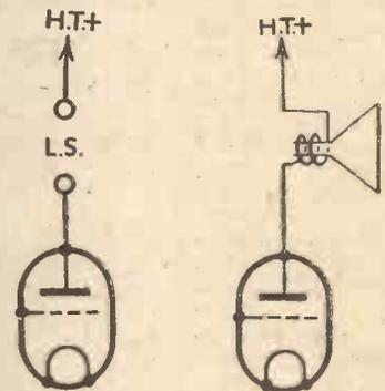
Fig. 1.—A simple output circuit. Fig. 2.—Incorrect method of coupling output valve to moving-coil speaker.
