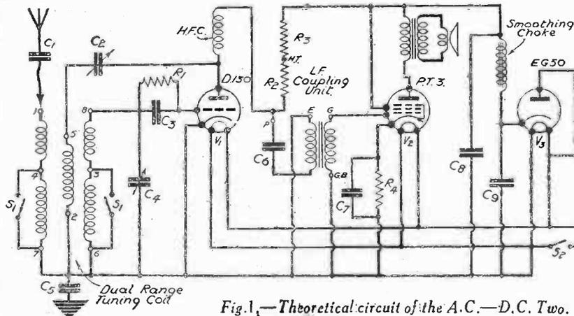
Fig. 1.—Theoretical circuit of the A.C.—D.C. T.W.O.
