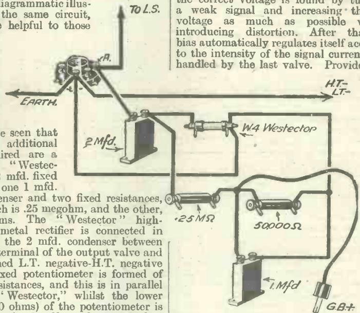
Fig. 1.—This sketch shows how the new components are connected to the output valve-holder.
