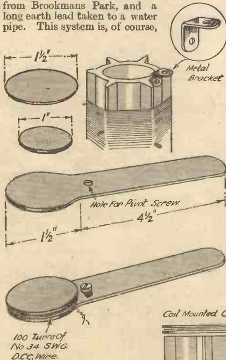
Fig. 2.—All constructional details for the reaction coil and its mounting are given in this sketch.
