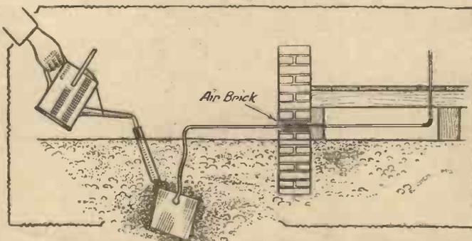
Fig. 2.—Earth plate (or bowl) with tube for watering, and lead from earth taken through air-brick of house and then through hole in floor-board to set.
