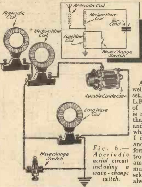
Fig. 6.—Aperiodic aerial circuit including a wave-change switch.
