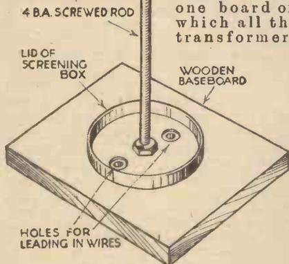
Fig. 1.—Method of attaching lid of screening box to baseboard.
