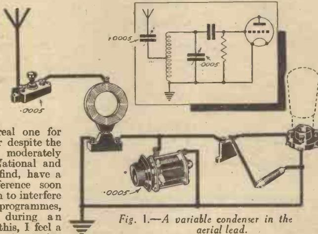
Fig. 1.—A variable condenser in the aerial lead.
