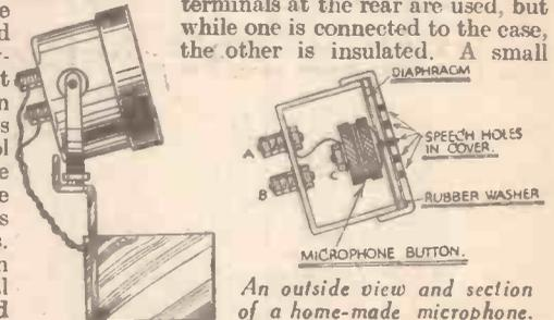
An outside view and section of a home-made microphone.
