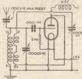
on the baseboard, and is utilized as a coil-holder, the grid terminal being connected to the grid condenser, filament negative terminal to earth, plate terminal to reaction condenser fixed vanes, and the other filament terminal to detector valve anode. The coil is now plugged in, and the aerial clipped on to the top of the grid winding.
