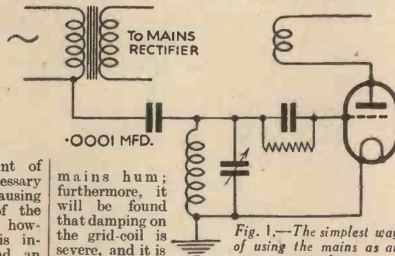
mains hum; furthermore, it will be found that damping on the grid-coil is severe, and it is very doubtful whether good oscillation can be maintained over the tuning range with the aerial con-
