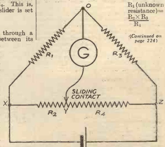
Fig. 1.—The theoretical circuit of the bridge.
