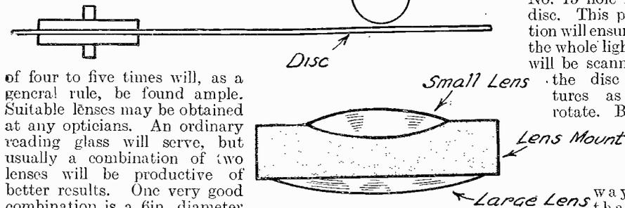
Fig. 1.—Showing the relative positions of disc, neon lamp, and lenses.
