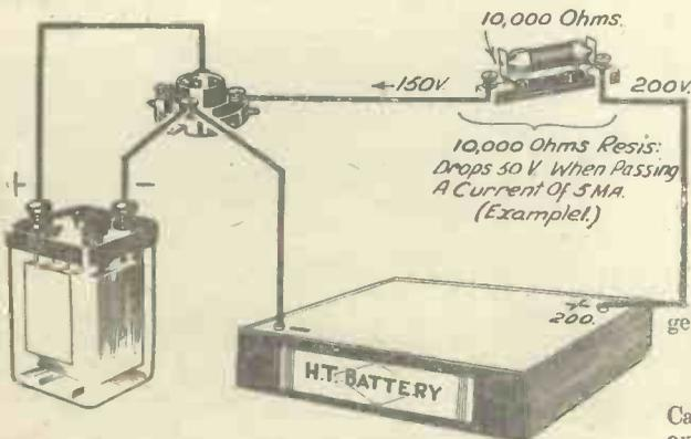
Fig. 3.—Here you see how the anode voltage of a valve may be reduced by inserting a fixed resistance in circuit.
