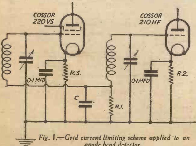
Fig. 1.—Grid current limiting scheme applied to an anode bend detector.
