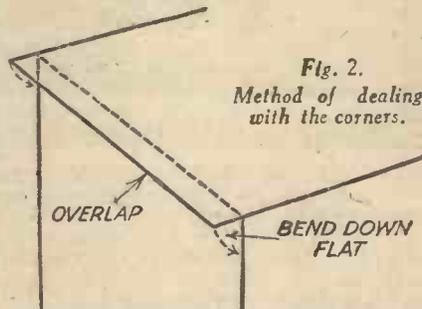
Fig. 2. Method of dealing with the corners.
