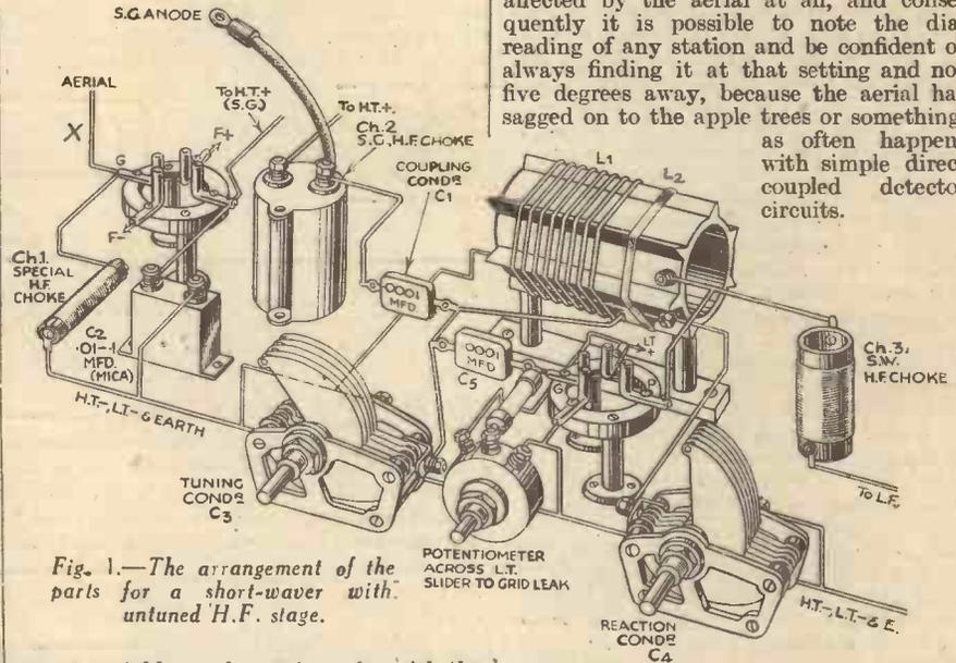
Fig. 1.—The arrangement of the parts for a short-waver with untuned H.F. stage.
