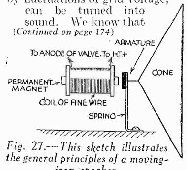
Fig. 27.—This sketch illustrates the general principles of a moving-iron speaker.
