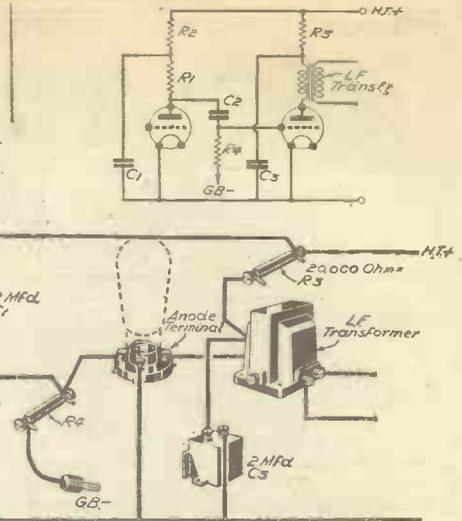
Fig. 3.—Method of decoupling resistance capacity and transformer-coupled low-frequency stages.
