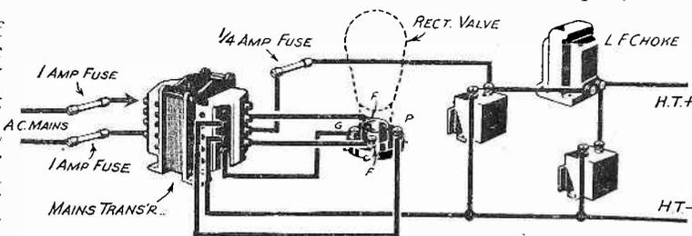
Fig. 15.—A rectifier unit showing suggested position of fuses:
