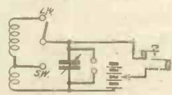
Circuit diagram of buzzer wavemeter.
