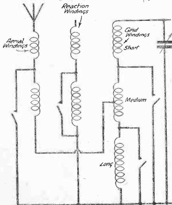
Fig. 2.—A simple arrangement for an all-wave tuner.
