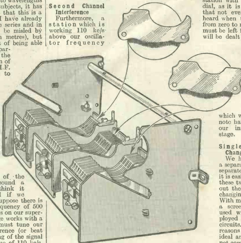
This illustration shows a three-gang condenser, with the top inset showing the special oscillator shaped plates.
