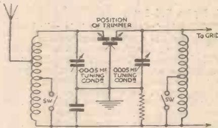
Fig. 2.—A trimmer for 2-gang condensers.
