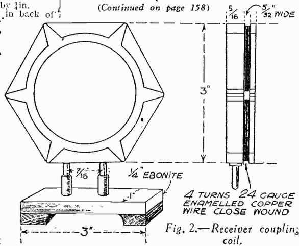
Fig. 2.—Receiver coupling coil.
