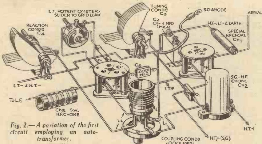
Fig. 2.—A variation of the first circuit employing an auto-transformer.
