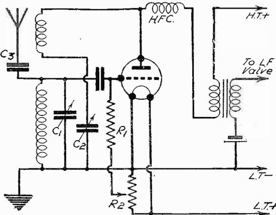
Fig. 1.—A simple reaction arrangement.
