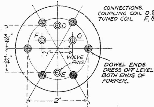
CONNECTIONS. COUPLING COIL D. & E. TUNED COIL F. & G.
