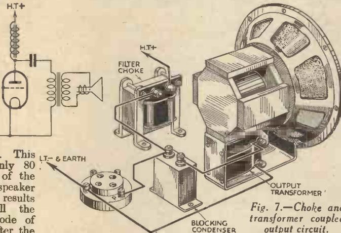
Fig. 7.—Choke and transformer coupled output circuit.
