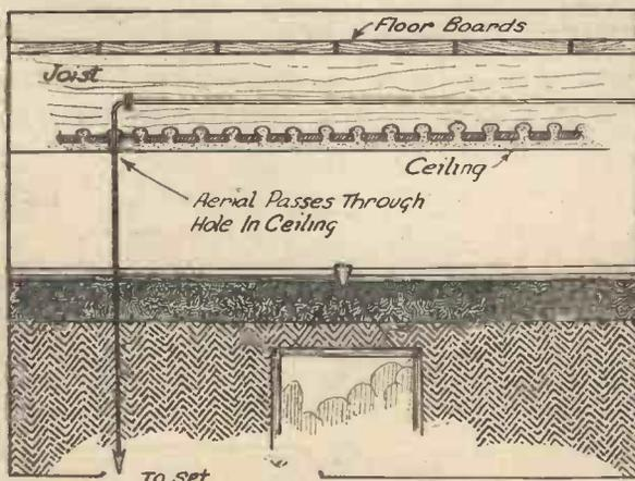
Fig. 4.—Aerial running between ground floor ceiling and floorboards of room above.
