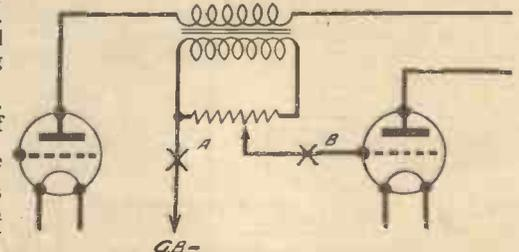
Fig. 6.—Make sure in continuity tests that there is not an alternative current path.
