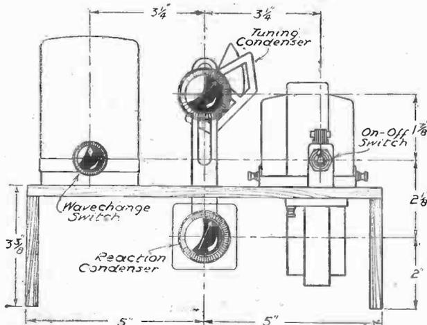
Fig. 2.—Disposition of controls.
