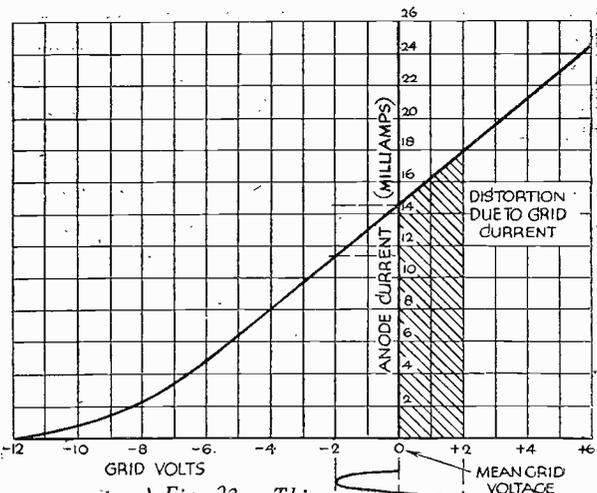
Fig. 23.—This figure shows how distortion occurs when the grid bias voltage is too low.
