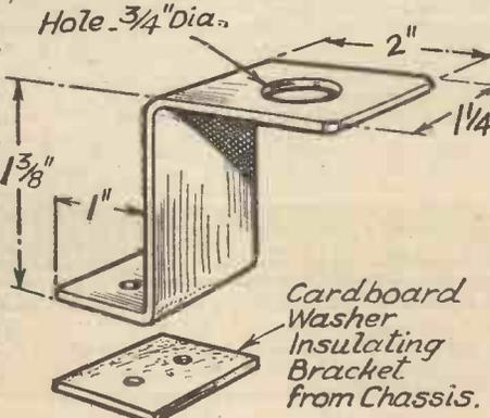
Fig. 1—Details of the condenser brackets.
