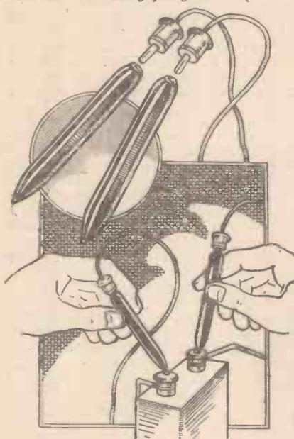
Special insulated test-prods. Note the wander-plug arrangement for the flex—another "Practical Wireless" idea.
