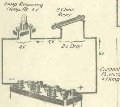
Fig. 2.—Showing how a resistance may be connected to produce a voltage drop.
