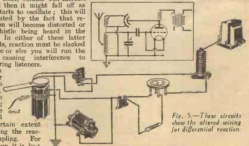
Fig. 5.—These circuits show the altered wiring for differential reaction.
