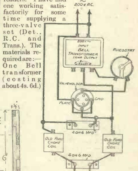
Fig. 1. Wiring diagram for a cheap H.T. eliminator.
