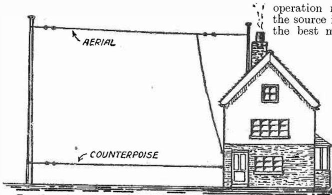
Fig. 5.—A counterpoise is sometimes useful in reducing interference.
