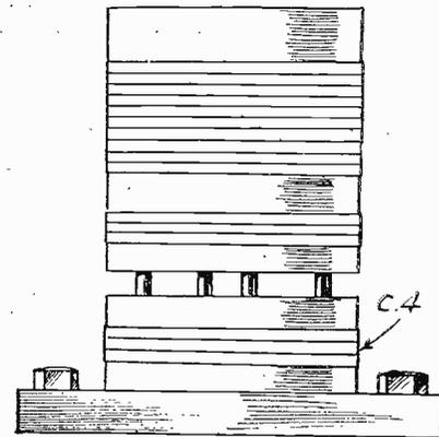
Fig. 4.—Mounting the coupling coil on the same base as the tuning coil.
