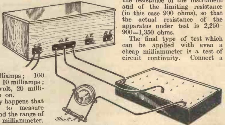
Fig. 4.—A shunt connected in parallel with a milliammeter measures its range.
