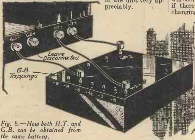
Fig. 8.—How both H.T. and G.B. can be obtained from the same battery.
