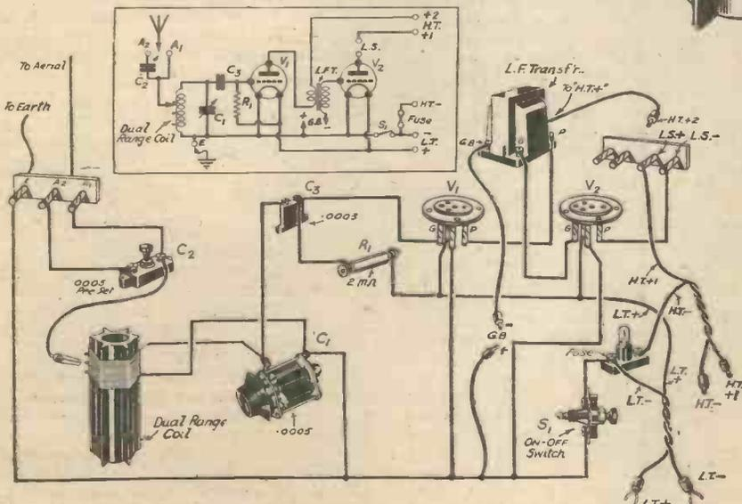
Fig. 5.—Here you have a pictorial circuit diagram, whilst the corresponding theoretical circuit is shown inset. By comparing the two you will be able to improve your knowledge of circuit diagrams.
