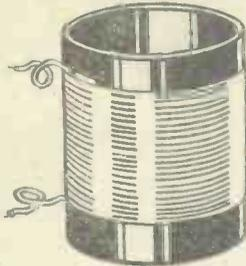
Fig. 1.—The simplest form of tuning coil.
