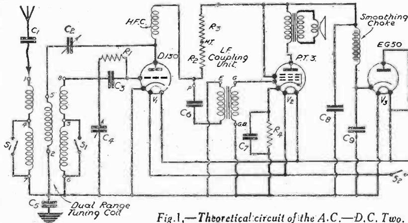
Fig. 1.—Theoretical circuit of the A.C.—D.C. T.W.O.
