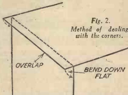
actual construction of the cabinet, except to say that deal is an easy wood to work in, besides being cheap and easily replaced if mistakes are made; if it is well dovetailed at the angles and at least  $\frac{1}{2}$  in. thick, it should be quite suitable for covering, and will make a very strong job, especially where batteries are contained in the cabinet.
