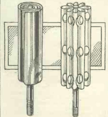
Fig. 6.—Two different types of anode used in electrolytic condensers.
