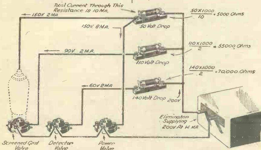
Fig. 5.—This illustrates the method of obtaining alternative anode voltages from an eliminator.
