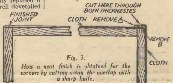
Fig. 3. How a neat finish is obtained for the corners by cutting away the overlap with a sharp knife.
