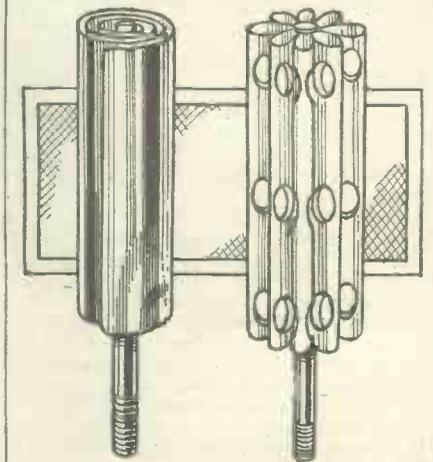
Fig. 6.—Two different types of anode used in electrolytic condensers.
