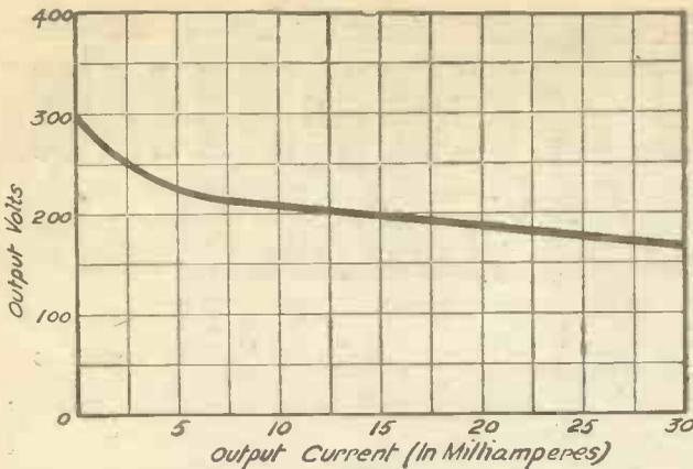
Fig. 4.—The above graph shows how the voltage output from an eliminator varies with the current drawn from it.
