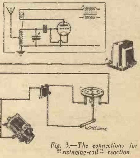
Fig. 3.—The connections for "swinging-coil" reaction.
