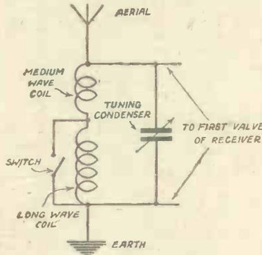
Fig. 6.—The circuit of a complete aerial tuner.
