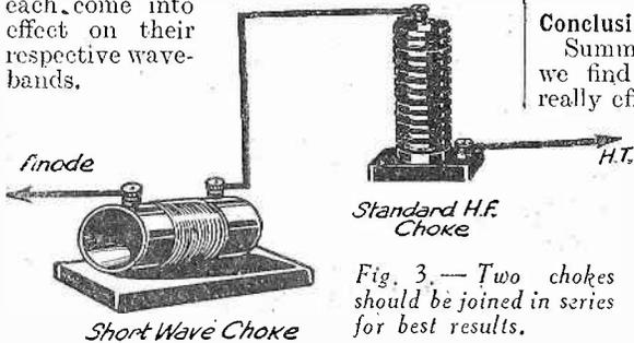
Fig. 3.— Two chokes should be joined in series for best results.
