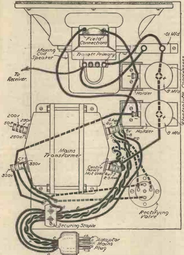
Fig. 2—Wiring diagram of the Mains Unit.
