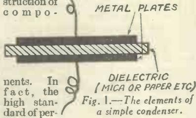
Fig. 1.—The elements of a simple condenser.
