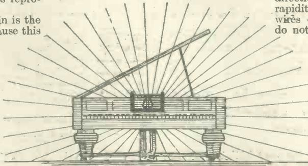
Fig. 2.—Sound does not radiate from the source in rays as above—it travels outward in waves as in Fig. 3.
