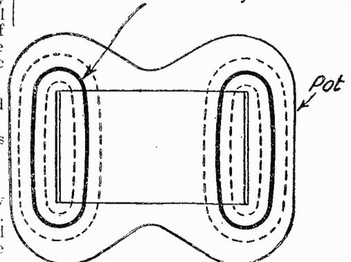
Fig. 2.—This diagram shows the arrangement of the magnetic field round a "potted" coil.
