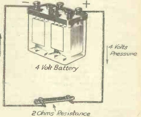
Fig. 1.—This sketch illustrates the principle of Ohm's law.
