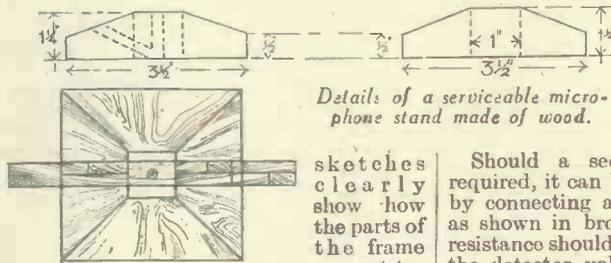
Details of a serviceable microphone stand made of wood.
