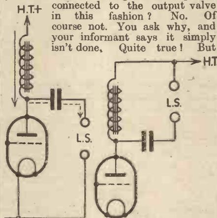
Fig. 3.—Typical choke capacity output filter.
