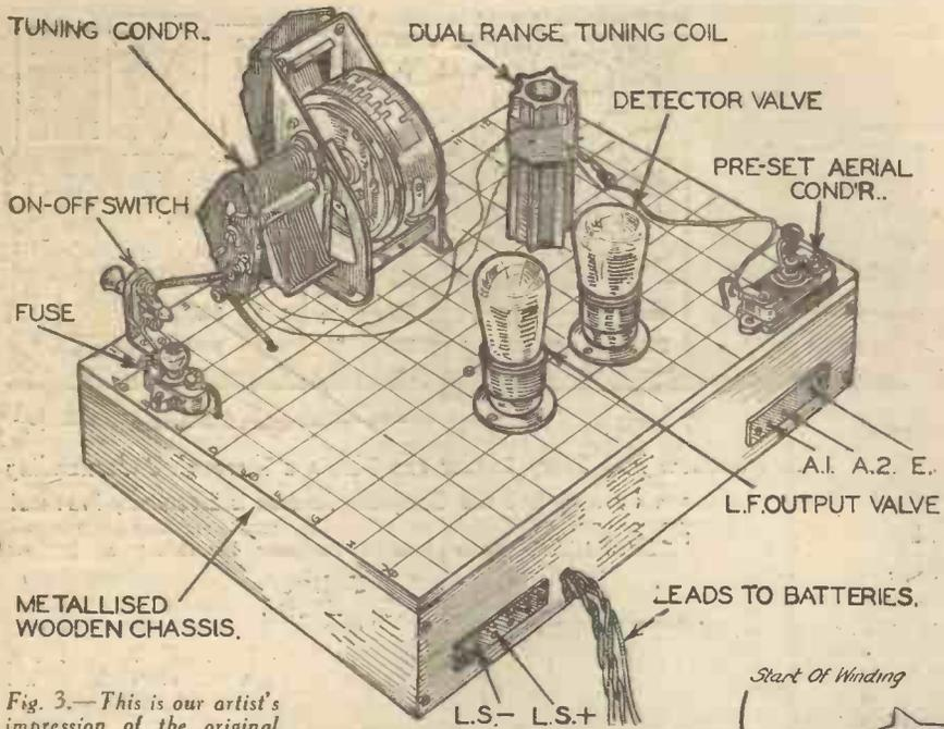
Fig. 3.—This is our artist's impression of the original receiver. The names will enable you to recognize the components.
