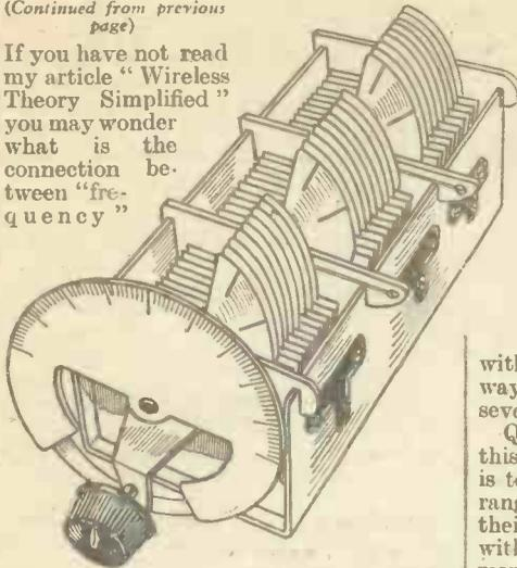
Fig. 7.—For tuning more than one circuit, a ganged condenser is used. This illustration shows a 3-gang condenser.
