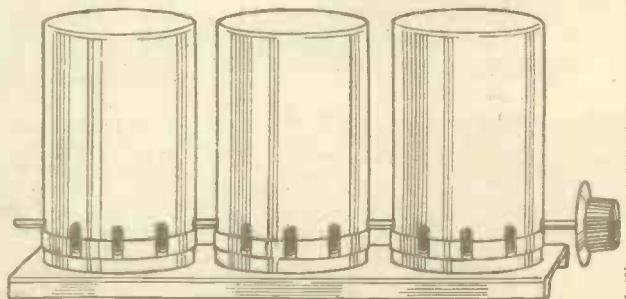
Fig. 8.—To avoid interaction the tuning coils are enclosed in cans. This is a 3-gang coil unit.
