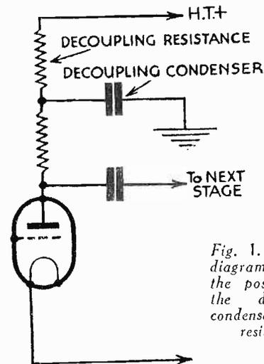
Fig. 1.— This diagram shows the positions of the decoupling condenser and resistance.
