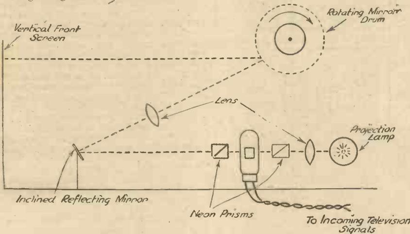
Fig. 2.—The schematic arrangement and light beam path of the Visor-Teledrom.
