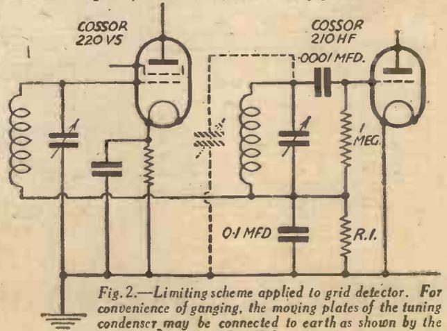
Fig. 2.—Limiting scheme applied to grid detector. For convenience of ganging, the moving plates of the tuning condenser may be connected to earth as shown by the dotted lines.
