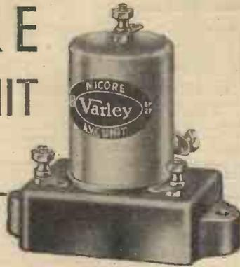
The Varley unit Automatic Volume Control can be fitted to any type of receiver. Connected immediately after the detector valve (second detector with Superhets) in place of the H.F. choke. Easily inserted into the circuit, only four connections being necessary.
