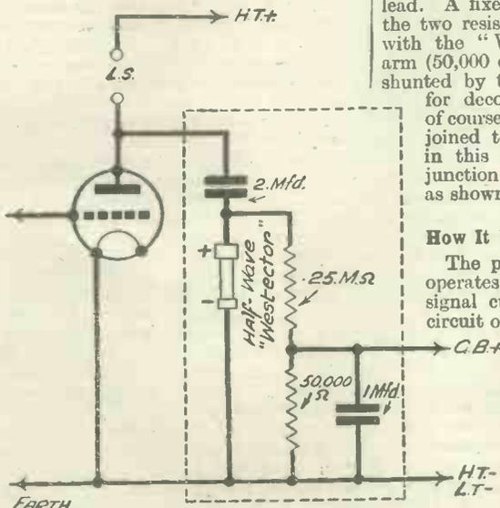
Fig. 2.—Circuit arrangement of the rectifier and resistance-condenser network used for reducing the H.T. current consumption of a power valve.
