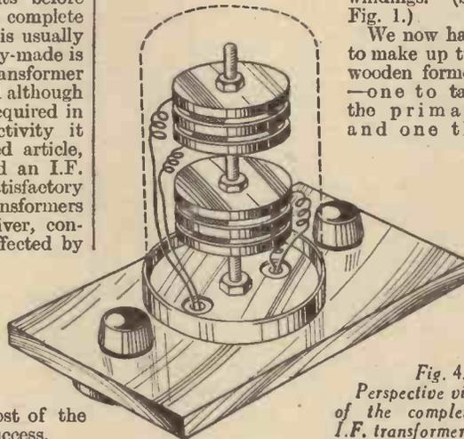
Fig. 4.—Perspective view of the completed I.F. transformer.
