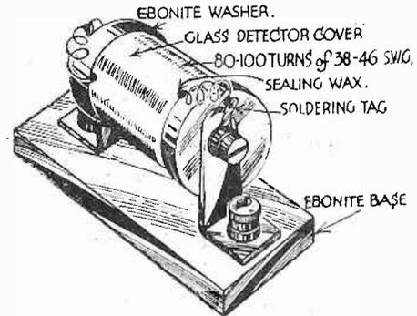
Making a short-wave choke from a crystal detector.
