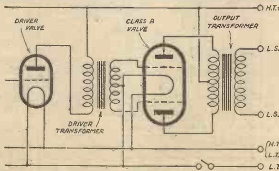
Diagram showing how a Class B valve is connected up.
