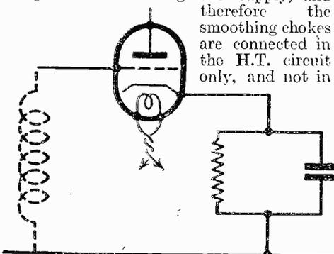
Fig. 5.—Automatic Bias is obtained by a resistance and condenser in the cathode lead.
