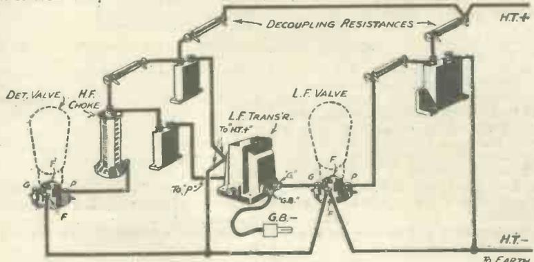
Fig. 13.—The addition of "decouplers" to stabilize a receiver.
