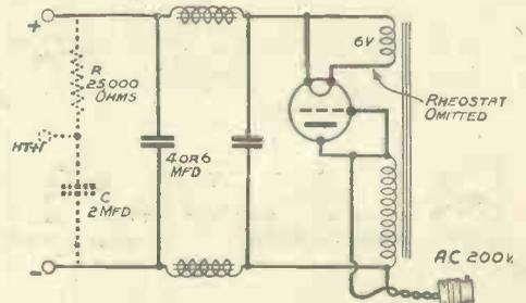
Fig. 2—Circuit diagram of a cheap H.T. eliminator.
