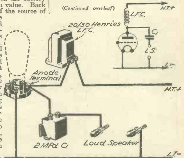
Fig. 2.—Choke filter output circuit.
