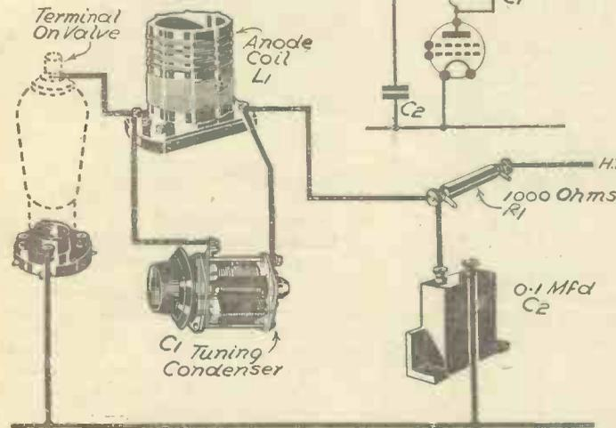
Fig. 4.—Decoupling the tuned-anode circuit.
