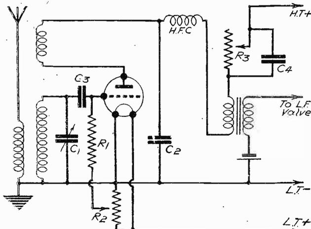
Fig. 3.—Controlling reaction by means of a resistance ( $R_3$ ).
