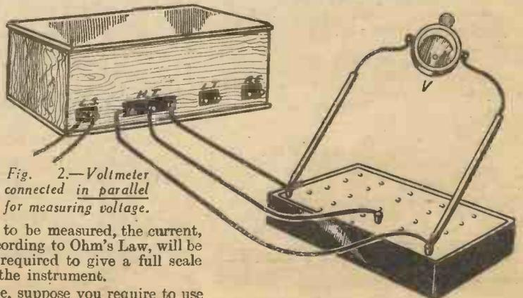
Fig. 2.—Voltmeter connected in parallel for measuring voltage.
