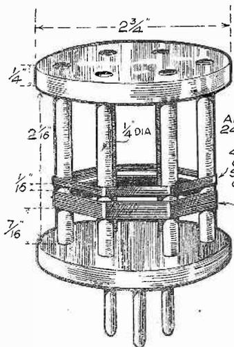
Fig. 1.—Details of coil-former and windings.
