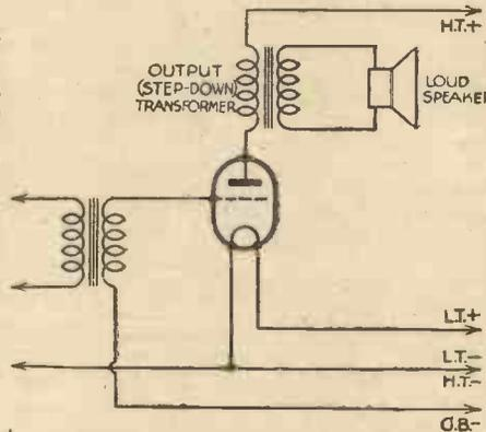
Fig. 30.—Matching the speaker and output valve by means of a step-down transformer.
