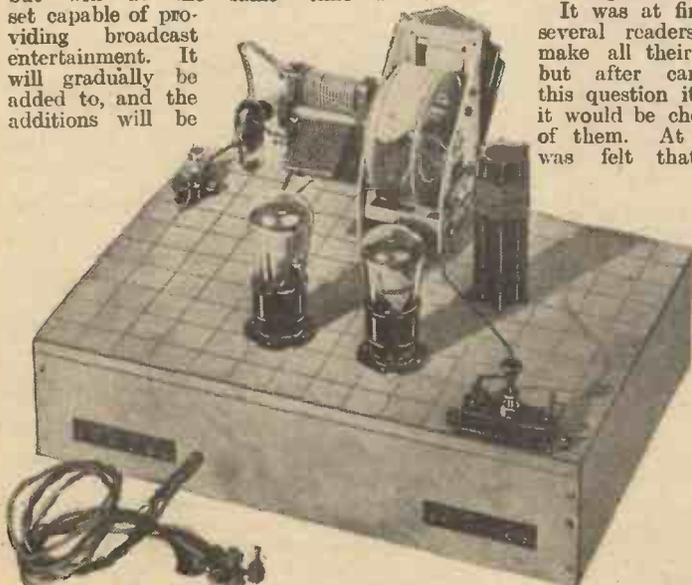
Fig. 2.—A view of the receiver as seen from the back; you can see the positions of all the components mounted on top of the chassis.
