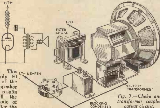
Fig. 7.—Choke and transformer coupled output circuit.
