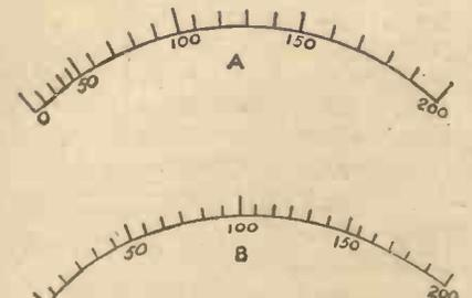
Fig. 4.—Comparison between scale of moving-iron and moving-coil instruments. A. Moving iron (crowded at bottom). B. Moving coil (equally divided).
