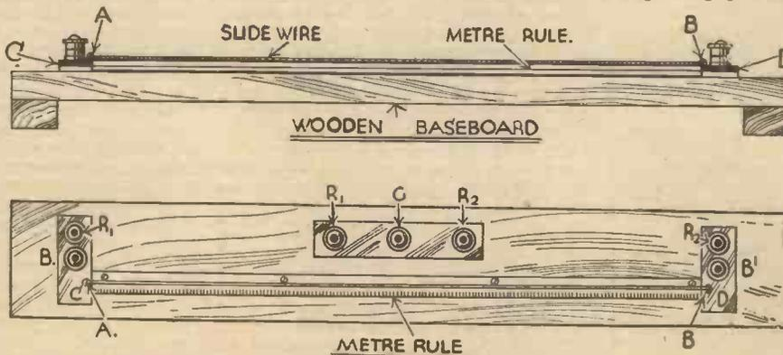
Fig. 3.—The lay-out of the adjustable arm, shown in plan and elevation. The rule by which values are computed may be seen.
