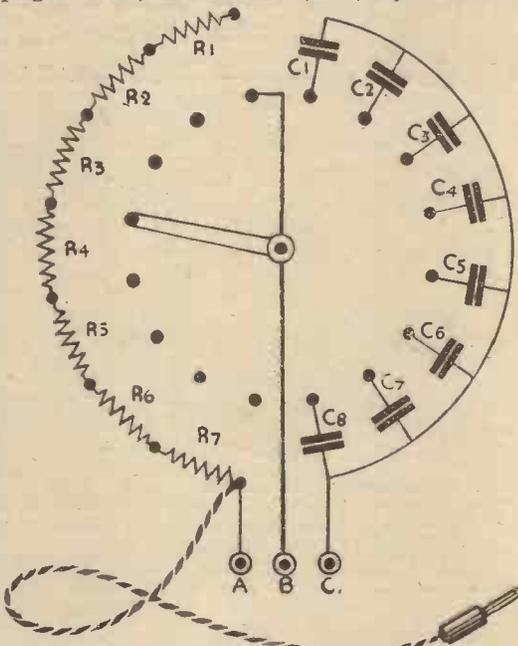
Diagram of connections for a simple test apparatus, and table of resistance and capacity values.
