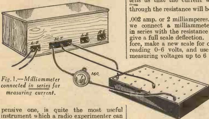
Fig. 1.—Milliammeter connected in series for measuring current.
