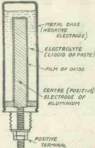
Fig. 5.—Diagrammatic representative of the inside of the electrolytic condenser.
