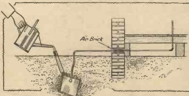
Fig. 2.—Earth plate (or bowl) with tube for watering, and lead from earth taken through air-brick of house and then through hole in floor-board to set.
