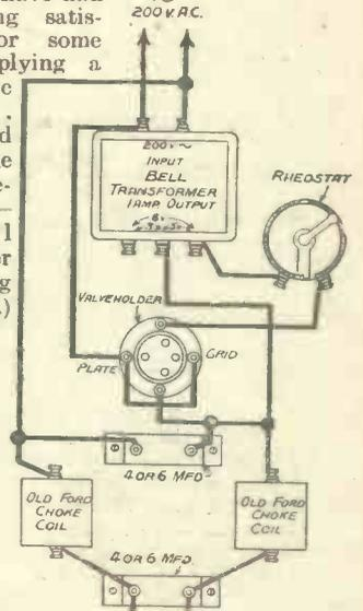
Fig. 1. Wiring diagram for a cheap H.T. eliminator.
