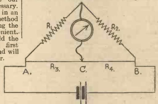
Fig. 2.—The two arms, R3 and R4, of Fig. 1 replaced by a fixed wire and adjustable contact point.
