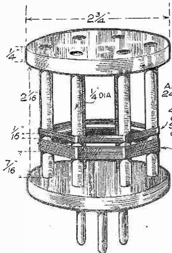
Fig. 1.—Details of coil-former and windings.
