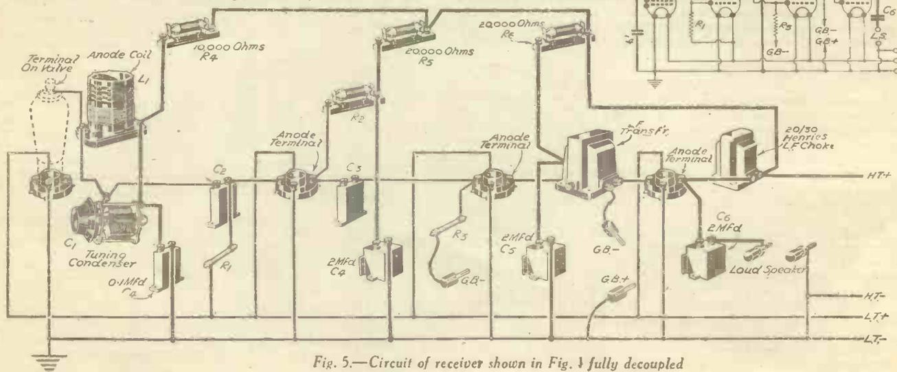
Fig. 5.—Circuit of receiver shown in Fig. 4 fully decoupled
