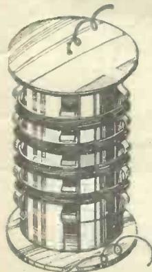
Fig. 1.—A novel method of making a coil former.
