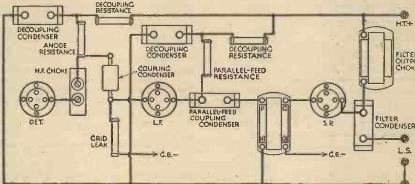
Fig. 1.—Showing anode circuit decoupling, parallel feed transformer coupling, and choke filter output.
