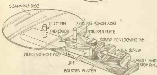
Device for punching holes in a scanning disc.
