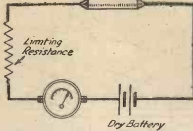
Fig. 5.—A milliammeter in series with a limiting resistance and small dry battery can be used to measure resistances.
