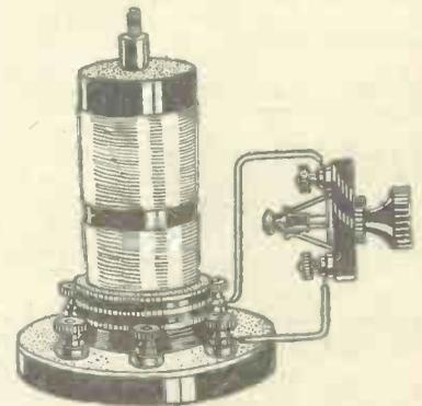
Fig. 5.—A dual-range coil and wave-change switch.
