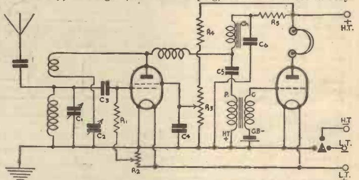
Fig. 1.—A very good short-wave circuit using choke fed L.F. coupling.
