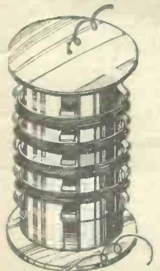
Fig. 1.—A novel method of making a coil former.
