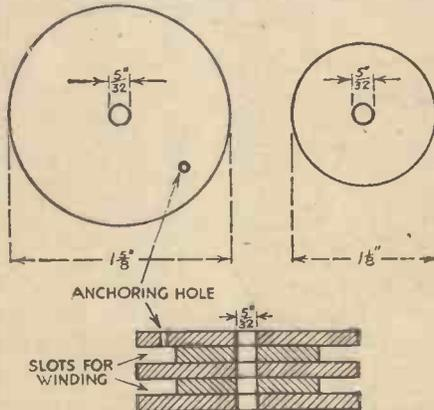
Fig. 2.—Showing wooden discs and method of assembly.
