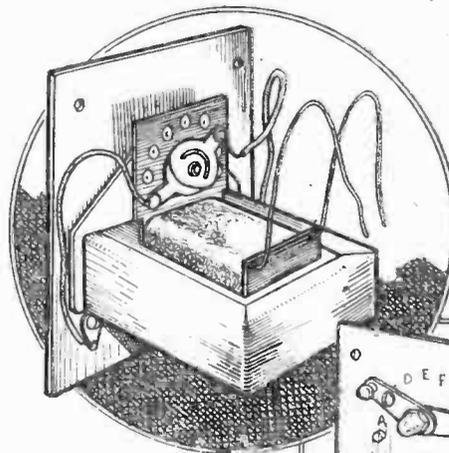
The transformer and selector switch which is fitted to the new W/B speakers. The two arms are adjusted to obtain any ratio in order to correctly match the output valve or valves.
