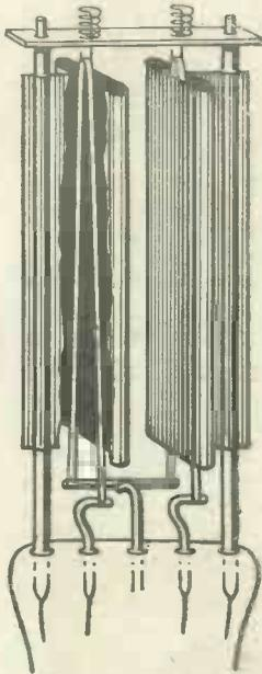
Fig. 4.—The internal construction of the 442BU rectifier showing the tape filament.
