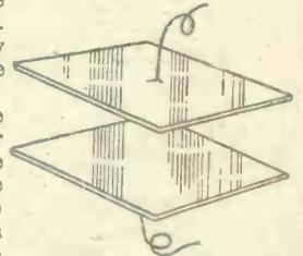
Fig. 2.—The simplest condenser.
