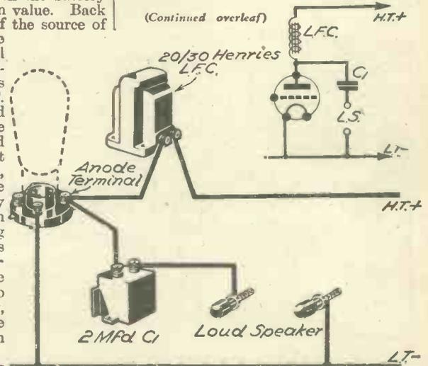
Fig. 2.—Choke filter output circuit.
