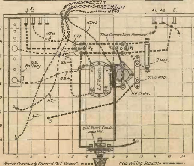
Fig. 7.—The wiring plans above clearly show the new wires which have been added during this week's experiments.
