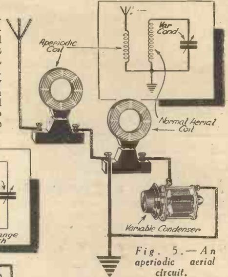
Fig. 5.—An aperiodic aerial circuit.
