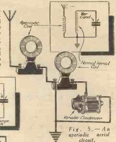
Fig. 5.—An aperiodic aerial circuit.
