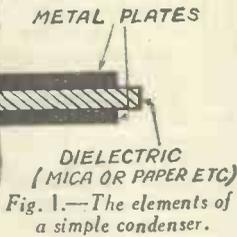
of the plates; (2) their distance apart, and (3) the nature of the dielectric. The bigger the plates are, the larger will be the capacity, also the nearer they are placed together the more it will increase. Actually the capacity does not vary directly with the distance between the plates, but is inversely proportional to the square of the distance. Thus, if the distance is halved, the capacity becomes four times as great. Regarding the
