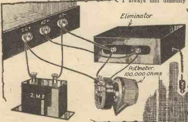
Fig. 7.—The method of obtaining the required S.G. potential from an eliminator not fitted with a special tapping for this purpose.
