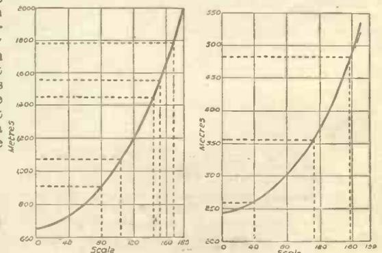
Calibration curves carried out with the buzzer wavemeter.
