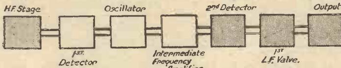
Fig. 1.—Diagrammatic representation of a 7-valve superheterodyne receiving circuit.
