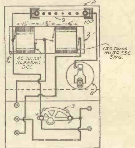
Panel and layout of a buzzer wavemeter.
