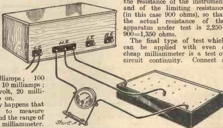
Fig. 4.—A shunt connected in parallel with a milliammeter measures its range.
