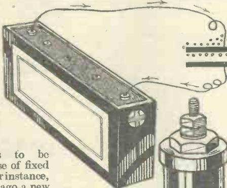
Fig. 2.—Charging a condenser from a battery. Arrows show the path of the electrons.
