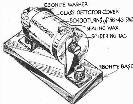
Making a short-wave choke from a crystal detector.
