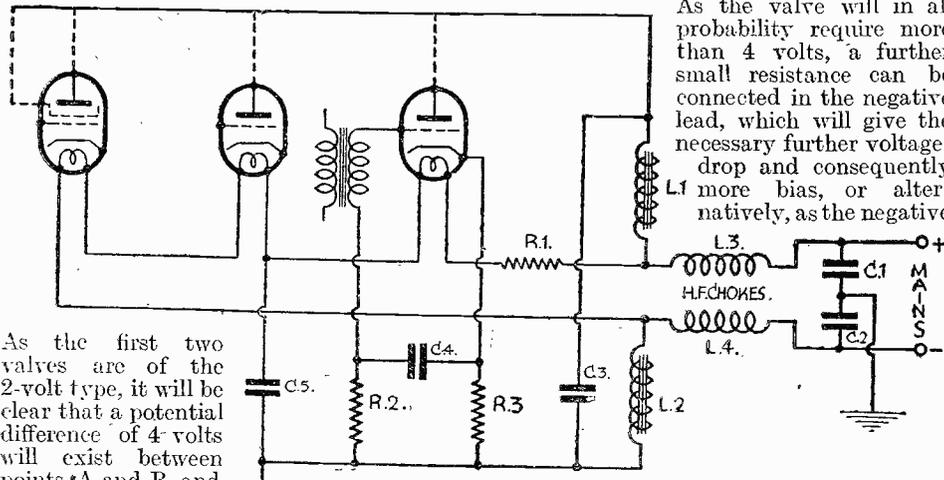
Fig. 4.—A circuit using Indirectly-heated D.C. Mains Valves.
