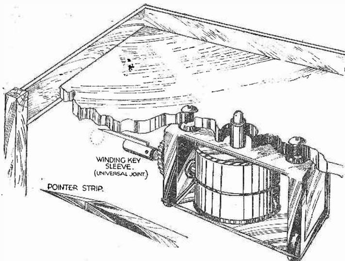
Marking out the hole in a radiogram cabinet for the winding handle.
