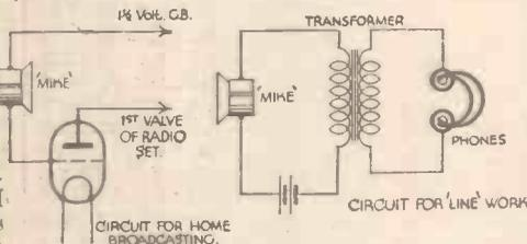
Circuit diagrams showing uses for a simple microphone.
