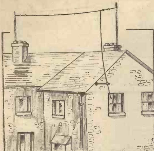
Fig. 3.—High aerial masts between two chimney stacks, with down lead held well away from the walls.
