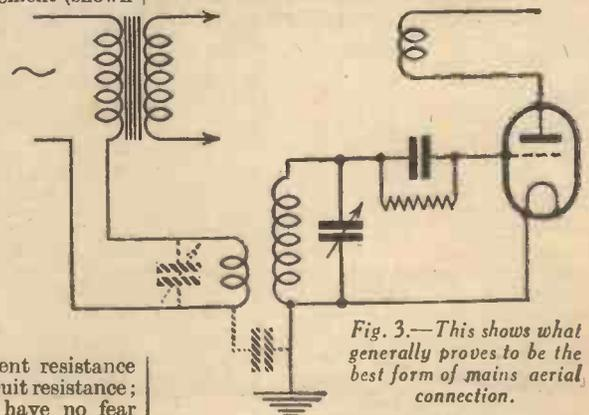
Fig. 3.—This shows what generally proves to be the best form of mains aerial connection.
