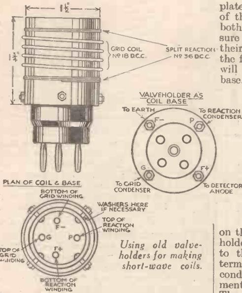
plate leg on the base, and the bottom of the winding to the other filament leg, both being soldered as before. Make sure all connections are well soldered to their respective valve legs, then put in the four bolts, and screw up tightly. This will hold the coil firmly against the valve base. The valve-holder is now secured
