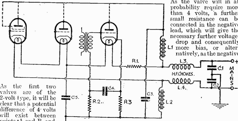
Fig. 4.—A circuit using Indirectly-heated D.C. Mains Valves.
