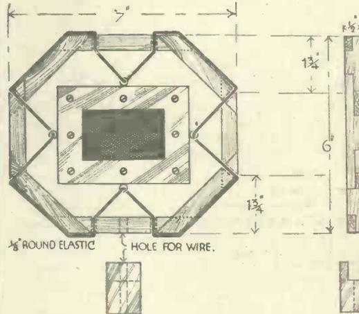
Details of a serviceable microphone stand made of wood.
