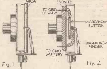
Fig. 1. A pick-up made from a grammo. sound-box.
