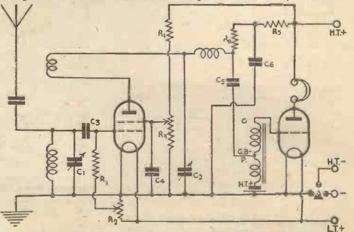
Fig. 2.—A similar circuit in which resistance fed L.F. transformer coupling is used.
