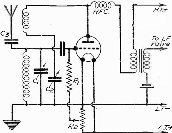
Fig. 1.—A simple reaction arrangement.
