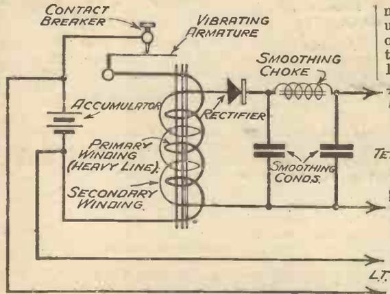
Fig. 6.—The schematic arrangement of the battery superseder.
