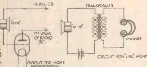
Circuit diagrams showing uses for a simple microphone.
