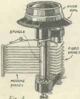
Fig. 4.—A typical tuning condenser.
