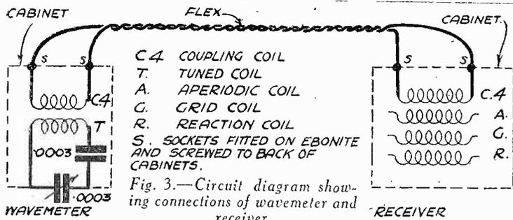
Fig. 3.—Circuit diagram showing connections of wavemeter and receiver.
