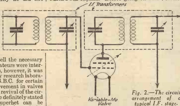
Fig. 2.—The circuit arrangement of a typical I.F. stage.
