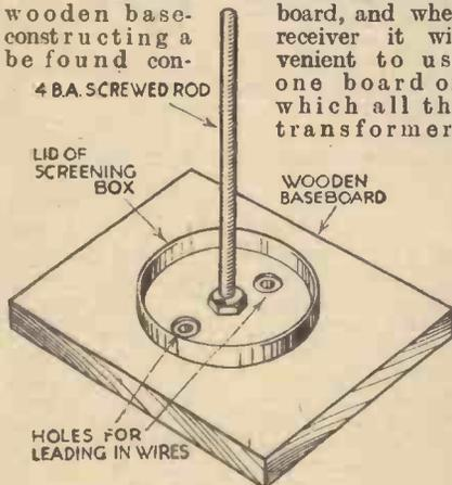
Fig. 1.—Method of attaching lid of screening box to baseboard.
