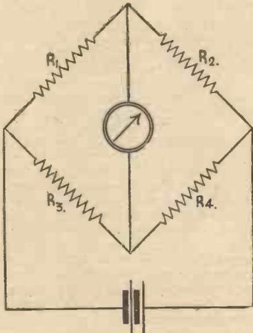
Fig. 1.—The circuit arrangement of a standard bridge.
