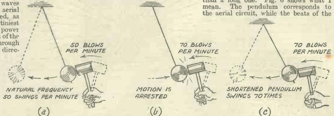
Fig. 6.—Tuning explained by the action of a pendulum and mallet.
