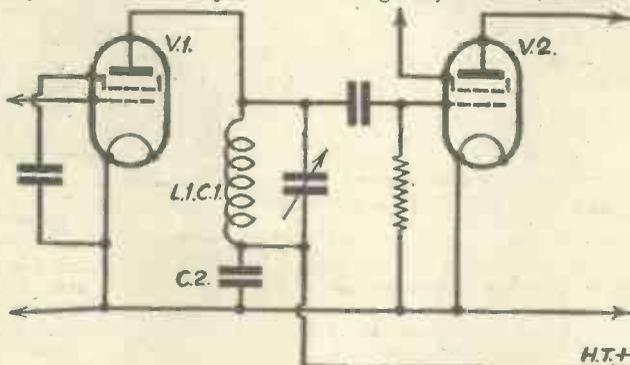
Fig. 2.—A conventional tuned anode circuit, drawn as above, readily shows that the valve V1, the tuned circuit L.C. and the grid-filament of valve V.2. are all in parallel. The condenser C.2. is the normal H.T. by-pass which would normally be shown on the extreme right-hand side of the circuit.
