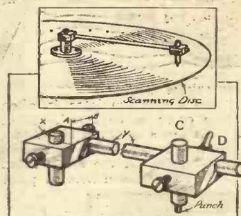
A device for punching holes in a scanning disc.
