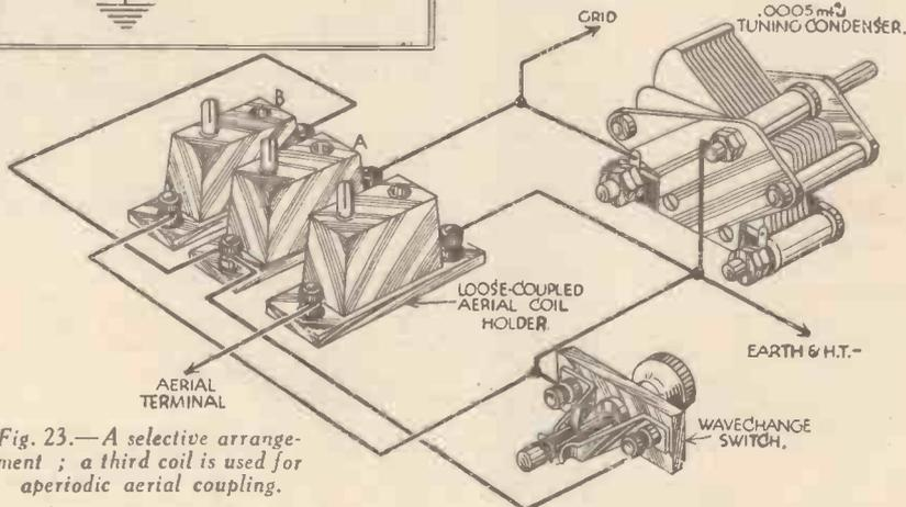
Fig. 23.—A selective arrangement; a third coil is used for aperiodic aerial coupling.
