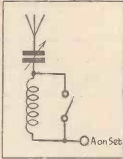
Fig. 11.—This diagram illustrates the pre-set condenser arrangement with the addition of an anti-break-through choke.
