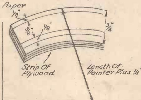
Fig. 3.—Showing how the paper scale is drawn and mounted on a strip of wood.
