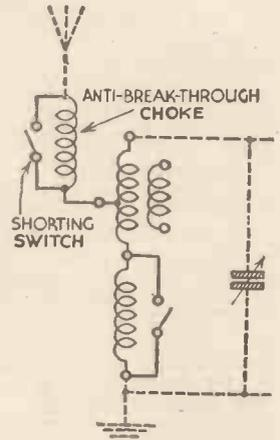
Fig. 22a.—This shows the connections for an anti-breakthrough choke.
