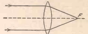
Fig. 5.—The focusing effect of a double convex lens on a parallel beam of light.
