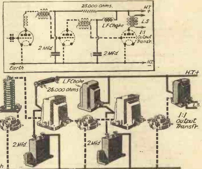
Fig. 1.—These theoretical and pictorial diagrams show how the detector and consequent L.F. valves can most easily be decoupled. The decoupling components and wiring are shown by full lines, the remainder of the circuit being in broken lines.
