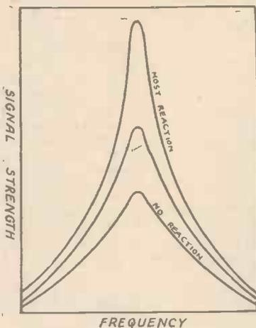
Fig. 4.—Graph showing how sensitivity and selectivity increase with the addition of reaction.
