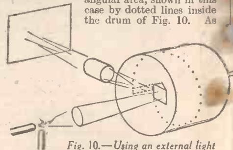
Fig. 10.—Using an external light source with a drum scanner.
