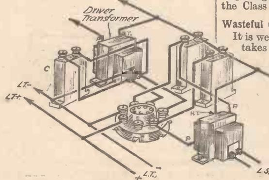
Circuit and pictorial diagrams of a Class B amplifier showing condenser C referred to in the text.
