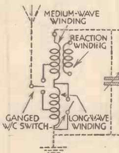
Fig. 18.—An aerial tuner circuit arrangement with transfer-tapping is illustrated by this diagram.
