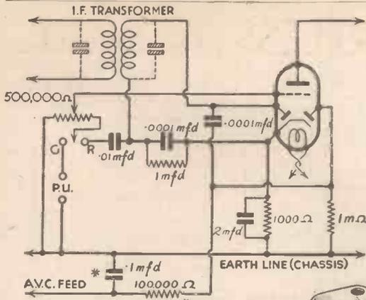
Fig. 1.—The double-diode-triode, arranged for A.V.C. with delay, with provision for gramophone pick-up. The circuit shown is that usually used for this valve in a superhet. Components marked\* are liable to considerable modifications.
