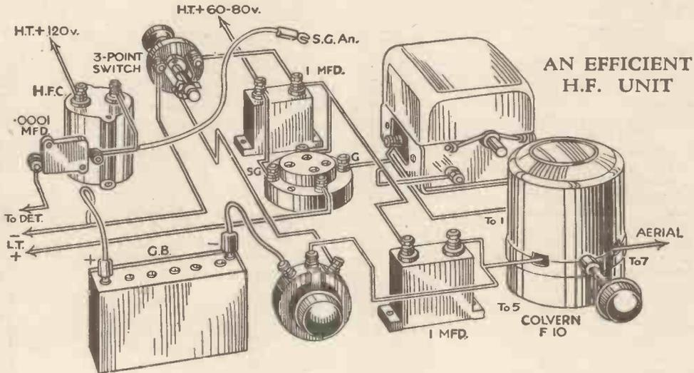
Fig. 25.—The theoretical circuit of Fig. 24 in pictorial form.
