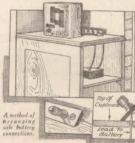
A method of arranging safe battery connections.
