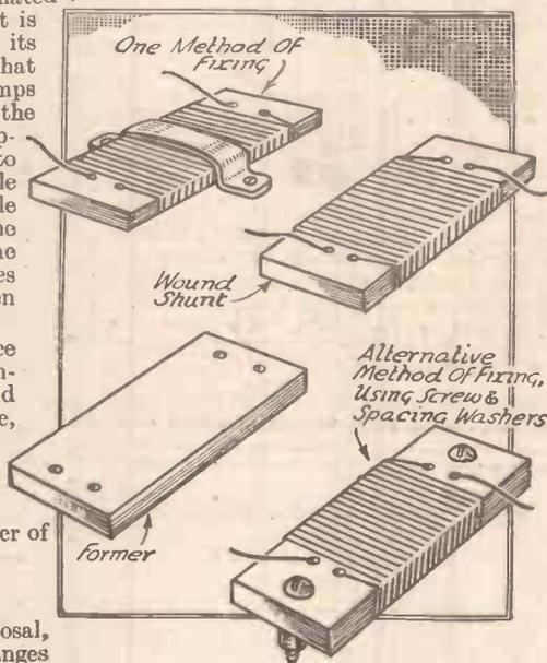
Fig. 2.—How to make up the shunt resistances.
