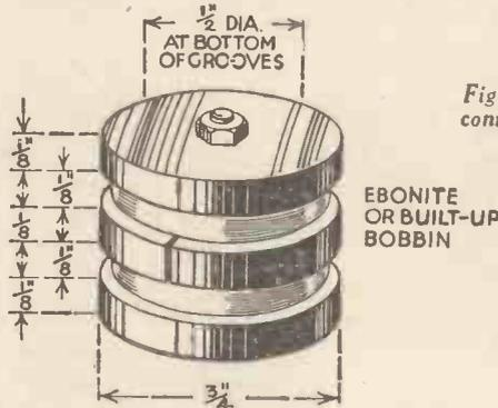
Fig. 21a.—Details of an easily made anti-breakthrough choke.
