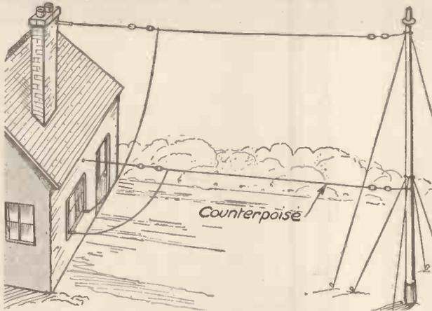
Fig. 8.—How to fix up a simple counterpoise earth.
