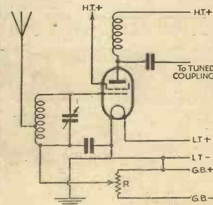
Fig. 2.—Variable bias to a battery variable-mu valve.
