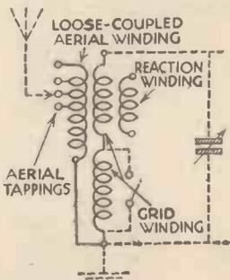
Fig. 17.—The circuit of a selective tuner with tapped loose-coupled aerial winding.
