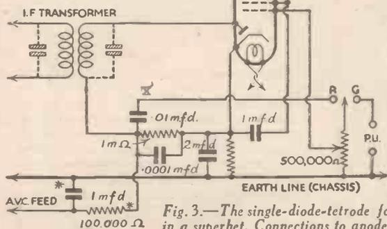
Fig. 3.—The single-diode-tetrode for A.V.C. and gramophone reproduction. The arrangement shown is suitable for use in a superhet. Connections to anode and screen are normal. An H.F. filter may be necessary at "x" in certain circuits. Components marked\* are liable to modification. Value of bias resistor varies widely with different makes of valve. That recommended by valve maker should be used.
