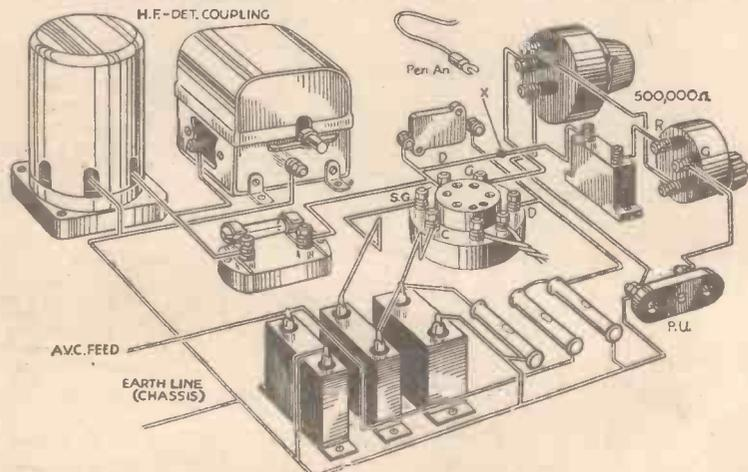
Fig. 5.—The double-diode-pentode for corrected and delayed A.V.C. with the addition of gramophone switch and terminals. Connections to anode and extra grid are normal. An H.F. filter may be desirable at "X" in some cases.
