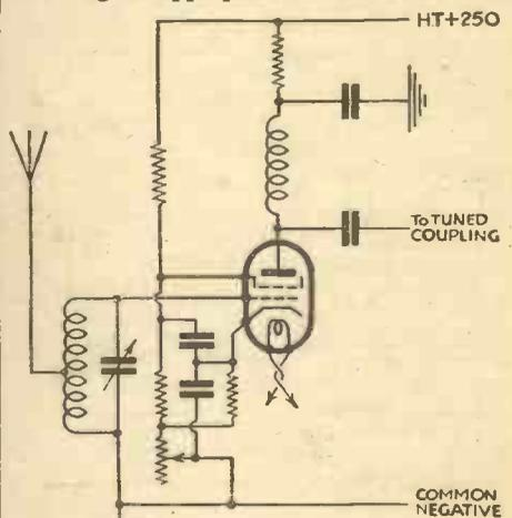
Fig. 4—Arrangement for variable bias and constant screen voltage for mains variable- $\mu$  valves.
