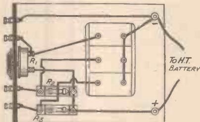
Wiring diagram for a useful filter pack.
