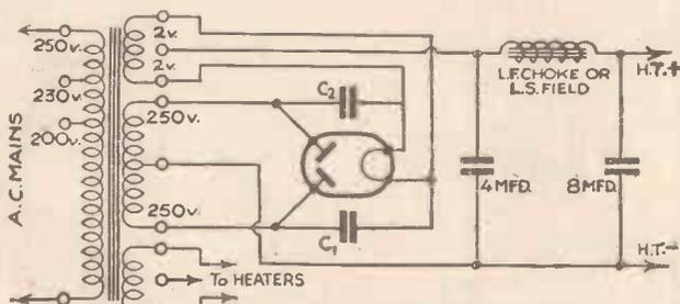
Fig. 2.—Two "buffer" condensers may be joined to the anodes of a full-wave rectifying valve to remove modulation hum.
