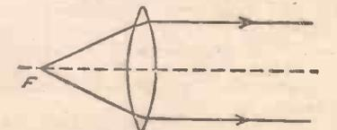
Fig. 6.—A parallel beam from a point source of light using a lens.
