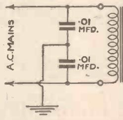
Fig. 4.—Two condensers connected across the primary winding, and the centre tap joined to earth.
