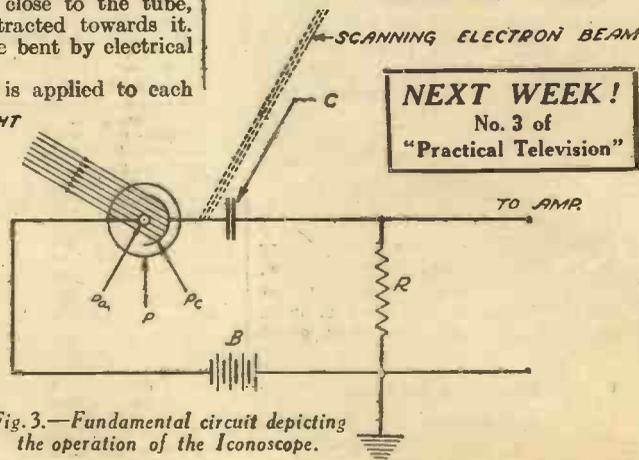
Fig. 3.—Fundamental circuit depicting the operation of the Iconoscope.
