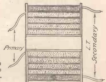
Fig. 3.—This sectionalized sketch shows the arrangement of windings in the L.T. transformer described.
