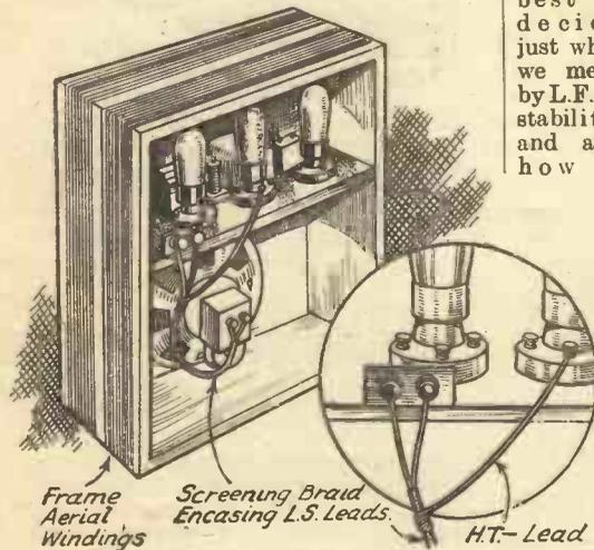
Fig. 2.—L.F. instability in portable sets can often be cured by screening the loud-speaker leads with metal braiding.
