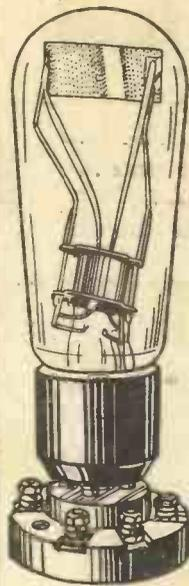
Fig. 3.—The small cathode-ray tuning device developed by Standard Telephones
