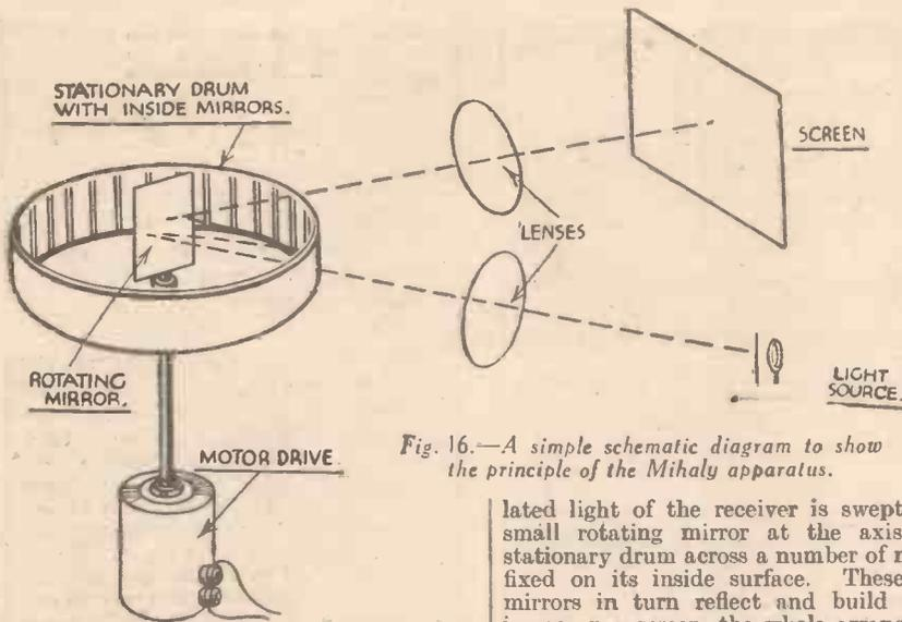
Fig. 16.—A simple schematic diagram to show the principle of the Mihaly apparatus.
