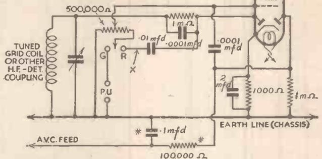
Fig. 2.—The double-diode-triode, arranged for A.V.C. with delay in a "straight" receiver, and fitted for reproducing gramophone records. A filter may be required at "x" in sets inclined to instability. Components marked\* are liable to modification.
