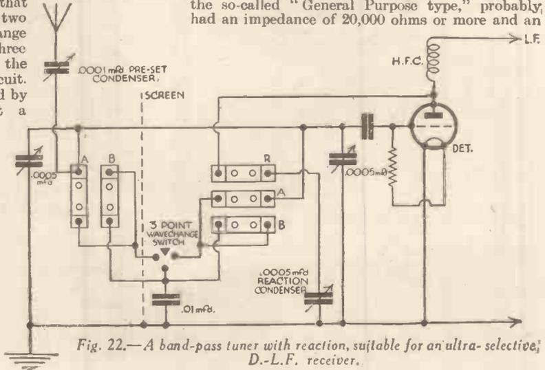
Fig. 22.—A band-pass tuner with reaction, suitable for an ultra-selective, D.-L.F. receiver.
