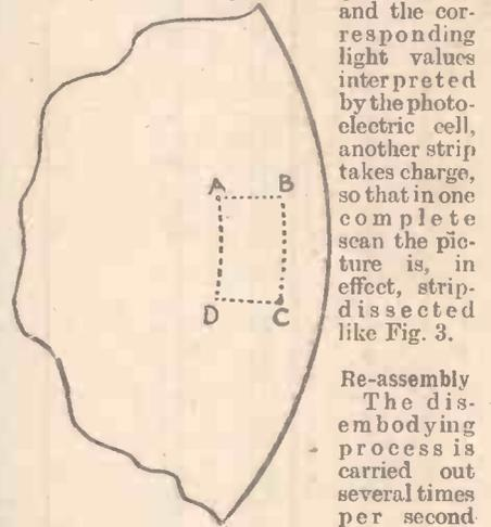
Fig. 5.—The rectangle ABCD represents the image area for this particular scanning disc.
