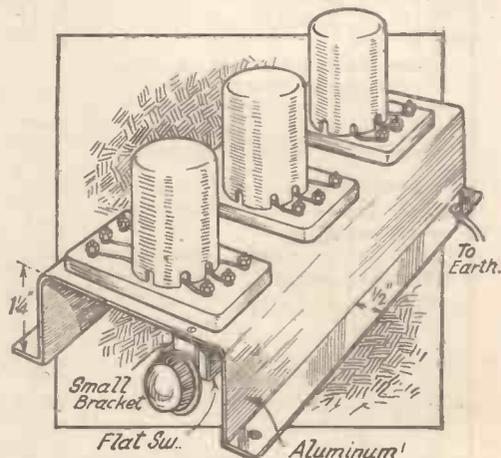
Fig. 4.—A neat way of building up a complete coil and switch assembly.
