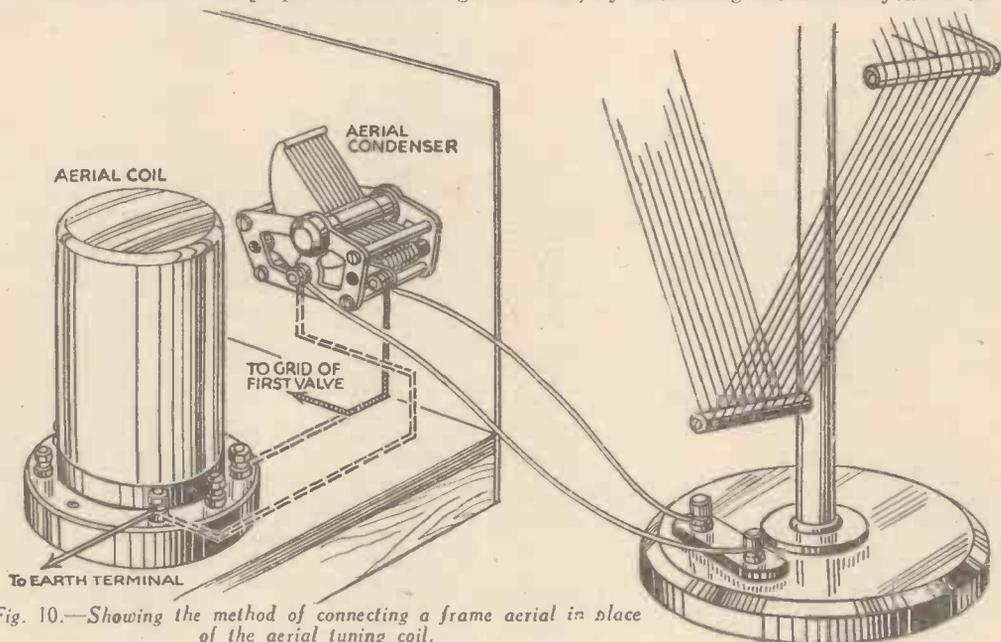
Fig. 10.—Showing the method of connecting a frame aerial in place of the aerial tuning coil.
