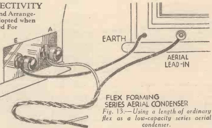
Fig. 13.—Using a length of ordinary flex as a low-capacity series aerial condenser.
