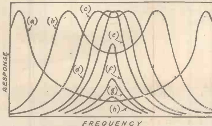
Fig. 5.—Resonance curves of a coupled circuit with various degrees of coupling.
