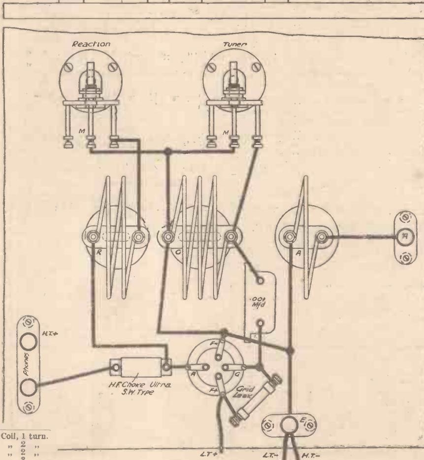
Fig. 1.—The lay-out of wiring of the experimental receiver.
