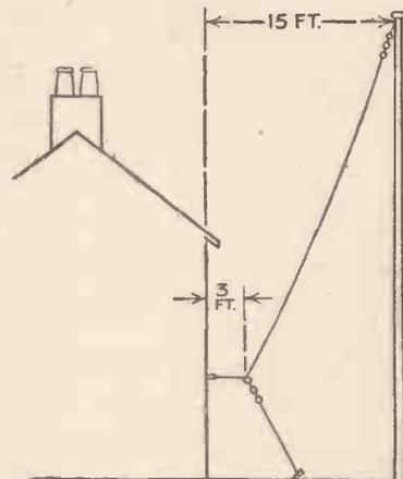
Fig. 7.—Excellent results are to be obtained by using an aerial consisting of an almost vertical wire as shown above; such an aerial is non-directional.
