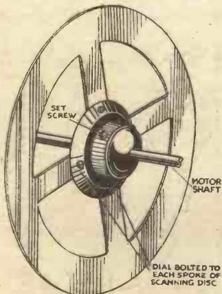
A method of mounting a scanning disc on a motor shaft.
