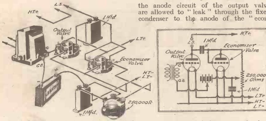
Fig. 3.—A good method of reducing the H.T. current consumption of the output valve by using an additional valve as an "economizer."
