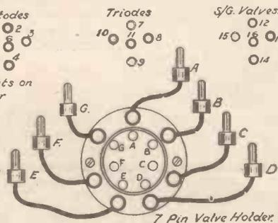
The connection for an additional valve-holder for testing Multi-pin valves on the Six-Sixty and similar test sets.
