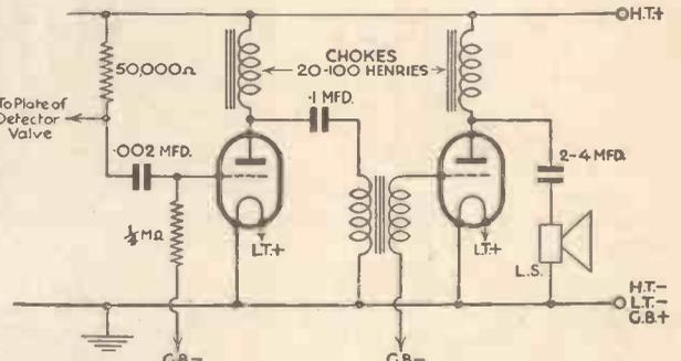
Fig. 2.—Using an L.F. choke in place of an anode resistance, and choke-coupling the speaker.
