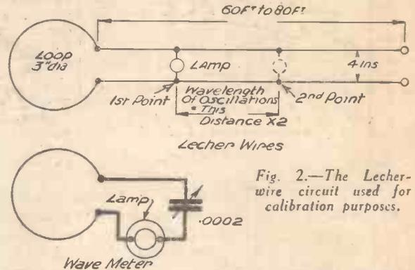
Fig. 2.—The Lecher-wire circuit used for calibration purposes.
