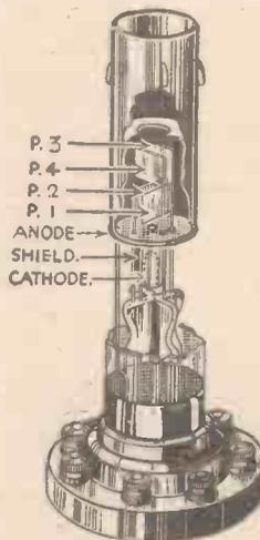
Fig. 18.—Showing the normal electrode system of a cathode ray tube.
