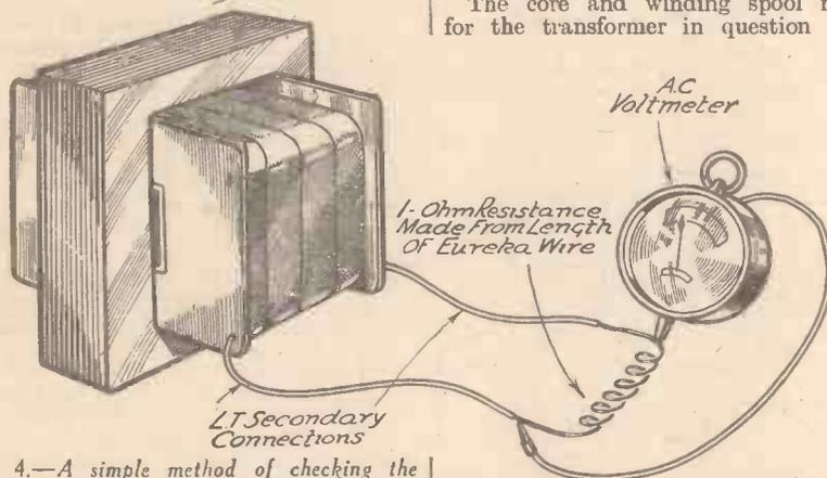
Fig. 4.—A simple method of checking the output voltage of the L.F. secondary winding conditions of "full load."
