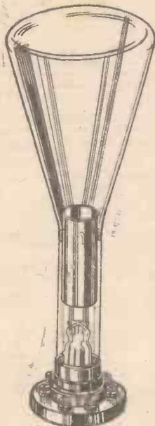
Fig. 17.—A simple illustration of a cathode ray tube.
