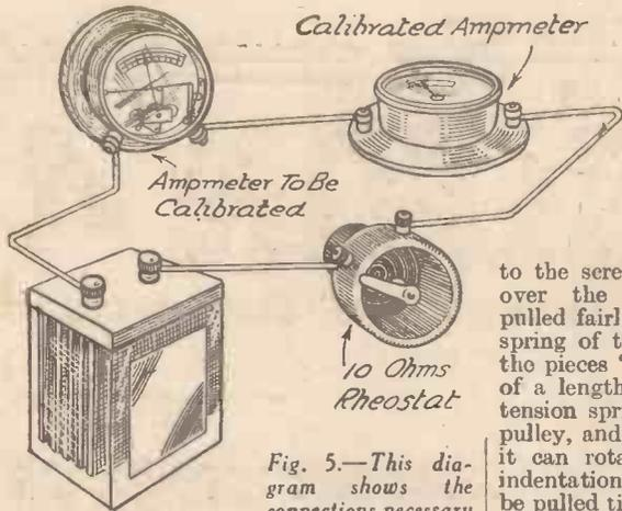
Fig. 5.—This diagram shows the connections necessary when calibrating the hot-wire ammeter.
