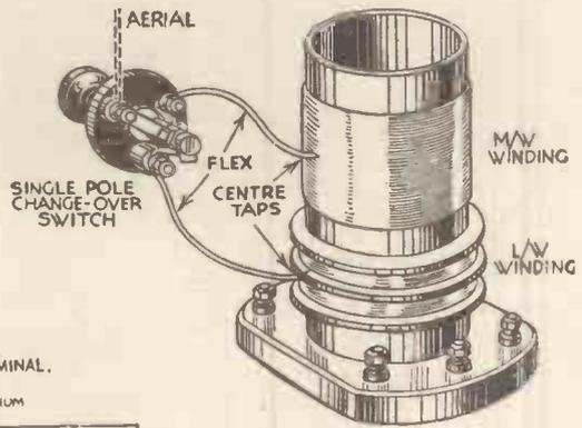
Fig. 20.—A simple method of providing a transfer aerial tapping on a standard type of dual-range coil.
