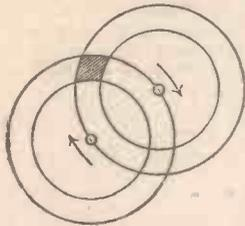
Fig. 7.—The combined action of two prismatic discs to give the required light beam motion.
