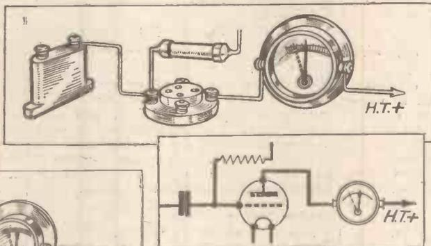
Fig. 1.—A leaky grid detector circuit milliammeter shows maximum depression of anode current when a station is accurately in tune.
