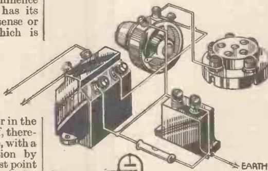
Fig. 2.—A good type of volume control with decoupling added.
