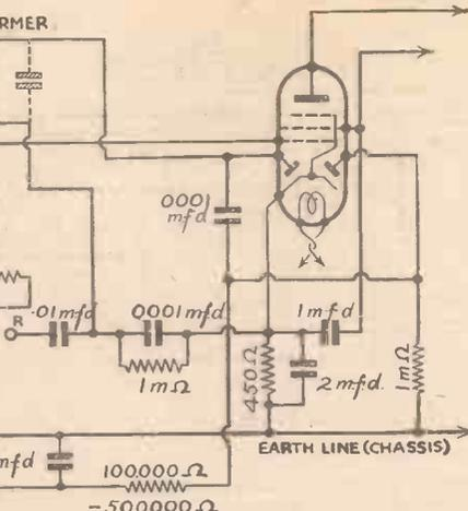
is arranged for use in a straight receiver. When using a pick-up with this type of valve it is often necessary to shield the leads as they are apt to cause mains hum in the speaker unless they are kept very short. This is due to the relatively high sensitivity of the pentode portion.
