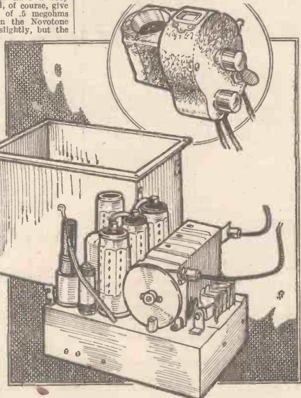
Of extremely small dimensions, this receiver is intended for operation in a car. The inset shows the small control which is fitted to the steering column. Page Car Radio are the makers of this item.
