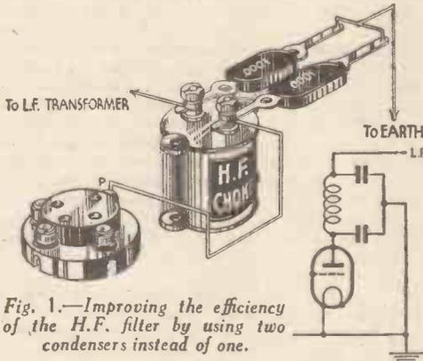
Fig. 1.—Improving the efficiency of the H.F. filter by using two condensers instead of one.
