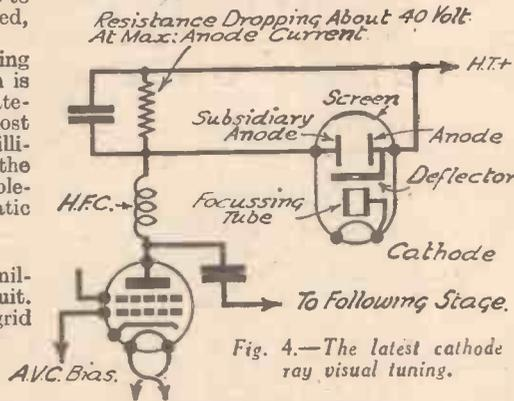
Fig. 4.—The latest cathode ray visual tuning.
