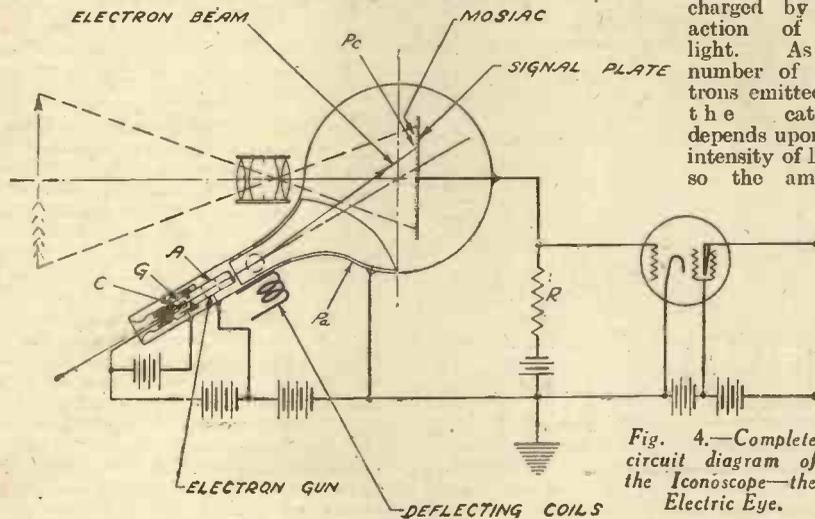
Fig. 4.—Complete circuit diagram of the Iconoscope—the Electric Eye.
