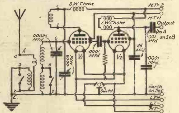
Circuit diagram of S.G. Short-wave Converter.
