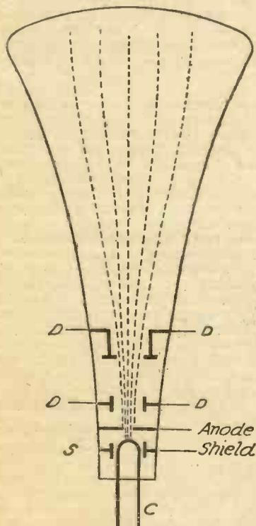
Fig. 2.—Theoretical diagram of a cathode ray tube.
