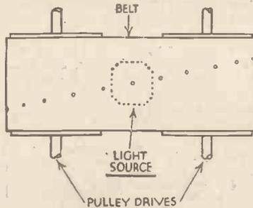
Fig. 12.—A simple scanning belt.
