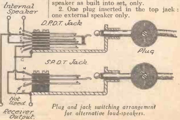
Plug and jack switching arrangement for alternative loud-speakers.
