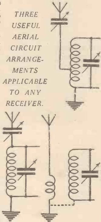
Fig. 3.—Various methods of obtaining selectivity in a single tuned circuit. They all suffer from certain drawbacks. (See text.)
