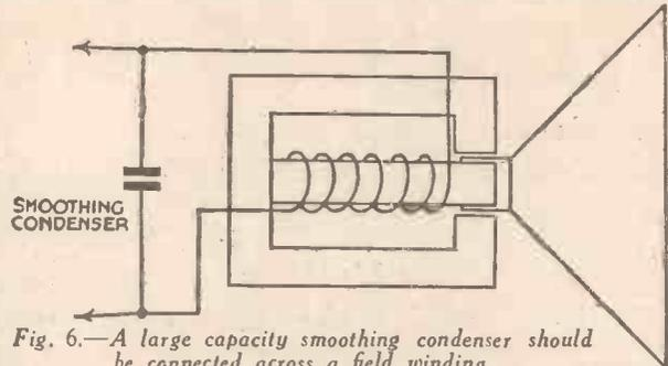
Fig. 6.—A large capacity smoothing condenser should be connected across a field winding.
