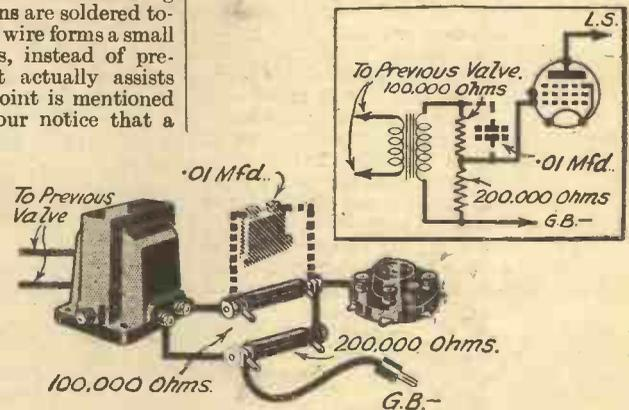
Fig. 5.—The amplification of an L.F. stage can easily be reduced by using the connections shown above and explained in the text.
