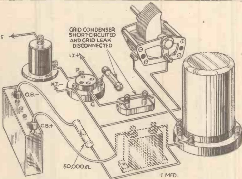
Fig. 15.—This shows the method of changing over from leaky-grid to anode-bend detection.
