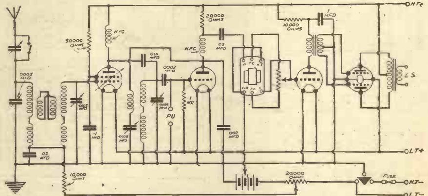
Fig. 3.—Circuit diagram of the Beta Universal Four.
