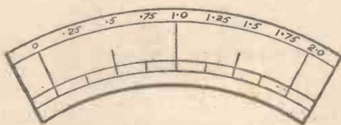
Fig. 4.—This sketch shows how the paper scale is calibrated in fractions of an ampere.
