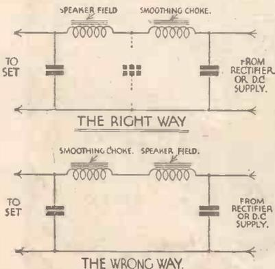
Using a field winding for a smoothing choke.
