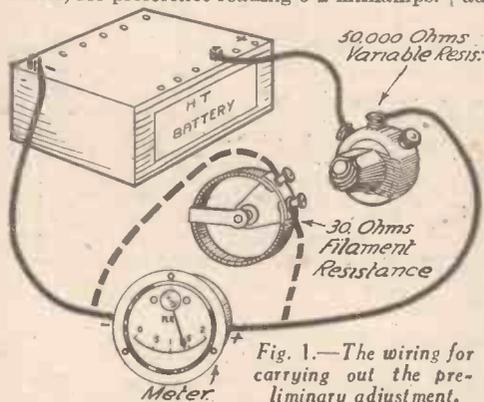
Fig. 1.—The wiring for carrying out the preliminary adjustment.
