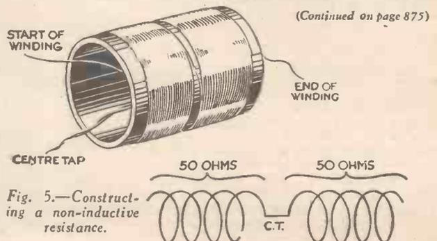
Fig. 5.—Constructing a non-inductive resistance.
