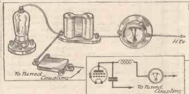
Fig. 2.—A milliammeter in the anode current of a variable- $\mu$  stage in an A.V.C. set, also shows maximum depression when a station is correctly tuned in.
