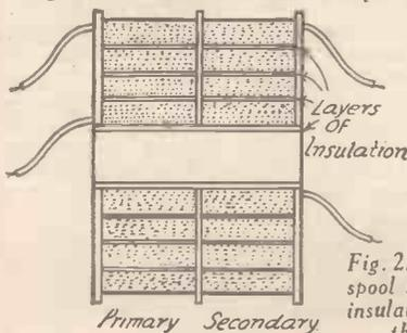
Fig. 2.—Section through the wound spool showing the arrangement of insulating layers used to "break" the windings into sections.
