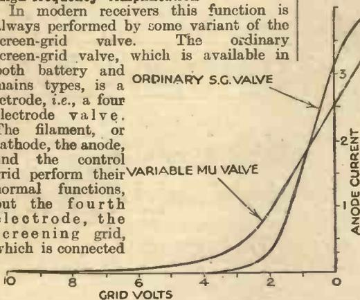
Fig. 1.—Comparison between characteristics of a variable-mu valve and an ordinary S.G. valve.
