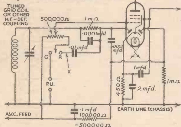
Fig. 4.—A pick-up added to the double-diode-pentode, arranged for delayed and corrected A.V.C. in a superhet. Connections to anode and extra grid are normal and not changed by the addition of the pick-up.
