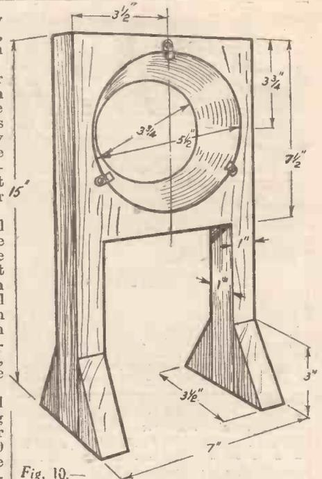
Fig. 10.—The lens mount. Note the bevelled hole.
