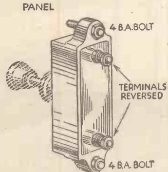
Fig. 12.—It is sometimes more convenient to mount the pre-set condenser on the panel and this can be done as shown, by reversing the terminals.
