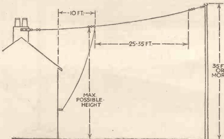
Fig. 6.—This sketch shows the approximate dimensions for a selective and efficient aerial.
