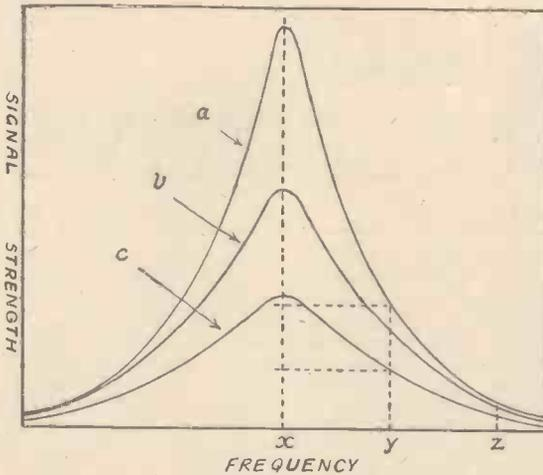
Fig. 1.—Group of resonance curves for circuits of varying efficiency. Curve b shows an average curve.
