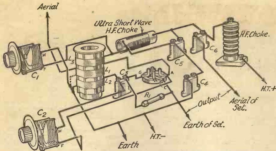
Fig. 3.—An interesting converter circuit showing in this case a mains-fed valve.
