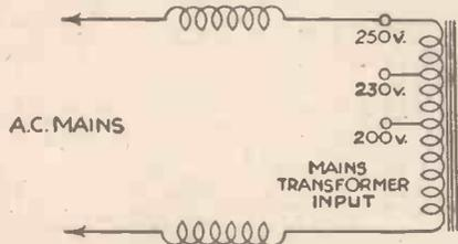
Fig. 1.—H.F. chokes (of correct design) may be advantageously included in each main lead.
