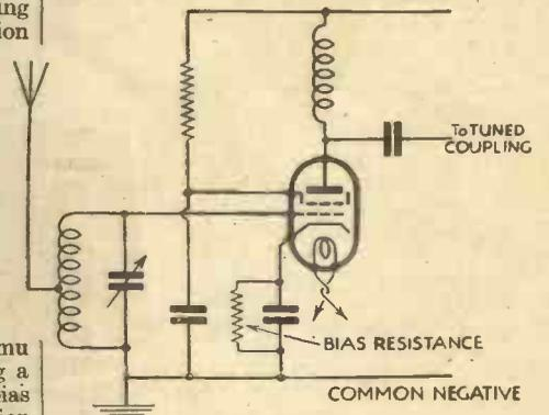
Fig. 3.—Method of auto-bias for mains S.G. valve.
