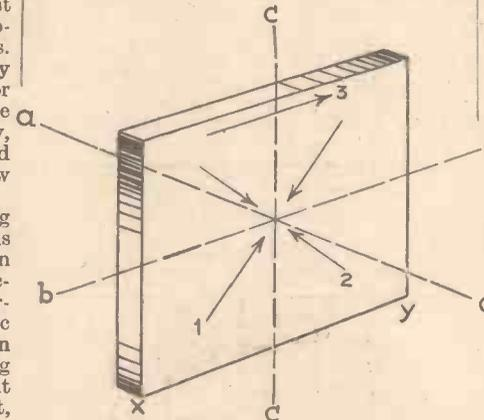
Figs. 1 and 2.—Diagrams illustrating the principle of the piezo-electric speaker.
