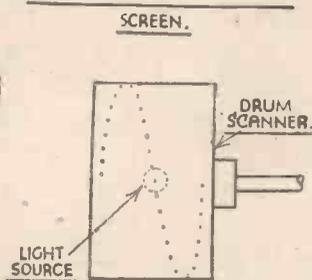
Fig. 8.—Illustrating the action of an apertured drum scanner.
