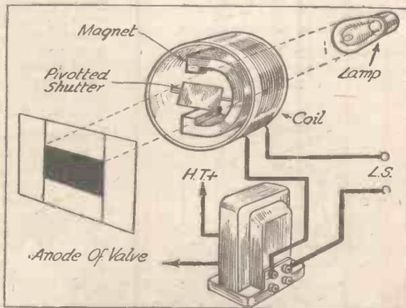
Fig. 3.—The shadow cast by a pivoted shutter, the position of which is controlled by the speech current acting in opposition to the pull of a magnet is of minimum thickness when the set is in "tune."
