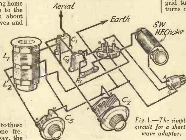
Fig. 1.—The simple circuit for a short-wave adaptor.
