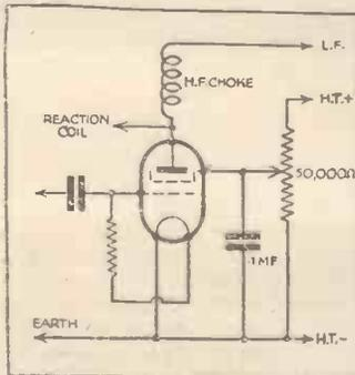
Fig. 14.—The additional connections required when using an S.G. valve as detector.
