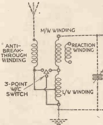
Fig. 20a.—Circuit arrangement of a tuner intended to prevent medium-wave breakthrough.
