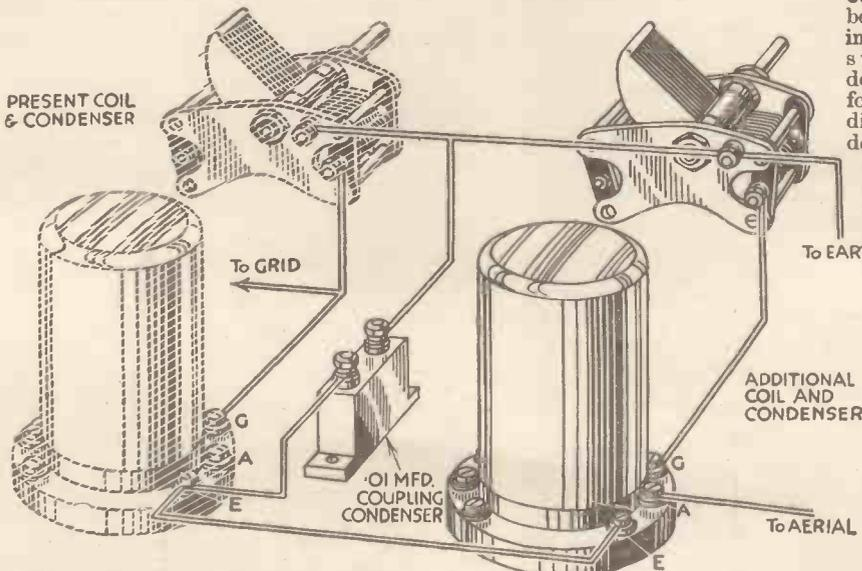
Fig. 19.—This sketch shows how nearly any tuner can be made into a band-pass arrangement by adding a new coil, tuning condenser, and coupling condenser.
