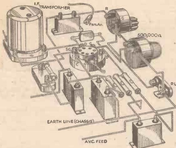
the slight rearrangement necessary to include the pick-up, and will enable the reader to identify the circuit that should be chosen when introducing a pick-up to a set already using a double-diode-tetrode for automatic volume control. In the circuits already described and also in those dealt with below, the volume control is so arranged that it functions on both radio and
