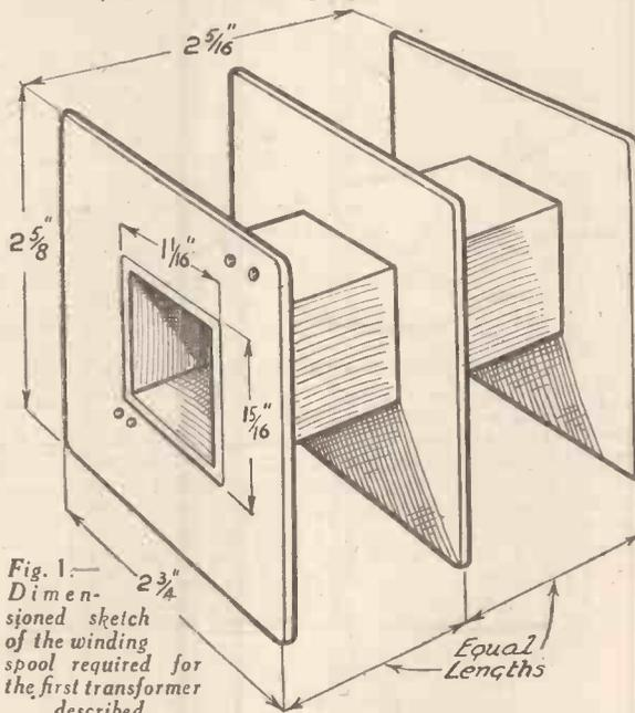
Fig. 1.—Dimensioned sketch of the winding spool required for the first transformer described.
