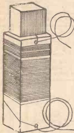
Fig. 4.—An experimental tuning coil with movable iron core.
