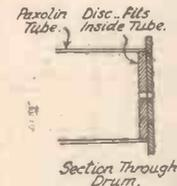
Additional details of the drum and containing case.
