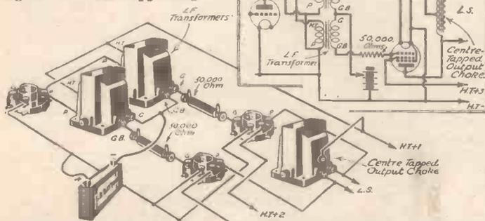
Fig. 4.—A system of Q.P.P. ordinary L.F. transformers amplification in which two are used in the input circuit.
