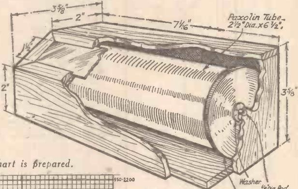
Fig. 2.—Details of the case.
