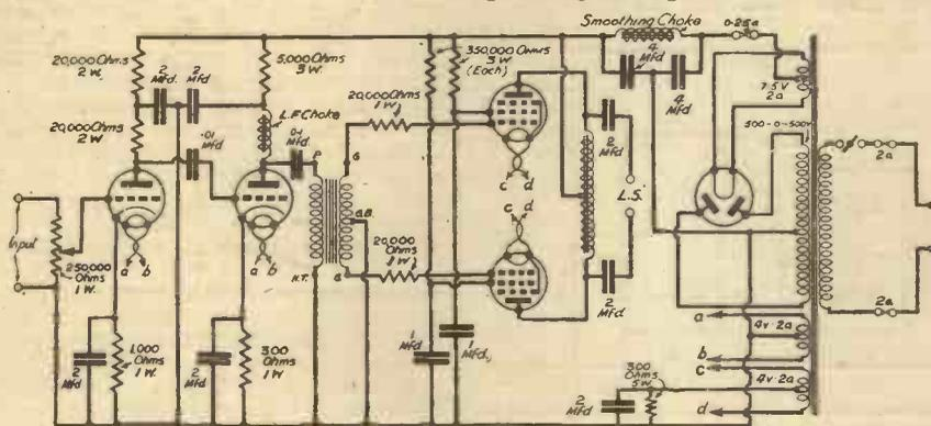
Fig. 3.—The circuit for a really powerful A.C. mains-operated amplifier. Indirectly heated valves are employed in the first two stages with a pair of directly heated pentodes in the push-pull output stage.
