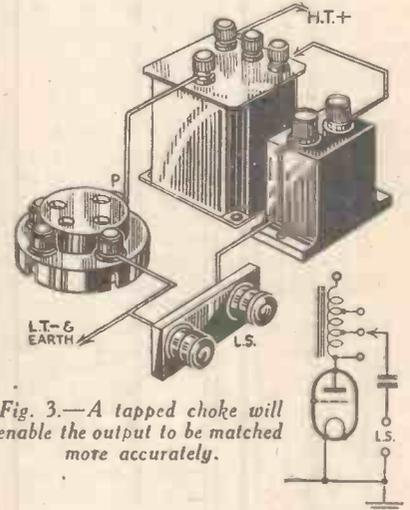
Fig. 3.—A tapped choke will enable the output to be matched more accurately.
