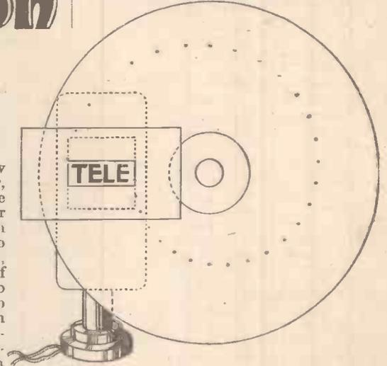
Fig. 4.—Showing how the holes are marked out at equi-angular intervals in a single turn spiral.
