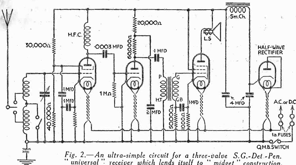
Fig. 2.—An ultra-simple circuit for a three-valve S.G.-Det-Pen. "universal" receiver which lends itself to "midget" construction.
