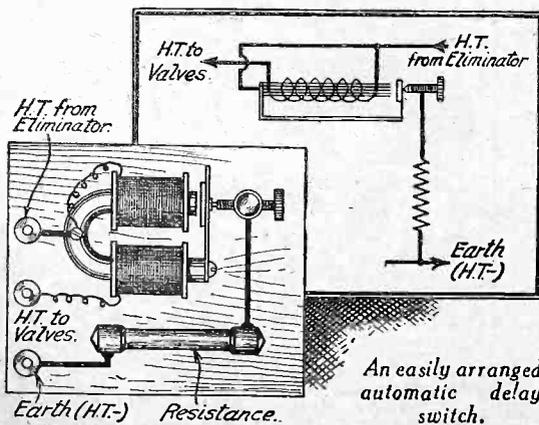
An easily arranged automatic delay switch.
