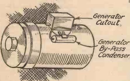
Fig. 3.—Showing the connections of a by-pass condenser used in conjunction with a generator. The condenser case is "earthed" to the frame of the generator.
