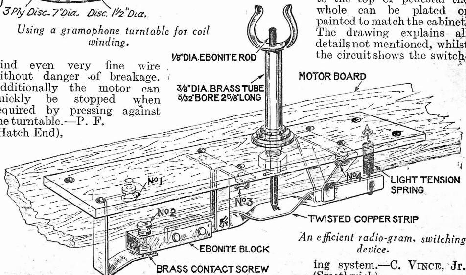
*An efficient radio-gram. switching device.*
