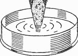
Fig. 2.—To tin the iron dip the point in non-corrosive soldering fluid after heating.
