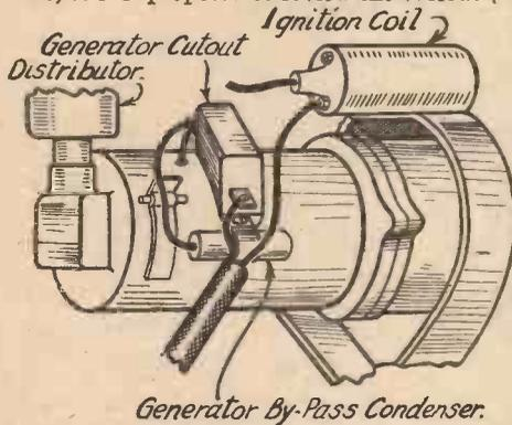
Fig. 2.—A by-pass condenser is here shown connected across the accumulator-charging dynamo. There is only a single lead to the condenser, but the other connection is made through the metal framework of the dynamo.
