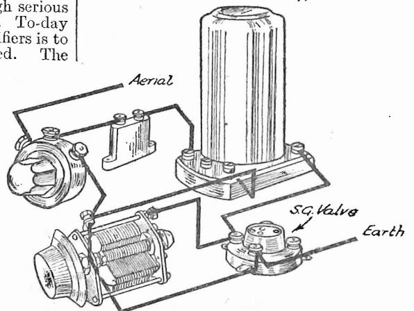
Fig. 2.—A pre-H.F. volume control using a potentiometer.
