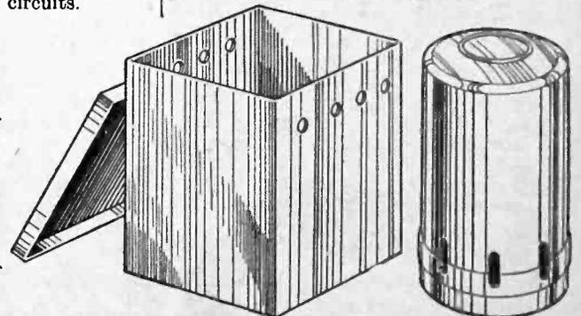
Fig. 4.—The screening box and "can."
