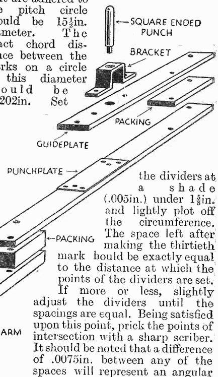
Fig. 7.—Assembly details of the complete apparatus.
