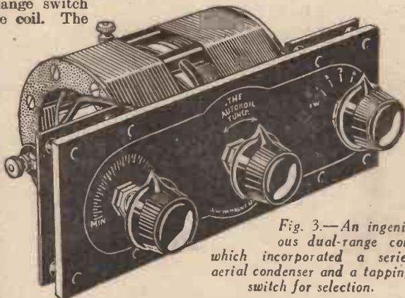
Fig. 3.—An ingenious dual-range coil which incorporated a series aerial condenser and a tapping switch for selection.
