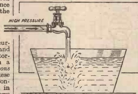
Fig. 2.—The same rate of flow produced by a small pipe but high pressure.
