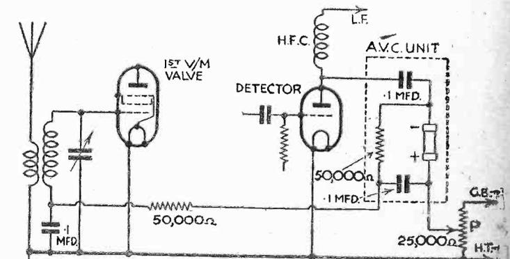
Fig. 2.—The method of fitting an A.V.C. unit to any type of variable-mu receiver.
