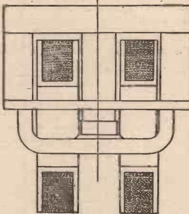
Fig. 6.—Illustrating a method similar to that of Fig. 5, but suitable for a magnet of the two-claw type.
