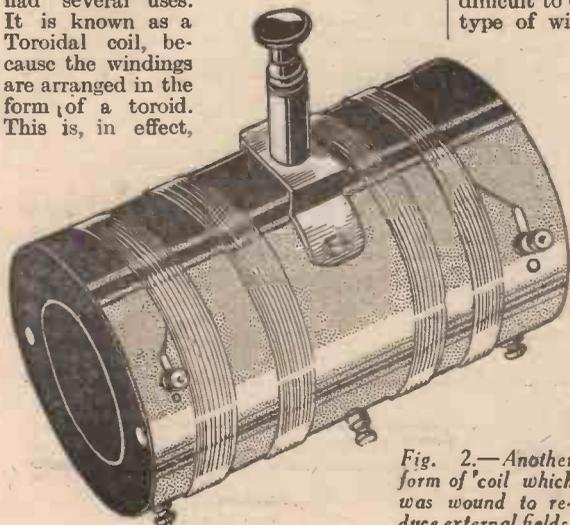
Fig. 2.—Another form of coil which was wound to reduce external fields.
