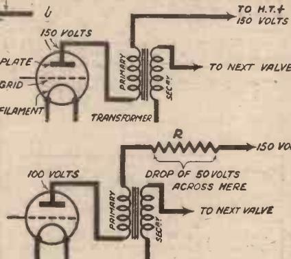
Figs. 5 & 6.—How a resistance can be used to reduce the plate voltage to a valve. Ohm's Law is used to find the value of the resistance.
