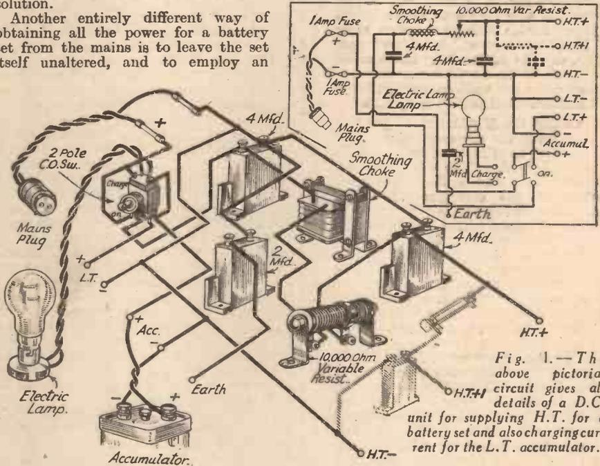
Fig. 1.—The above pictorial circuit gives all details of a D.C. unit for supplying H.T. of a battery set and also charging current for the L.T. accumulator.
