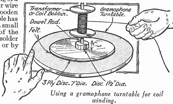
wind even very fine wire without danger of breakage. Additionally the motor can quickly be stopped when required by pressing against the turntable.—P. F. (Hatch End).
