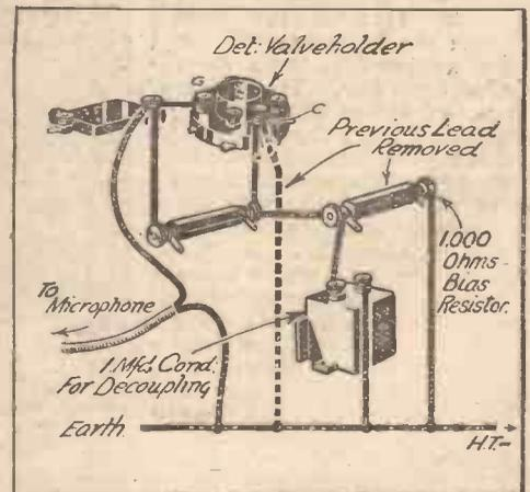
Fig. 2.—Showing the slight alterations to be made to the wiring when connecting a pick-up to the detector valve of an all-mains receiver.
