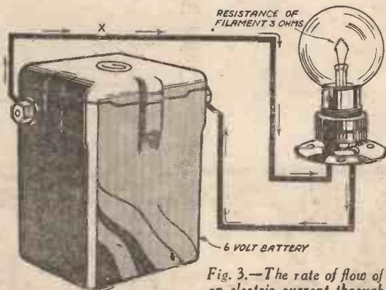
Fig. 3.—The rate of flow of an electric current through a lamp can easily be determined by Ohm's Law when the voltage and resistance are known.
