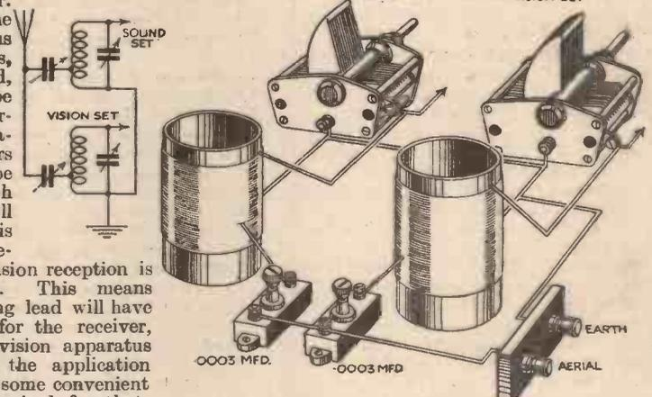
Fig. 2.—Two fixed (or pre-set) condensers, used to feed the sound and the vision receiver where ordinary tapped coils are employed.
