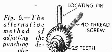
Fig. 6.—The alternative method of adjusting the punching device.
