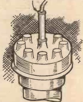
Fig. 4.—A "suppressor," also in the form of a fixed resistance, is fitted to the main supply lead to the ignition distributor. This system applies particularly to cars which employ coil ignition, and the "suppressor" illustrated would not be required where a magneto was used.
