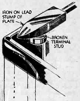
Method of removing broken terminals from accumulators.
