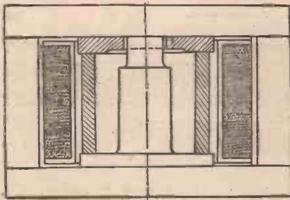
Fig. 5.—Another method of magnetizing, in which the complete magnet assembly is placed within a field winding with iron yoke.
