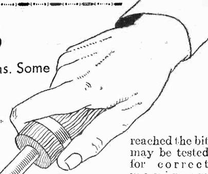
reached the bit may be tested for correct maximum temperature by holding it against a piece of newspaper held in the hand. The iron should char the paper, not merely scorch it, without burning a hole.
