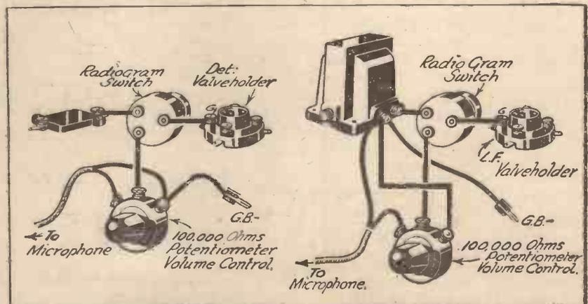
Fig. 3.—On the left the method of fitting both a change-over switch and volume control to the detector valve is shown. The method of making the same additions to an L.F. valve is shown on the right.
