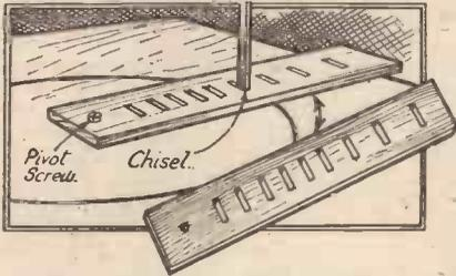
A simple method of cutting circular holes.
