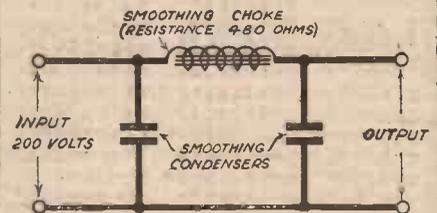
Fig. 7.—The voltage obtainable from this mains unit after the current has passed through the smoothing choke can be determined by Ohm's Law.
