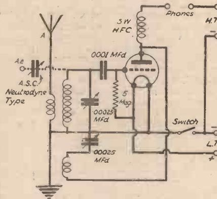
Fig. 1.—A one-valve circuit, suitable for all wave-lengths.
