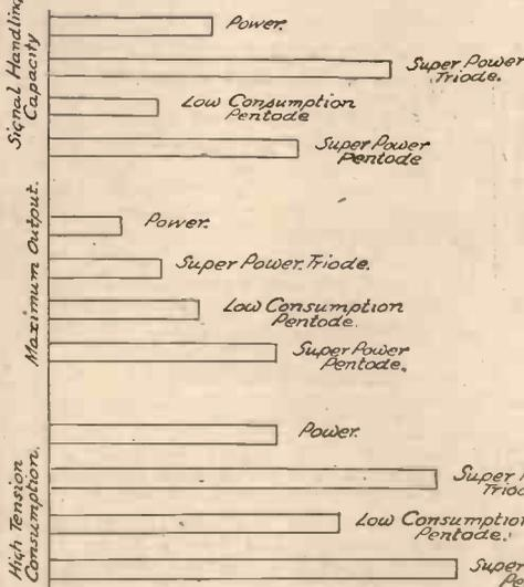
A comparison chart of output valves according to signal handling capacity, output, and H.F. consumption.
