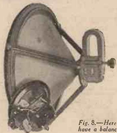
Fig. 8.—Here we have a balanced-armature speaker chassis of normal type compared with a midget moving-coil unit. The latter is a "Sonochorde."
