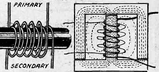
Figs. 7 and 8.—Two forms of iron core. Left, a simple iron rod; right, a core which completely surrounds the coils of the transformer.
