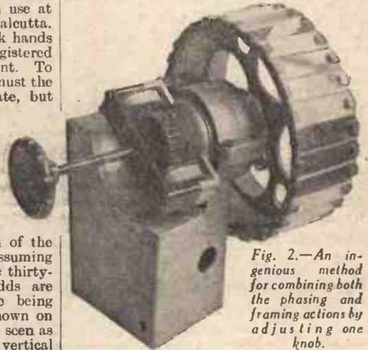
Fig. 2.—An ingenious method for combining both the phasing and framing actions by adjusting one knob.
