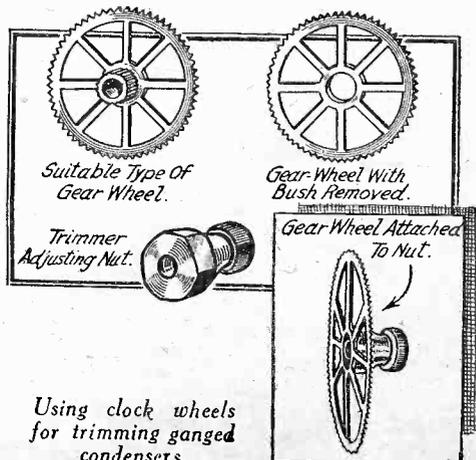
Using clock wheels for trimming ganged condensers.
