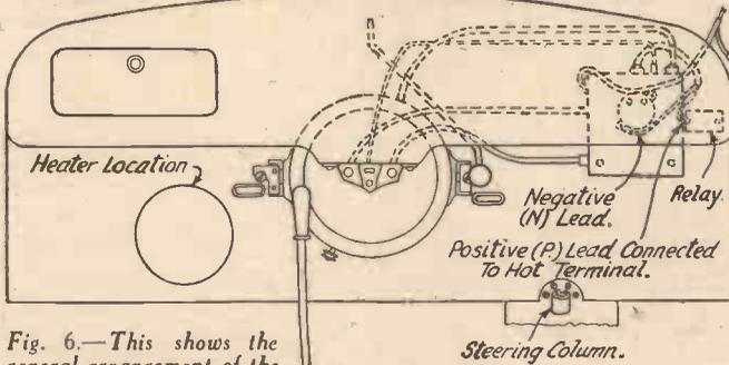
Fig. 6.—This shows the general arrangement of the receiver on the dashboard of a car. The principal connections and controls are illustrated, and the neatness of the scheme is apparent.
