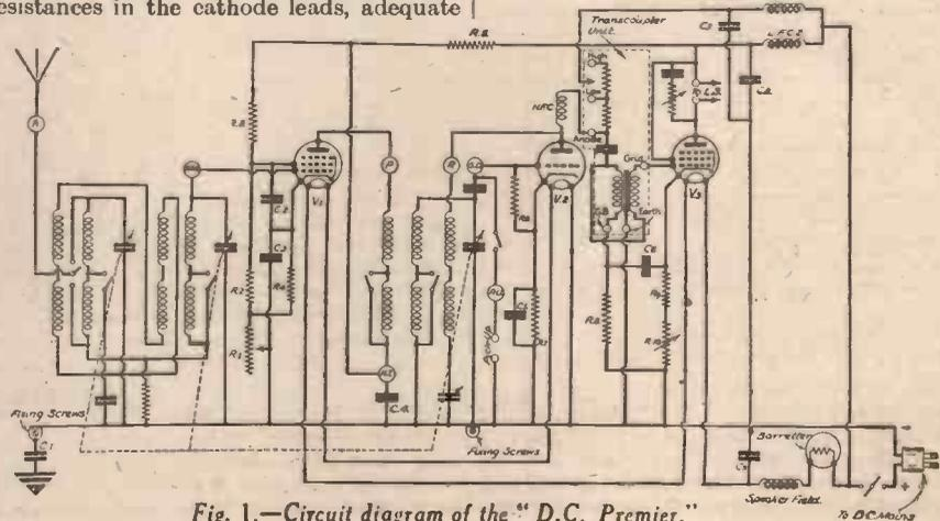
Fig. 1.—Circuit diagram of the "D.C. Premier."
