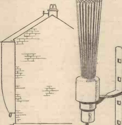
The "No-Mast" Aerial Device showing how it is fixed and the novel "collector" device.
