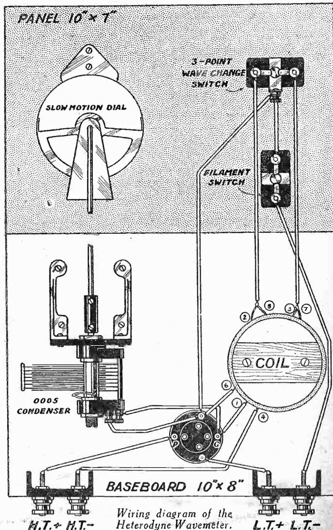
Wiring diagram of the Heterodyne Wavemeter. L.T. + L.T. -
