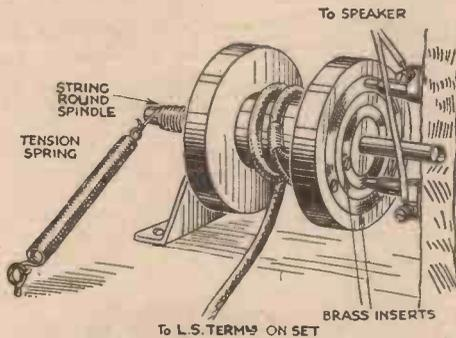
An automatic winding device for L.S. leads.
