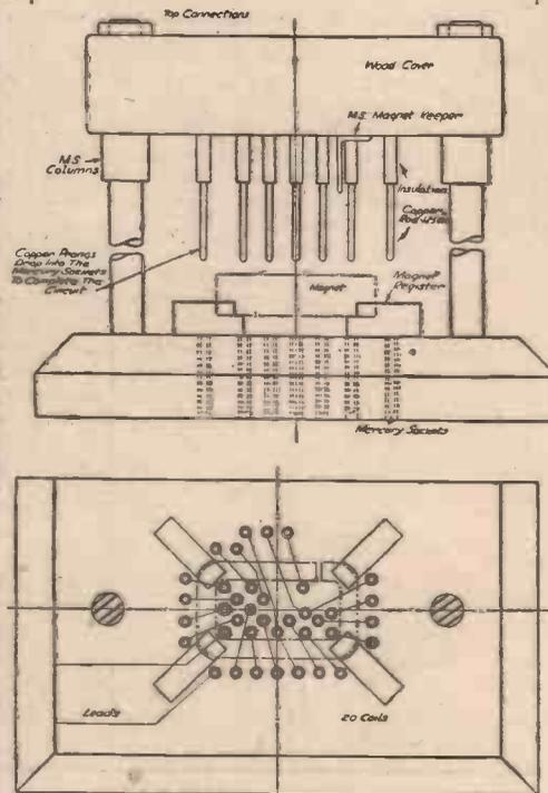
Figs. 7 and 8.—Details of a commercial form of magnetizer; this is described in the text.
