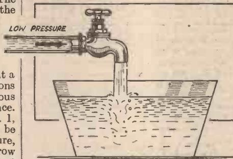
Fig. 1.—The water analogy. A certain rate of flow is produced by a large pipe and low pressure.
