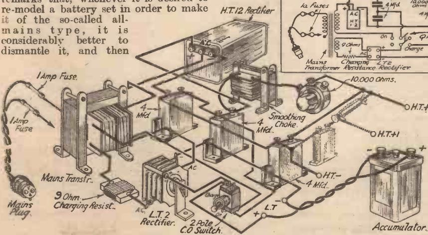
Fig. 2.—The combined H.T. unit and trickle charger shown above is for A.C. operation.
