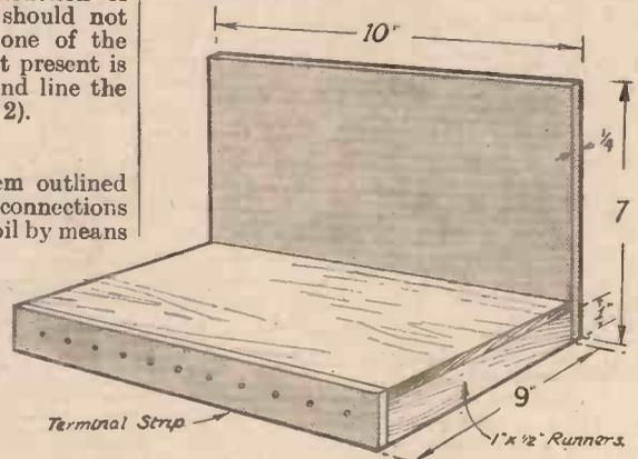
Fig. 2.—Chassis details for the all-range receiver
