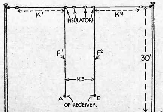
Fig. 4.—A divided aerial: K1 and K2 are equal in length & half the wavelength. K3 = 4 1/2 inches.
