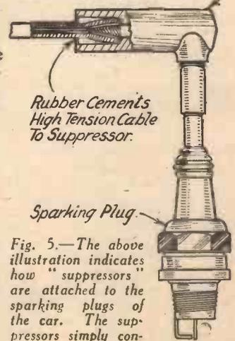
Fig. 5.—The above illustration indicates how "suppressors" are attached to the sparking plugs of the car. The suppressors simply consist of non-inductive resistances of about 50,000 ohms each.
