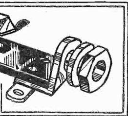
Fig. 6.—A convenient arrangement of a jack for connecting external aerial and earth leads to a portable set.
