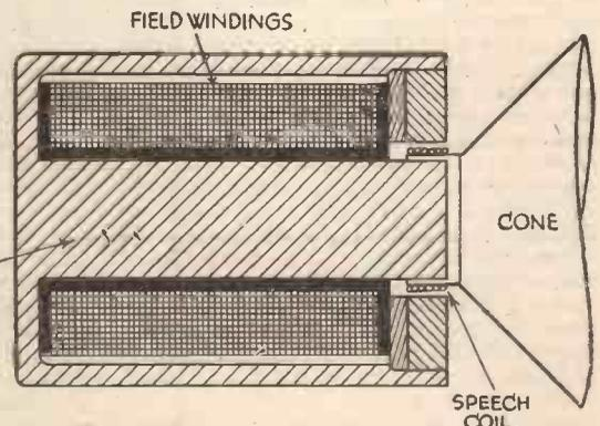
Fig. 3.—Section through an energized moving-coil speaker showing the most important parts.
