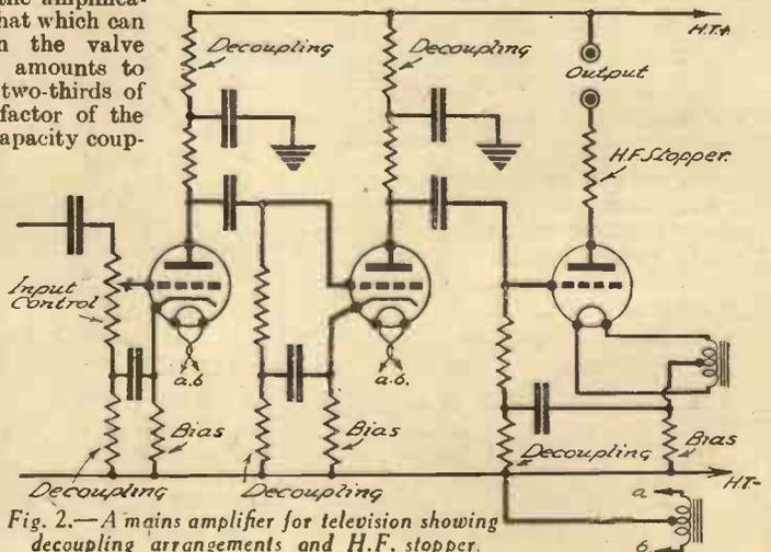
Fig. 2.—A main amplifier for television showing decoupling arrangements and H.F. stopper.
