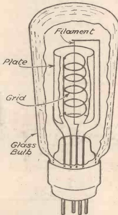
A sketch of a simple valve showing the general arrangement of the electrodes.
