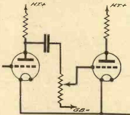
Fig. 1.—The correct position for a volume control in a television amplifier.
