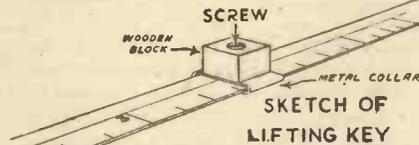
Fig. 2.—The lifting key.
