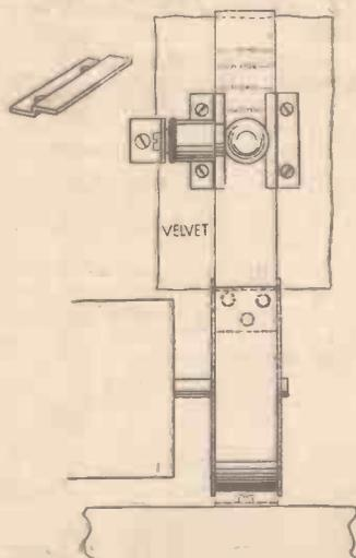
Fig. 3.—Rear view of the simple wavelength, or tuning scale.
