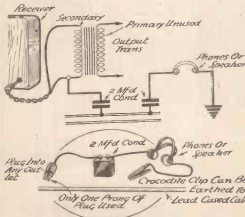
A novel method of fixing an extension speaker.
