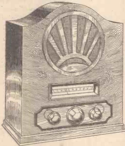
Fig. 1.—The oblong overlay is useful in concealing spindle holes not suited to the chassis.
