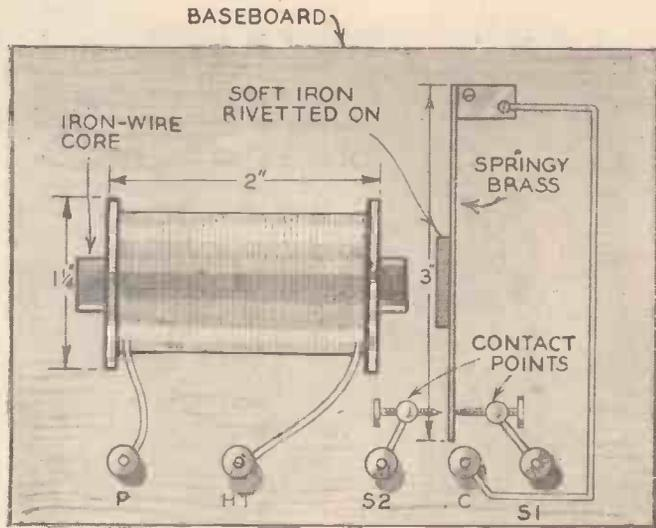
Fig 3.—Showing the constructional details of the relay.
