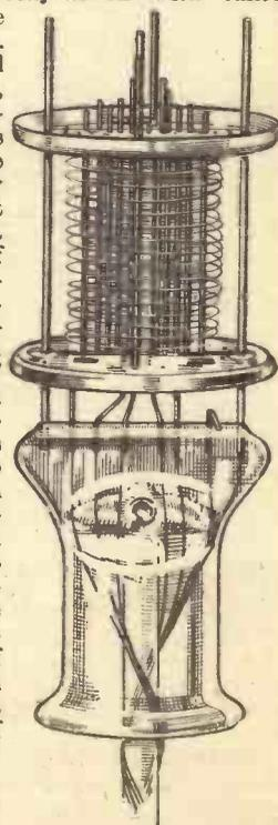
Fig. 3.—The electrode assembly of an octode.
