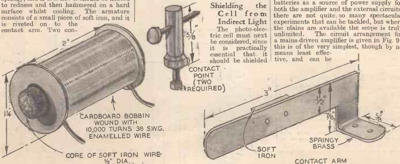
Fig. 4.—Details of the various parts of the relay shown in Fig. 3.
