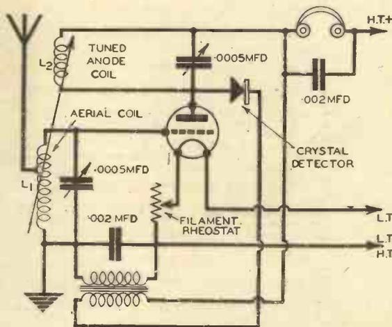
Fig. 1.—An early type of reflex circuit in which a crystal detector was employed.
