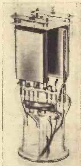
Fig. 2.—Showing the interior construction of a class "B" valve.
