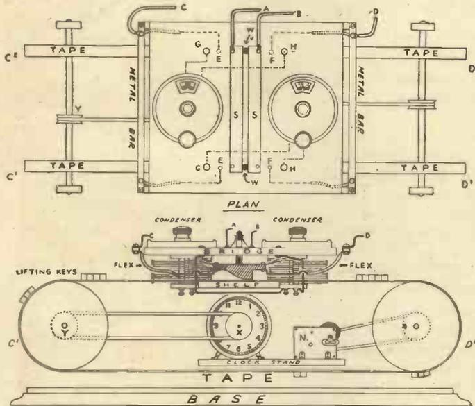
Fig. 1.—Showing the framework, bridge, shelf, clock stand and base.
