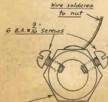
Brass nut drilled out to  $\frac{5}{16}$ " dia
