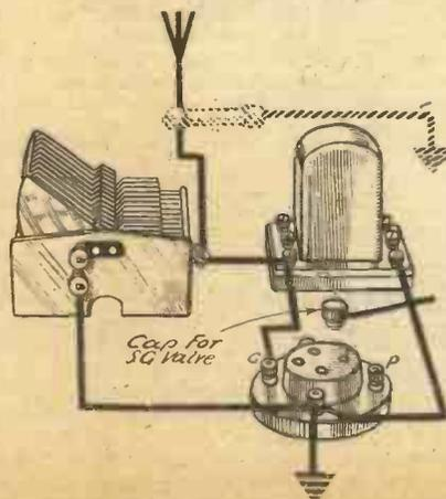
Fig. 2.—When the aerial is connected directly to the "grid" end of the first tuned coil, its low impedance acts as a parallel resistance across the grid-filament circuit of the valve, as shown in broken lines.
