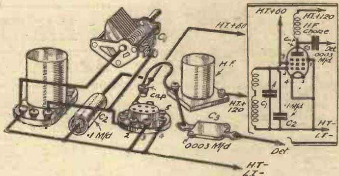
Fig. 2.—Circuit showing a typical H.F. stage using a 7-pin H.F. pentode.
