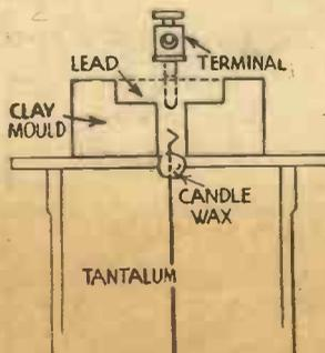
Fig. 1.—How the mould is built up from clay.
