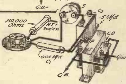
Fig. 6.—Push-pull output stage with separate L.T. supply for each valve.
