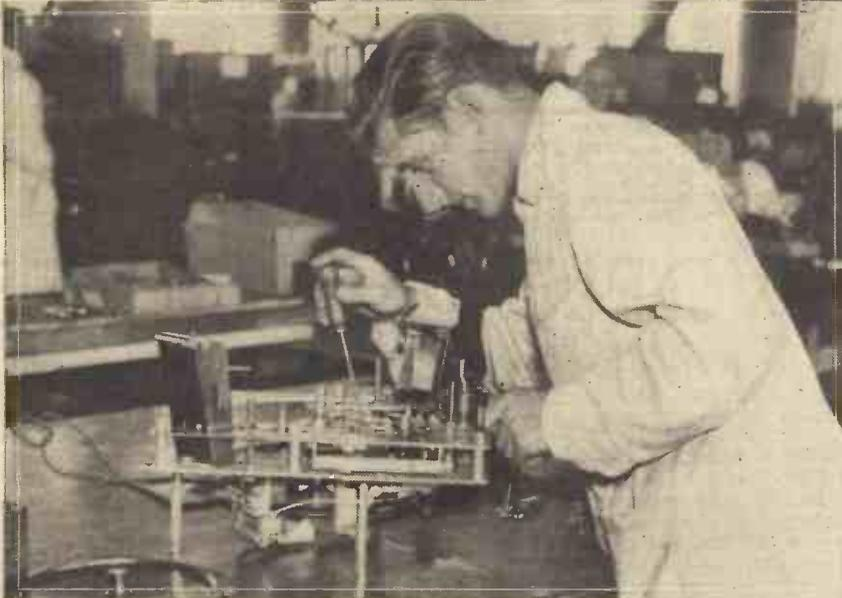
Automatic mechanisms are now an integral part of medium- and higher-priced H.M.V. radio-gramophones. An engineer is seen here making a final adjustment before the automatic chassis is installed in a radio-gramophone at the H.M.V. factories at Hayes, Middlesex.
