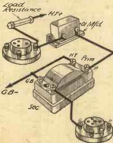
Fig. 1.—Showing the usual connections for parallel-fed transformer coupling.
