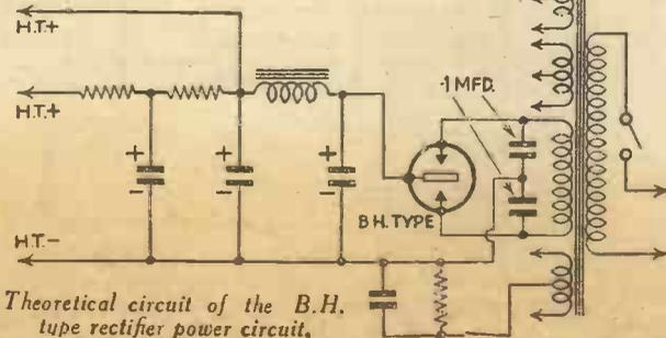
Theoretical circuit of the B.H. tube rectifier power circuit.
