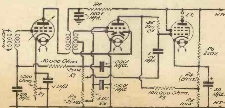
Fig. 2.—The circuit for a double-diode triode used as second detector, automatic-volume control and noise suppressor.
