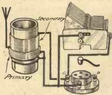
Fig. 4.—The use of a tapping for the aerial gives the same effect as that shown in Fig. 3. The virtual "primary" and "secondary" windings are shown in this drawing.
