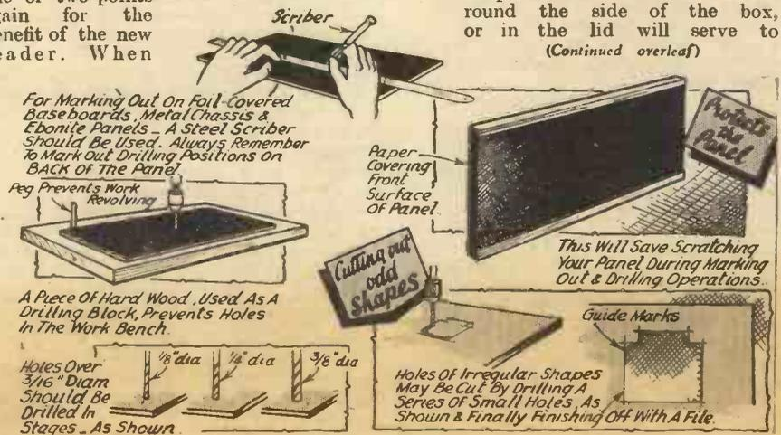
*For Marking Out On Foil-Covered Baseboards, Metal Chassis & Ebonite Panels - A Steel Scriber Should Be Used. Always Remember To Mark Out Drilling Positions On BACK OF THE PANEL.*
