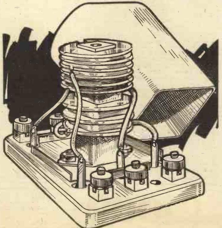
The novel iron-core coil produced by Formo. This illustration is nearly double the size of the actual coil.
