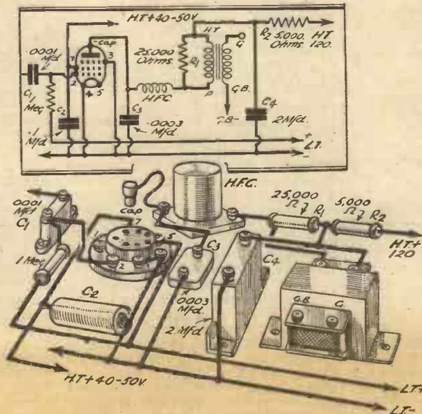
Fig. 3.—An H.F. pentode used as a detector.
