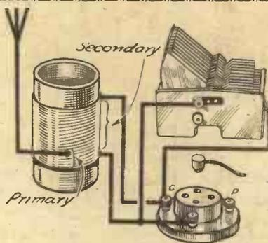
Fig. 3.—When a separate aerial winding is employed, this acts as the primary winding of a step-up transformer and assists in securing correct H.F. matching as explained in text.
