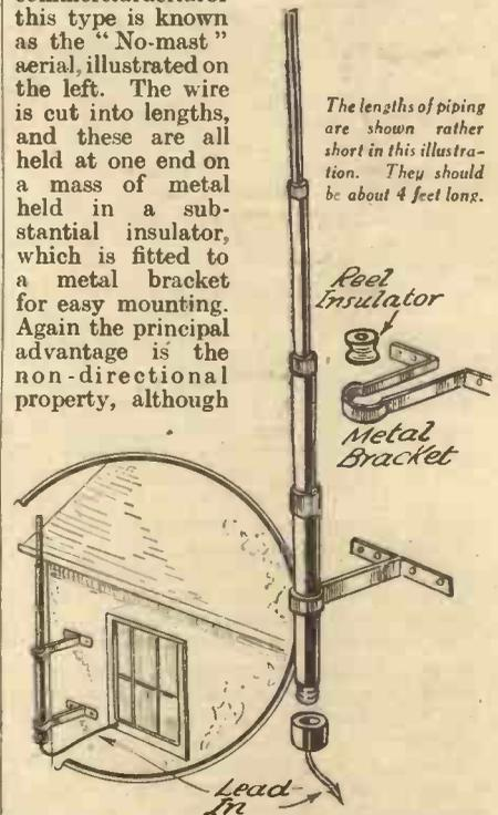
Details of construction of a vertical aerial built up from lengths of gas piping.
