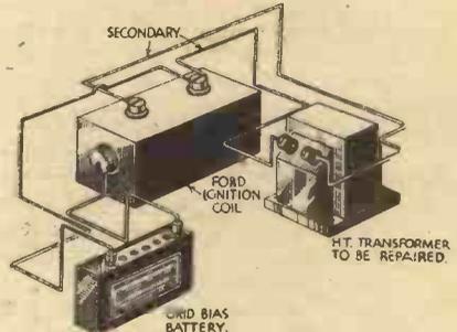
Method of repairing a transformer.
