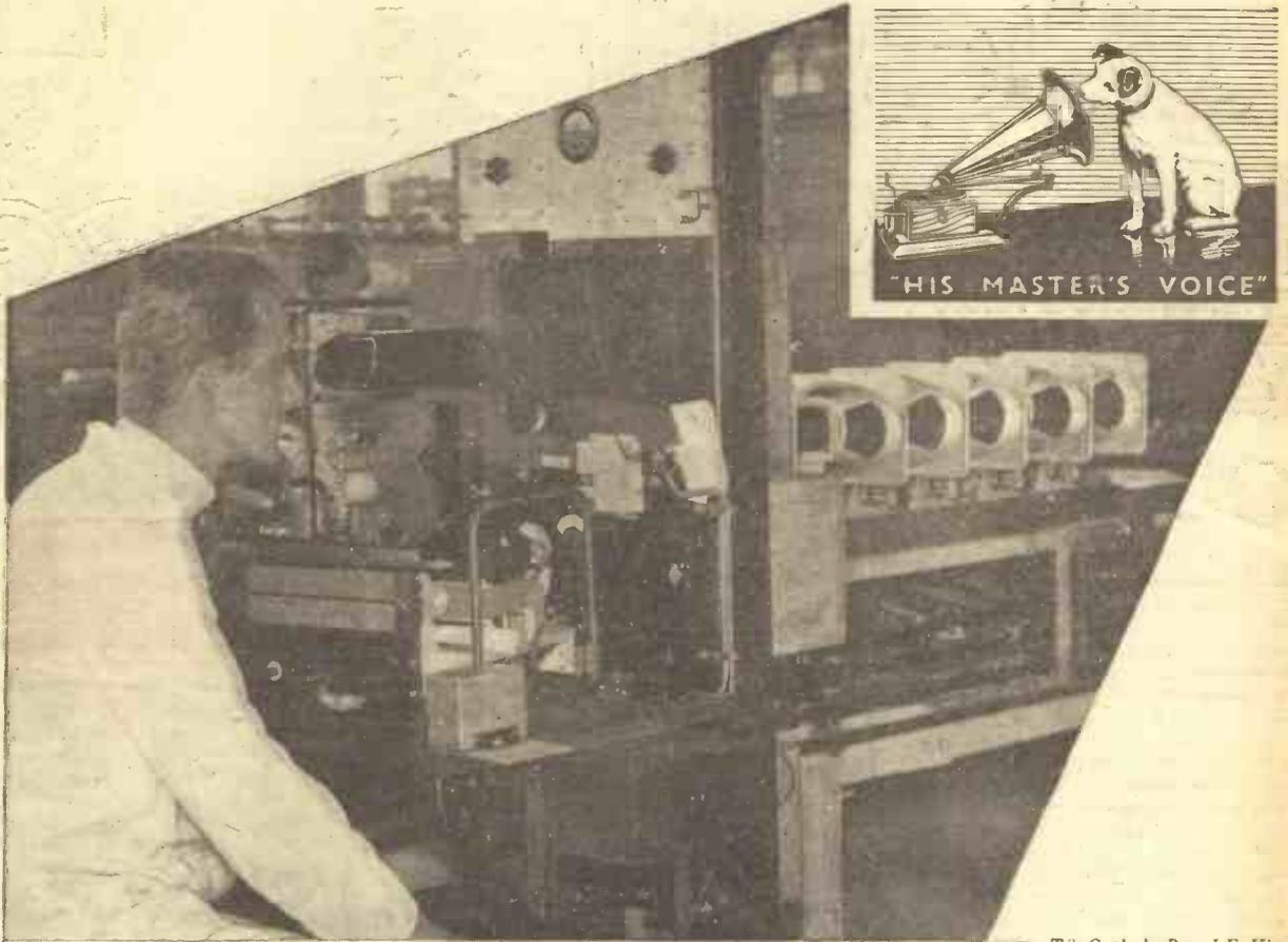
Science and sight combine to test "His Master's Voice" true-to-life tone. The Cathode Ray oscillograph is one of the wonders of science, for it turns sound into something you can see. It converts a musical composition into a graph. This has been incorporated in apparatus specially designed by "His Master's Voice" Research engineers for checking the performance of the intermediate frequency stages of "His Master's Voice" superheterodyne instruments.
