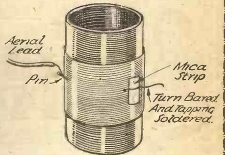
Fig. 5.—The optimum tapping point can be found by connecting the aerial lead to a pin which can be connected to various turns. After that a permanent tapping can be made as shown.
