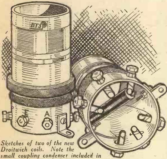
Sketches of two of the new Droitwich coils. Note the small coupling condenser included in the lower end of the coil.
