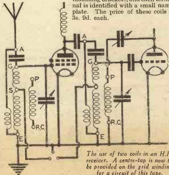
The use of two coils in an H.F. receiver. A centre-tap is now to be provided on the grid winding for a circuit of this type.
