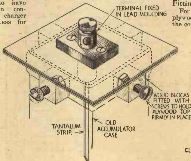
Fig. 3.—Full details of the terminal assembly.
