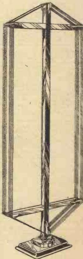
There is no necessity for the windings to be arranged in plane. This square form as is shown by this type of aerial.
