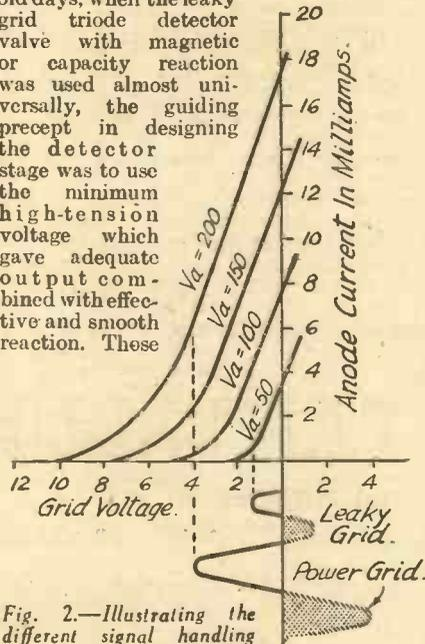
Fig. 2.—Illustrating the different signal handling capabilities of leaky-grid and power-grid detection.
