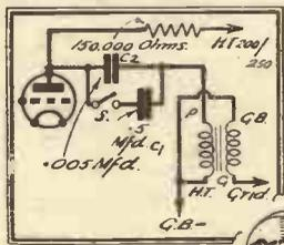
Fig. 5.—Showing bass-boosting coupling.
