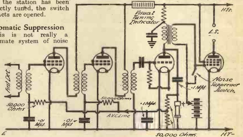
Fig. 1.—Skeleton circuit showing how a switch can be provided for noise suppression with a receiver fitted with a visual-tuning indicator. In this case A.V.C. is provided by means of a Westector. Component values are average ones.
