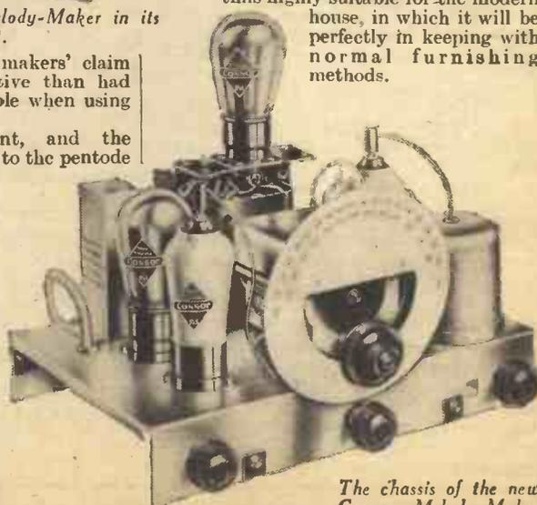
The chassis of the new Cossor Melody-Maker is made of blue steel, and employs a rather unusual form of mounting for the rectifying valve.
