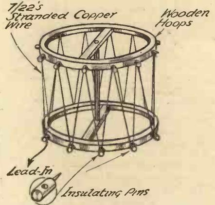
Details for constructing a simple cage-type aerial.
