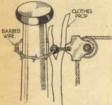
Fixing an aerial pulley to a mast after the halyard has broken
