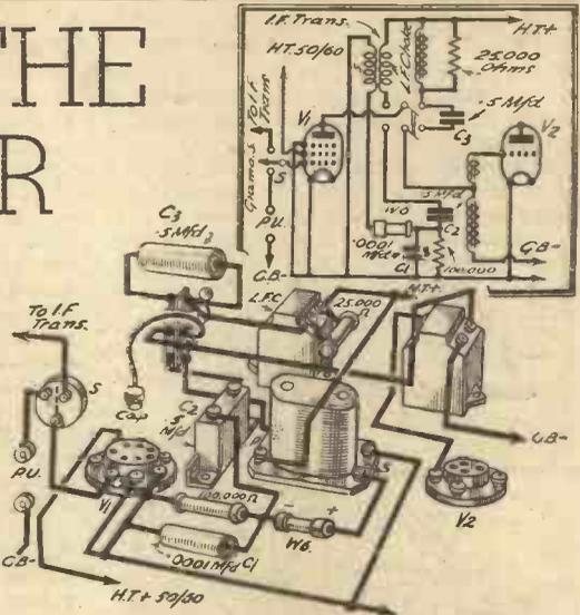
Fig. 4.—H.F. pentode used as L.F. amplifier.
