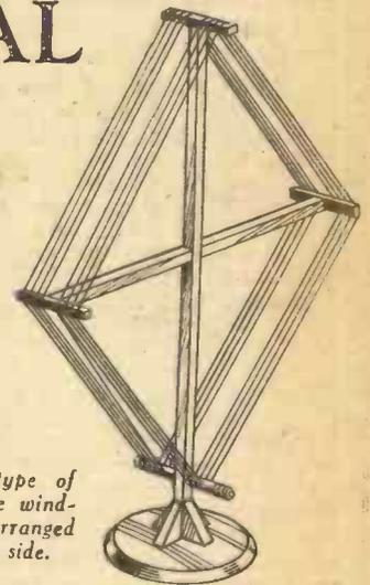
In this type of frame the windings are arranged side by side.
