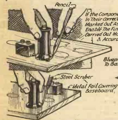
*If the Components Are Arranged In Their Correct Positions & Marked Out As Shown, It Will Enable The Final Assembly To Be Carried Out More Quickly & Accurately.*
