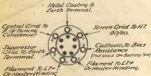
Fig. 1.—The valve holder terminal wiring of a 7-pin H.F. pentode.
