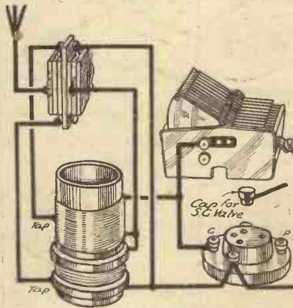
Fig. 6.—Best results are obtained by tapping both long and medium wave windings and using a double-pole wavechange switch connected as shown above.
