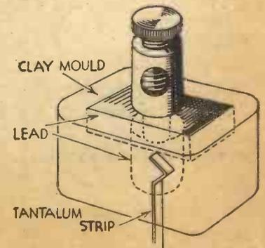
Fig. 2.—Further details of the method of fitting the terminal.
