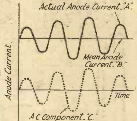
Fig. 3.—The steady or mean output current with the alternating component superimposed.
