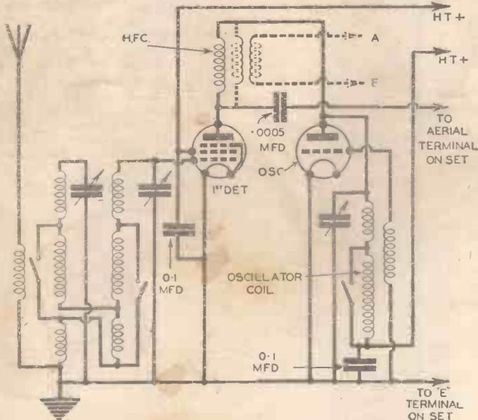
Fig. 1.—The circuit of a simple superhet unit intended for working at an intermediate frequency of 150 kilocycles.
