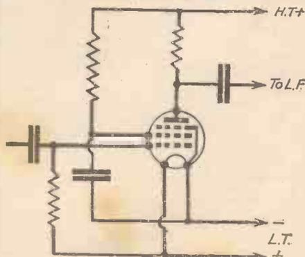
Fig. 2.—Circuit connections for a typical H.F. pentode detector circuit.
