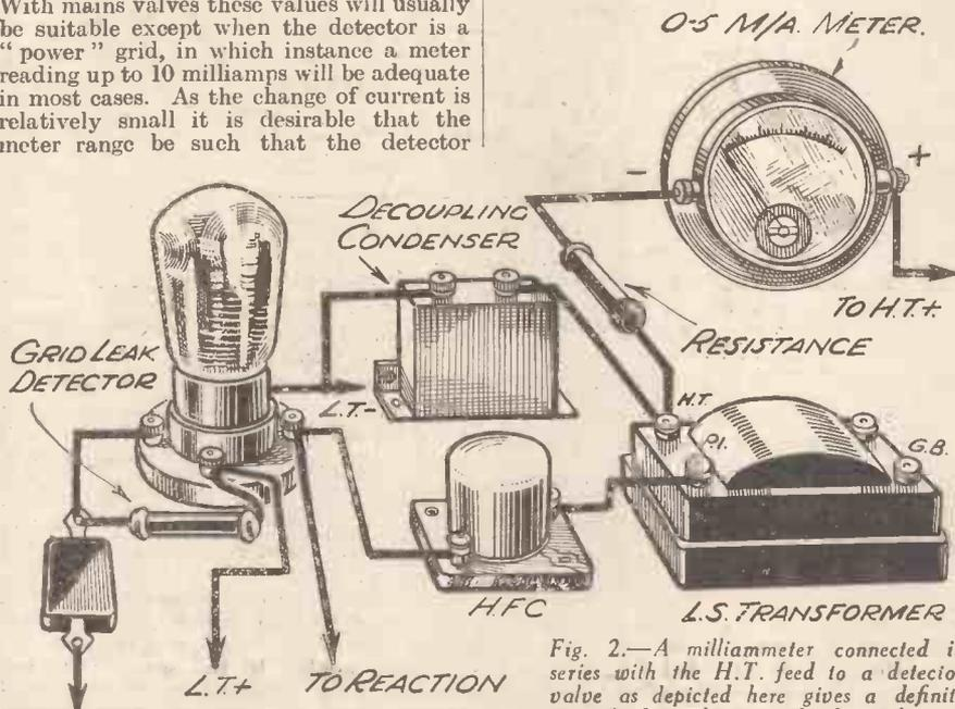
Fig. 2.—A milliammeter connected in series with the H.T. feed to a detector valve as depicted here gives a definite check on the strength of signals.
