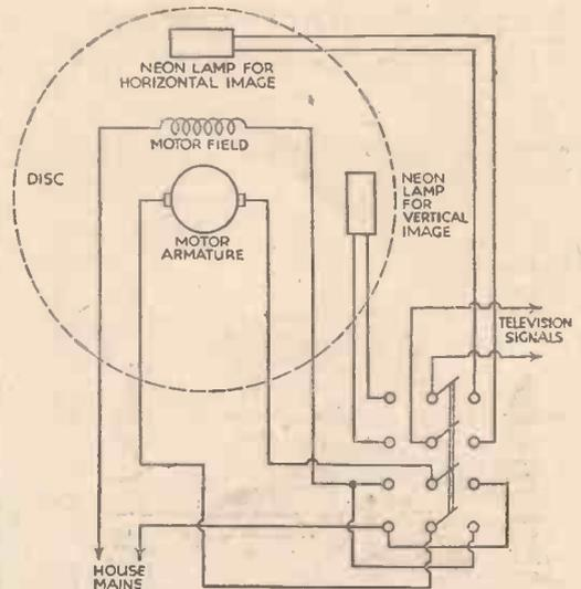
Fig. 10.—The simple switching arrangement for changing motor direction and neon lamp connections.
