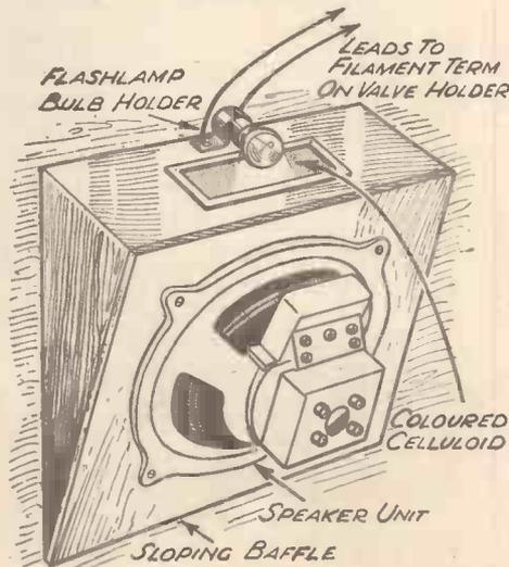
Fig. 3.—This drawing shows a small refinement which might well be fitted to a speaker mounted on a sloping baffle—it takes the form of a lamp for floodlighting the speaker opening.
