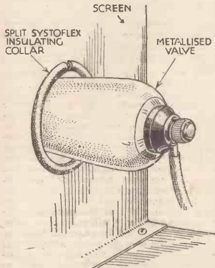
Using a piece of systoflex for protecting a metallised valve where it passes through a screen.
