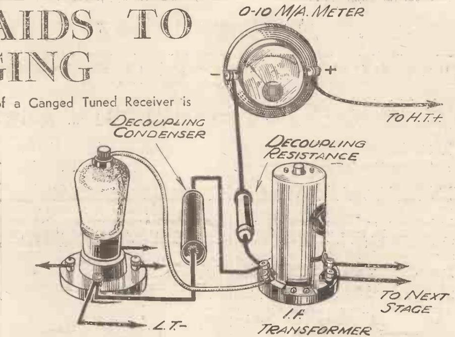
Fig. 1.—This shows a milliammeter connected in the anode circuit of an A.V. controlled I.F. valve of a superhet to serve as a tuning indicator for both ganging and normal tuning purposes.
