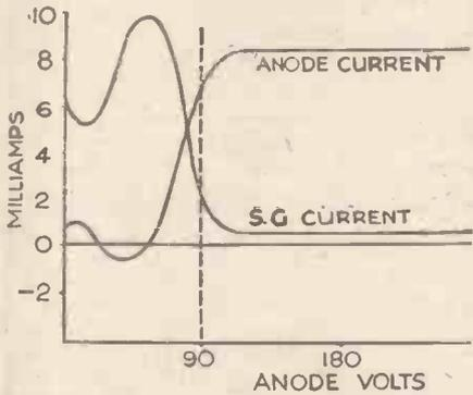
Fig. 1.—Typical curves for an S.G. valve
