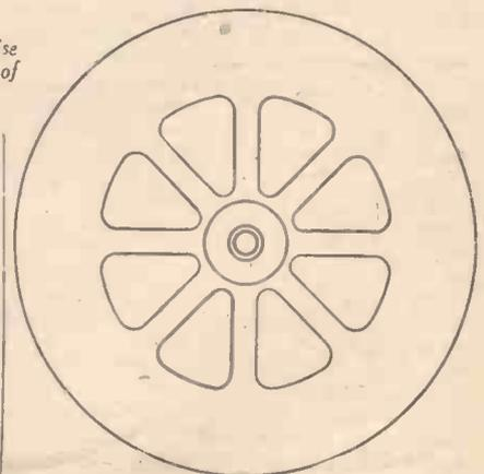
Fig. 9.—Lightening the disc by cutting away sectors to give eight spokes.
