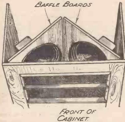
Fig. 5.—It is frequently worth while to arrange a pair of speakers on baffle boards set at an angle to each other, as shown here..
