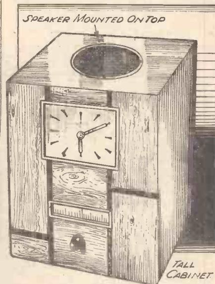
Fig. 4.—Excellent reproduction can often be obtained by mounting the speaker in the top of a tall cabinet, etc., so that it faces upwards.
