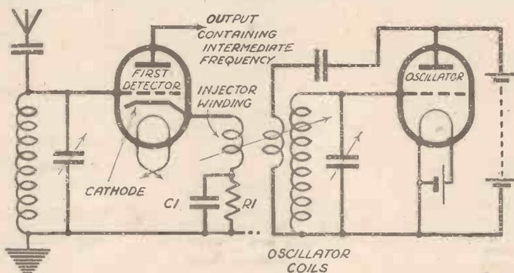
Fig. 8.—The "cathode injector" method of frequency changing.
