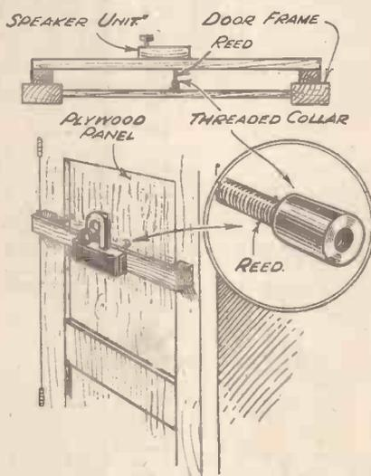
Fig. 2.—A type of speaker which often functions admirably, and can be made from an old moving-iron or reed-type unit.
