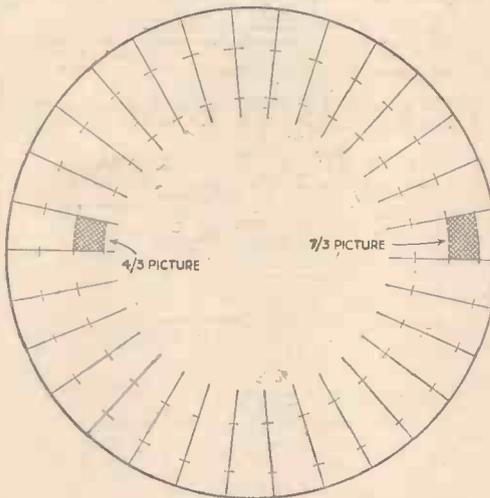
Fig. 7.—The disc marked out with an outer clockwise spiral of holes and an inner with a clockwise spiral of holes.
