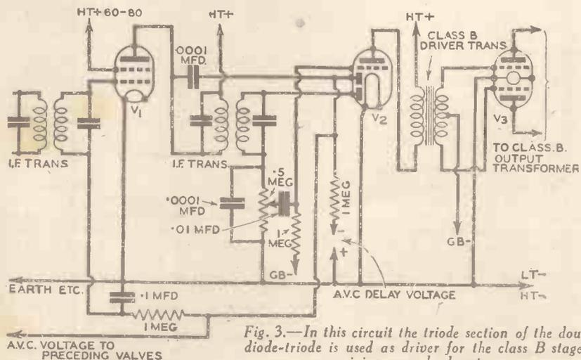
Fig. 3.—In this circuit the triode section of the double-diode-triode is used as driver for the class B stage, so giving several advantages.
