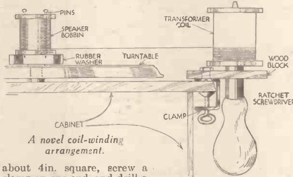
A novel coil-winding arrangement.
