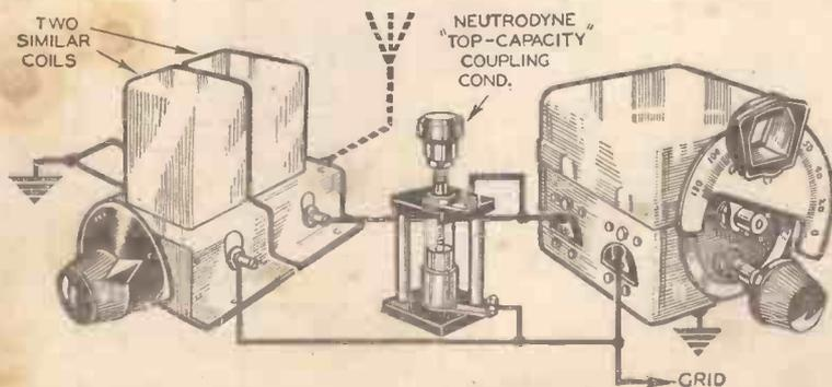
Fig. 3.—Showing how two ordinary and similar coils can be used in a band-pass circuit by employing a neutrodyne condenser to provide "top-capacity" coupling.
