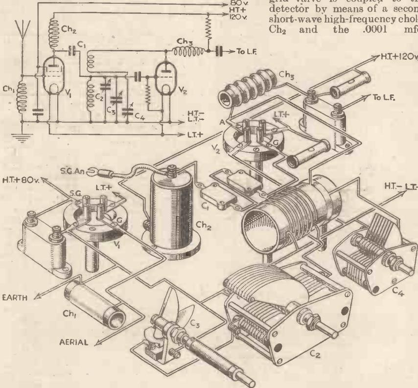
A typical two-valve short-wave circuit using an untuned H.F. stage and band-spread tuning.
