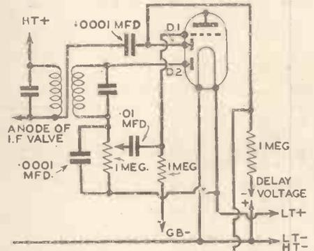
Fig. 2.—A delayed automatic-volume-control circuit.
