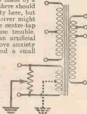
Fig. 1.—Hum may be prevented by connecting the earth lead to a potentiometer across the heater winding.
