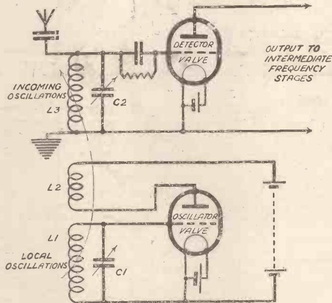
Fig. 7.—A simple frequency changer. A local alternating current is produced by the oscillator valve and "mixed" with the incoming oscillation by the coupling of the coils L1, L2, and L3, thus producing the intermediate frequency.
