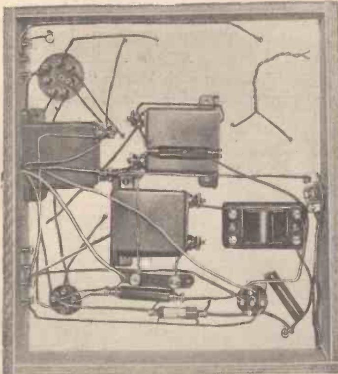
This illustration shows the underside of chassis, from which it will be seen that there is ample room for decoupling components when an inefficient mains unit is employed.
