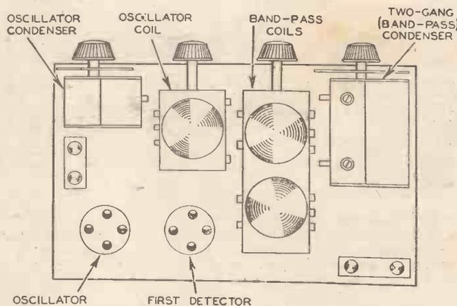
Fig. 4.—A good arrangement of components in a superhet unit in which separate valves are used for first detector and oscillator and separate coil and condensers. The layout could be simplified if a multi-electrode valve were used in conjunction with a special coil assembly.
