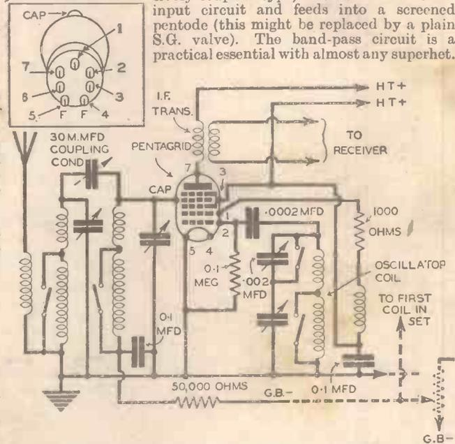
Fig. 2.—The general circuit for a superhet unit employing a pentagrid frequency-changer. If desired, the I.F. transformer shown may be replaced by a choke-condenser combination. Inset shows the connections (underside) to the pentagrid 7-pin valveholder.
