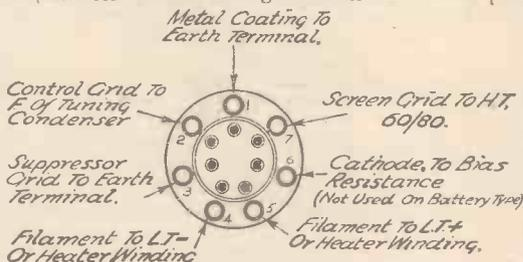
Fig. 1.—Indicating the valveholder terminal connection of a 7-pin H.F. pentode.
