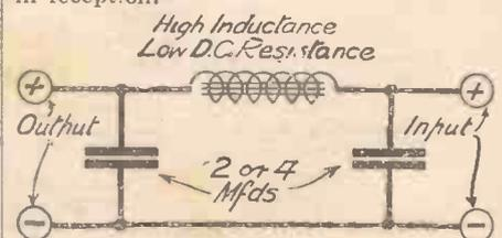
Fig. 4.—The normal A.C. mains smoothing circuit for use on D.C. or universal receivers.
