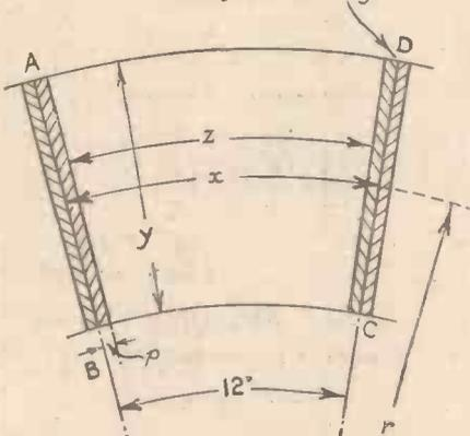
Fig. 6.—Details for marking out a disc to receive the German transmission.
