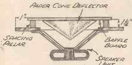
Fig. 1.—The ingenious speaker arrangement used in the "All-Pentode" Three, and which is described in the accompanying text.
