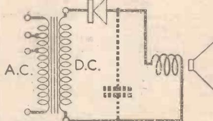
Fig. 2.—A large capacity fixed condenser across the low-voltage field winding.
