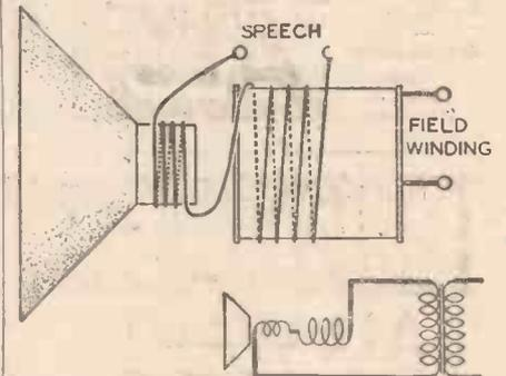
Fig. 3.—A hum-bucking coil used with a mains-energised speaker.
