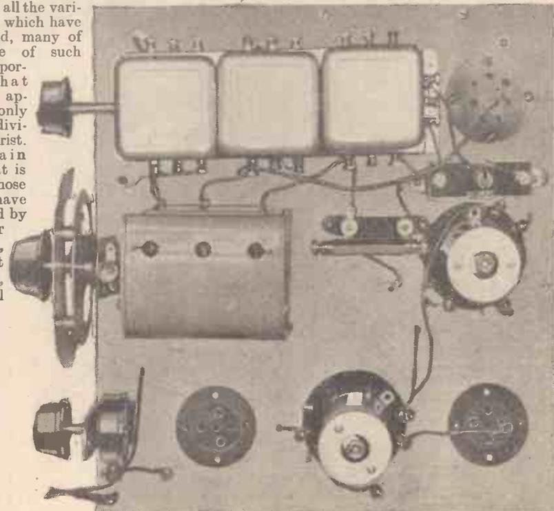
This plan view shows the neat and simple appearance of the upper side of the chassis.
