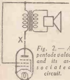
Fig. 2.—A pentode valve and its associated circuit.
