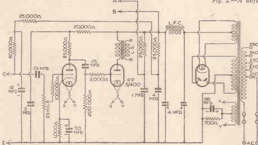
Fig. 1.—Circuit of a small A.C. mains amplifier.
