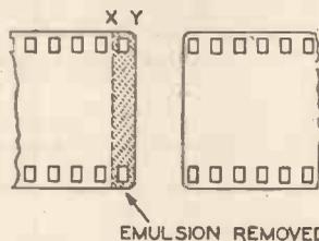
Fig. 5.—Preparing the film for jointing.
