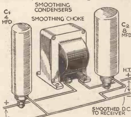
Fig. 1.—The simplest and most usual type of H.T. smoothing circuit. A usual value for the choke is 20-30 henries (at the full H.T. current), while C1 and C2 generally have values of 4 mfd. and 8 mfd. respectively.
