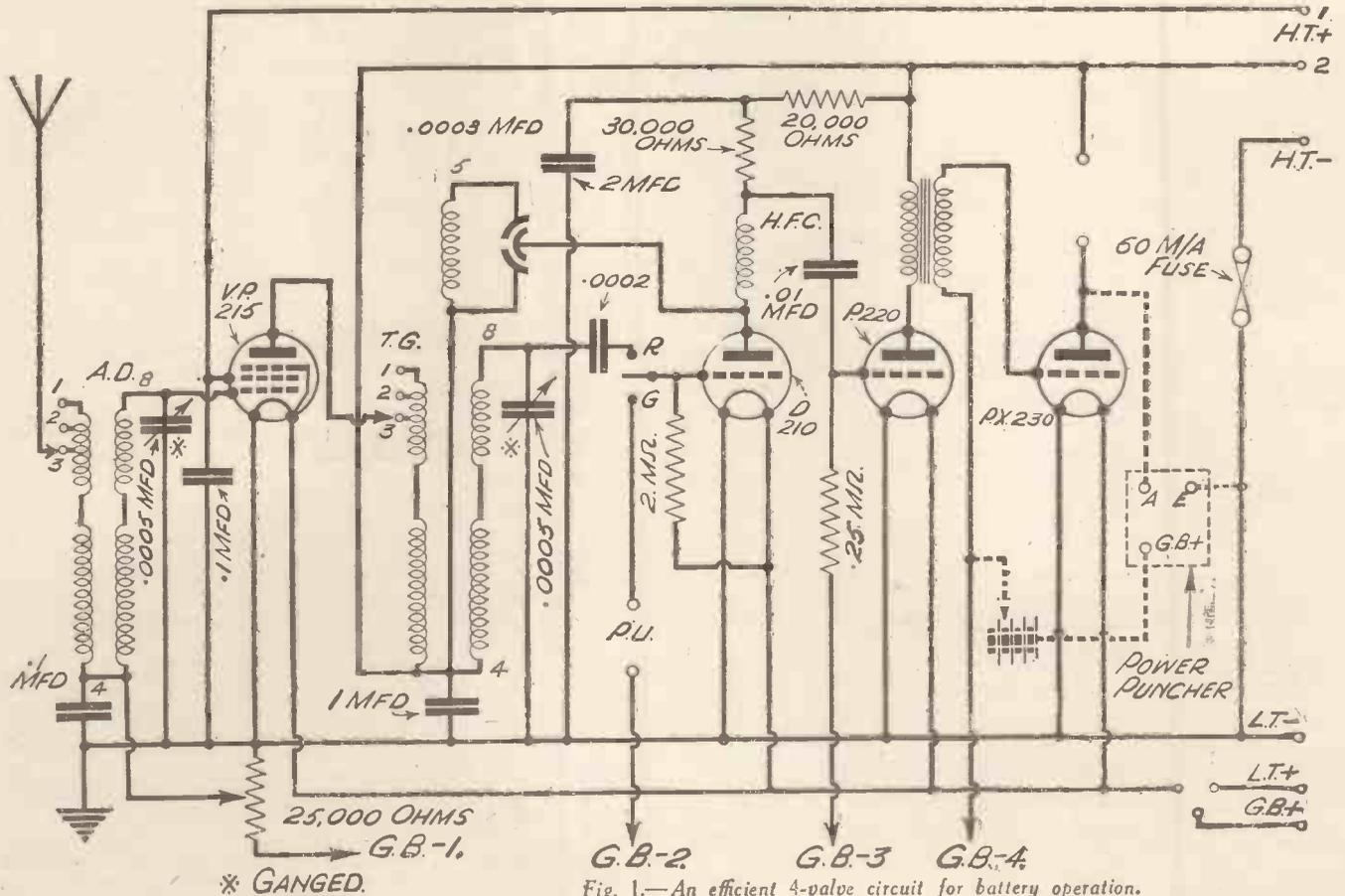
Fig. 1.—An efficient 4-valve circuit for battery operation.
