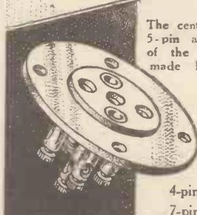
The centre socket of the 5-pin and two sockets of the 7-pin type are made longer than the others; this reduces the possibility of short-circuits and adds to the ease of wiring.
