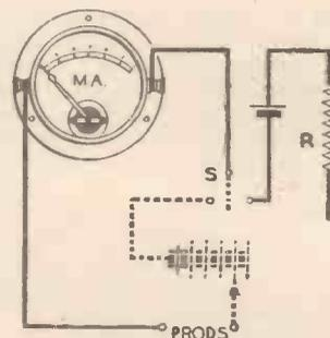
Fig. 5.—Testing a component, here represented by the resistance "R."
