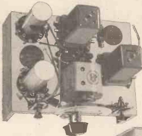
Three views of the Two-valve Superhet showing the compactness and simplicity of wiring.
