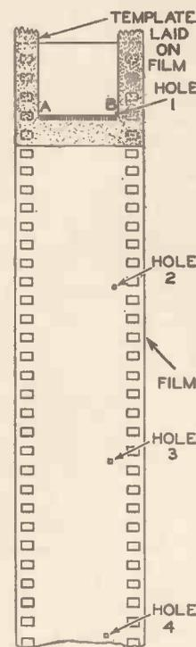
Fig. 3.—Showing how the separate scanning holes are marked off on the film.
