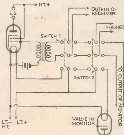
Circuit diagram of a switching arrangement for an amplifier and monitor valve.
