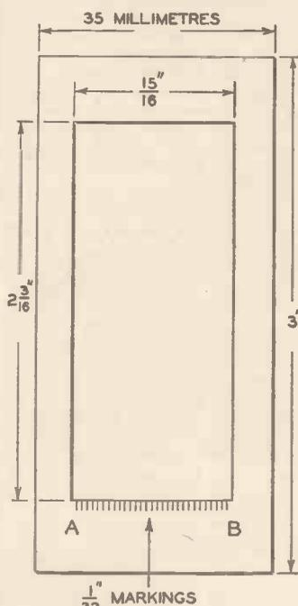
Fig. 2.—Details of the metal template.
