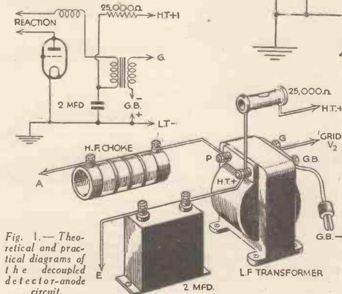
Fig. 1.—Theoretical and practical diagrams of the decoupled detector-anode circuit.
