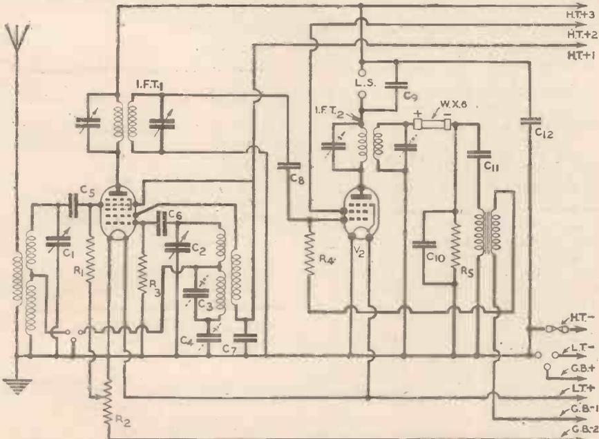
Fig. 1.—Theoretical circuit of the 2-valve Superhet.
