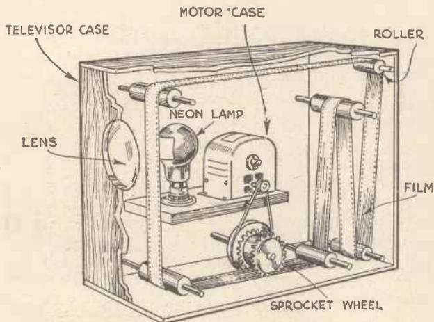
Fig. 1.—Constructional details of a film scanner receiver.
