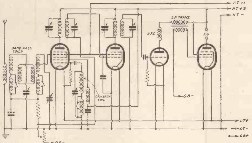
Fig. 4.—A theoretical circuit showing the principal features of a modern 4-valve superhet of simple type.
