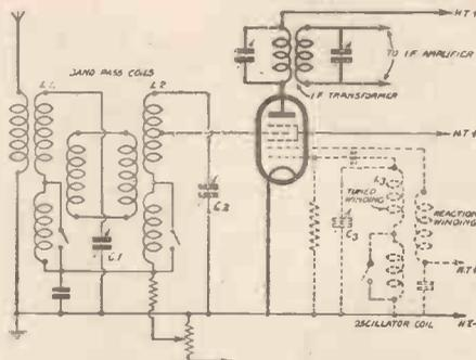
Fig. 2.—This circuit of a pentagrid frequency changer shows the valve actually comprising two sets of electrodes. The circuit of the S.G. first detector portion is shown in full lines, that of the triode oscillator in broken lines, and that portion which is common to both is in heavy lines. Values of components are not shown because these are interdependent.
