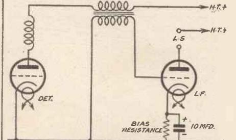
Fig. 3.—A single-valve L.F. output stage for A.C. operation. This will give an output equal to, or greater than, that provided by the circuits in Figs. 1 and 2.
