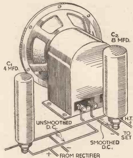
Fig. 2.—This circuit is similar in principle to that shown in Fig. 1, but the smoothing choke is replaced by the field windings of an energized moving-coil speaker.
