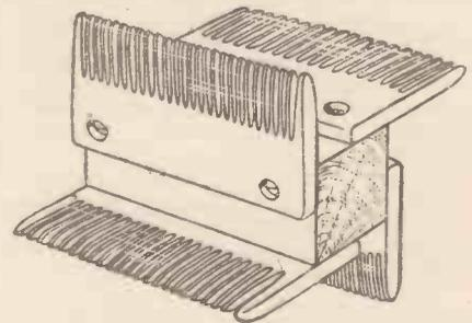
A short-wave coil former made with combs.
