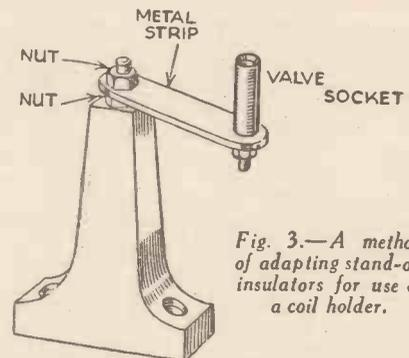
Fig. 3.—A method of adapting stand-off insulators for use as a coil holder.
