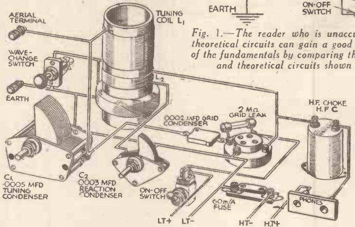
Fig. 1.—The reader who is unaccustomed to theoretical circuits can gain a good knowledge of the fundamentals by comparing the pictorial and theoretical circuits shown here.
