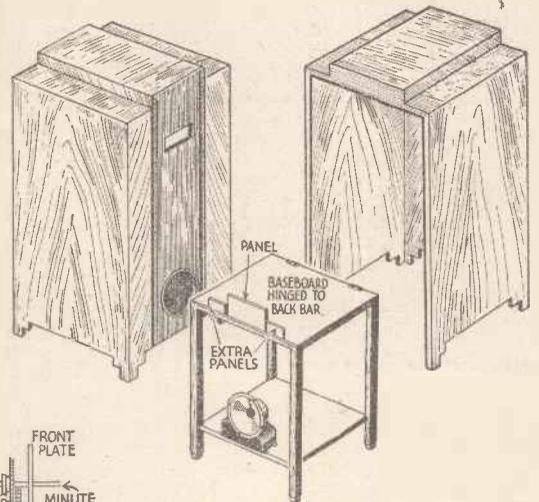
A method of cabinet construction which combines good appearance with easy accessibility.
