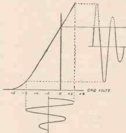
Fig. 2.—If a signal is too powerful, or the wrong type of valve is employed, grid current will flow and introduce distortion.
