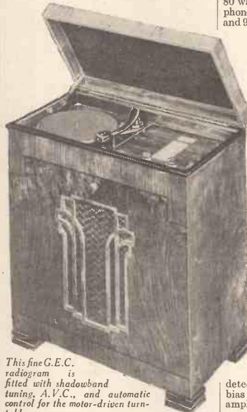
This fine G.E.C. radiogram is fitted with shadowband tuning, A.V.C., and automatic control for the motor-driven turntable.
