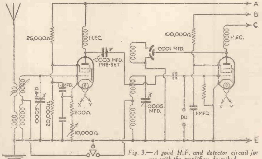
Fig. 3.—A good H.F. and detector circuit for use with the amplifiers described.
