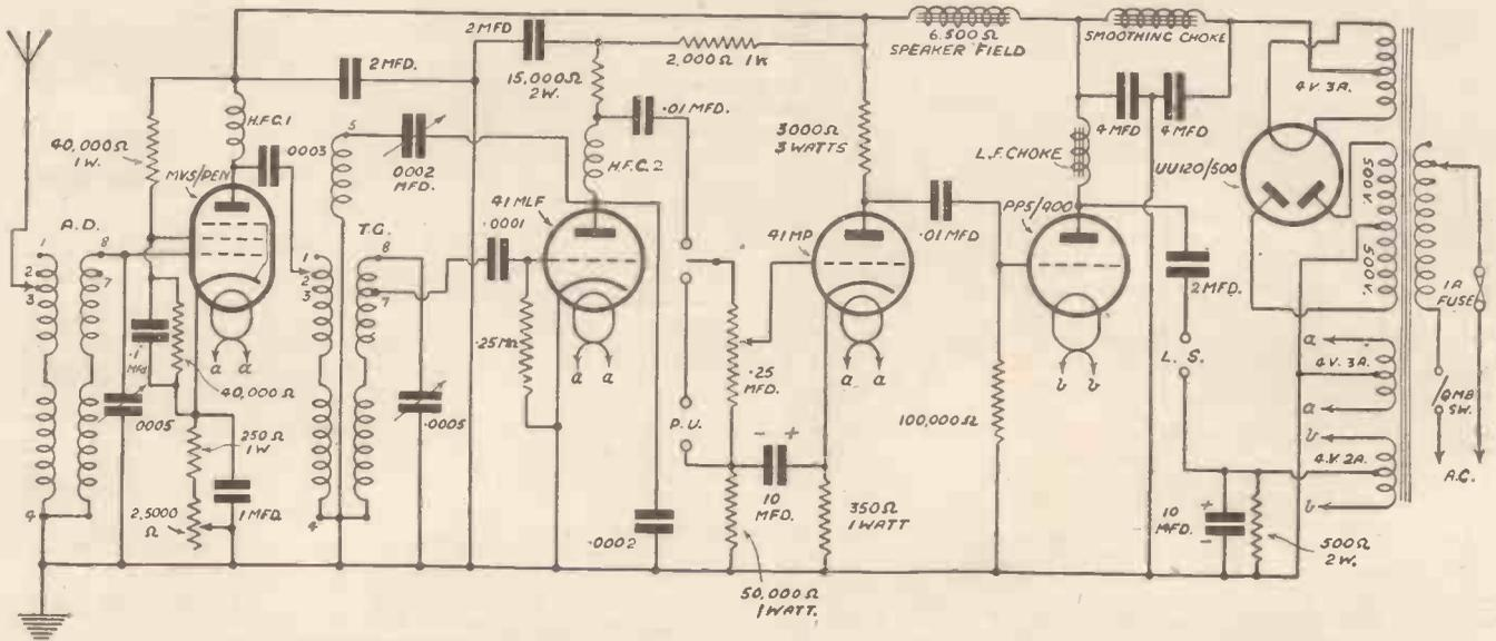
The circuit described.—Wave-change switches are not shown, since they are incorporated in the coils.
