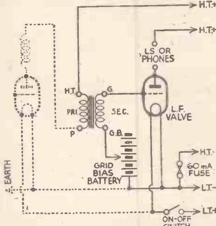
Fig. 3.—Theoretical and pictorial circuits for a simple transformer-coupled L.F. amplifier suitable for use in conjunction with the H.F. and detector circuits shown in Figs. 1. and 2. Notice that the on-off switch is transferred from the position shown in Fig. 1. and is in series with the lead from the + terminal of the accumulator.
