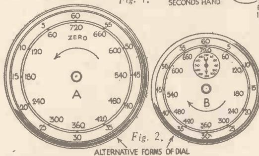
Adapting the works of an alarm clock for use as a turns counter.
