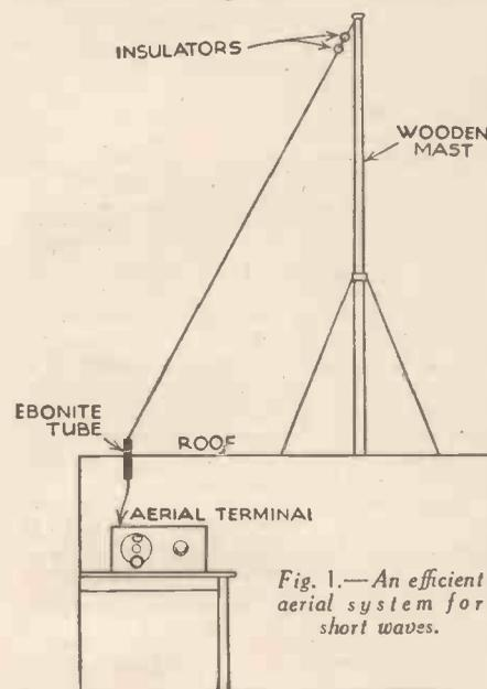
Fig. 1.—An efficient aerial system for short waves.
