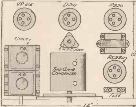
Fig. 2.—Suggested layout for the components of the 4-valve set.
