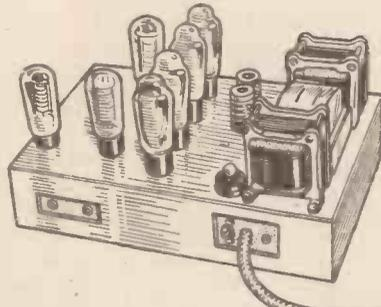
Fig. 2.—A separate amplifier unit is generally connected to the receiver through a multi-cable. Care is necessary in the selection of the gauge of wires for such cable.
