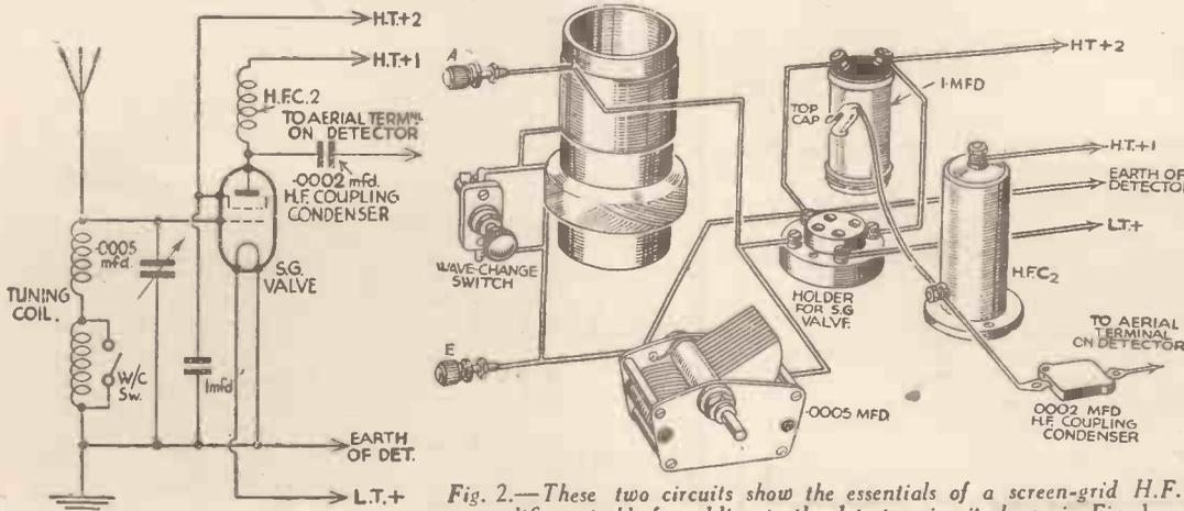
Fig. 2.—These two circuits show the essentials of a screen-grid H.F. amplifier suitable for adding to the detector-circuit shown in Fig. 1.
