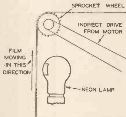
Fig. 6.—Showing how the sprocket wheel should act as a drive on the film.
