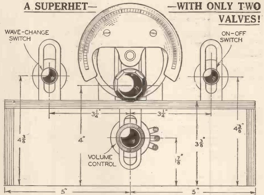
Fig. 2.—Control layout which will assist in drilling the cabinet front.
