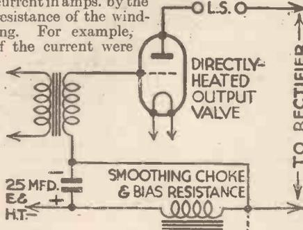
Fig. 4.—Showing how the smoothing choke may sometimes be used as a bias resistance when connected in the negative H.T. lead.
