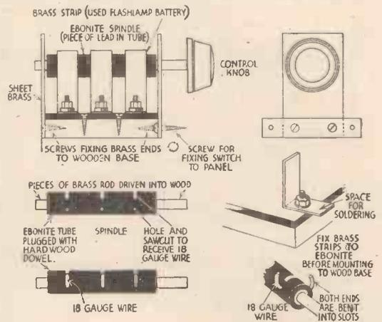
Details of construction of a compact three-way switch.
