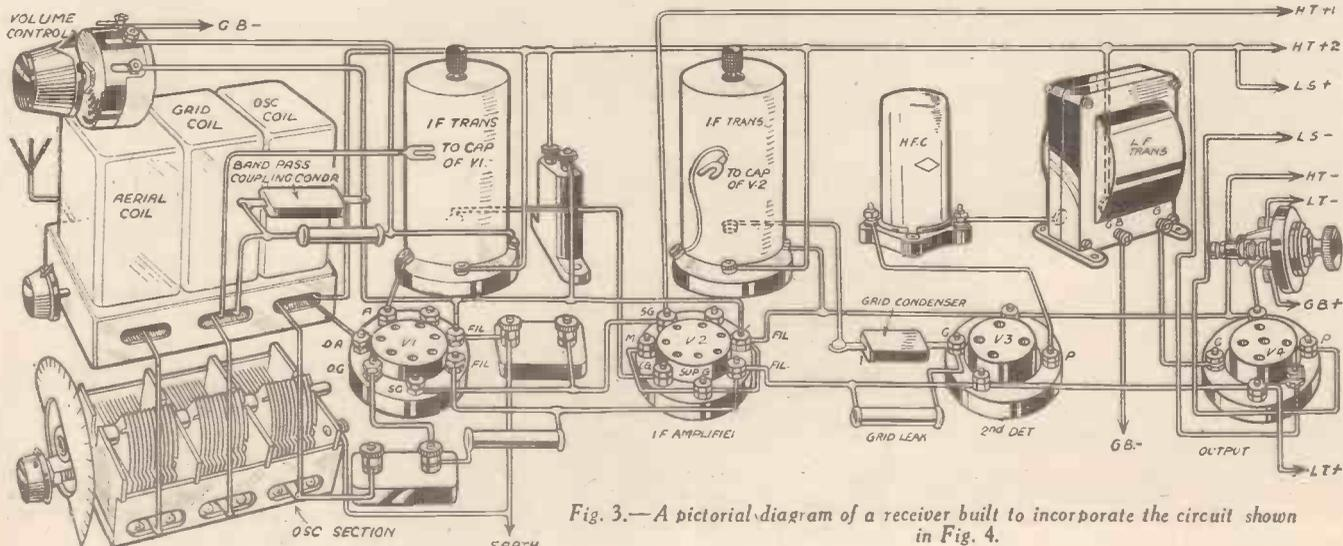
Fig. 3.—A pictorial diagram of a receiver built to incorporate the circuit shown in Fig. 4.
