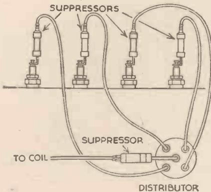
The method of fitting noise suppressors.
