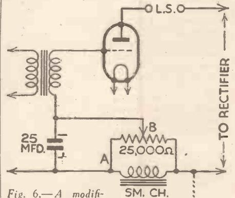
Fig. 6.—A modification of the circuit shown in Fig. 5. In this case the bias voltage is obtained from a potentiometer in parallel with the smoothing choke.
