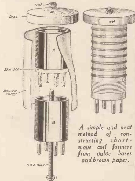
A simple and neat method of constructing short-wave coil formers from valve bases and brown paper.
