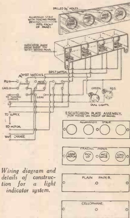
Wiring diagram and details of construction for a light indicator system.
