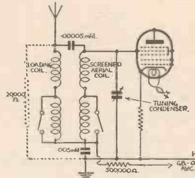
Fig. 6.—Showing the connections for an "image filter" suitable for use in conjunction with a single-circuit aerial tuner of a 465 kc/s superhet.
