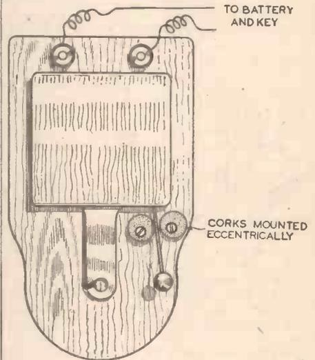
A high-note buzzer made from an old bell.
