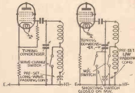
Fig. 2.—These circuits show alternative connections for the long-wave padding condenser.
