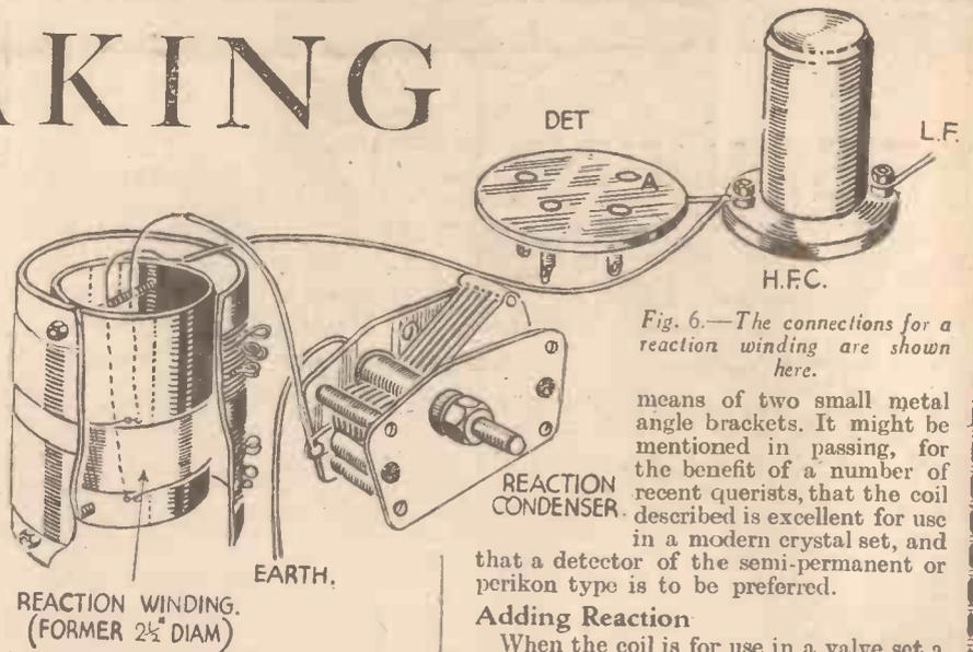
Fig. 6.—The connections for a reaction winding are shown here.
