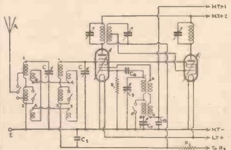
Fig. 4.—An inductive coupling arrangement with Ward and Goldstone coils.
