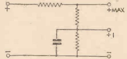
Fig. 3.—A simple method of obtaining a lower H.T. voltage.
