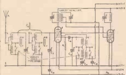
Fig. 3.—An inductive coupling arrangement using Varley coils.
