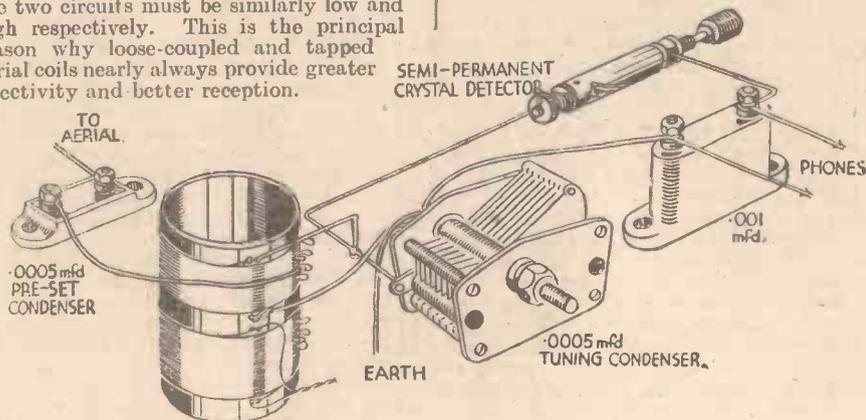
Fig. 4.—This shows the method of using the coil in a modern crystal-set circuit.
