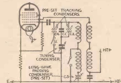
Fig. 1.—This skeleton circuit shows the complicated system of condensers required in the oscillator circuit when using certain types of coil in a 465 kc/s circuit.
