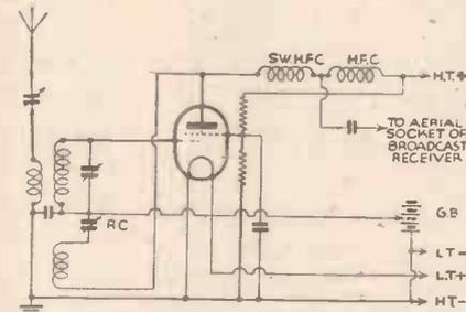
Fig. 1.—A simple S.W. converter in which an S.G. valve operates as an anode-bend first detector and frequency changer.
