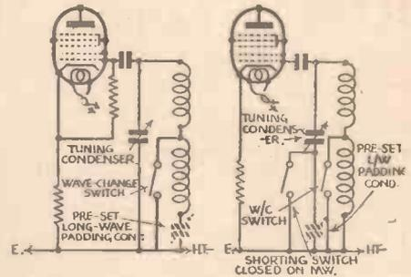
Fig. 2.—These circuits show alternative connections for the long-wave padding condenser.
