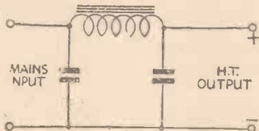
Fig. 1.—The essential circuit of the D.C. mains unit.
