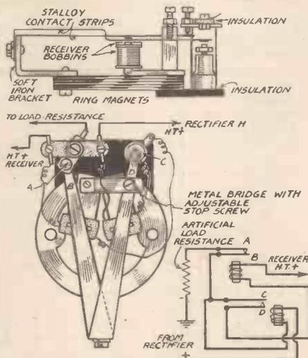
A telephone earpiece is used for making this delay action relay.
