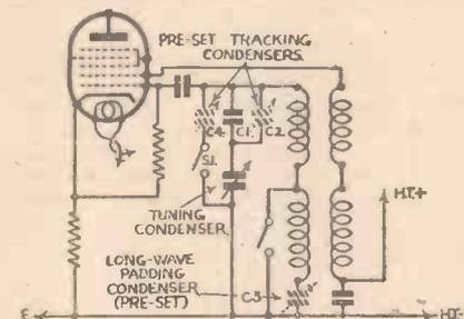
Fig. 1.—This skeleton circuit shows the complicated system of condensers required in the oscillator circuit when using certain types of coil in a 465 kc/s circuit.
