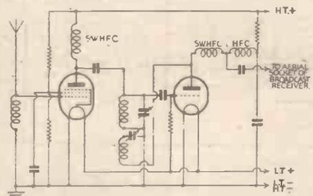
Fig. 2.—A superhet S.W. converter using simple autodyne circuit with an untuned H.F. amplifier to reduce re-radiation.
