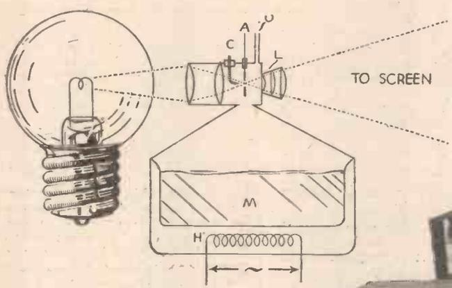
The illustration, Fig. 1, below shows the complete dual apparatus, and the diagram on the left, Fig. 2, shows the theoretical arrangement of the picture producer.
