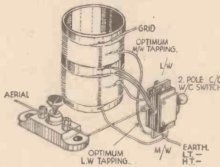
Fig. 5.—Connections for a wave-change switch.
