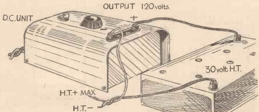
Fig. 5.—How the voltage output of a D.C. mains unit may be augmented.
