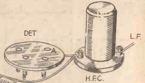
Fig. 6.—The connections for a reaction winding are shown here.
