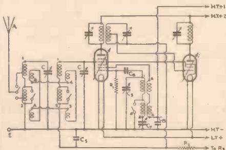
Fig. 4.—An inductive coupling arrangement with Ward and Goldstone coils.
