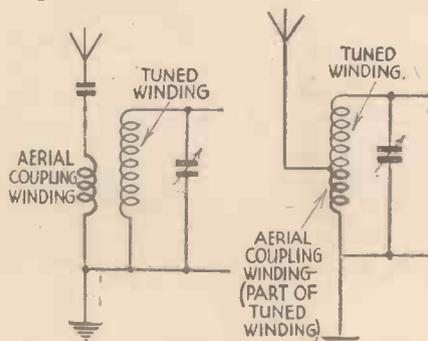
Figs. 1 and 2 (left and right).—These circuits show the similarity between a loose-coupled and tapped aerial coil.
