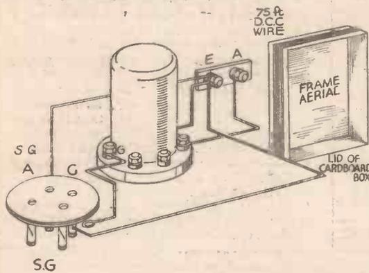
Showing the connection for an improvised frame aerial used with a det.-L.F. receiver (right) and with an S.G. receiver (left).
