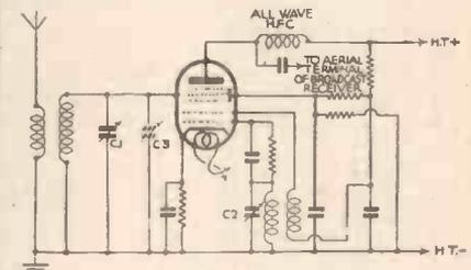
Fig. 3.—A mains-operated S.W. superhet converter using heptode frequency changer. C1 and C2 are ganged, and C3 is a variable trimmer.
