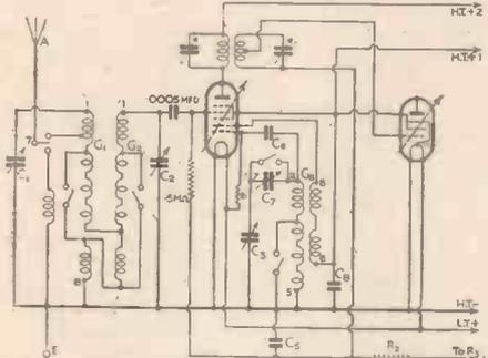
Fig. 5.—Circuit diagram showing the terminal connections for Colvern superhet coils.
