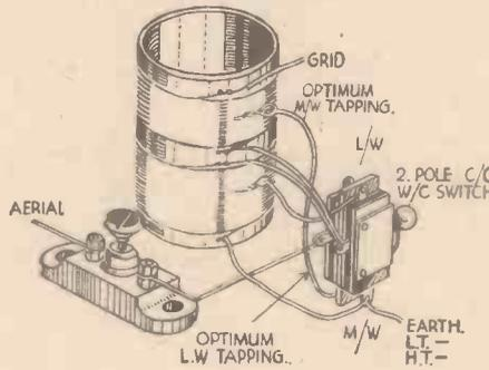
Fig. 5.—Connections for a wave-change switch.
