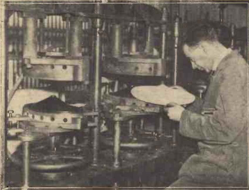
Removing a cone from the blocking machine which reduces it from a thick pulpy cone to a closely-woven cone of the correct thickness and weight.
