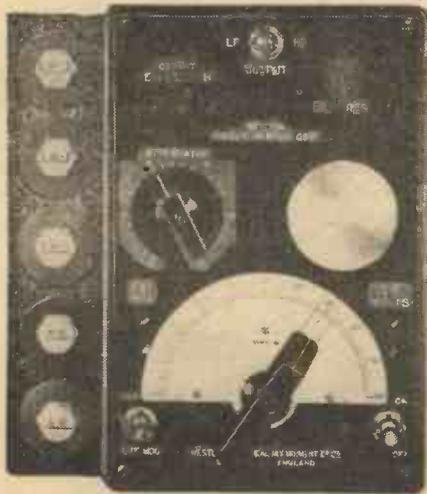
The Weston Oscillator, one of the many measuring devices produced by the Weston Electrical Instrument Company.
