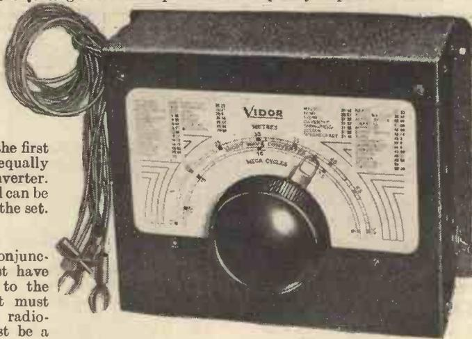
A useful commercial converter—the Vidor Battery Model, covering the Band from 13 to 50 metres.
