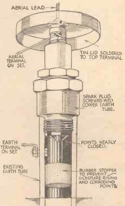
A novel lightning arrester, incorporating an old sparking plug.
