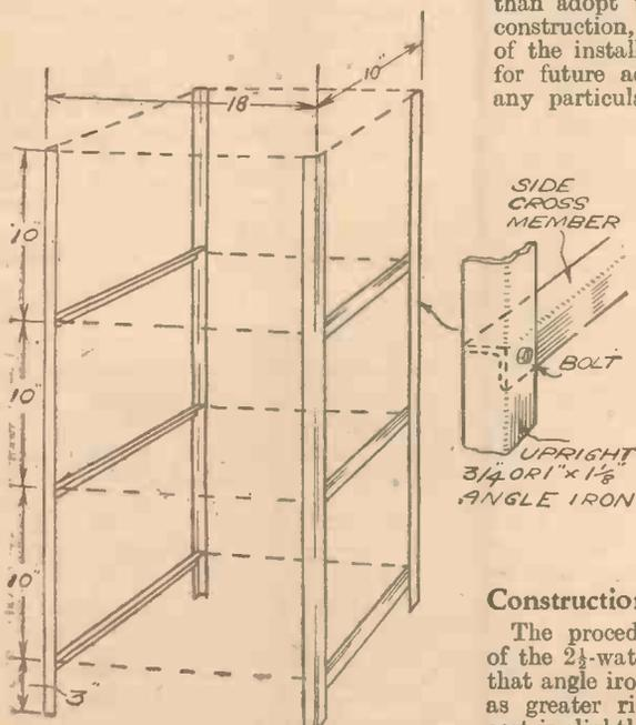
Fig. 1.—Method of building up the rack frame-work for the 10-watt transmitter.
