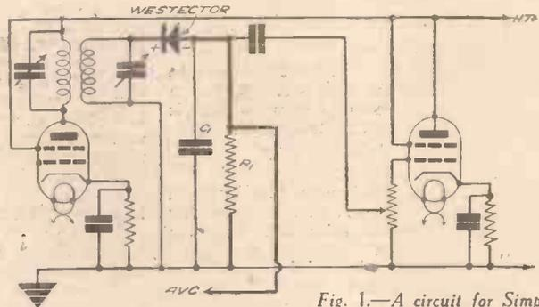
Fig. 1.—A circuit for Simple A.V.C. using a Westector.
