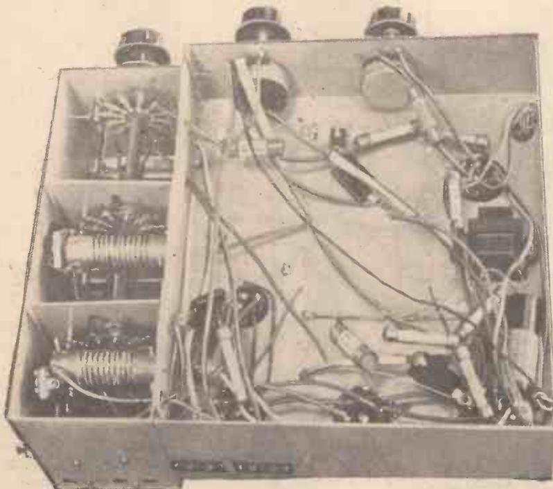
View of the underside of the chassis showing the small amount of wiring which has to be carried out.
