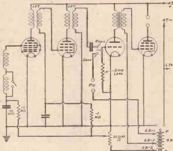
Fig. 1 (left).—The bias circuits of a typical four-valve superhet.
