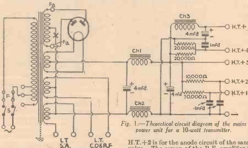
Fig. 1.—Theoretical circuit diagram of the mains power unit for a 10-watt transmitter.
