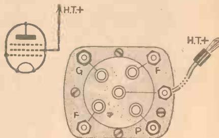
Fig. 3.—This illustration shows the theoretical representation of a pentode valve and how the additional connection is made to the 5-pin valveholder.
