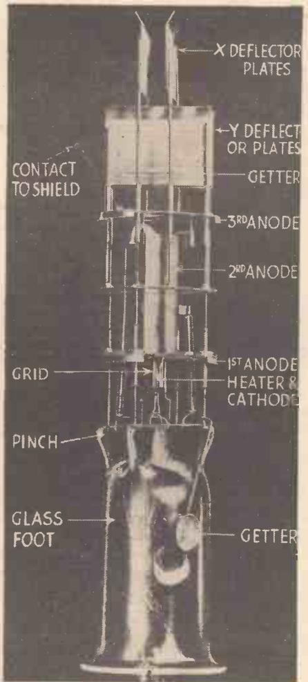
Fig. 2.—A typical electrode assembly for a commercial electrostatically operated C.R. tube for television.
