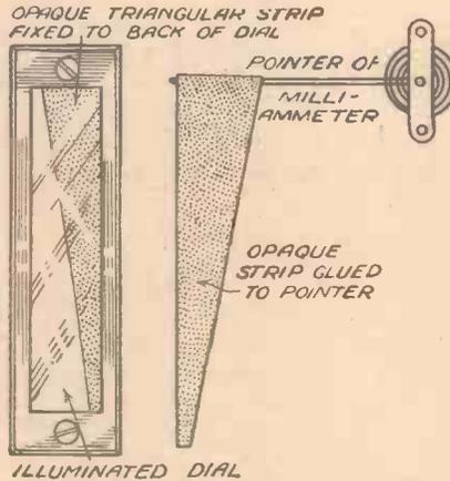
Fig. 4.—Method of arranging for an "eye" or varying angle indicator. If the escutcheon is round, an eye effect will be given.
