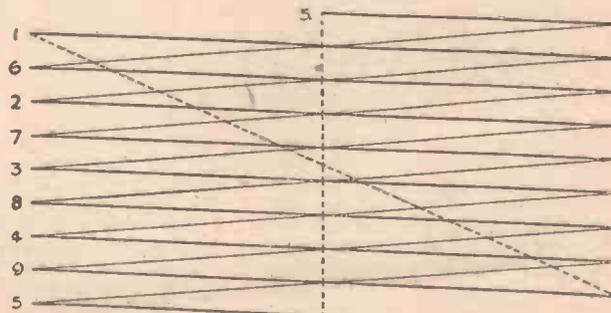
Fig. 2.—How the lines are interlaced to build up the screen in the case of the Marconi-E.M.I. transmissions.
