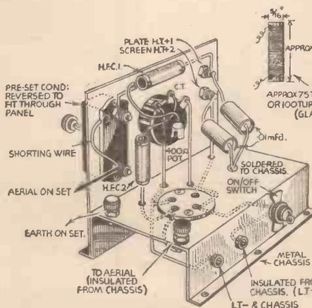
General view and theoretical circuit diagram of a pre-detector H.F. amplifier unit. (Stroud).
