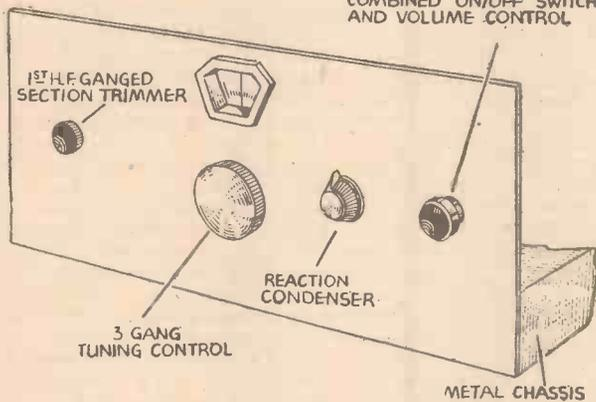
Fig. 3.—When ganged tuning is employed a panel layout on the above lines is recommended.
