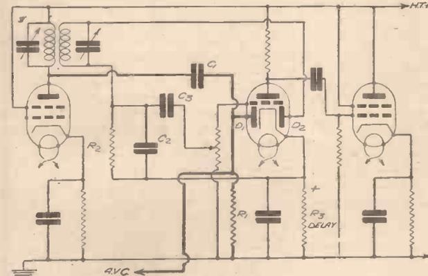
Fig. 4.—A circuit for Delayed A.V.C. using a double-diode-triode valve.
