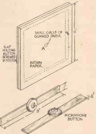
A view of the finished microphone, and details of construction.
