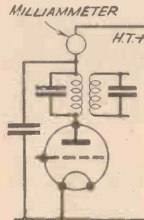
Fig. 3.—Showing the use of a milliammeter as a tuning indicator.
