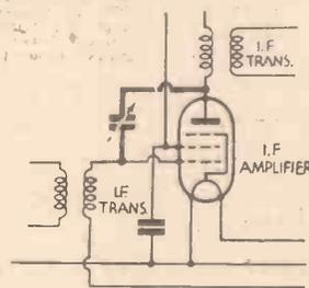
Fig. 2.—Showing a simple method of producing I.F. oscillation for reception of C.W. morse.
