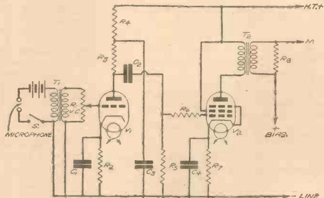
Fig. 3.—The microphone or speech amplifier circuit.
