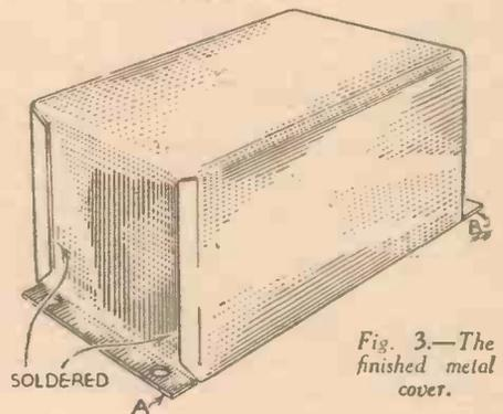
Fig. 3.—The finished metal cover.
