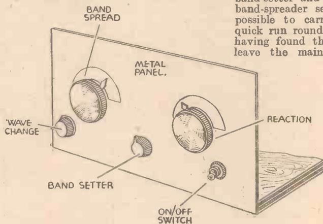
Fig. 1.—A suggested panel and baseboard scheme of construction showing an effective panel layout of controls.
