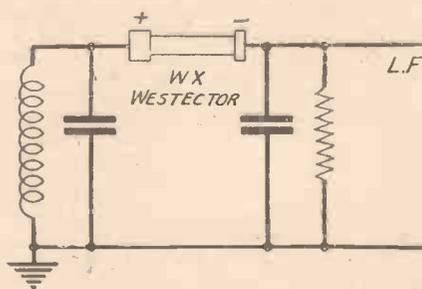
Fig. 5.—Circuit of a detector stage utilizing a Westector.
