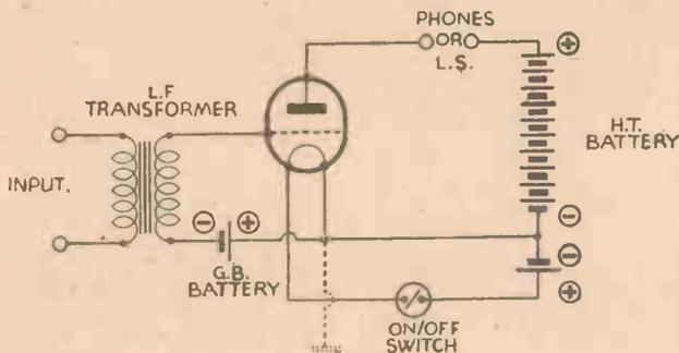
Fig. 1.—Theoretical circuit of the amplifier, with the various components clearly identified.
