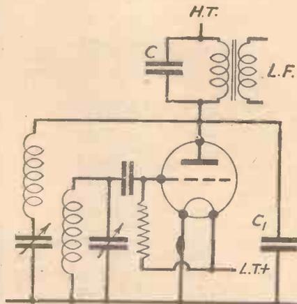
Fig. 3.—The standard leaky-grid detector circuit.
