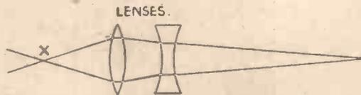
Fig. 3.—A simple lens arrangement for focusing a light beam.
