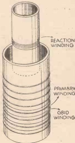
Fig. 1.—An efficient method of winding a short-wave coil.
