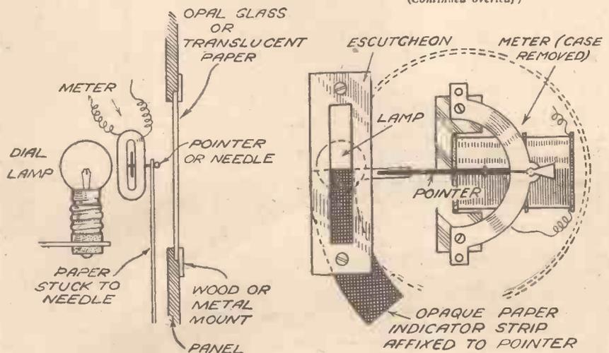
Fig. 3.—Elevation and side view of the method of converting an ordinary milliammeter to give an indication of tuning by light or shadow.
