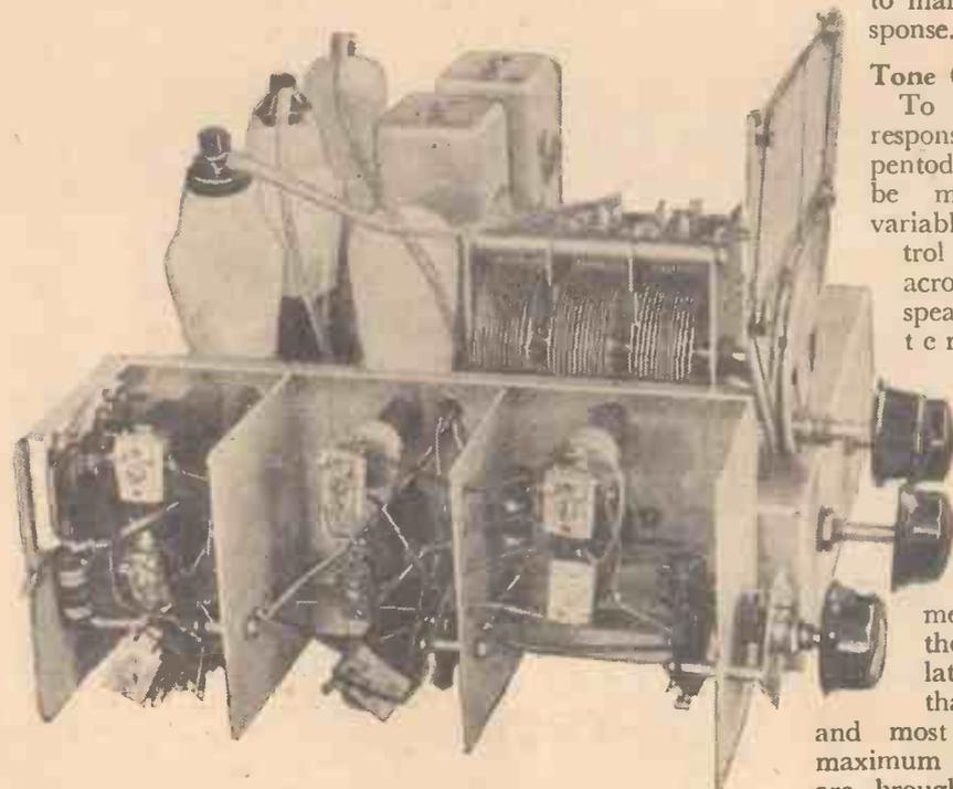
A view of the coil unit with screen removed to show the general arrangement of coils, padding condensers, and switches.
