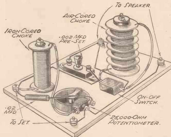
Fig. 2.—Pictorial diagram of the unit, showing how the components are mounted on a plywood panel.
