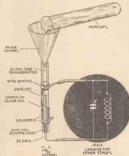
A novel trimming device in which mercury is used for varying the capacity.
