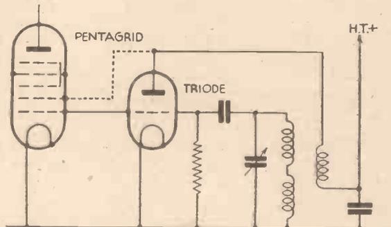
Fig. 3.—Showing the addition of a triode to a pentagrid for improved S.W. reception.
