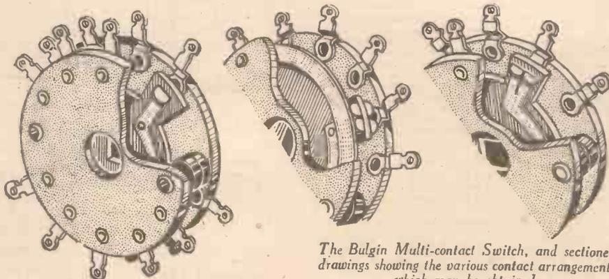
The Bulgin Multi-contact Switch, and sectioned drawings showing the various contact arrangements which may be obtained.
