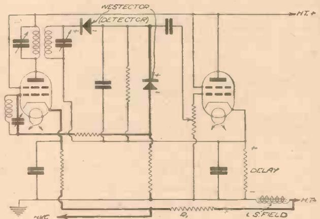
Fig. 5.—(Left) Circuit diagram of Amplified Delayed A.V.C. using a double-diode-triode valve.
