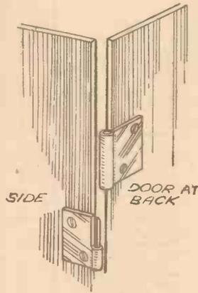
Fig. 2.—Detail showing method of fitting the back of the cabinet.
