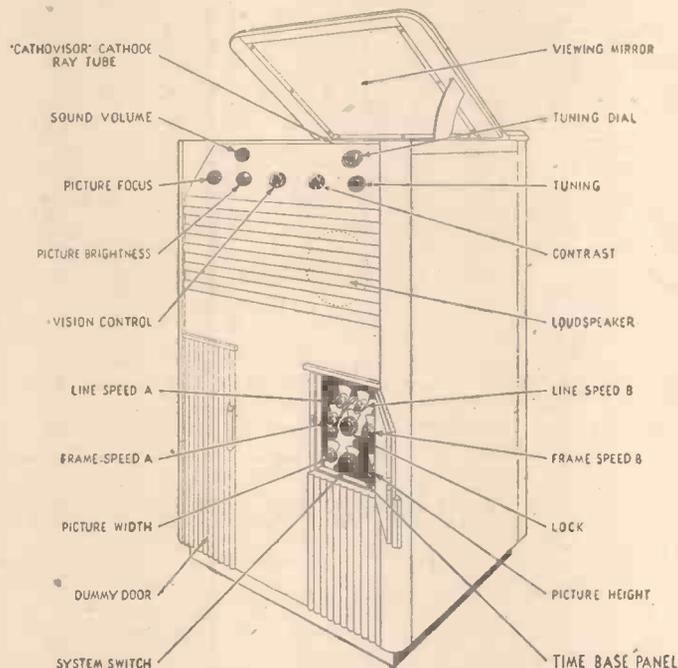
Fig. 1.—A pictorial representation of the controls on a present-day Baird television receiver.
