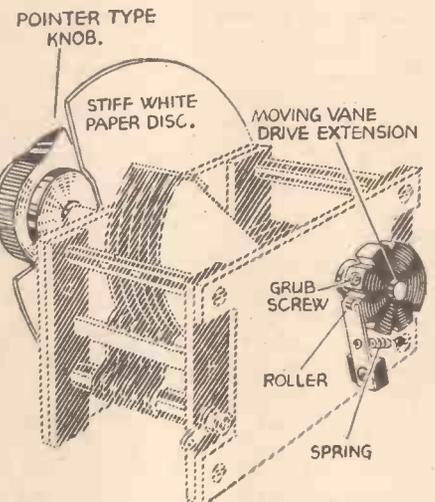
A method of setting a band-spread condenser.
