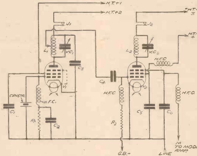
Fig. 4.—The oscillator and power amplifier circuit.
