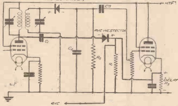
Fig. 2.—(Left) A circuit for Delayed A.V.C. using Westectors.
