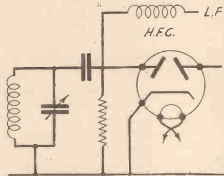
Fig. 4.—The diode detector stage in theoretical form.
