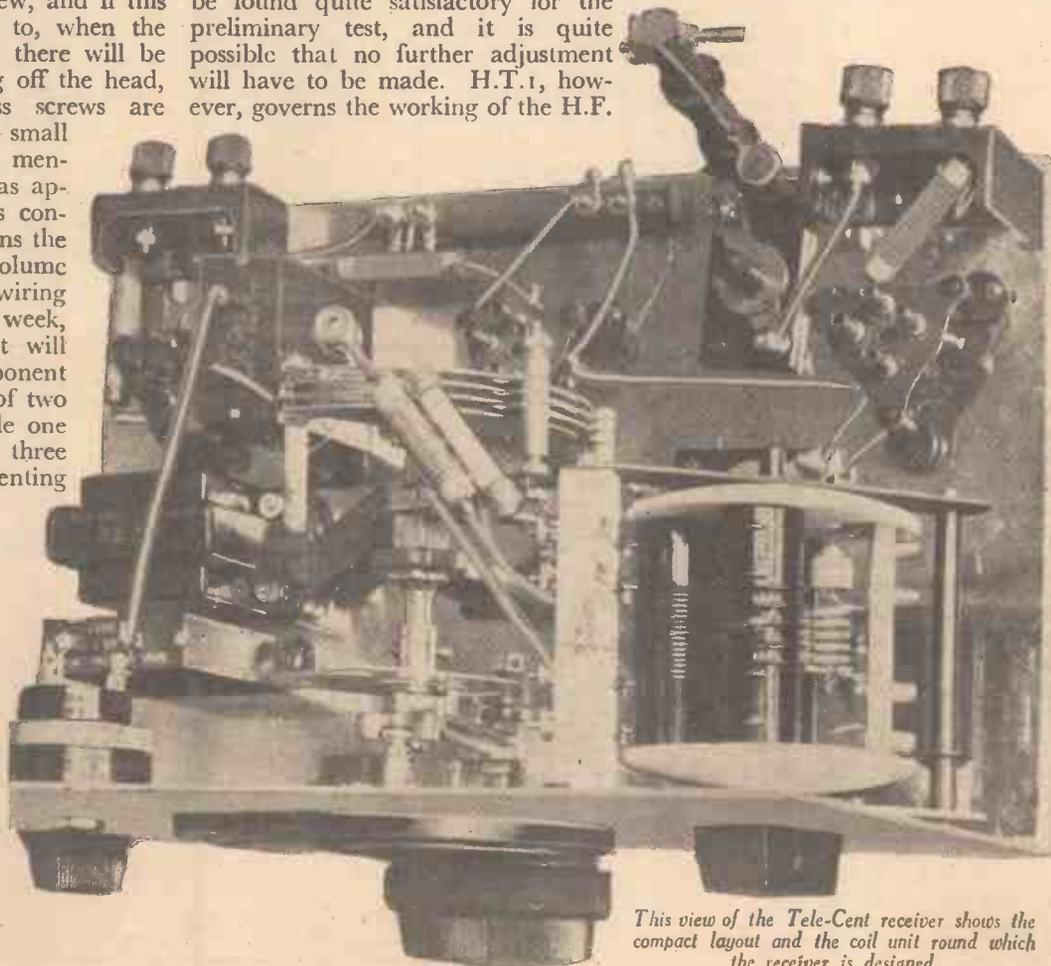
This view of the Tele-Cent receiver shows the compact layout and the coil unit round which the receiver is designed.
