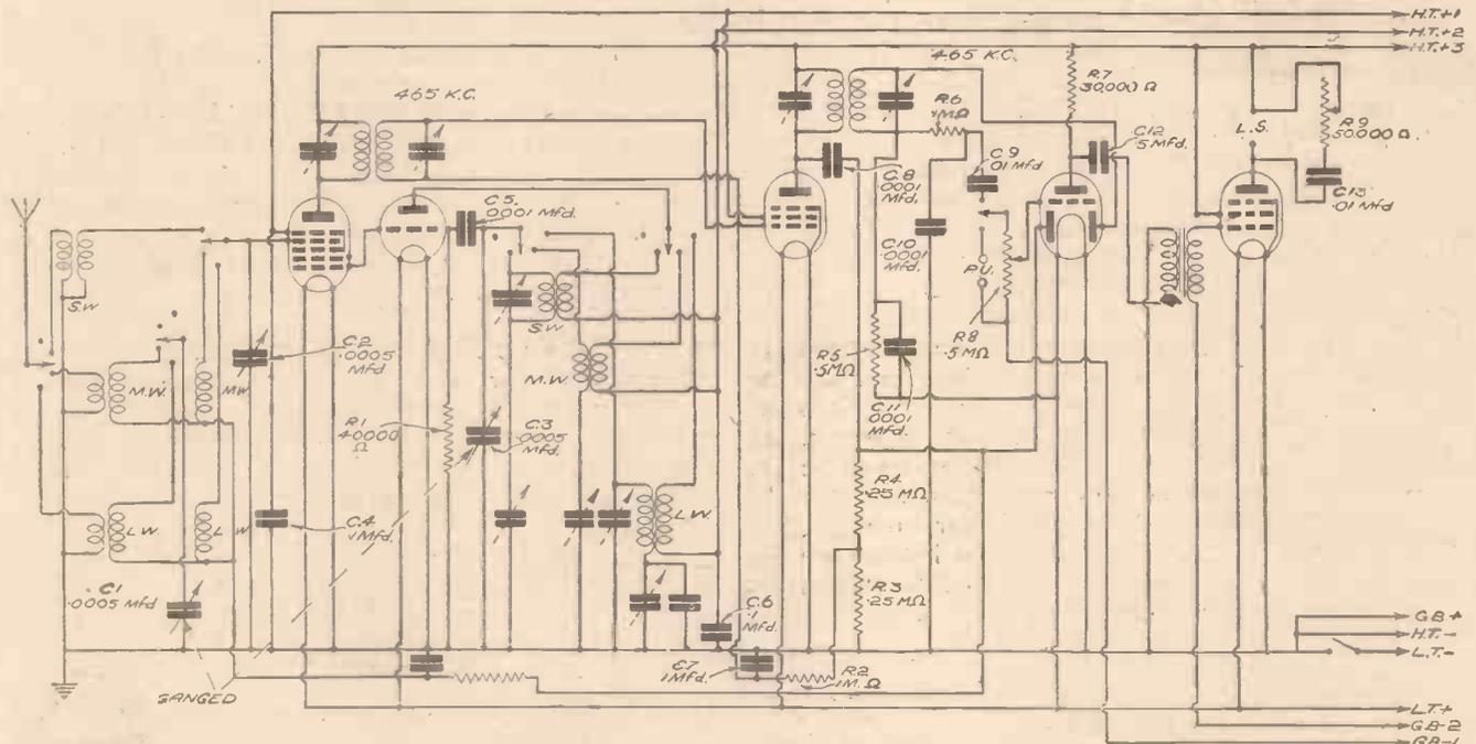
Theoretical Circuit of the "Vitesse" All-waver. It will be noted that certain components do not bear any reference number or value, and these parts are already included in the special coil unit. The make and type numbers of the remaining components may be seen in the list given below.
