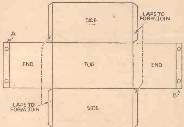
Fig. 2.—Developed blank for making the metal cover for the mains unit.
