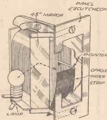
Fig. 1.—(Left) how to modify an "end-type" meter to obtain a "climbing light" or "climbing shadow" effect. Fig. 2 (right) the effect given by the cathode-ray tube indicator, which is shown in a receiver in the illustration below.
