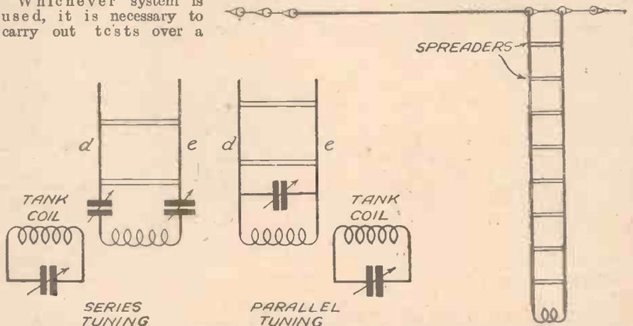
Fig. 2.—Two methods of coupling parallel feeders to the transmitter.
