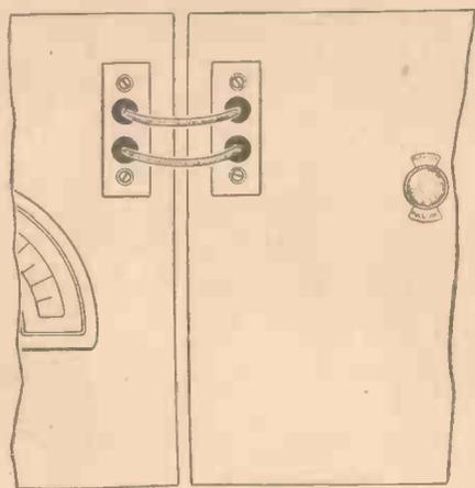
Fig. 4.—How the crystal set and the amplifier are connected together.
