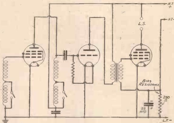
Fig. 3.—This circuit shows how "automatic" bias can be provided for the output valve in a simple three-valve battery circuit.
