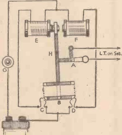
General arrangement and connections for a single-push remote control.
