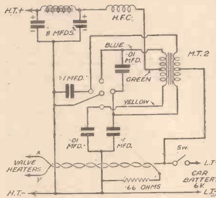
Fig. 3.—Circuit of the H.T. and L.T. unit, using the Bulgin vibratory rectifier and special transformer.
