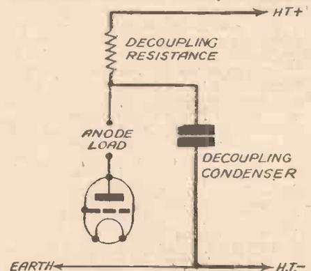
Fig. 1.—This diagram shows how a shorted decoupling condenser will short-circuit the H.T., and probably damage the decoupling resistance.
