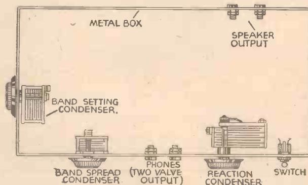
Fig. 2.—A different scheme in which 'phone connections may be easily made, and the tuning circuit is more efficiently wired.
