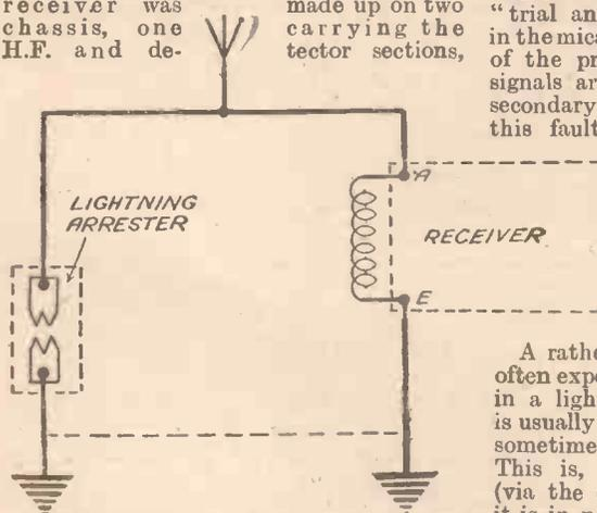
Fig. 2.—How the lightning arrester is included across the aerial coil.
