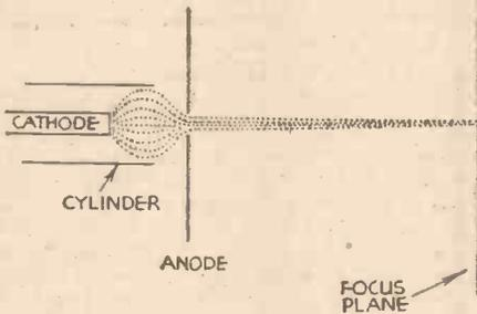
Fig. 1.—Showing the constricting effect produced on the electron stream by the negatively charged cylinder.
