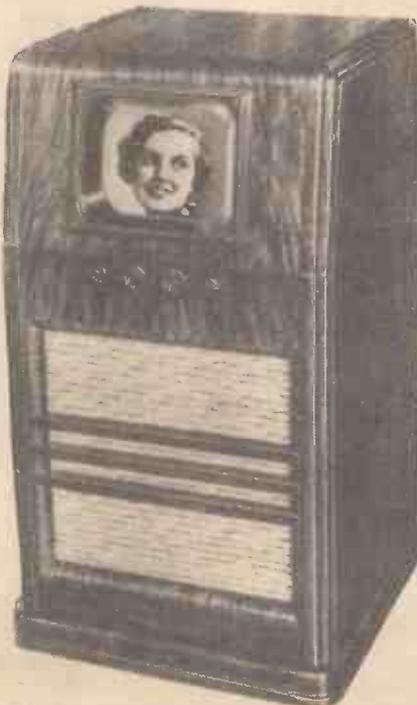
*The new Ultra television receiver which also incorporates an all-wave chassis.*
