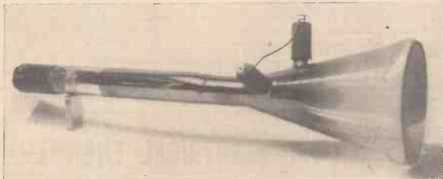
Fig. 1.—An example of the Baird projection tube, as shown at the Science Museum, South Kensington.
