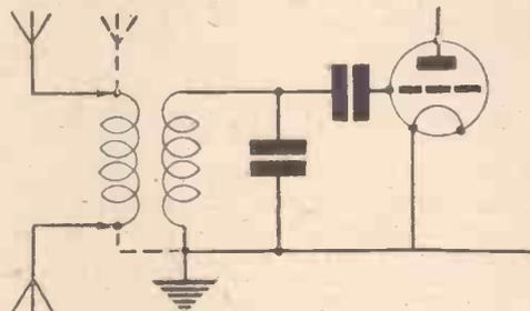
Fig. 2.—When using a four-pin aerial coil, it is often worth while to add a separate aerial winding. This may be connected to a doublet, or to an aerial and earth in the usual manner. If using aerial and earth, as in broken lines, try the effect of reversing the aerial and earth connections.
