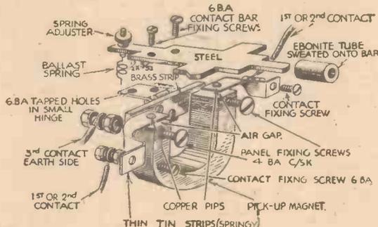
The assembly of parts for making a novel 3-point switch.
