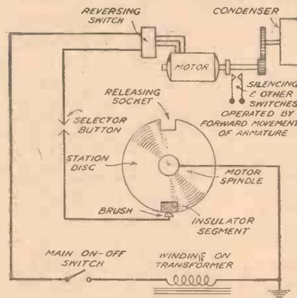
Fig. 4.—One of the American commercial motor-driven pre-selectors is operated as shown here. The disc is repeated for each station required.
