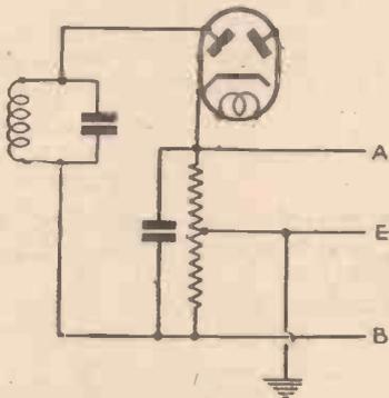
Fig. 19.—Obtaining a split output from a single valve for an R.C. push-pull stage.
