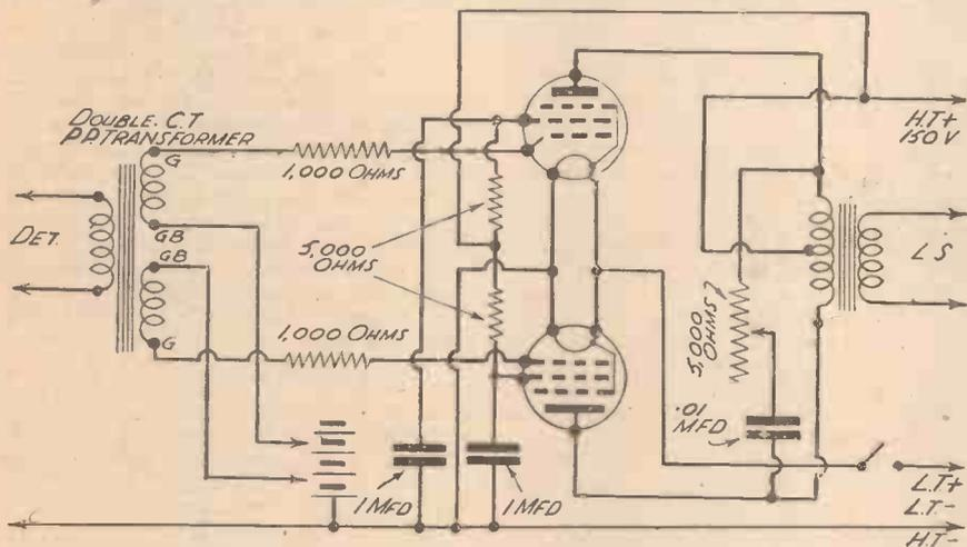
Fig. 1.—A useful type of push-pull amplifier circuit, which is about the best that the builder of a "quality" battery set can adopt.
