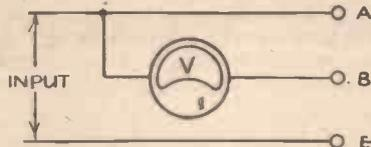
Fig. 20.—Diagram illustrating one method of phase-splitting.
