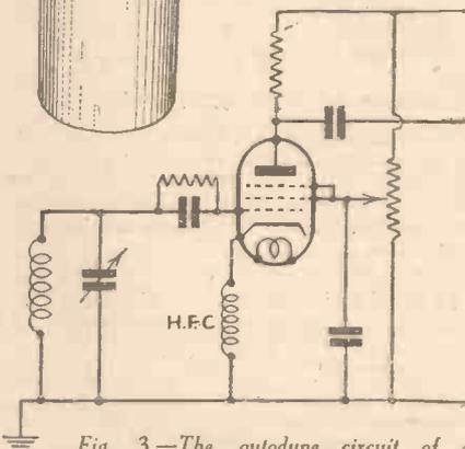
Fig. 3.—The autodyne circuit of a commercial receiver for the ultra-short waveband.
