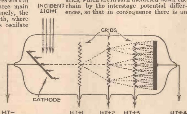
Fig. 1.—Showing the drawing of the cell with the channels indicated by dotted lines.
