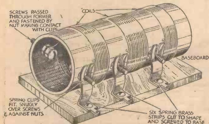
A handy coil mount with spring contact supports.
