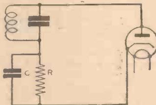
Fig. 27.—This circuit shows the main principles of the mains-operated diode rectifier.
