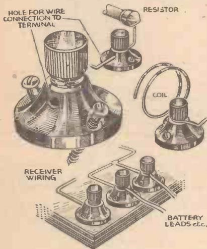
Neat terminal mounts made from old screen-grid valve tops.
