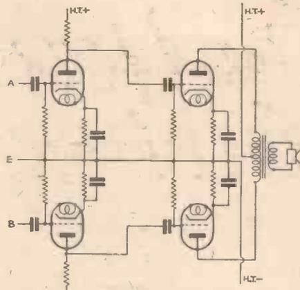
Fig. 17.—Double R.C. push-pull circuit.
