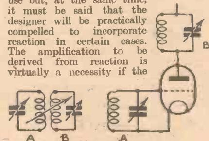
Fig. 35.—Two closed circuits coupled together. Fig. 36.—In this arrangement the only coupling which exists is through the valve.
