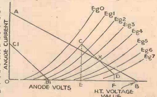
Fig. 16.—The dynamic curves of an amplifying valve.
