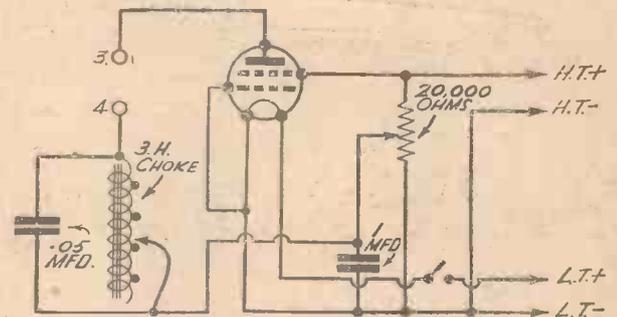
Fig. 6.—A modulated dynatron oscillator, which can be used with the tuner for wavelength checking, or for adjusting the trimmers in a set having ganged tuning condensers.
