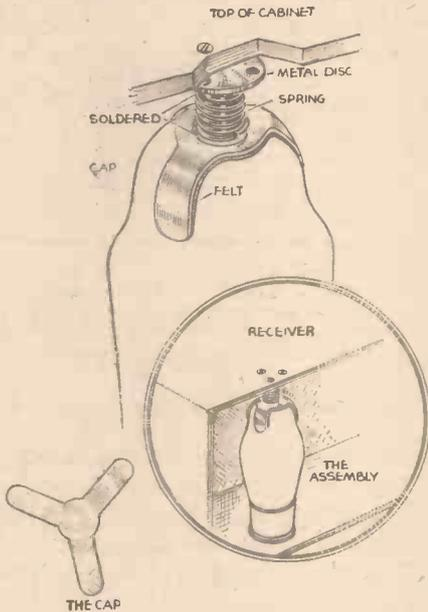
Method of making anti-vibration valveholders.
