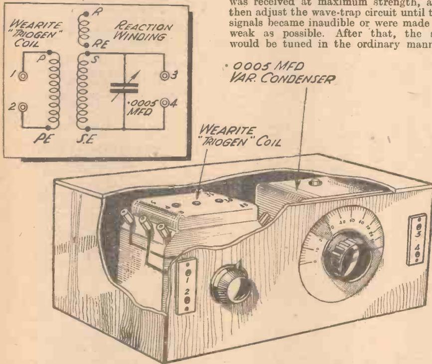
Fig. 1.—Theoretical and practical arrangements of the three-range tuning circuit. A Wearite "Triogen" coil is shown, but wave-change-switch connections are omitted for simplicity.
