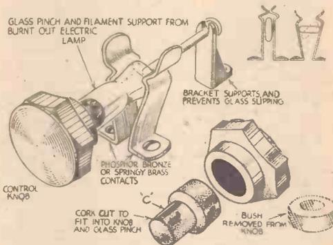
Details of a simple low-loss switch.
