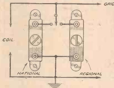
Fig. 1.—The basis of automatic tuners—pre-set condensers, each tuned to a different station and brought into circuit by a switch.
