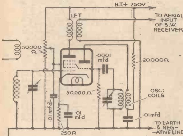
Fig. 1.—Theoretical circuit diagram of an ultra-short-wave converter using a triode-hexode.
