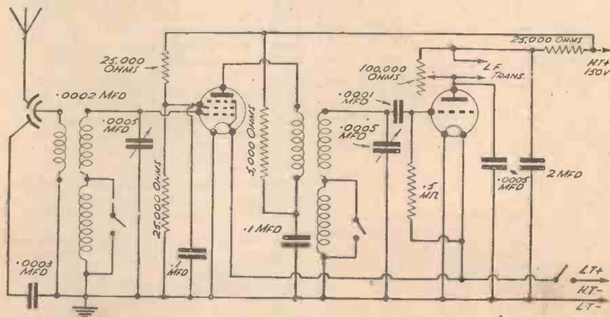
Fig. 2.—This simple H.F.-detector circuit cannot well be bettered for local station reception.
