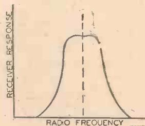
Fig. 30.—How the band-pass tuner approaches the ideal shown in Fig. 29.
