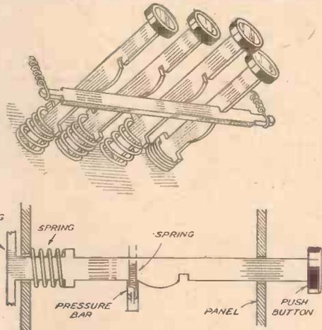
Fig. 3.—How you can build a push-button tuner—with a detailed illustration of the separate push rods.
