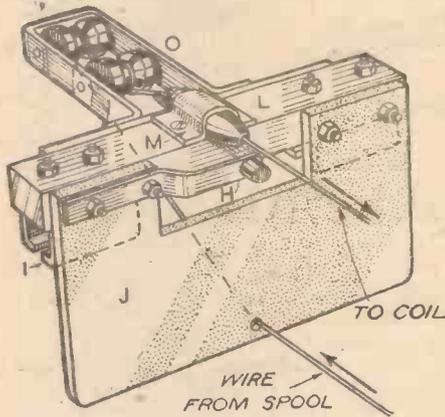
Fig. 3.—This diagram shows how the wire is fed to the coil.
