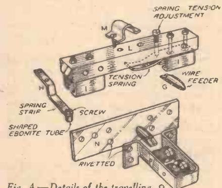
Fig. 4.—Details of the travelling shuttle and wire guide.
