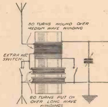
Fig. 7.—How a normal two-range coil, without separate aerial winding, can be modified for use with a doublet.
