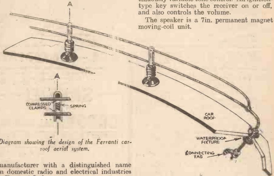
Diagram showing the design of the Ferranti car-roof aerial system.
