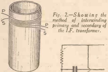
Fig. 2.—Showing the method of interwinding primary and secondary of the I.F. transformer.
