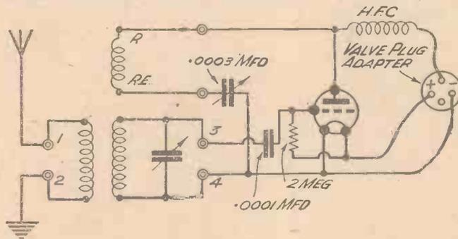
Fig. 5.—A three-range adapter circuit, incorporating the tuning unit described.
