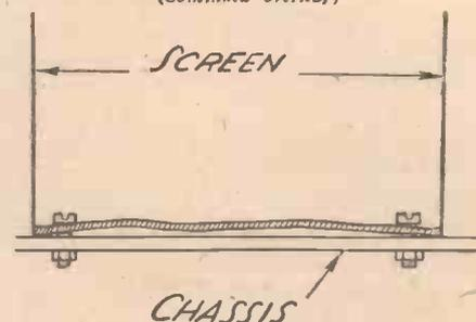
Fig. 3.—How a badly-made screen may cause trouble due to poor workmanship.
