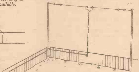
Fig. 2.—How a doublet can sometimes be erected between two masts at the end of the garden so that it is well away from the source of interference. In this case the aeriels' span can rarely be more than 33ft. each, the total length of the lead-in being 66ft.
