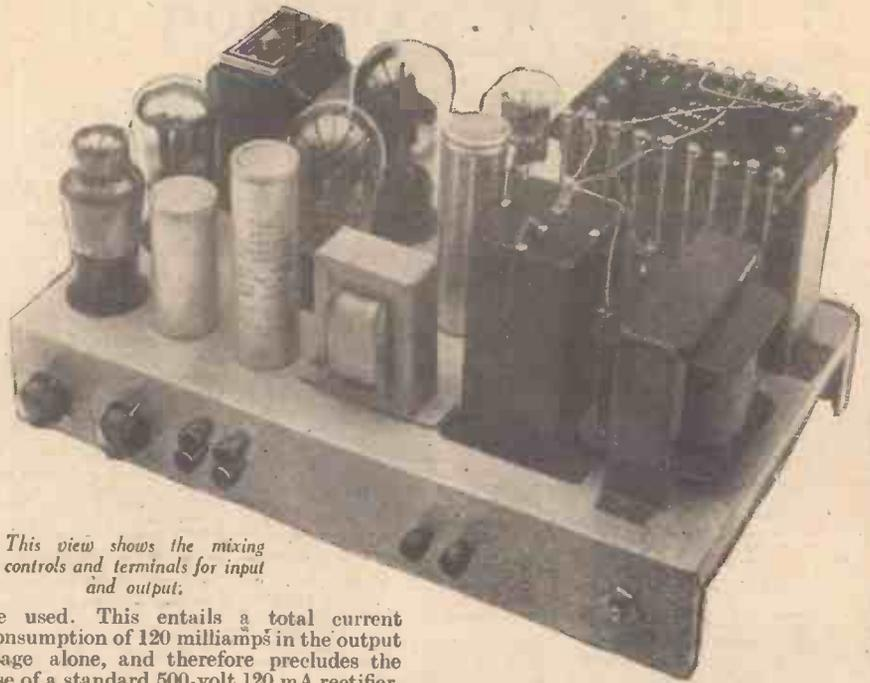
This view shows the mixing controls and terminals for input and output.
