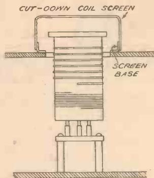
Fig. 7.—General arrangement of the coil screen shown at G, Fig. 6.
