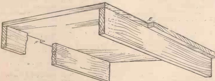
Fig. 4.—Showing how the chassis face is stepped back to accommodate the ends of the brackets.
