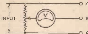
Fig. 21.—Reducing input by potentiometer control.
