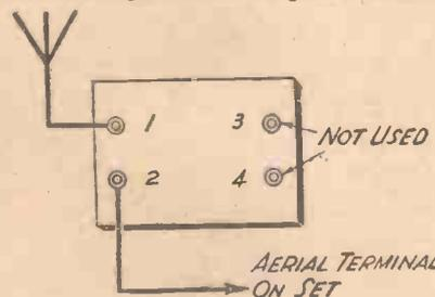
Fig. 2.—How the tuning unit can be used as a series wave-trap, by connecting it between the aerial down-lead and the aerial terminal on the set.
