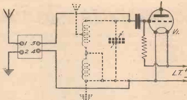
Fig 4.—How a tuner in an existing set can be checked by connecting the tuning unit in its place.
