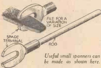
Useful small spanners can be made as shown here.
