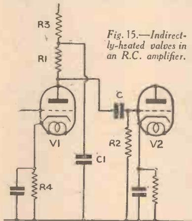
Fig. 15.—Indirectly-heated valves in an R.C. amplifier.
