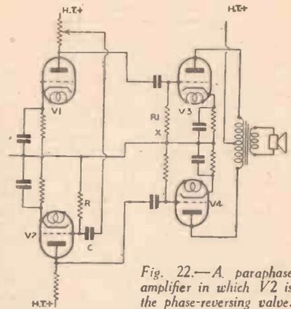
Fig. 22.—A paraphase amplifier in which V2 is the phase-reversing valve.
