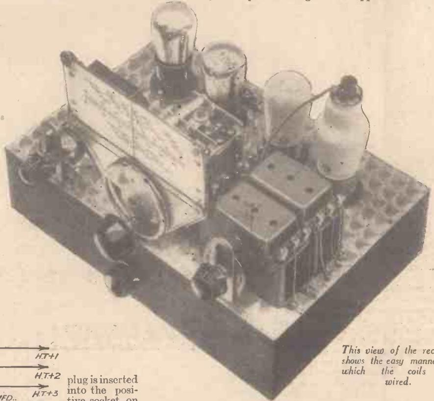
This view of the receiver shows the easy manner in which the coils are wired.
