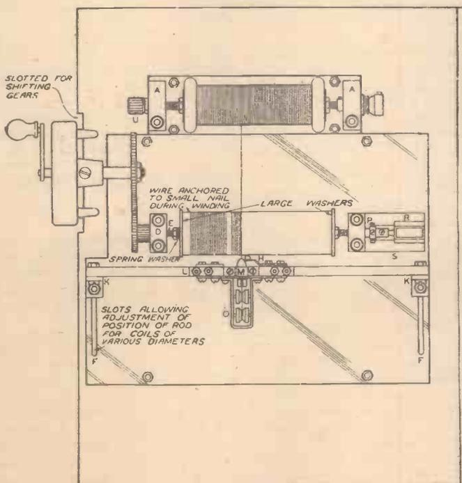
Fig. 2.—Plan showing the main details of the winder.
