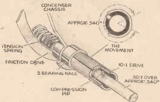
This is the ingenious driving mechanism fitted to the new Polar horizontal drive, which will be found ideal for receivers employing all-wave tuning circuits.
