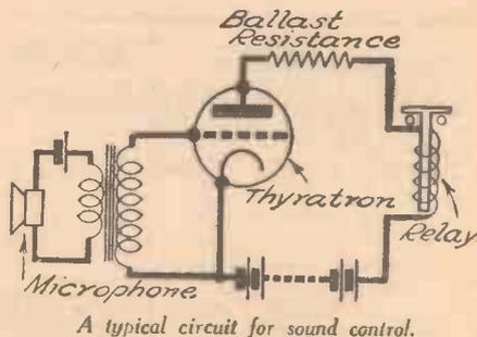
A typical circuit for sound control.
