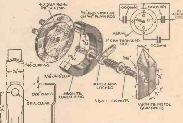
Constructional details of an aerial-selectivity switch made from a chassis-mounting valve holder.
