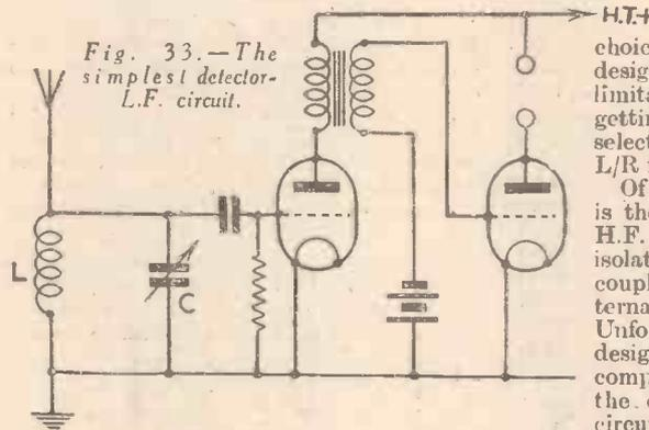
Fig. 33.—The simplest detector-L.F. circuit.
