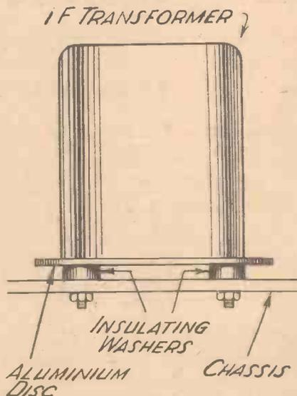
Fig. 5.—How an I.F. transformer may have to be separately screened.
