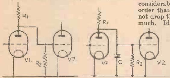
Figs. 12 and 13.—R.C. coupling showing the stray capacity (C1).
