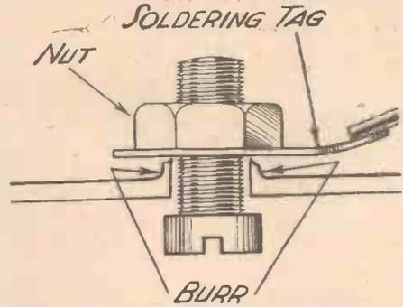
Fig. 4.—Leave the burr caused by the drill to assist in making good contact.
