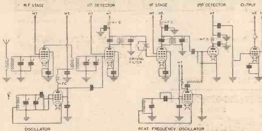
Fig. 1.—The theoretical circuit in outline. The H.T. positive points will be joined to the H.T. output through decoupling components.
