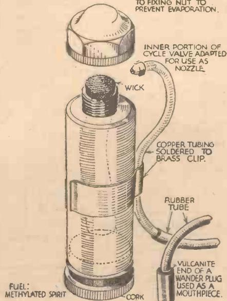
A small blow-lamp making use of a disused electrolytic condenser casing for the spirit reservoir.
