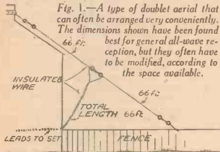
Fig. 1.—A type of doublet aerial that can often be arranged very conveniently. The dimensions shown have been found best for general all-wave reception, but they often have to be modified, according to the space available.
