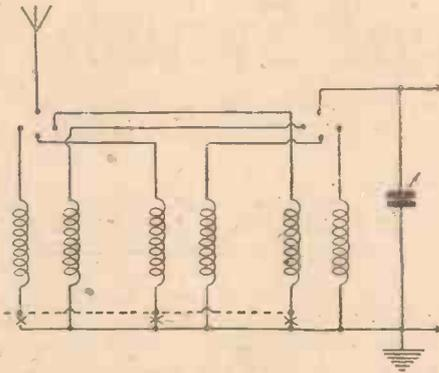
Fig. 6.—In some all-wave coils having separate aerial windings one end of each of these is joined to a common earth terminal. In that case a doublet can be used by breaking the leads marked X and connecting them together, as indicated by the broken line, and to earth.
