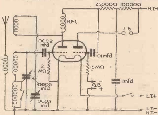
Fig. 1.—A simple type of circuit in which a class B valve is used for detection and L.F. amplification.
