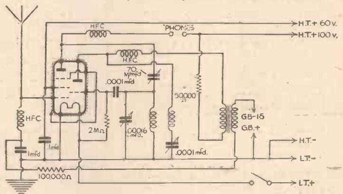
Fig. 3.—An interesting circuit sent in by a reader. A triode-pentode acts as H.F., Det., and L.F.
