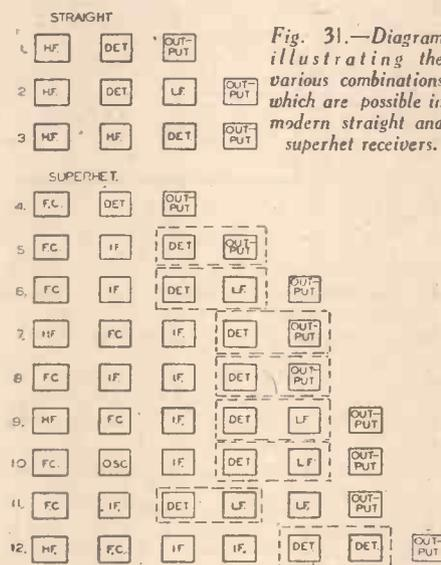
Fig. 31.—Diagram illustrating the various combinations which are possible in modern straight and superhet receivers.
