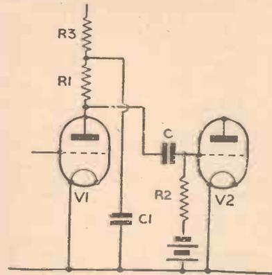
Fig. 14.—The full resistance-capacity circuit with decoupling components added.
