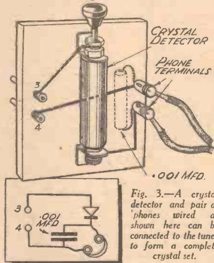
Fig. 3.—A crystal detector and pair of 'phones wired as shown here can be connected to the tuner to form a complete crystal set.
