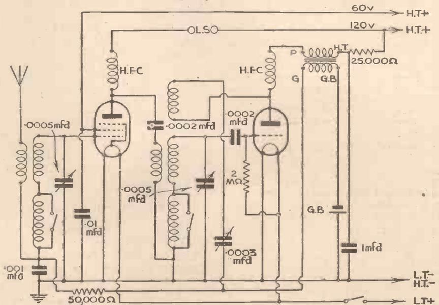
Fig. 2.—This is a reflex arrangement where the H.F. pentode is also used for low-frequency amplification.
