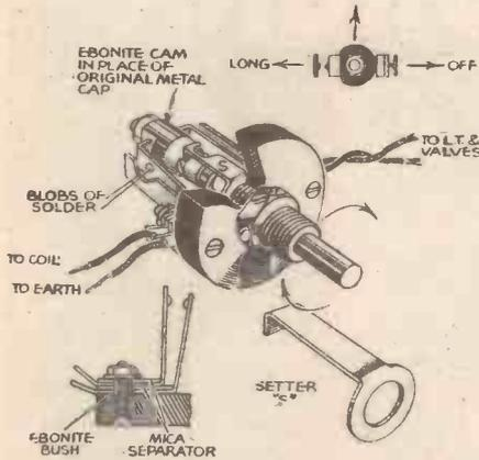
A method of converting a push-pull switch.
