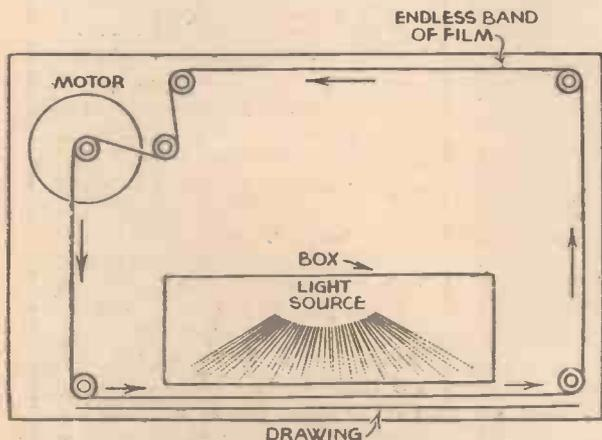
Fig. 2.—(left) A plan view of the model showing the endless band of film.
