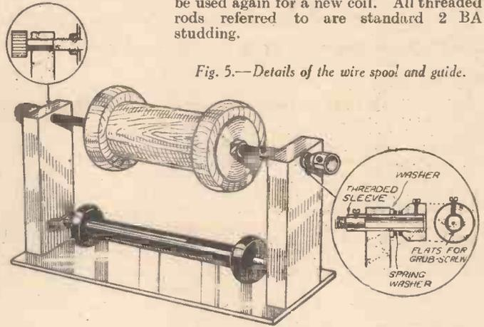
Fig. 5.—Details of the wire spool and guide.
