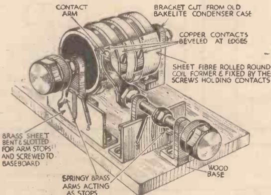
A switch for controlling wave-trap, and other inductances.
