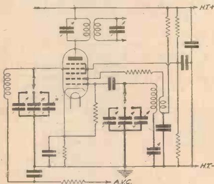
Fig. 2.—A modern superhet may be operated by selector switches by a similar arrangement to that shown here.
