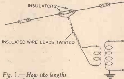
Fig. 1.—How two lengths of insulated wire are used to form a doublet aerial; also, how the aerial is connected to a separate winding on the tuning coil.
