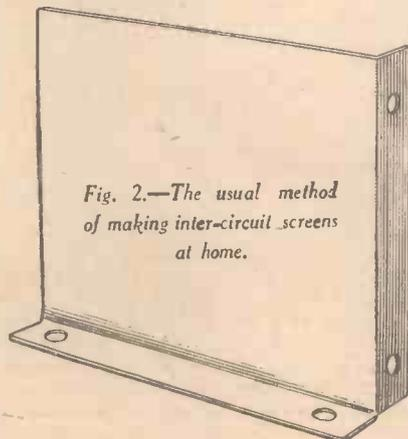
Fig. 2.—The usual method of making inter-circuit screens at home.
