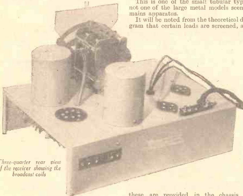
Three-quarter rear view of the receiver showing the broadcast coils
