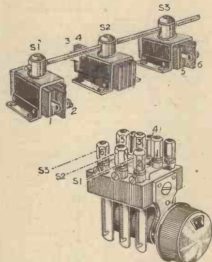
Fig. 5.—Two transmit-receive switch arrangements. The terminal numbers correspond with those in Fig. 4.
