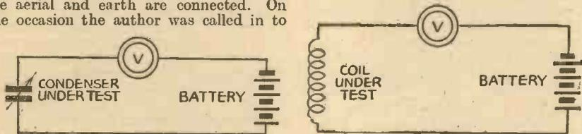
Figs. 4 and 5.—Circuit diagrams for testing a condenser, and a coil, respectively.
