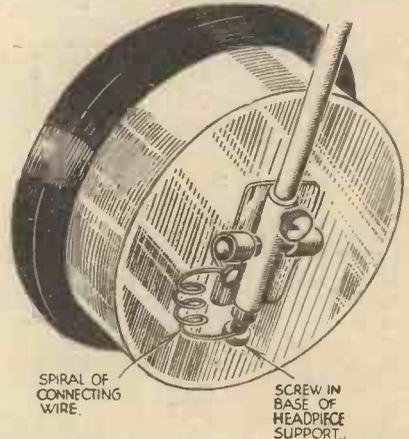
A method of preventing cracking in headphones.
