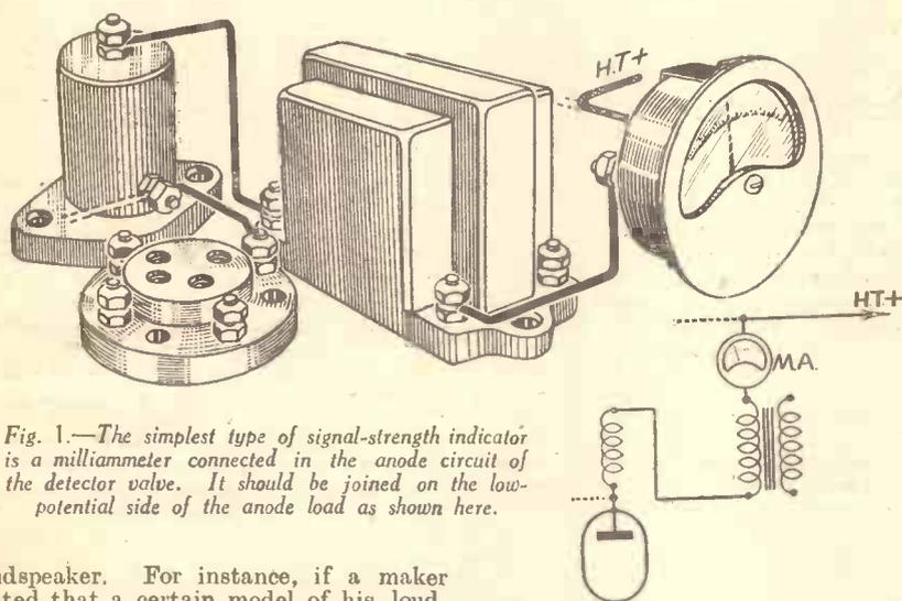
Fig. 1.—The simplest type of signal-strength indicator is a milliammeter connected in the anode circuit of the detector valve. It should be joined on the low-potential side of the anode load as shown here.
