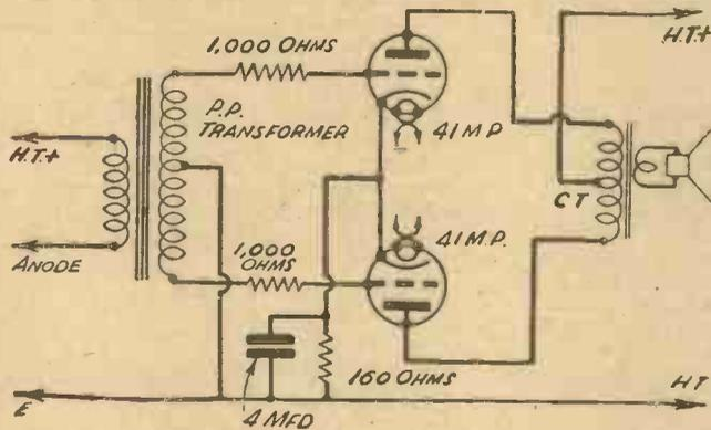
Fig. 1.—Skeleton circuit of a push-pull amplifier using two Cossor 41 M.P. indirectly-heated power valves.
