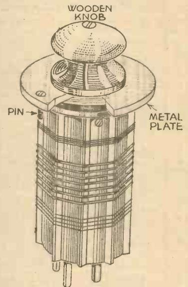
Fig. 2.—A simple plug-in device to ensure easy registration of pins and sockets.
