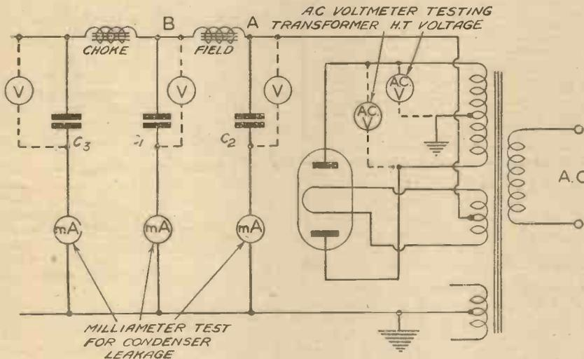
Fig. 16.—Testing a valve rectifier and its smoothing circuit.
