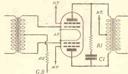
Fig. 15.—Circuit diagram of a Q.P.P. output stage. Note the stabilising resistance R2 and tone correcting circuit R1 and C1.
