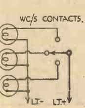
this purpose, fitting over the ebonite caps snugly. The fitment is wired to the wave-change switch contacts as shown in the theoretical circuit drawing. The holes to be drilled for the bulb holders should be
