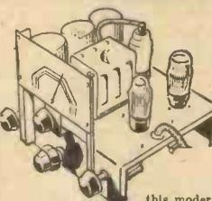
Wavelengths 14-31, 28-62, 200-550, 900-2100 metres. Illustrated on the left is the assembled Peto-Scott All-Wave S.G.3 Kit. Efficiency, economy and simplicity of construction and operation are the keynotes of this modern to-the-minute circuit.
