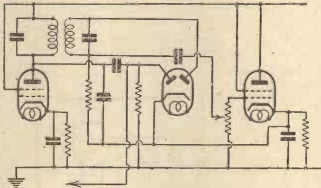
Fig. 8.—The A.V.C. circuit of a superhet receiver which may be tested as described in this article.
