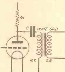
Fig. 11.—Parallel-fed transformer coupling.
