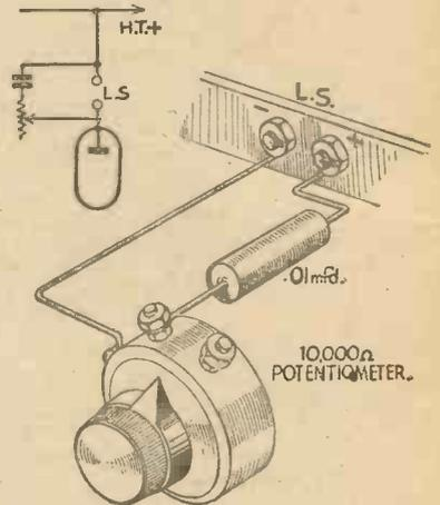
Fig. 2.—A tone control will generally be found advisable with a pentode output valve, a .01-mfd. fixed condenser and a 10,000-ohm volume control being used for the purpose. They are joined across the L.S. terminals, as shown here.
