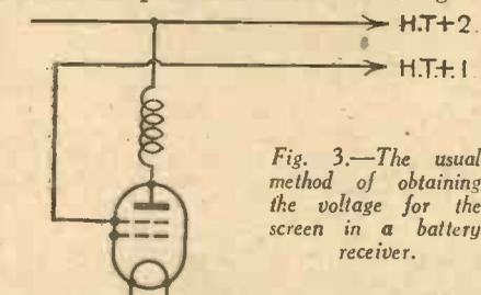
Fig. 3.—The usual method of obtaining the voltage for the screen in a battery receiver.
