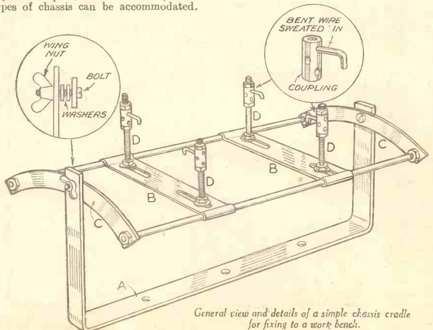
General view and details of a simple chassis cradle for fixing to a work bench.
