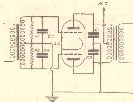
Fig. 14.—Class B output stage, showing the inclusion of condensers and resistances to counteract instability and oscillation.
