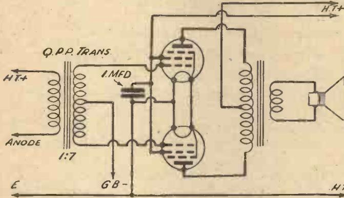
Fig. 4.—This diagrammatic circuit is for two pentodes in Q.P.P.
