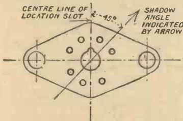
This diagram shows the relative shadow area of the G.E.C. Tuning Indicator in relation to the pin positions.
