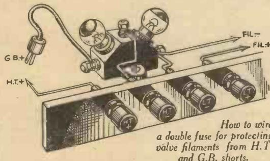
How to wire a double fuse for protecting valve filaments from H.T. and G.B. shorts.
