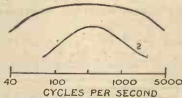
Fig. 3.—Showing what happens to speaker response when frequency range is restricted.
