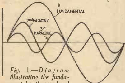
Fig. 1.—Diagram illustrating the fundamental with second and third harmonics.
