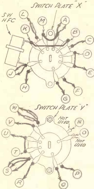
This diagram shows the wiring points on the two switch units, viewed from the rear of the chassis.
