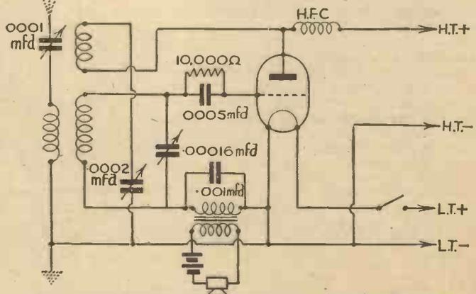
Fig. 3.—The similarity between this simple transmitting circuit and the receiving circuit shown in Fig. 1 is obvious. Aerial and earth are shown broken because these will be replaced by a "dummy" aerial when a full transmitting licence is not held.
