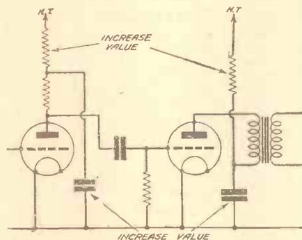
Fig. 12.—Showing how to increase decoupling efficiency.
