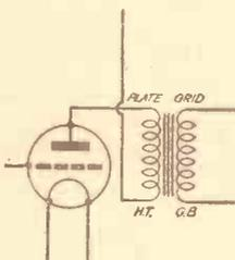
Fig. 10.—Transformer coupling.
