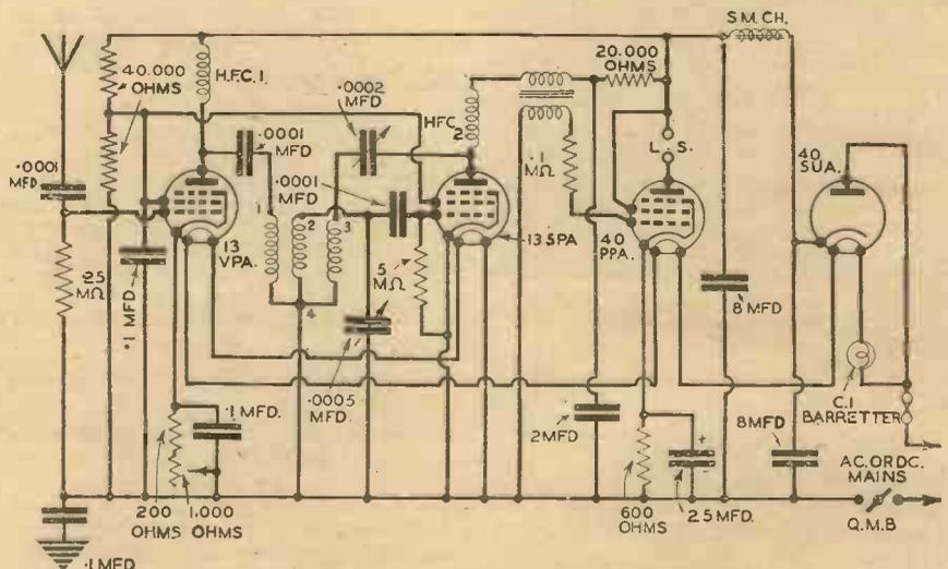
Fig. 2.—Here is an "all-mains" S.W. receiver in which an aperiodic H.F. stage is employed.
