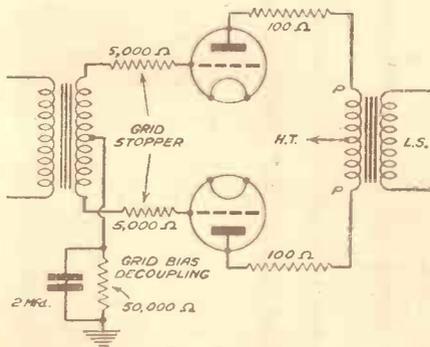
Fig. 13.—Circuit diagram of a push-pull output stage.
