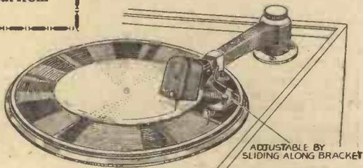
General view and details of construction of a home-made tracking device.
