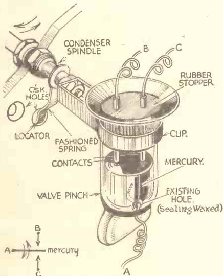
A simple two-way mercury-operated tip-switch.
