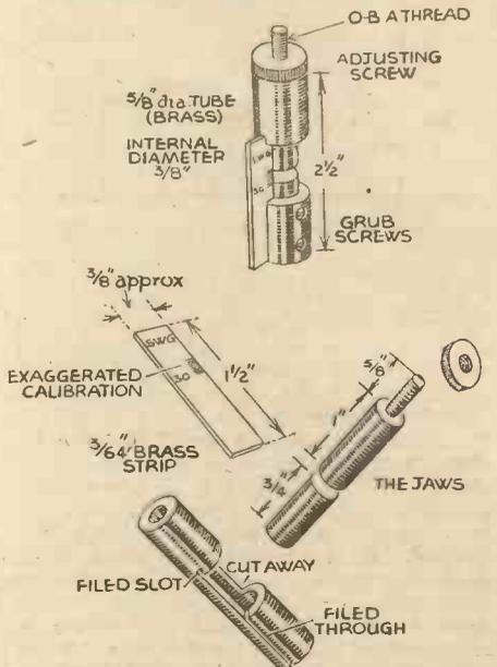
A simple wire gauge, and details of construction.
