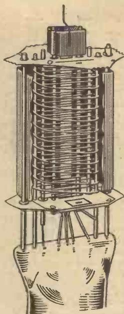
Fig. 4.—An indirectly heated pentode, the Cossor 402 Pen; the relatively close spacing of all three grids can be clearly seen. Observe the open nature of the suppressor grid and also the box cooling fin at the end of the grid supports to assist in cooling them.
