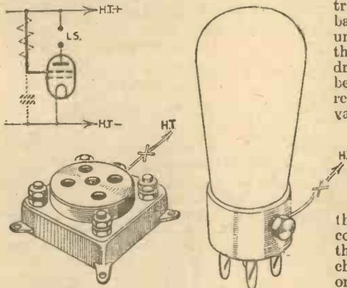
Fig. 1.—An output triode may be replaced by a pentode or tetrode as shown here. In some cases it may be preferable to include a resistance in the additional H.T. lead as shown in broken lines and by the "X" in the above sketch, joining a 2-mfd. condenser to earth, as shown.
