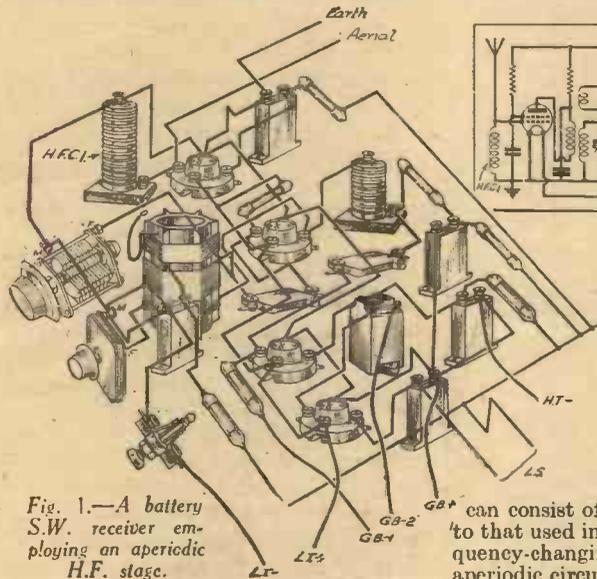
Fig. 1.—A battery S.W. receiver employing an aperiodic H.F. stage.
