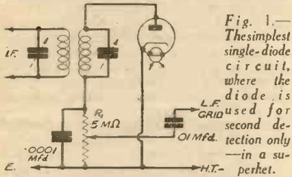
Fig. 1.—The simplest single-diode circuit, where the diode is used for second detection only—in a superhet.
