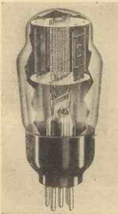
Fig. 1.—A modern high-slope output valve—the Cossor 42 OT. Note the close grid spacing which with the 2-watt heater gives the high slope of 7 mA/V.
