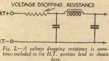
Fig. 2.—A voltage dropping resistance is sometimes included in the H.T. positive lead as shown here.
