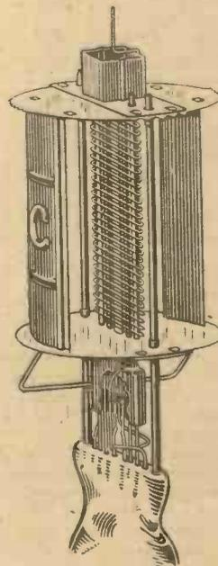
Fig. 3.—A well-designed output tetrode, the *Cossor 42 OTDD*; note the close spacing of cathode, control grid and screening grid, and the remote position of the anode.
