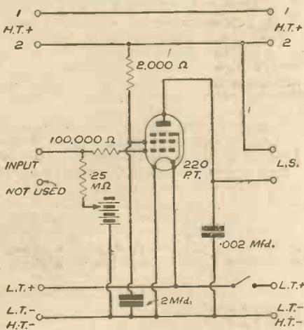
Fig. 1.—Circuit for a resistance-coupled pentode amplifier.
