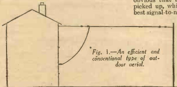
Fig. 1.—An efficient and conventional type of outdoor aerial.
