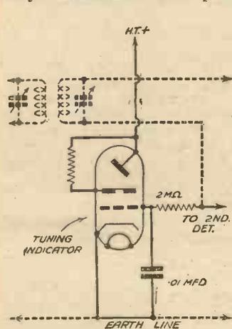
Connections for the Osram visual tuning indicator.
