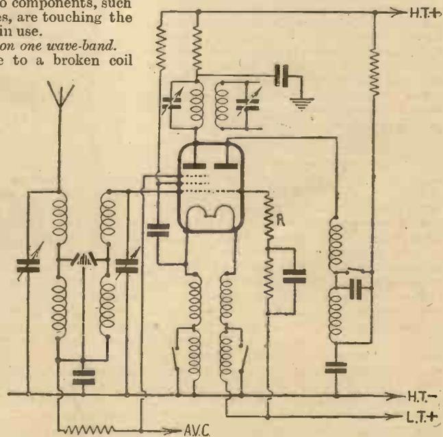
Fig. 6.—Circuit diagram incorporating a battery triode-pentode frequency changer (Mazda T.P.22).
