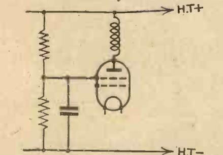
Fig. 4.—How to obtain the screen voltage by means of a potentiometer.
