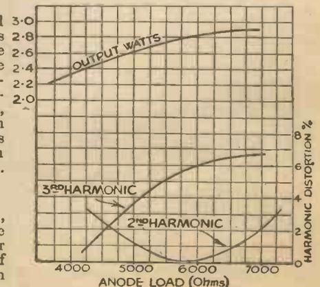
Fig. 2.—This curve shows the relationship between optimum load and harmonic distortion, and also the relationship between optimum load and power output.
