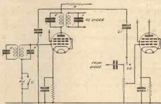
Fig. 73.—It is possible to use an I.F. valve for the first L.F. stage in the circuit as shown here.
