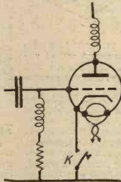
Fig. 5 (Above).—Cathode and filament keying for mains valves.
