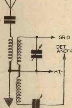
Fig. 9.—How reaction connections are made when all three windings are internally joined together. Heavy lines show the connections that are made inside the coil.
