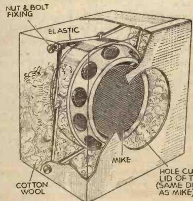
An effective method of mounting a microphone to avoid "boom" effects.
