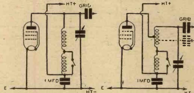
Fig. 3.—Tuned-anode coupling, using tapped and untapped dual-range coil.
