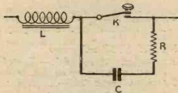
Fig. 4.—A simple form of filter to prevent keying clicks.
