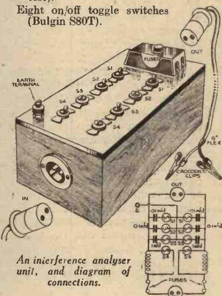
An interference analyser unit, and diagram of connections.
