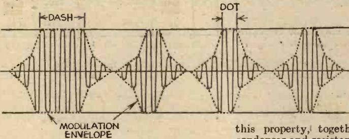
Fig. 1.—Showing the new formation of the wave-train when key is operated for letter "B."
