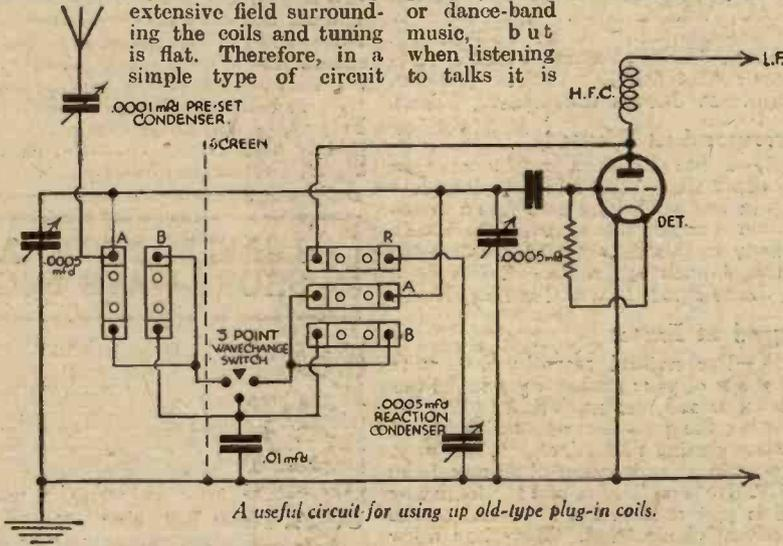
A useful circuit for using up old-type plug-in coils.
