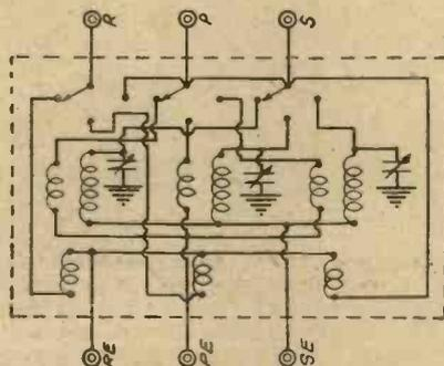
Fig. 2.—The circuit which is employed in the Wearite all-wave tuner.
