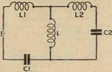
Fig. 11.—Two coupled circuits with a common inductance.
