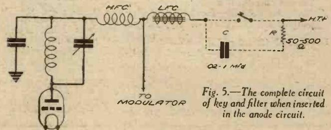
Fig. 5.—The complete circuit of key and filter when inserted in the anode circuit.
