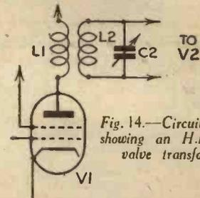
Fig. 14.—Circuit diagram showing an H.F. intervalve transformer.
