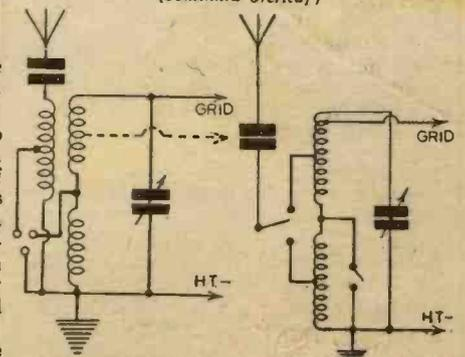
Fig. 5.—How both aerial and grid winding can be tapped, a section of each being short-circuited for medium-wave reception.
