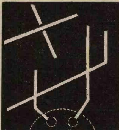
Fig. 1.—Wires which cross without touching are always indicated by one of the schemes shown above.
