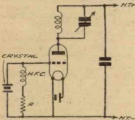
Fig. 1.—A simple triode crystal-controlled oscillator.
