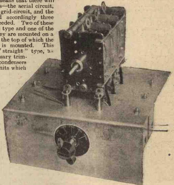
Fig. 1.—The complete tuner ready for insertion in a receiver.
