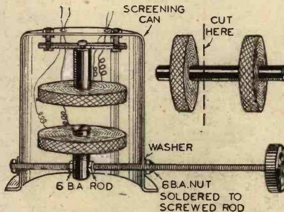
Fig. 1.—Details of a variable coupling I.F. transformer, arranged so that one coil can be rotated through an angle of 90 degrees.
