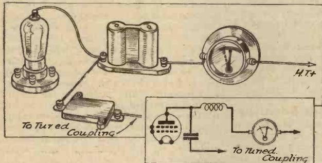
When using a milliammeter in an anode circuit it should be on the earth side of the anode load.
