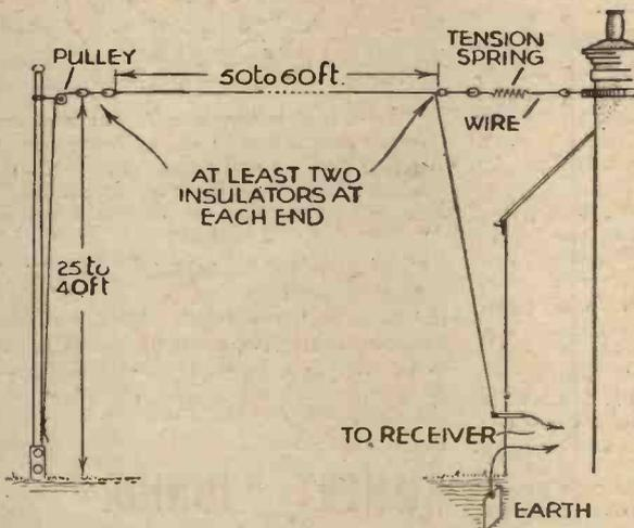
Fig. 2.—An ideal arrangement for an inverted "L" type of aerial.
