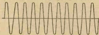
Fig. 3.—Graphical representation of continuous oscillations.
