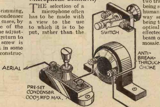
How to include an anti-breakthrough choke in the aerial circuit, with a switch to short-circuit it when not needed.
