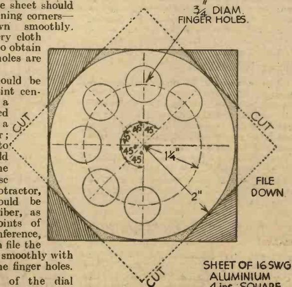
Fig. 4.—How to mark out and cut the dial.
