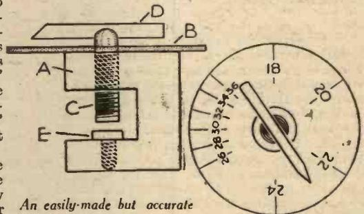
An easily-made but accurate wire gauge.
