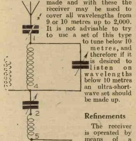
Fig. 3.—How a 4-pin coil may be used.
