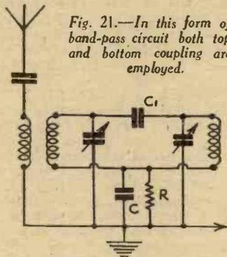
Fig. 21.—In this form of band-pass circuit both top and bottom coupling are employed.
