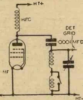
Fig. 1.—Simplest arrangement of tuned-grid coupling.
