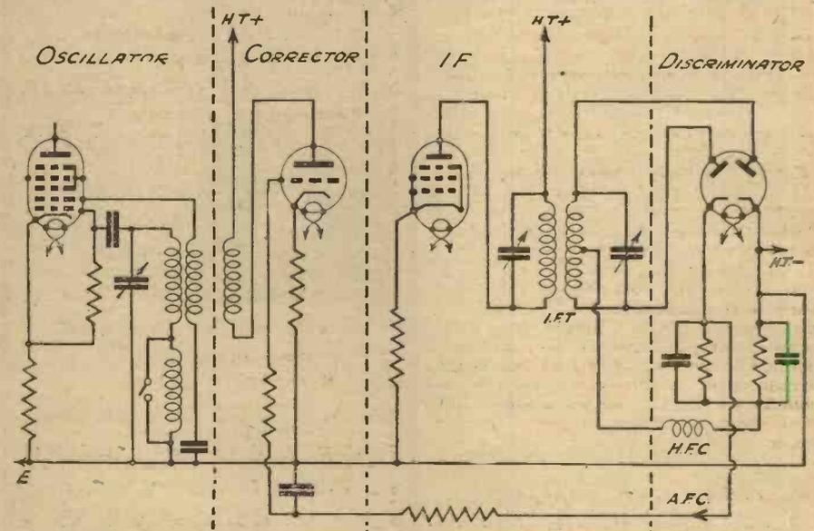
This skeleton diagram illustrates the principles described, and shows how the discriminator and corrector valves are connected.
