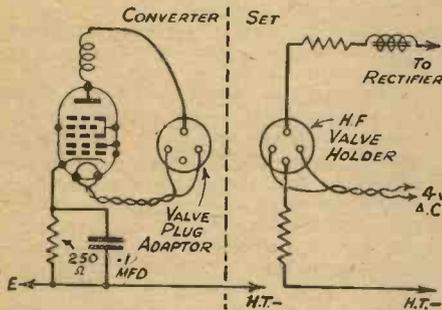
Fig. 4.—How an A.C. converter can be fed with H.T. and L.T. from most existing H.F.-type A.C. receivers.
