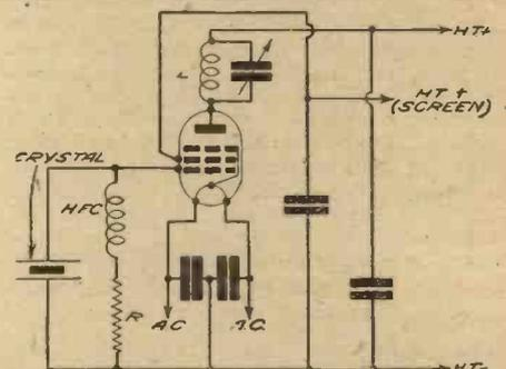
Fig. 2.—The fundamental circuit of a pentode C.O.
