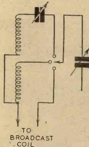
Fig. 5.—Efficiency on the ultra-short wavelengths may be increased by including a small capacity in series with the ultra-short-wave coil.
