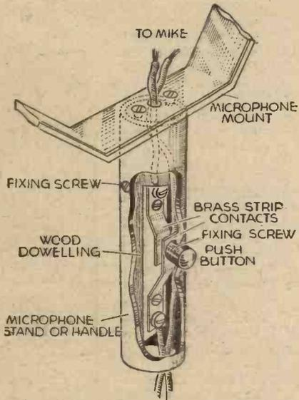
A safety-switch for a home-made microphone stand.
