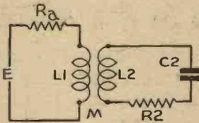
Fig. 16.—This diagram represents the theoretical equivalent of Fig. 14.
