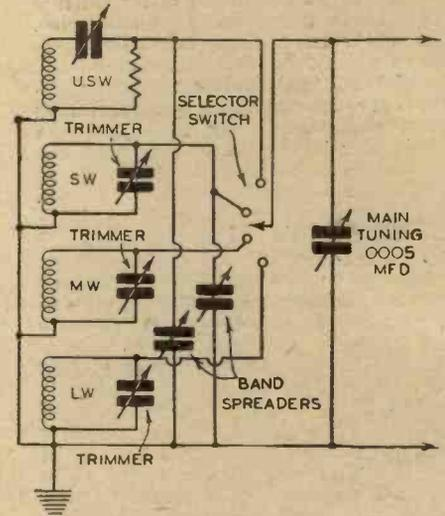
Fig. 7.—A comprehensive all-wave tuning circuit, showing how to incorporate all refinements as mentioned in this article.
