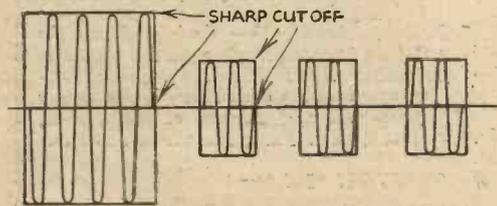
Fig. 2.—A distorted wave-form caused by sharp cut-off or sudden break in power circuit.
