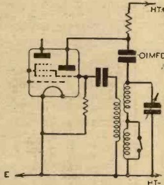
Fig. 7.—"Standard" connections for the oscillator coil used with a triode-hexode frequency-changer.
