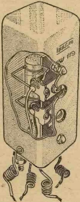
The H.F. transformer produced by Bulgin for use in television receivers
