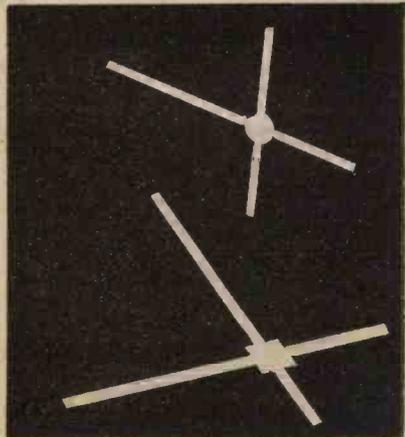
Fig. 2.—Wires which are connected or attached to each other are shown as above.
