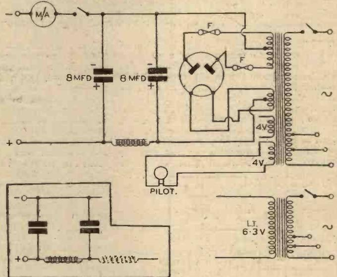
The three switches must be of the Q.M.B. type, and of a good make. I would suggest Bulgin, and this firm can also supply a very neat pilot light bracket and lamp holder, the lamp being wired across one of the 4-volt supplies of the Varley transformer, thus allowing it to indicate when the main supply is switched on, and when the rectifiers heater is alive.
