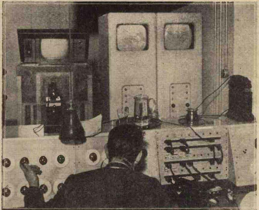
In the producer's control gallery. On the screens in the background appear the televised pictures as picked up by the three television cameras employed, one being transmitted. Through a large window on the right he can follow the performance in the studio.
