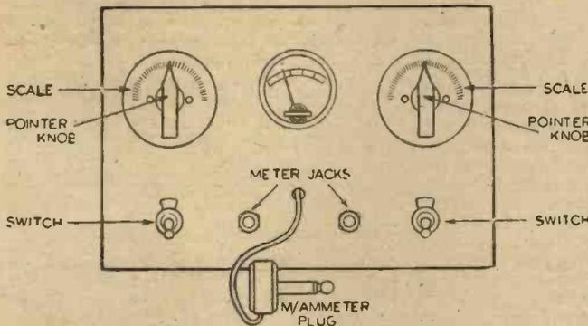
Fig. 6.—A suggested lay-out for the panel of the Tritet section. Keep the condensers below the centre line.
