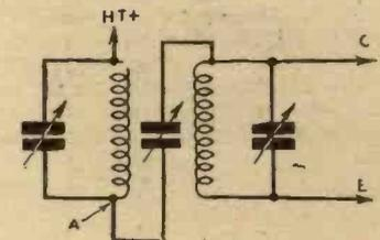
Fig. 10.—A simple means of obtaining variable selectivity by connecting a pre-set condenser between the high-potential ends of the I.F.T. windings.
