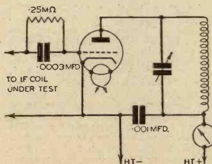
Fig. 2.—Circuit diagram of a test oscillator for checking the frequency of I.F. coils.
