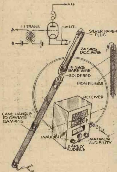
A novel tester rod for detecting resonance.
