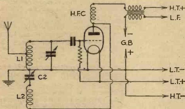
Fig. 1.—A typical cumulative grid detector circuit.
