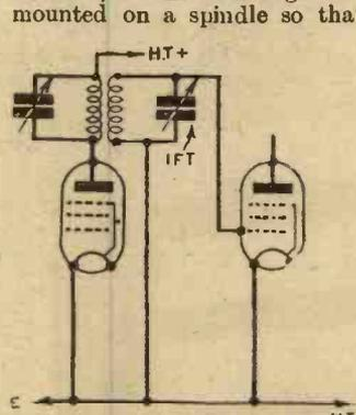
Fig. 8.—Usual connections for an untapped I.F. transformer.
