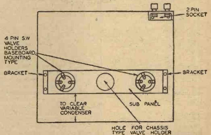
Fig. 7.—Showing the approximate position of the coil and valve platform. The two-pin socket and terminal strip is for H.T. supply.
