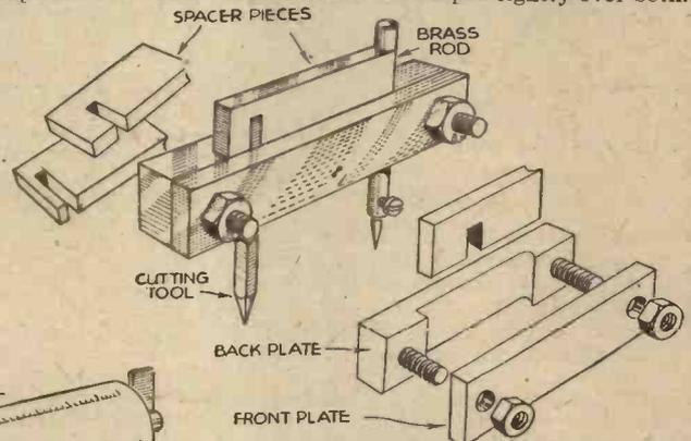
A handy tool for cutting circular holes in speaker baffles or chassis.
