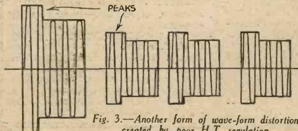
Fig. 3.—Another form of wave-form distortion created by poor H.T. regulation.
