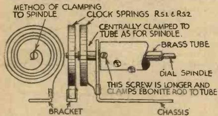
Fig. 2.—This diagram shows how the return spring is mounted on the spindle
