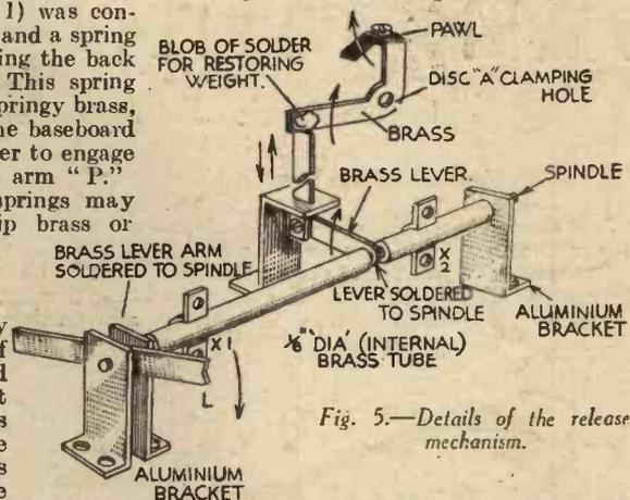
Fig. 5.—Details of the release mechanism.
