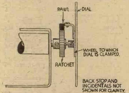
Fig. 3.—The ratchet device which provides the "locator."
