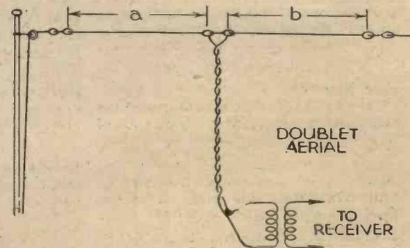
Fig. 3.—An efficient doublet aerial. Lengths a and b are equal to 1/4 wavelength depending on the waveband concerned.
