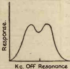
Fig. 18.—A double-humped response curve.
