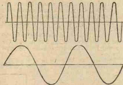
Fig. 1.—A train of continuous waves before modulation is applied. The lower curve represents an L.F. oscillation which will be used for modulating purposes.
