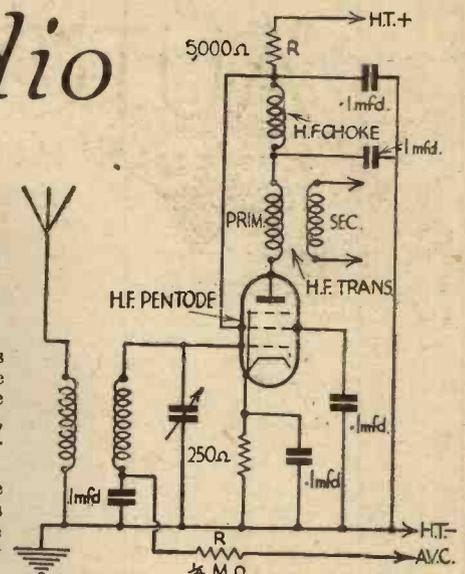
A typical circuit for an H.F. amplifier.
