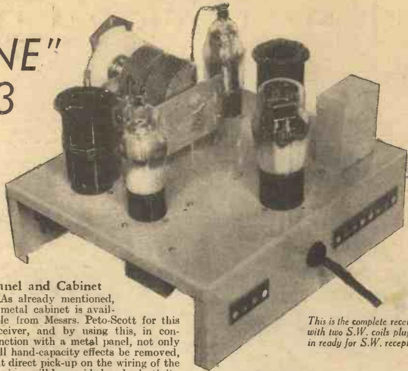
This is the complete receiver, with two S.W. coils plugged in ready for S.W. reception.
